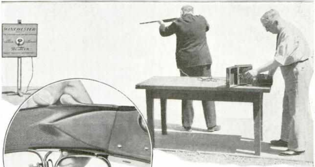
Using Electric Timer to Record Speed of Reaction to Firing Signal; Left, Timer Attached to Gun
