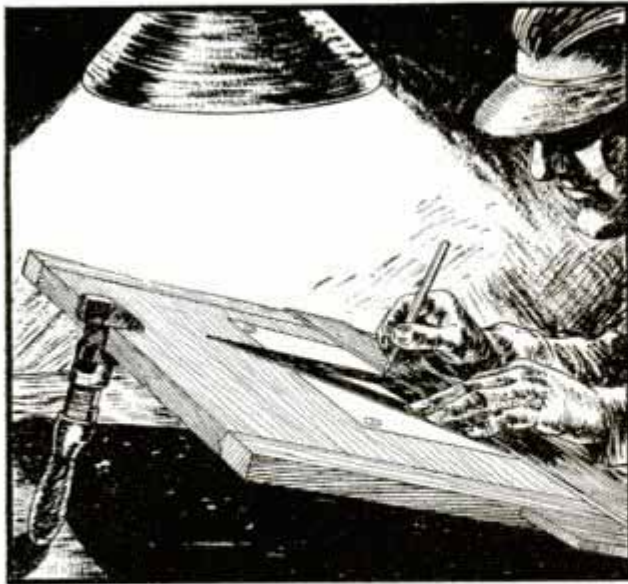
Monkey Wrench Clamped to Edge of Drawing Board Supports It at Angle on Bench Top
