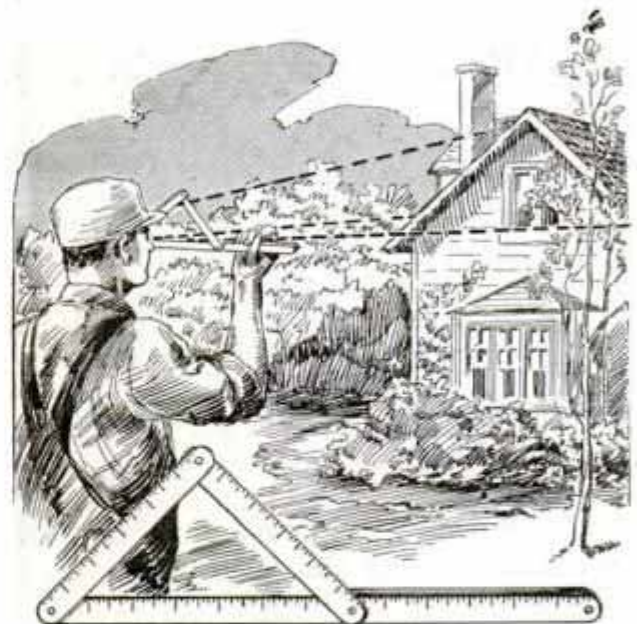
Pitch of a Roof Can Be Closely Estimated from the Ground by Using a Folding Rule
