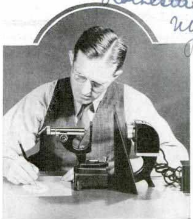
Tracing Microscope Specimen on Paper with Aid of Projector Which Throws Image on Notebook
