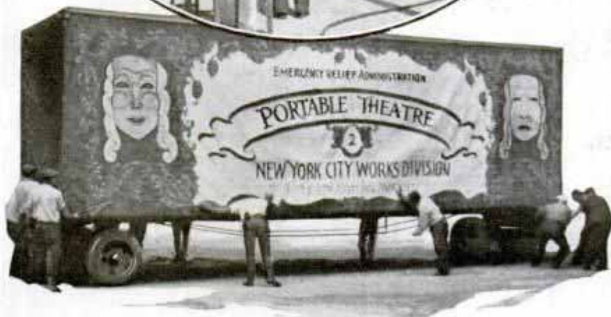
Stage of Portable Theater, Lowering One of Aprons, and the Theater on Wheels Ready to Travel; the Van Carries a Complete Stage and All Necessary Equipment
