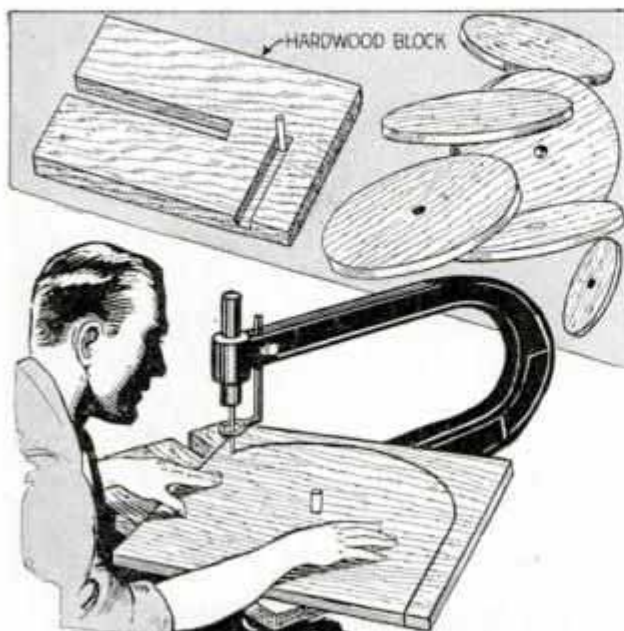
Attachment Enables You to Cut Accurately Disks with Radii from 2 to 24 In. on a Jig Saw
