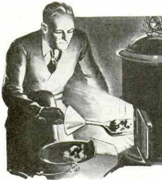
Large Funnel Slipped over Shovel Handle Protects Hand against Heat When Cleaning Stove Fire
