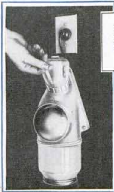
Above, Electric Coffee Grinder Solves Problem of Fresh Coffee; Its Top Container Holds One Pound of Bean Coffee and, Being Transparent, Indicates the Amount of Coffee on Hand; Grinding Unit Is Adjustable to Produce Coffee of the Fineness Desired; the Grounds Container Is Quickly Removable and Is Graduated in Per Cup Requirements; the Machine May Be Finished to Harmonize with Kitchen Decorations
