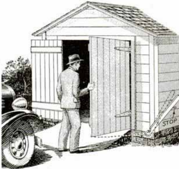
Notched Hardwood Strips Pivoted to Corners of Garage Hold Hinged Doors Open
