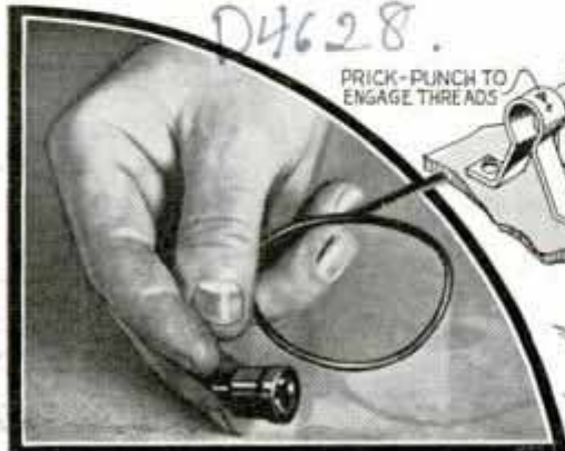
Insulated Tube Cap and Lead Makes Firm Contact and Is Easily Removed
