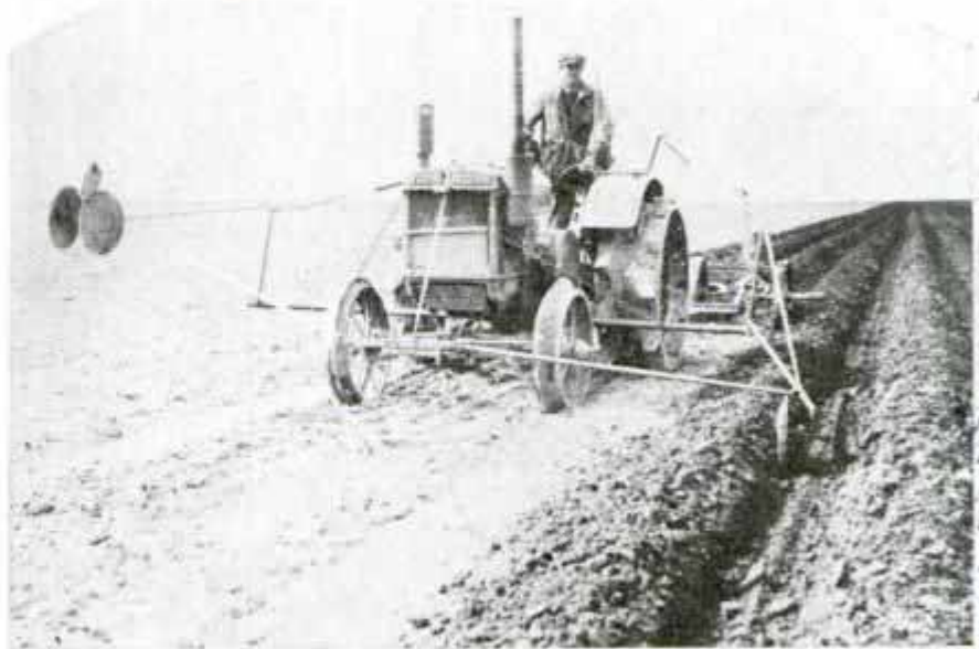
Tractor Guide Which Does Most of Work of Steering When Plowing; a Lever Lift Enables the Operator to Raise or Lower It Easily
