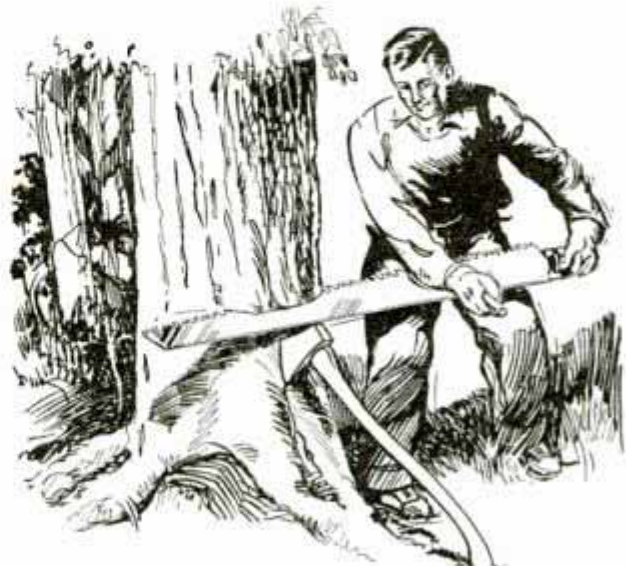
Single-Bit Ax Supports Blade of One-Man Saw While Starting the Cut to Fell a Tree
