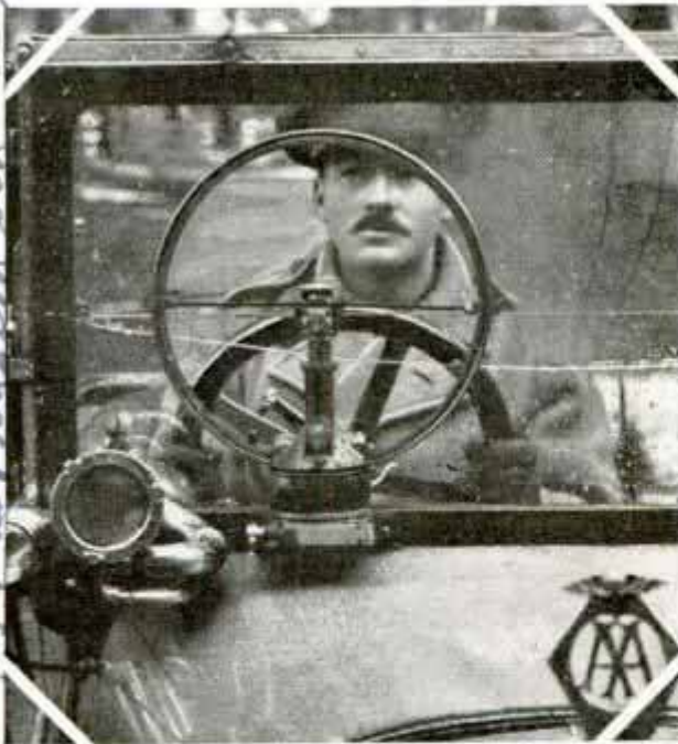
Bendis Animation Corp Chas Cory 754 Lexington Ave Revolving Disk on Windshield Operated by Electric Motor to Keep Off Rain and Snow
