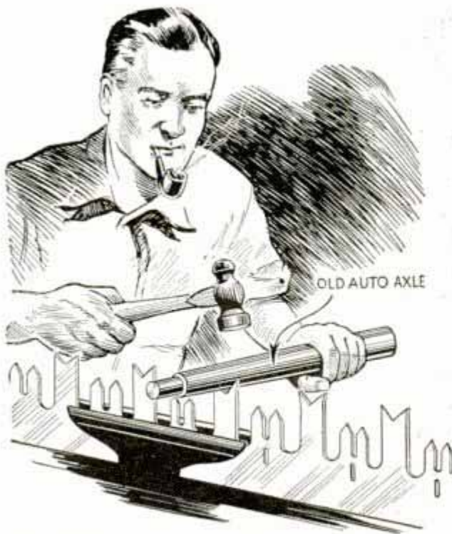
Using Old Auto Axle and Hammer to Spread Drag Teeth of Crosscut Saw
