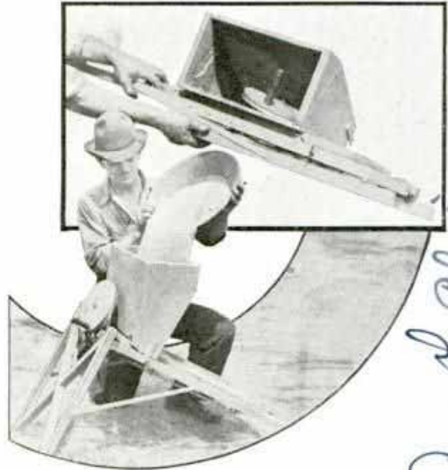
Collapsible Dry Gold Washer Which Is Capable of Handling One and One-Half Tons of Dirt per Day
