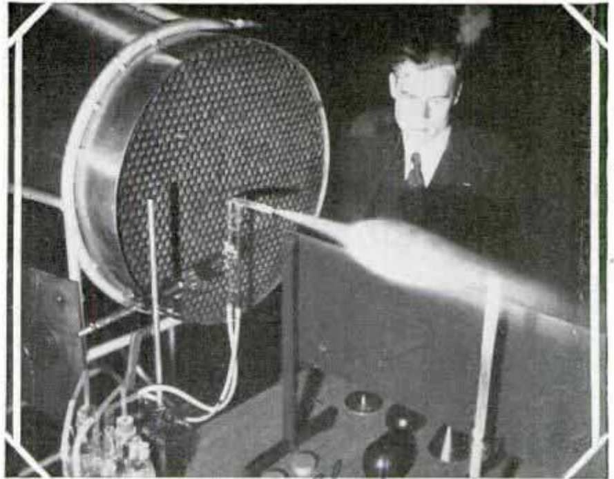
By Using Smoke in the Air Current, as Shown Above, the Effects of Streamlining Are Made Visible in Testing Models in the Laboratory
