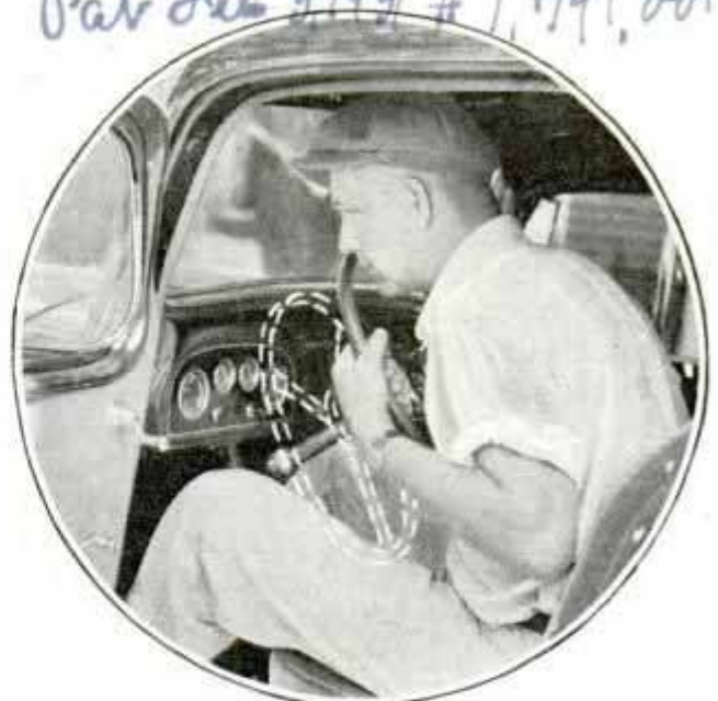
Driver Holding Collapsible Steering Wheel; Dotted Lines Show How Far Post Lowers
