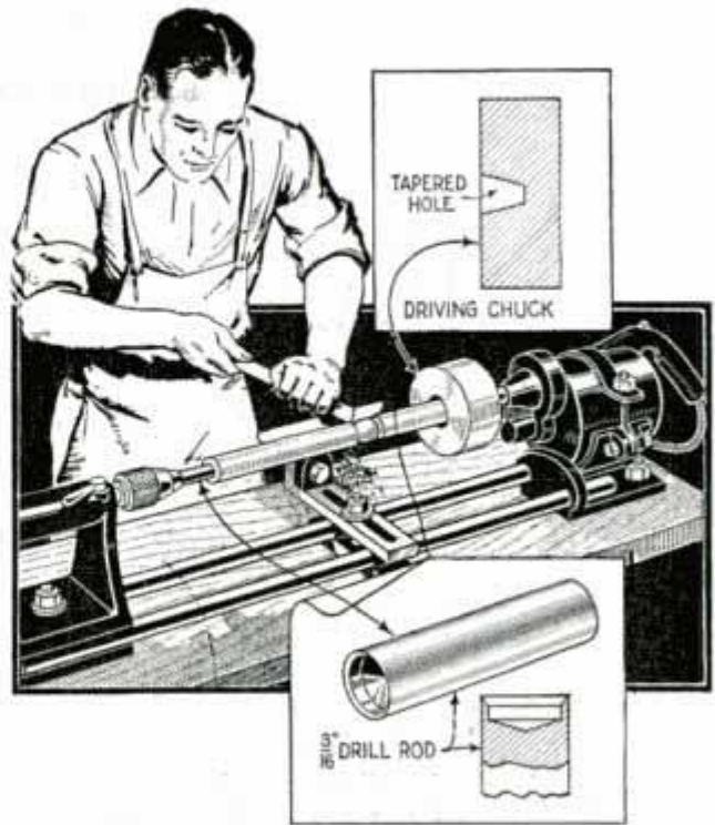
Chuck and Tailstock Center for Turning Small Work in Wood-Turning Lathe
