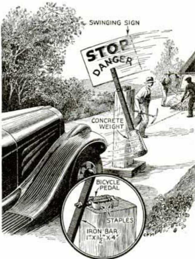
Swinging Sign at Street-Repair Job Attracts Motorists' Attention Quicker Than Stationary One
