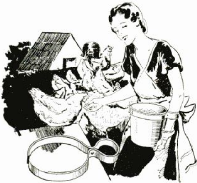
Band around Feed Bucket, with Loop for Arm, Holds Latter Conveniently for Scattering Contents
