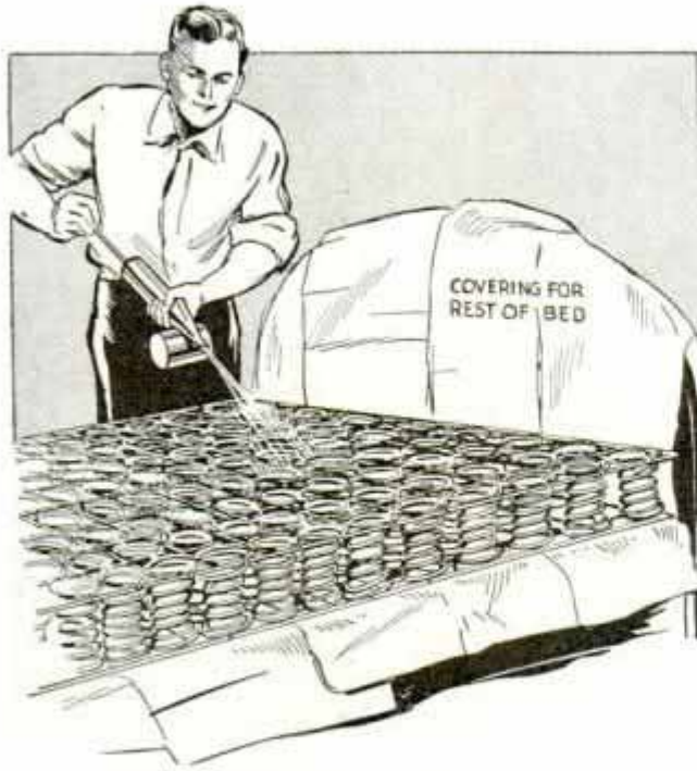
Mixture of Oil and Kerosene Sprayed on Bed Springs Eliminates Squeaks During Dry Weather
