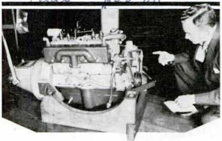
Model A Engine as It Appears Mounted for Use in Boat; Special Kit Facilitates Conversion of Motor to Marine Purposes
