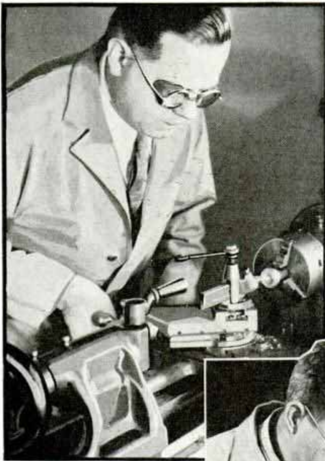
Above, It Pays to Protect Your Eyes from Small Flying Bits of Metal When Using a Lathe or Grinder; Right, Keep the Circular-Saw Table Clear and Hold the Work on Each Side of the Blade
