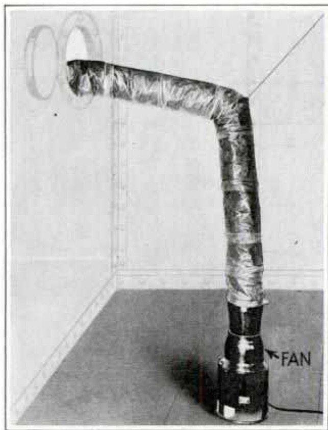
This Unit, with Arrow Pointing to Location of Fan, Removes Fumes at Rapid Rate
