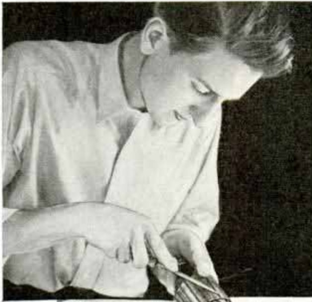
Armature slot is marked with a file
