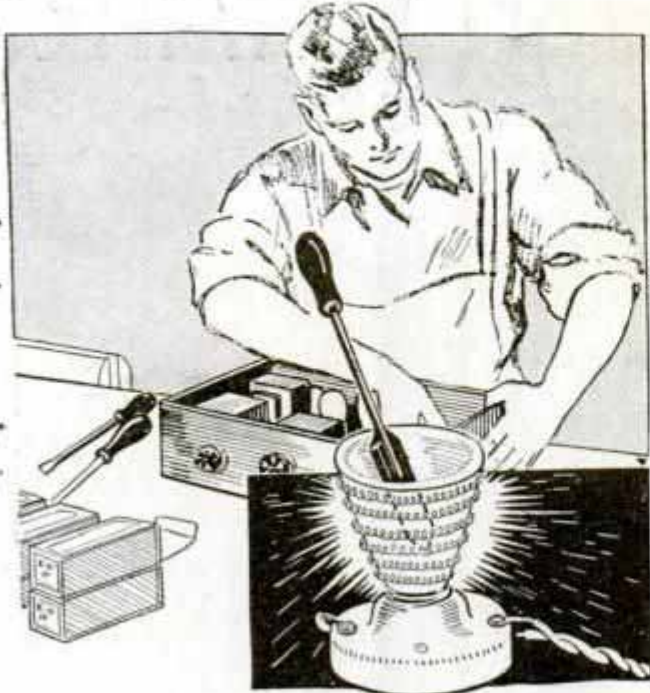
Radio Mechanic Heats His Small Soldering Iron with an Electric-Heater Element
