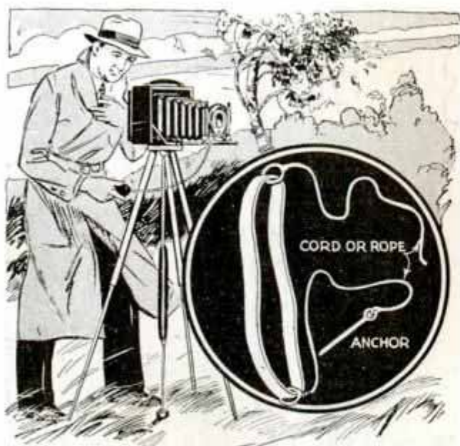
Anchor for Steadying Camera Tripod in Wind Made from Rubber Band, Cords and Wire Stake
