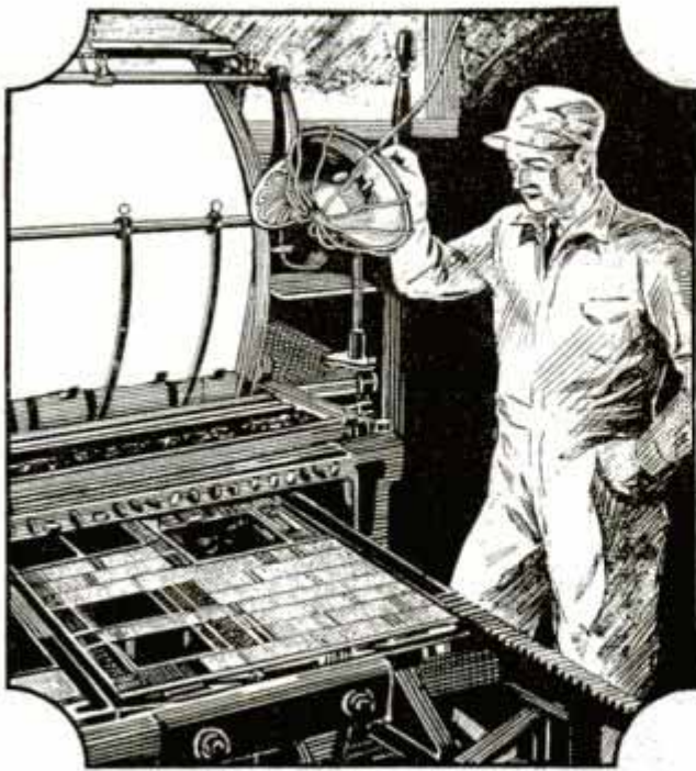
Electric Heater Warms Ink in Printing Press and Prevents Paper Sticking to Type
