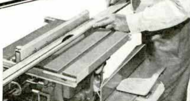
Upper Left, Upper Guide of Band Saw Is Adjusted to Just Clear the Work; Upper Right, Using a Push Stick When Ripping Off Narrow Strips
