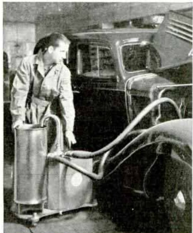
Pump Driven by Electric Motor Which Cleans Auto Radiator and Block Quickly and Efficiently
