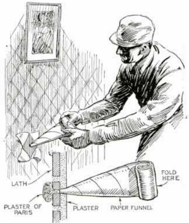
Loose Plaster on Wall Securely Anchored to Lath with Plaster of Paris
