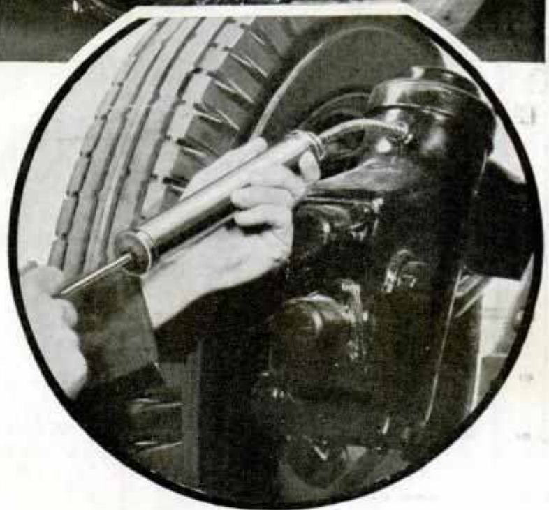
Top, Reaching Valves by Removing Plate under Fender; Bottom, Adding Fluid to Knee-Action Unit
