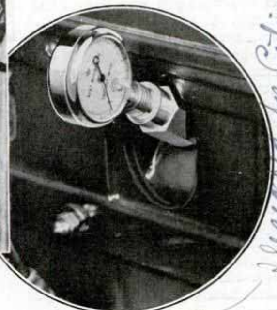
Compression Gauge, Shown in Place, Replaces Method of "Feeling" Resistance to Hand Cranking
