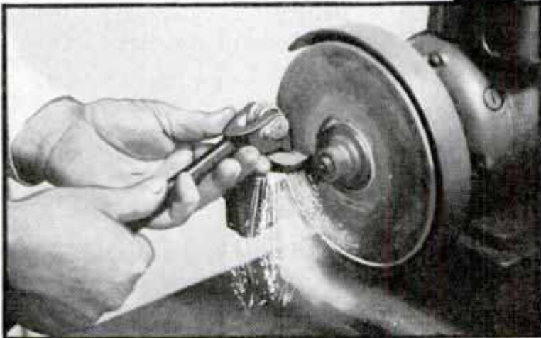
When Dressing Emery Wheels, Stand to One Side and Not Directly in Front of the Wheel
