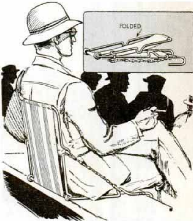
Made from Iron Rods and Canvas, This Portable Back Rest Folds into Compact Bundle
