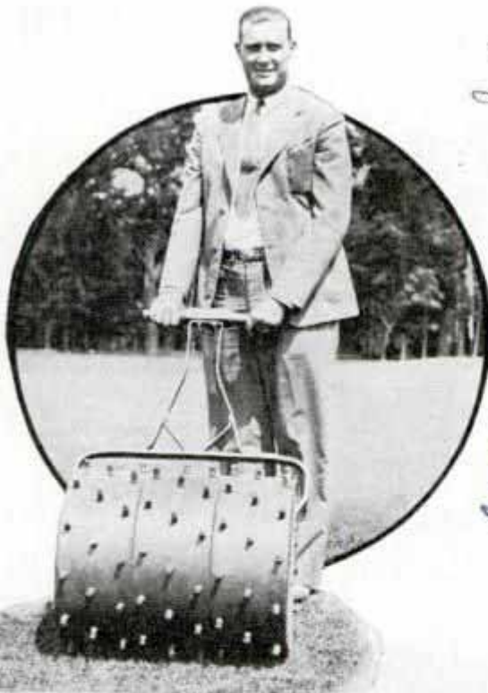
Roller with Spikes Cuts Small Holes in Lawn to Make Cultivation of Grass Easy
