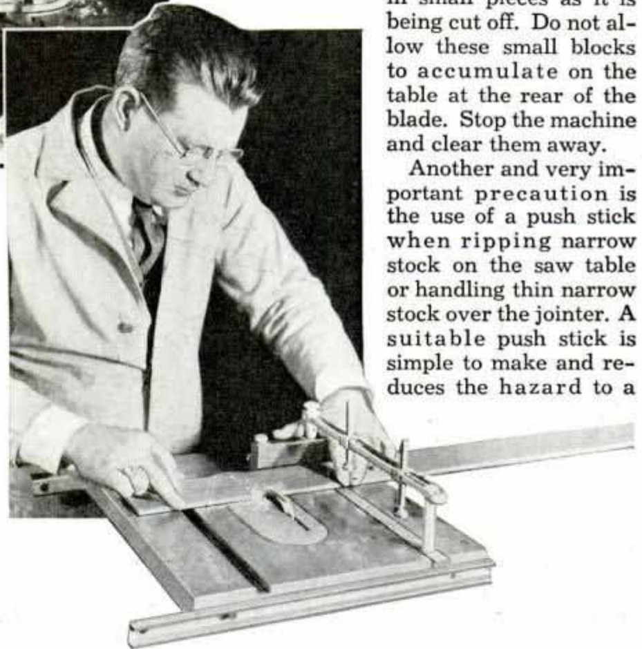
Above, It Pays to Protect Your Eyes from Small Flying Bits of Metal When Using a Lathe or Grinder; Right, Keep the Circular-Saw Table Clear and Hold the Work on Each Side of the Blade
