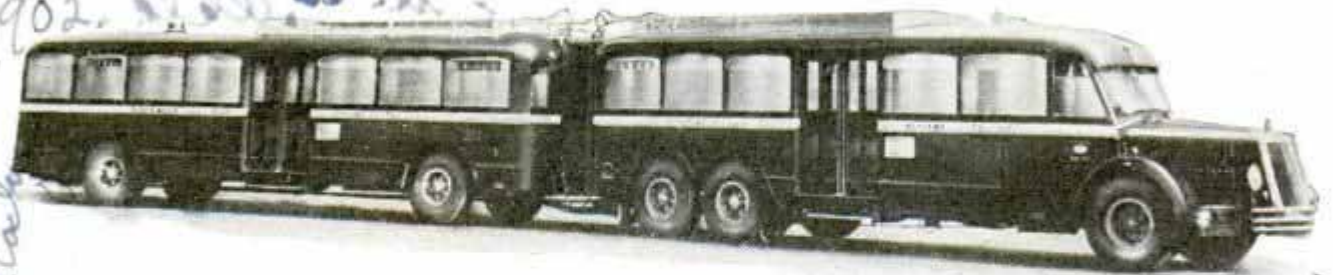
Articulated Motor Coach "Train" Consisting of Two Units Joined by a "Concertina" Gangway; Only the Front Unit Is Motorized and the Conveyance Is Used in the Italian Alps
