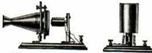
Telephone Transmitter and Receiver used at the Philadelphia Centennial
