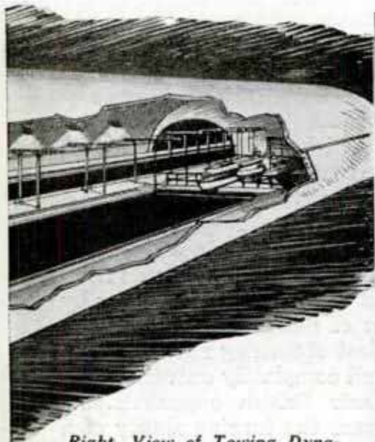
Right, View of Towing Dynamometer, Showing the Chronograph Drum Recorder
