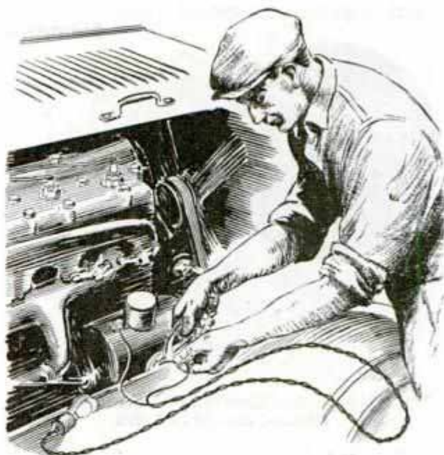
The "Live" Side of the Generator Cutout Is a Readily Accessible Place to Attach a Trouble Light
