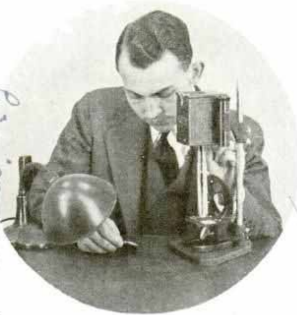
Combination Camera and Microscope Which Makes It Easy for Amateur to Make Microphotographs
