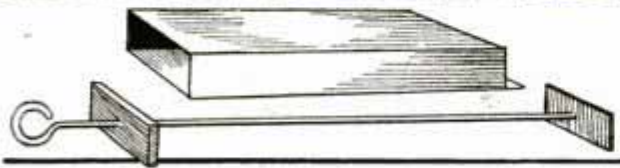
Soot Raked into Sheet-Metal Container That Fits into Cleaning Hole of Stove
