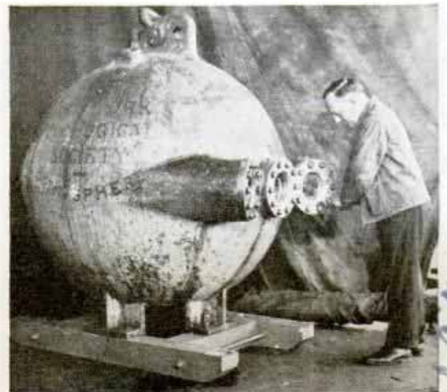
Dr. Beebe's Bathysphere, Showing the Windows Made of Fused Quartz Three Inches Thick
