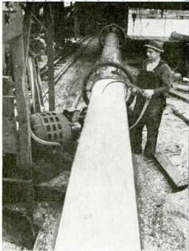
Big Lathe Running on Its Own Track and Converting a Big Tree into a Lofty Flagpole
