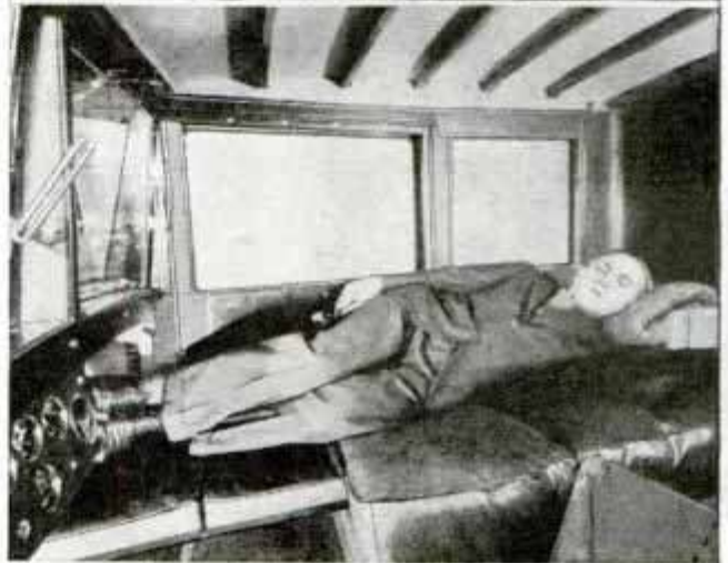
Adjustable Seat in Truck Cab Which Is Quickly Converted into a Comfortable Bed
