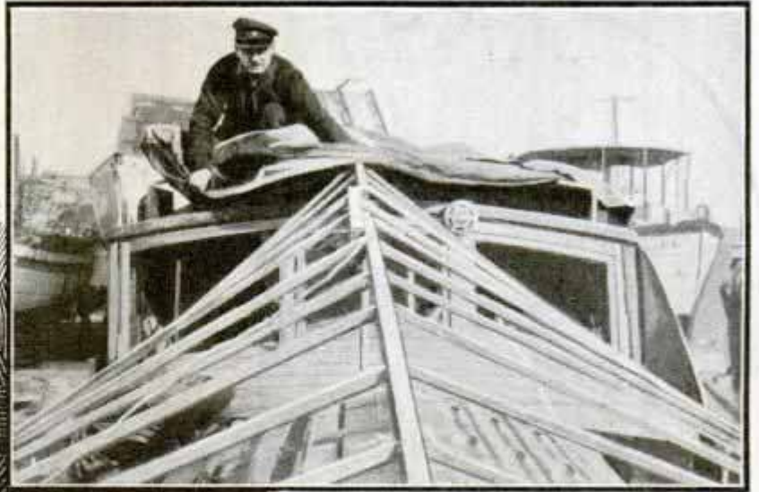
Left, a liberal application of oil on top of the pistons prevents rust inside the motor. Above, light wood frame holds tarpaulin off the upper surfaces of the boat
