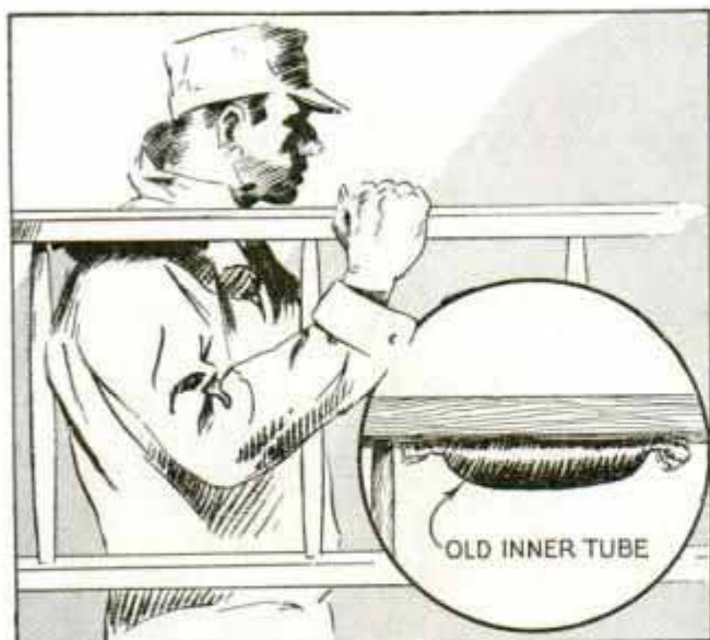
Section of Inner Tube Filled with Sawdust Makes Good Shoulder Pad for Carrying Ladder
