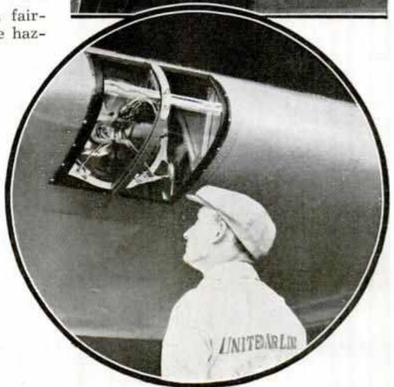
Above, Instrument Panel of Early Air-Mail Plane and Modern Ship; Below, Light Recessed in Mail-Plane Wing
