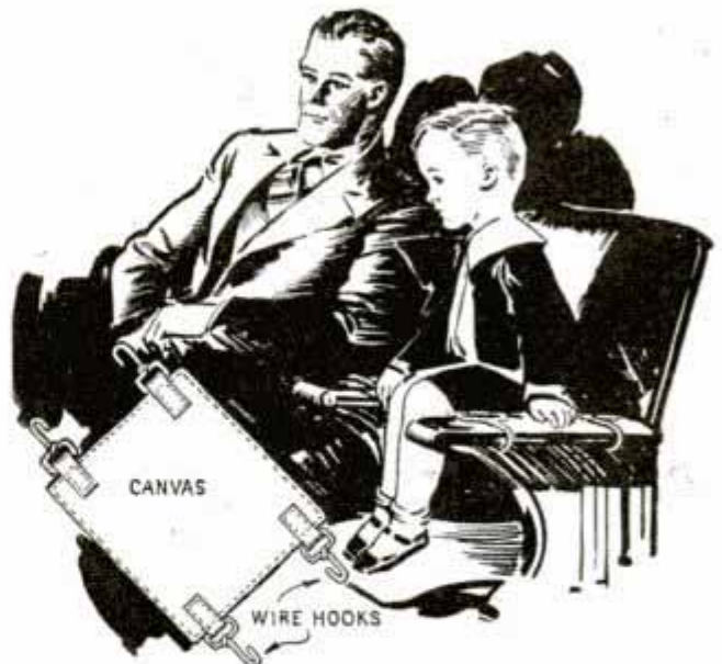
Heavy Canvas Seat Stretched between Arms of Theater Chair Enables Child to See Movies
