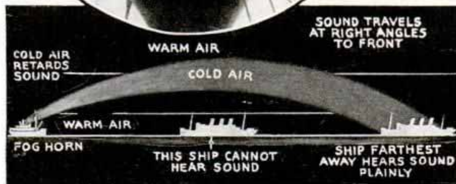
Lighthouse in Delaware Bay, Masthead Light of Lightship and Diagram Showing How Differences in Air Temperature Distort Sound
