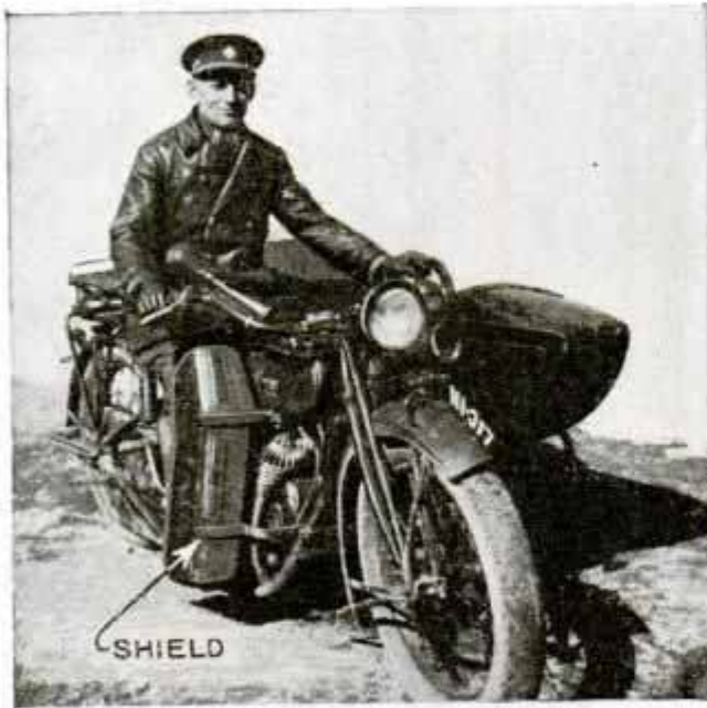
Leg Shields Clamped to Frame of Motorcycle Protect Rider from High Winds and Storms
