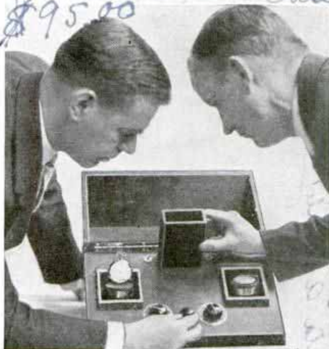
Instrument Which Tells in One Minute Whether a Watch Is Gaining or Losing Time and How Much
