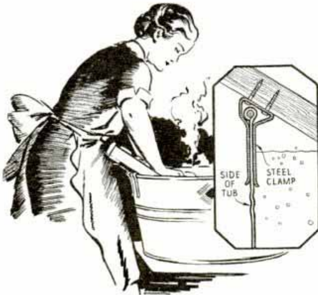
Washboard Held in Tub with Clamps Reduces Back Strain When Rubbing Clothes
