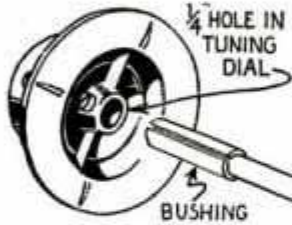
Left, Brass Strip Makes Reducing Bushing for Standard Dial; Right, Screwdriver with Spring Screw Grippers for Awkward Places
