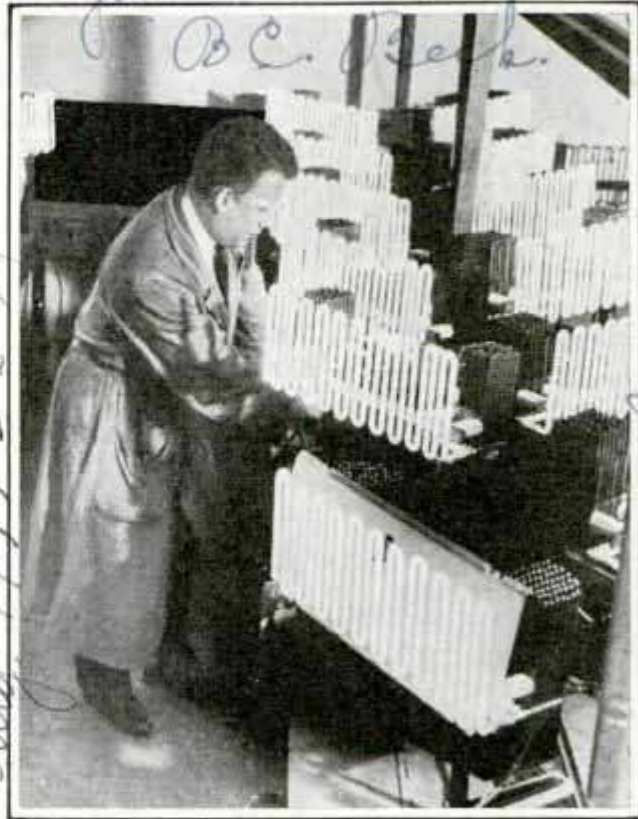
Several Sets of "Daylight" Tube Lamps under Test Before Being Installed in Cabinets
