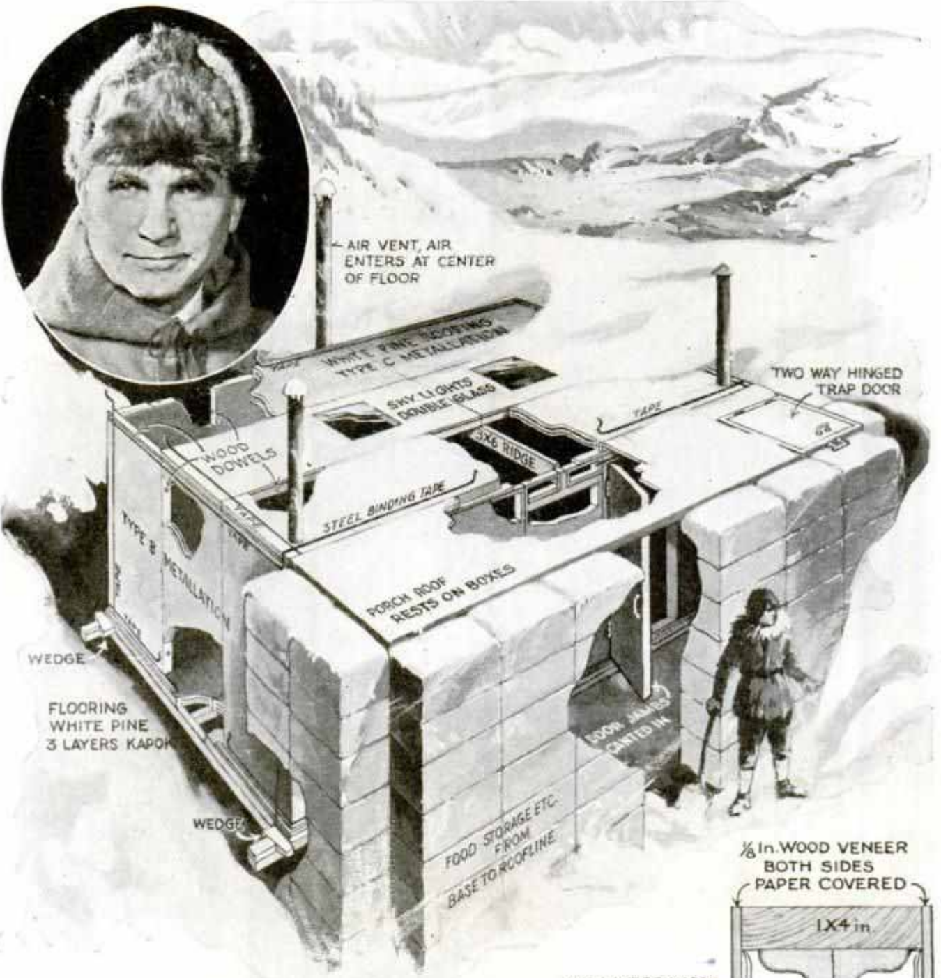
Sectional Drawing of Admiral Byrd's Antarctic Hut; Inset (Top), Victor H. Czegka, Designer of Hut; Bottom, Method of Insulation
