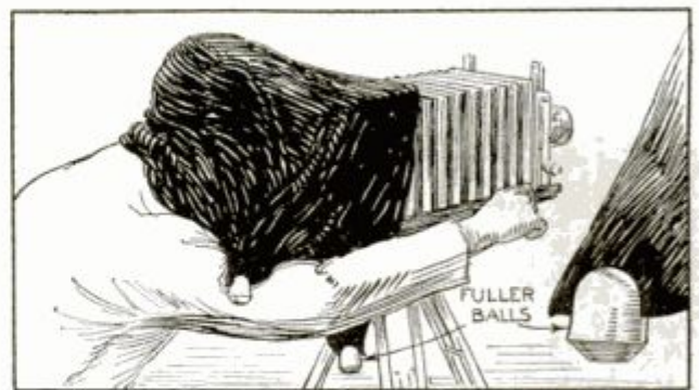
Fuller Balls Attached to Corners of Focusing Cloth Hold It Down in Wind
