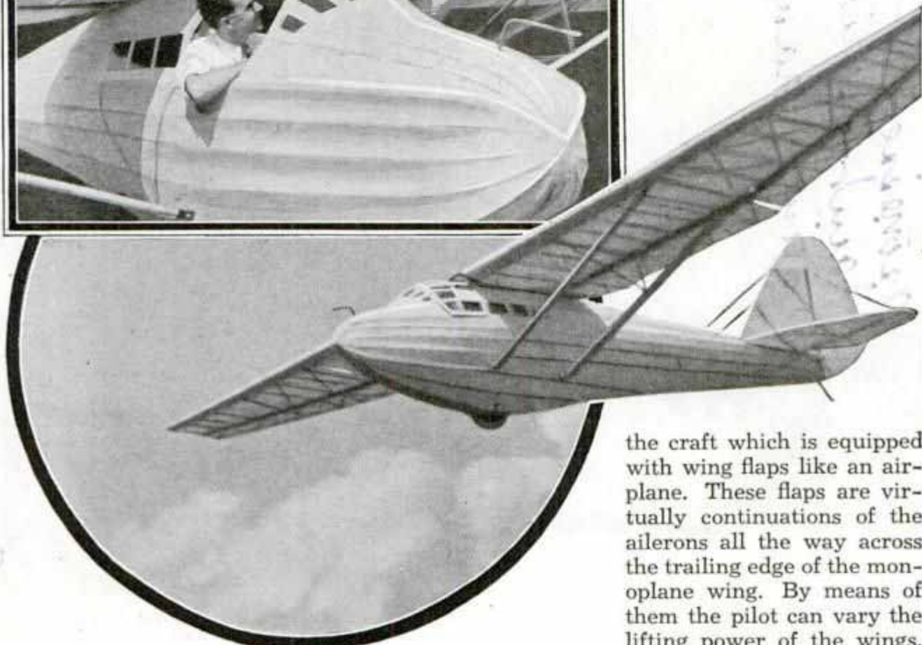
Four-Passenger Glider Which Is Equipped with Wing Flaps to Regulate the Lifting Power; It also Has an Adjustable Stabilizer; Note the Single Landing Wheel
