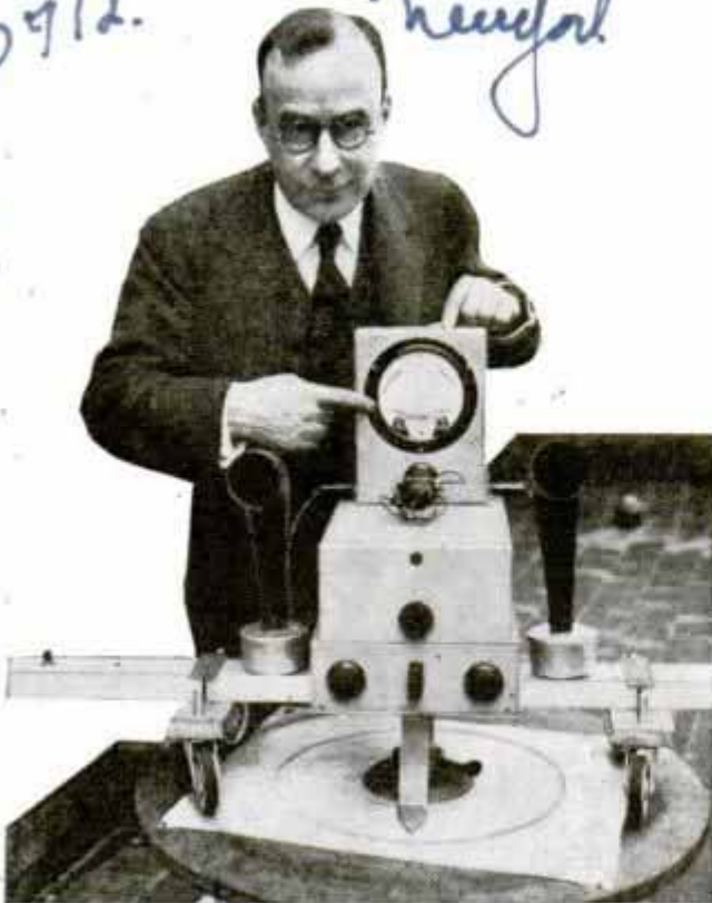
Range Finder for Boats Which Records Distance as Well as Direction of a Radio Signal
