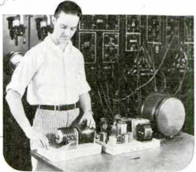
Disks on Cylinder Ready to Reproduce Tones of Pipe Organ When Proper Keys Are Touched
