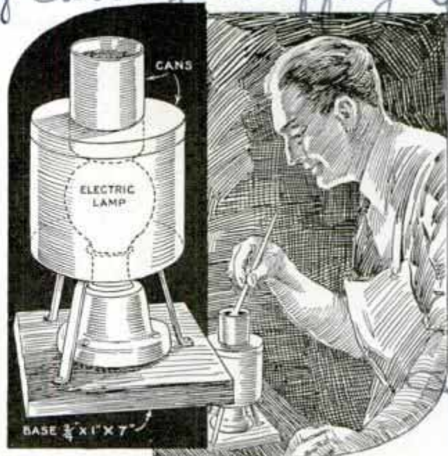
This Gluepot Is Operated by an Electric Bulb and Boils Glue Quickly
