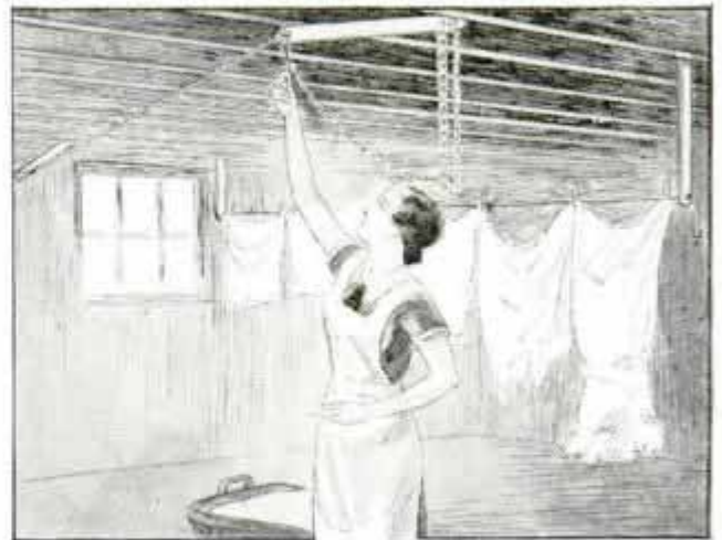
Clothesline in Basement Pivoted to Floor Joist Swings Out of Way When Not in Use
