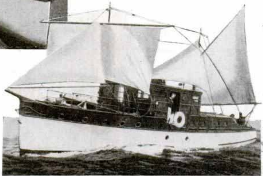
Combination Power and Sail Cruiser Built in the Designer's Backyard; the 150-Horsepower Engine Develops Twenty Miles per Hour
