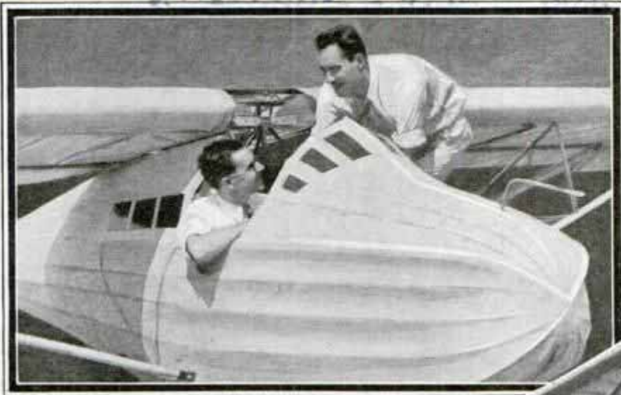
Four-Passenger Glider Which Is Equipped with Wing Flaps to Regulate the Lifting Power; It also Has an Adjustable Stabilizer; Note the Single Landing Wheel
