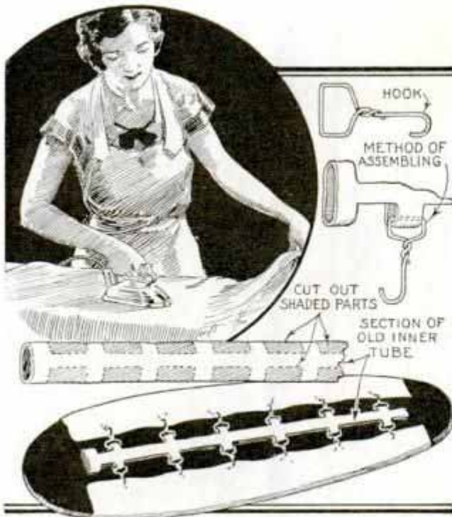
Inner Tube Cut to Shape and Fitted with Hooks Holds Pad on Ironing Board
