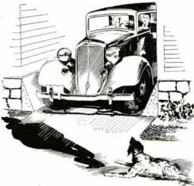
Curbs on Narrow Driveways Beveled with Concrete Prevent Fenders from Scraping Sides of Buildings
