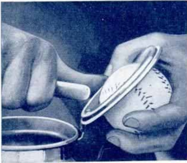
Lip Holding Glass Top in Percolator Lid Repaired with Knife and Baseball
