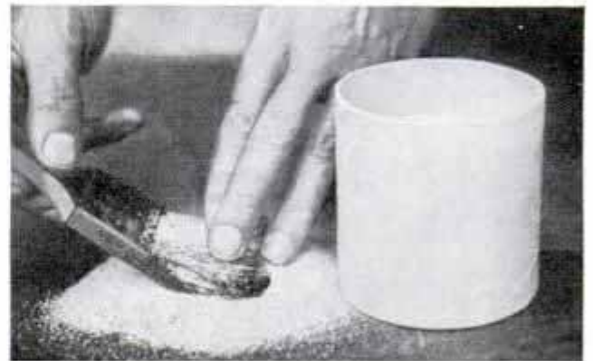
Paint and Varnish Removed from Brushes by Working Sand in between Bristles
