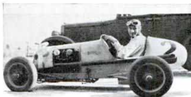
Small Auto Built Mostly of Junked Parts Reaches Speeds above 100 Miles per Hour
