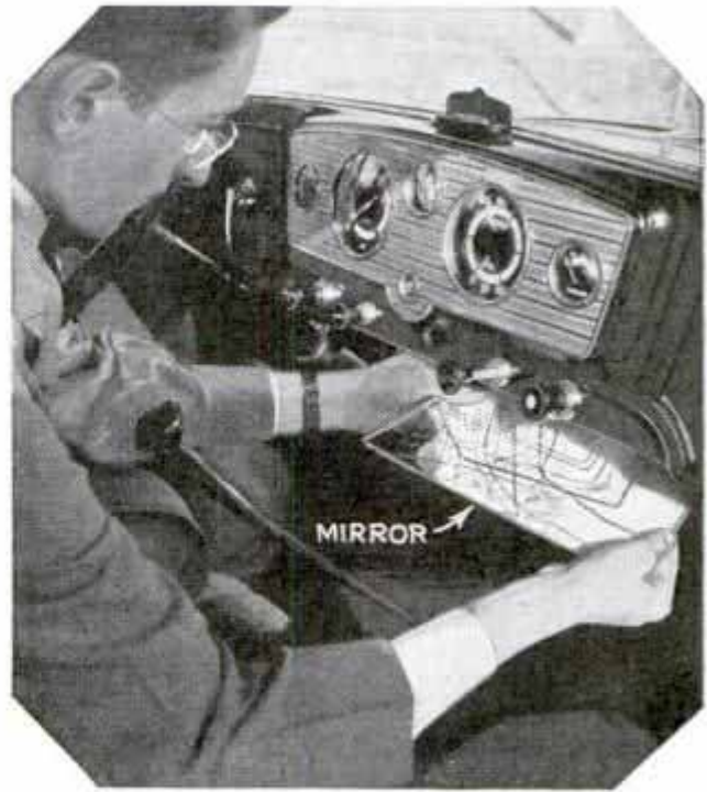
Mirror Held under Instrument Panel Reflects Wires and Connections So They Are Easily Examined
