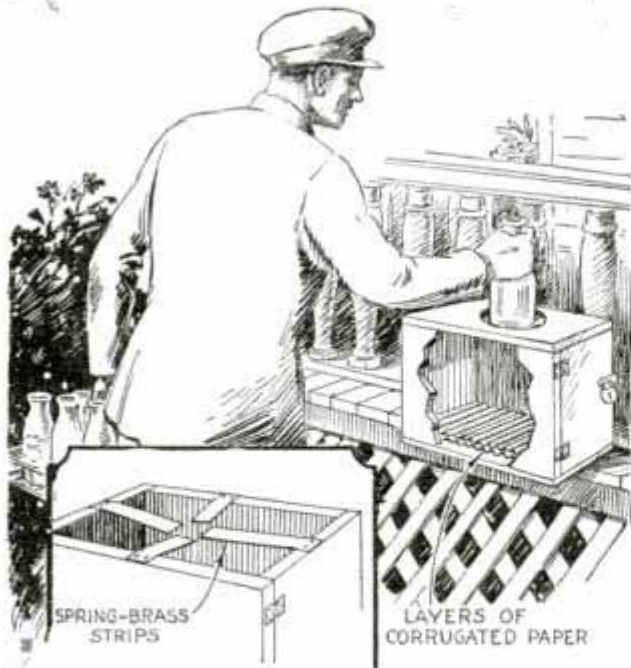
Milk-Delivery Box Permits Bottles to Be Inserted Easily but Hard to Remove
