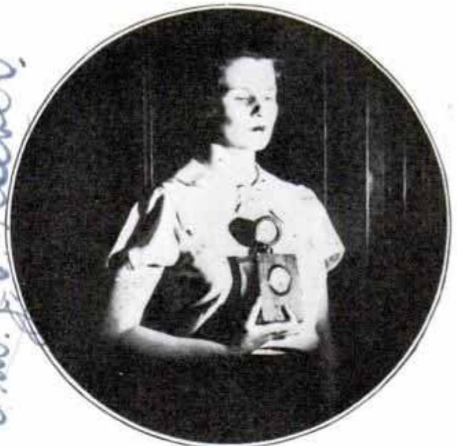
Buzzer Signal Box, Shown in Hand, Guides Blind Person through an Entire Building
