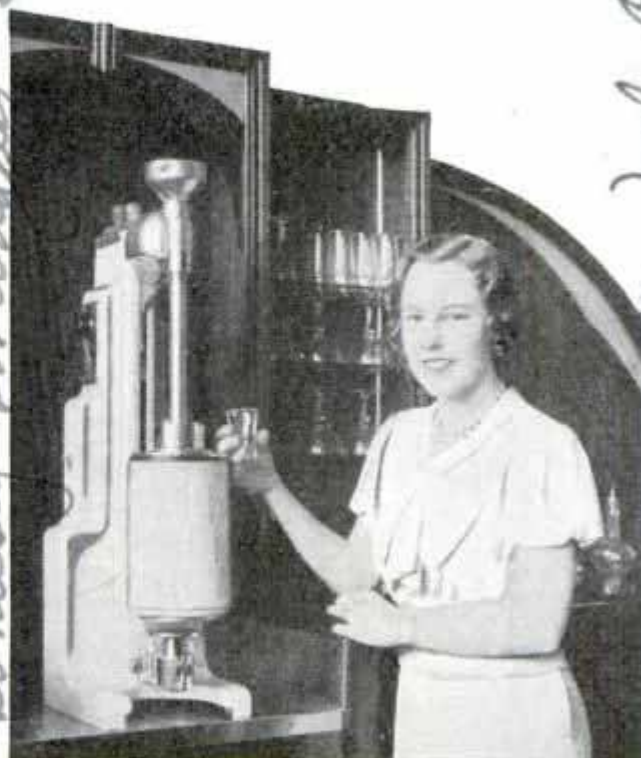
Freezer for Store Counter Which Makes Frozen Drinks or Ice Cream in Less Than a Minute
