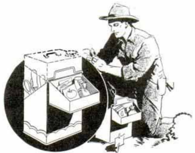
Handy Carrier for Small Garden Tools and Seeds Made from Discarded Square Can
