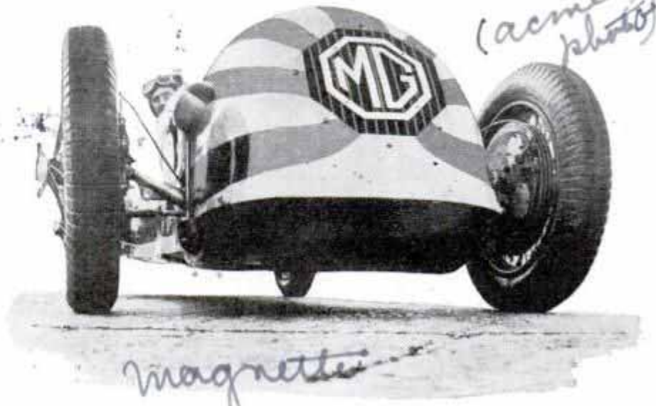
Front of Racer Constructed along Aerodynamic Lines; Note Unusual Nose of Car; Built Low, It Rounds Curves at High Speed
