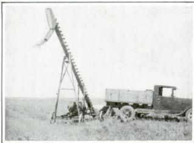
Weed Seed Blown Away from Threshed Wheat by Elevating It Outdoors in the Wind
