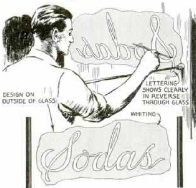
Window Signs Lettered in Reverse by Tracing Design in Coating on Outside of Glass
