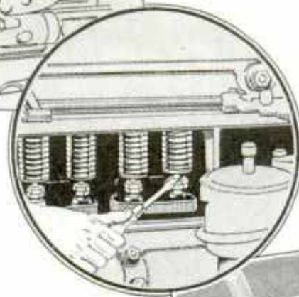
Above, Using Paper Strips to Locate Noisy Tappets; Center, Tip of Screwdriver Blade Carefully Inserted between Tappet and Valve Stem to Find Loose Camshaft Bearing; Right, Cylinder Wall Scored by Broken Piston Ring
