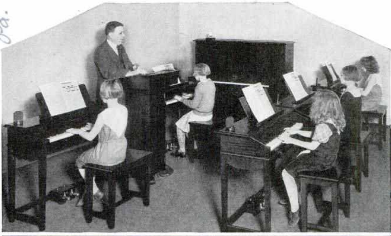
Standard Electric Piano with Remote-Control Keyboards for Group Instruction; Students Do Not Know Which Instrument Is Actuating the Master Piano at Any Instant
