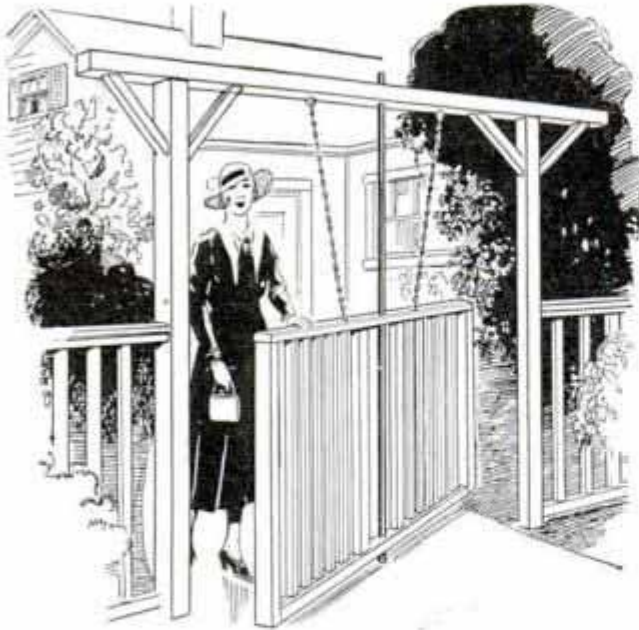
Gate Pivoted on Pipe Standard Is Supported by Chains Fastened to a Crossbeam Above
