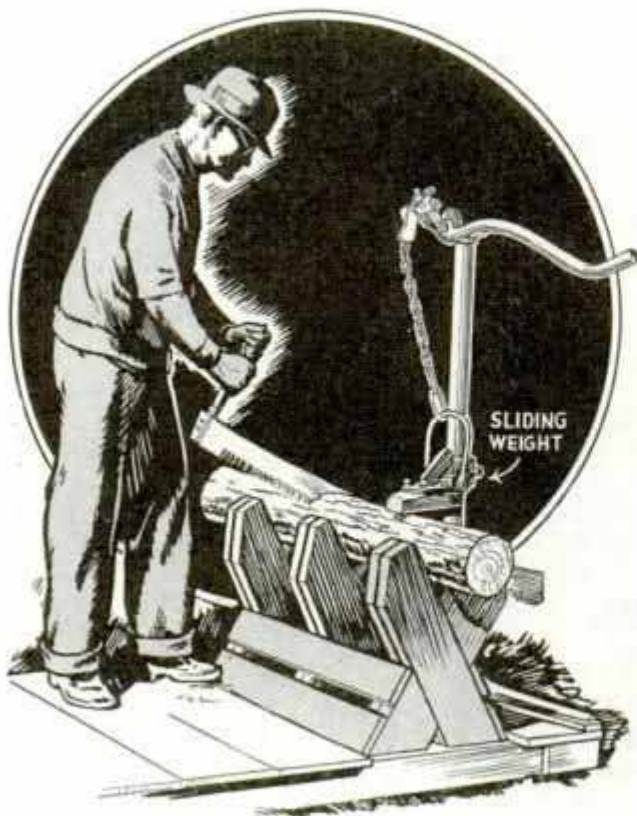
Clamp on Sawbuck Aids in Sawing Logs into Lengths Suitable for a Stove
