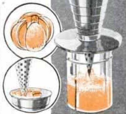
Above, Combined Juice Extractor and Strainer Does the Work in Half the Time and Saves About Ten Per Cent of Juice Lost by Similar Devices; Illustrations Show Simplicity of Operation; Left, Hot-Water Tank Is Heated with Radiator Alcohol; the Fuel Tank, When Filled, Heats Full Tank of Water to Almost Boiling Point; When Half Tank of Water Is Required, the Fuel Container Is Filled Only Half Full; When Fuel Is Exhausted, the Burner Stops without Attention or Danger
