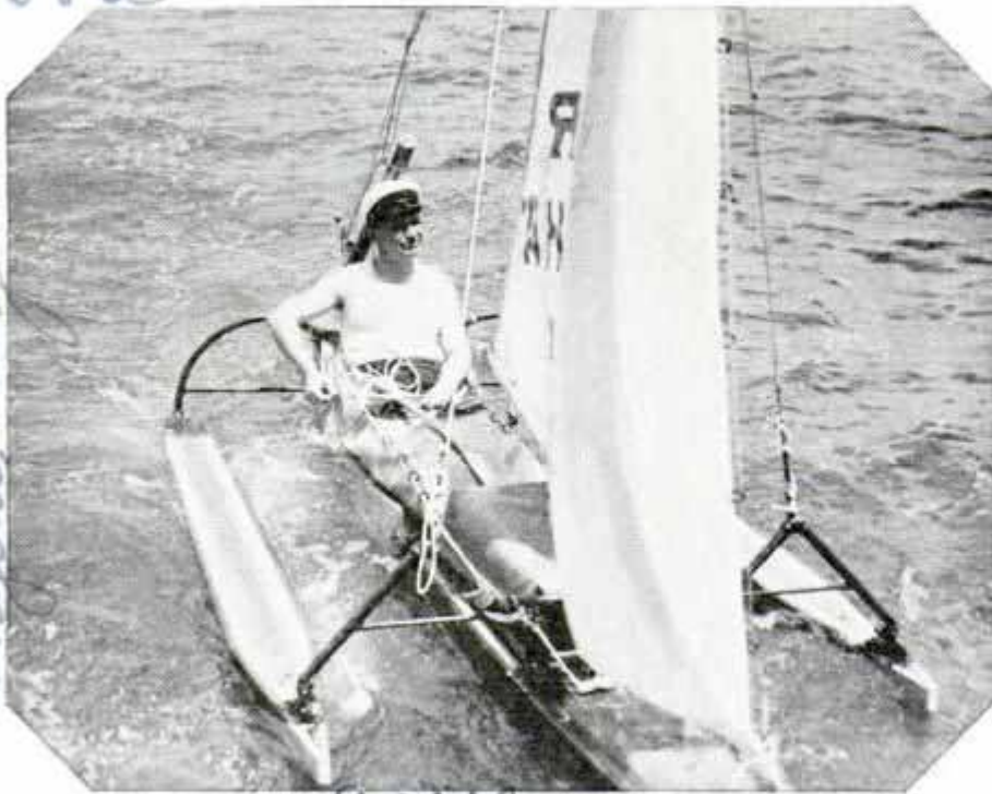
Acme Small Craft Used for Ocean Voyage; It Is a Fourteen-Foot Paddle Board with Eight-Foot Outriggers and Fifty Square Feet of Canvas
