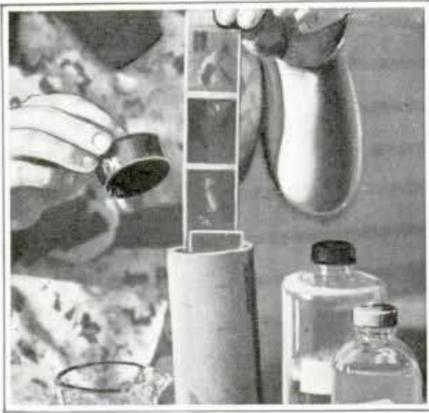
Section of Radiator Hose Plugged at the Ends Is Used as a Film-Developing Tank
