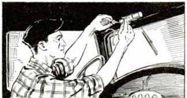
Windshield Wiper Lubricated by Working Blade While Oil Is Squirted into Intake Pipe
