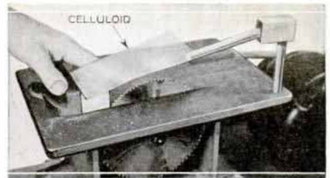
Celluloid Guard to Protect Eyes When Cutting Metal on Circular Saw
