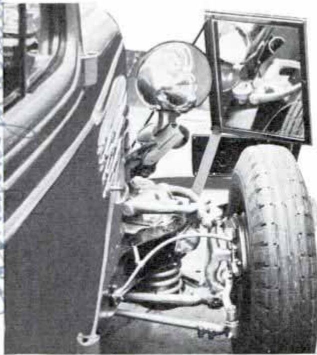
Movements of Wheel Mounting Are Reflected to Passenger's Eye by Mirror above Wheel
