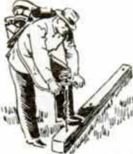
Small Gas Engine Carried on the Back Like a Knapsack Has Attachments for Doing Various Kinds of Cutting and Sawing
