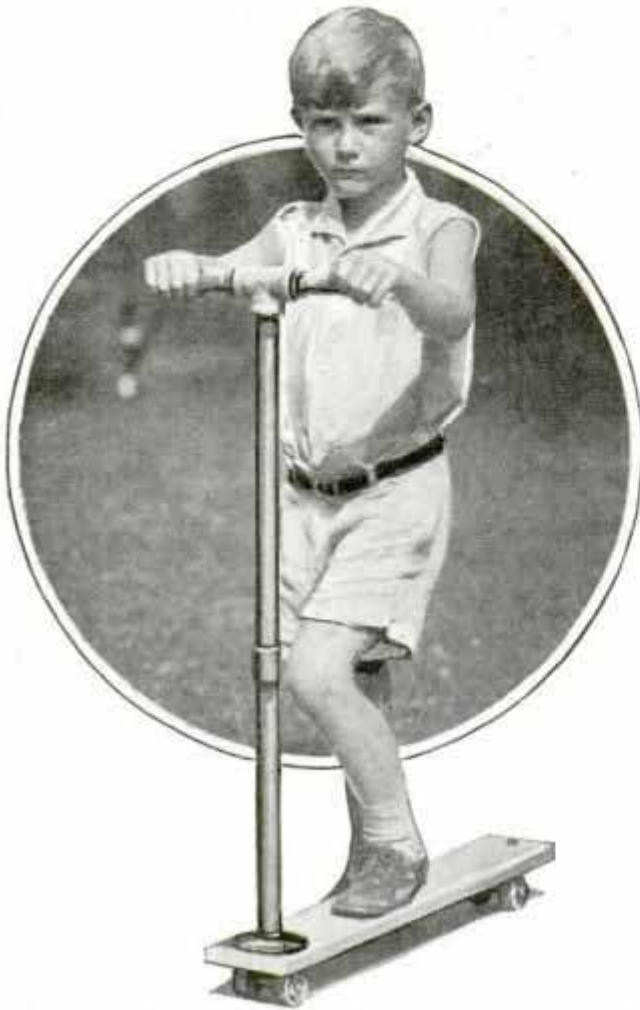
Utilizing Skate Rollers as Wheels, This Scooter Has a Steering Column of Pipe
