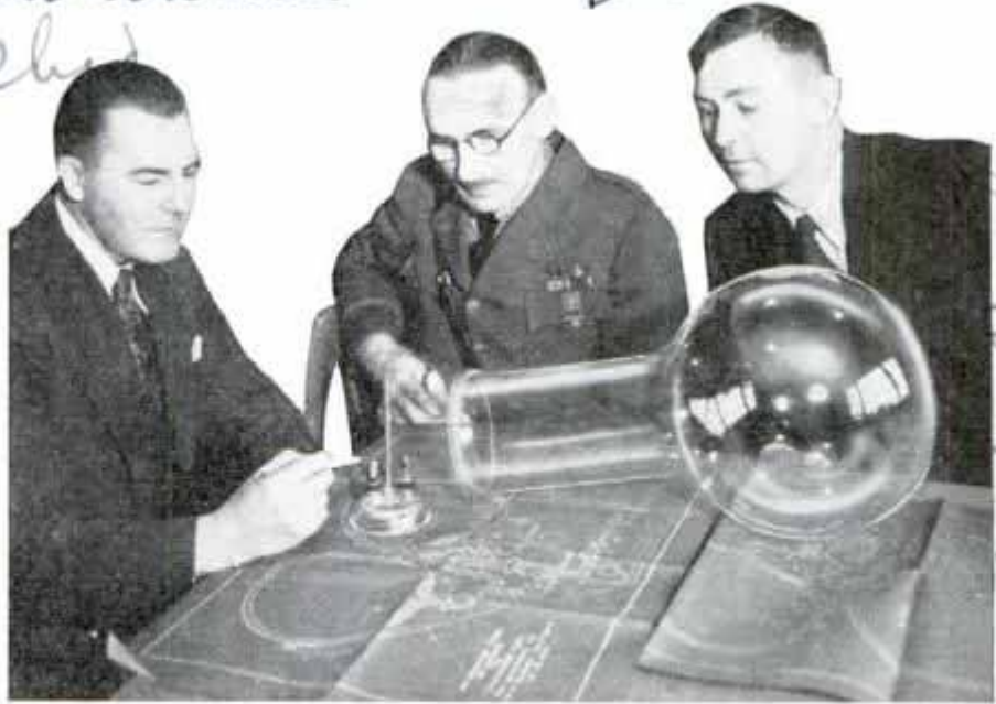
Giant Bulb Designed for Stratosphere Flight; Base Contains Valves for Capturing Samples of the Upper Air
