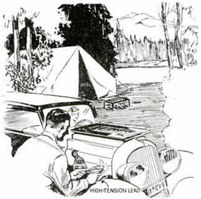
Small Gasoline Torch Lighted by Hot Spark from Ignition System of Car
