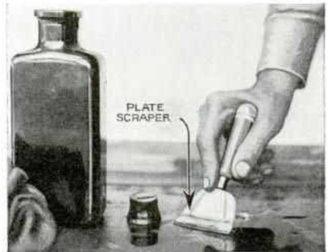
Rubber Plate Scraper for Applying Cleaning Solutions to Surfaces Before Painting Them
