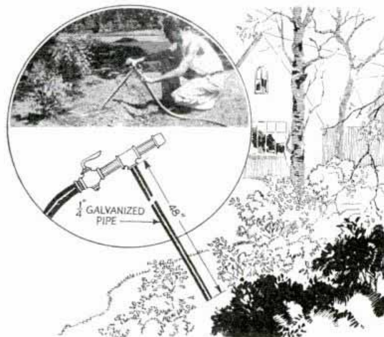
Water Injected around Roots of Trees and Shrubs with "Needle" Protects Them from Drouth
