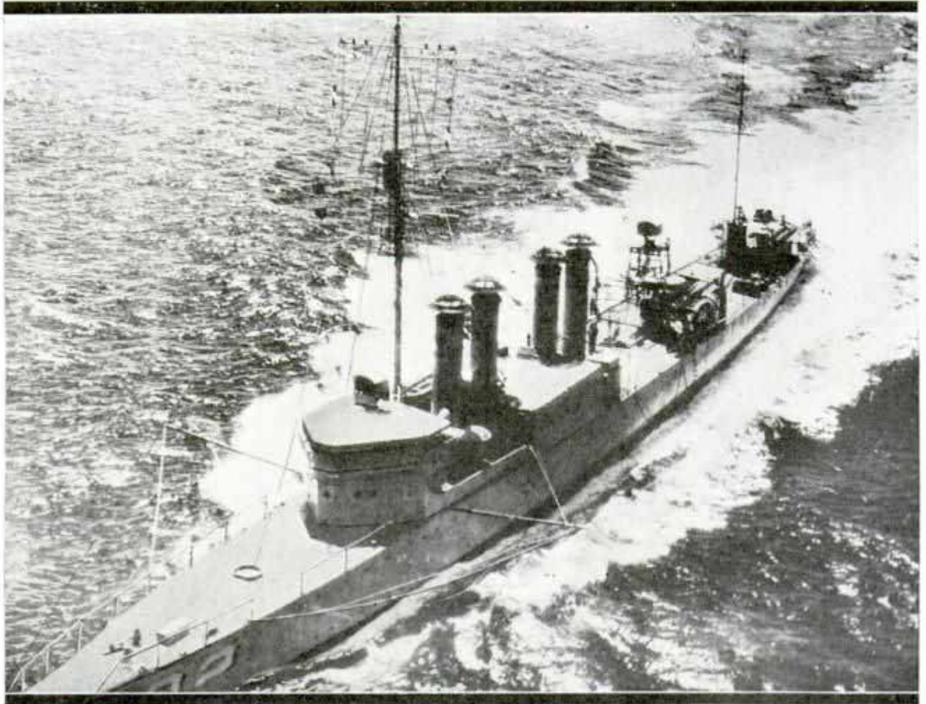
Air View of the Robot Ship at Sea Showing the Deserted Decks; the Vessel Controlling the Ship by Radio Is Far in the Rear but the Robot Responds to Every Command
