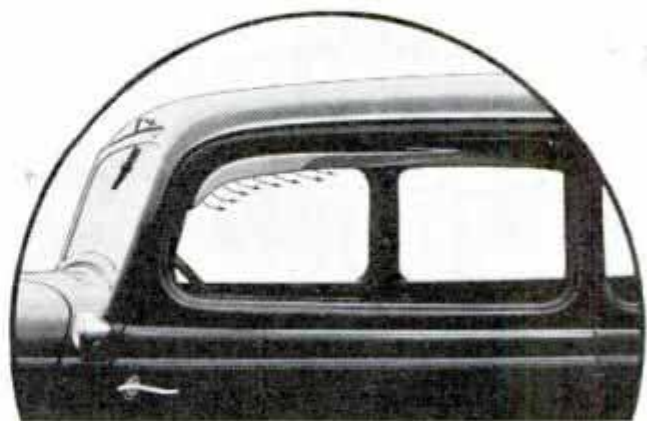
Ventilator for Top of Car Window Which Maintains Air Circulation but Keeps Out the Rain
