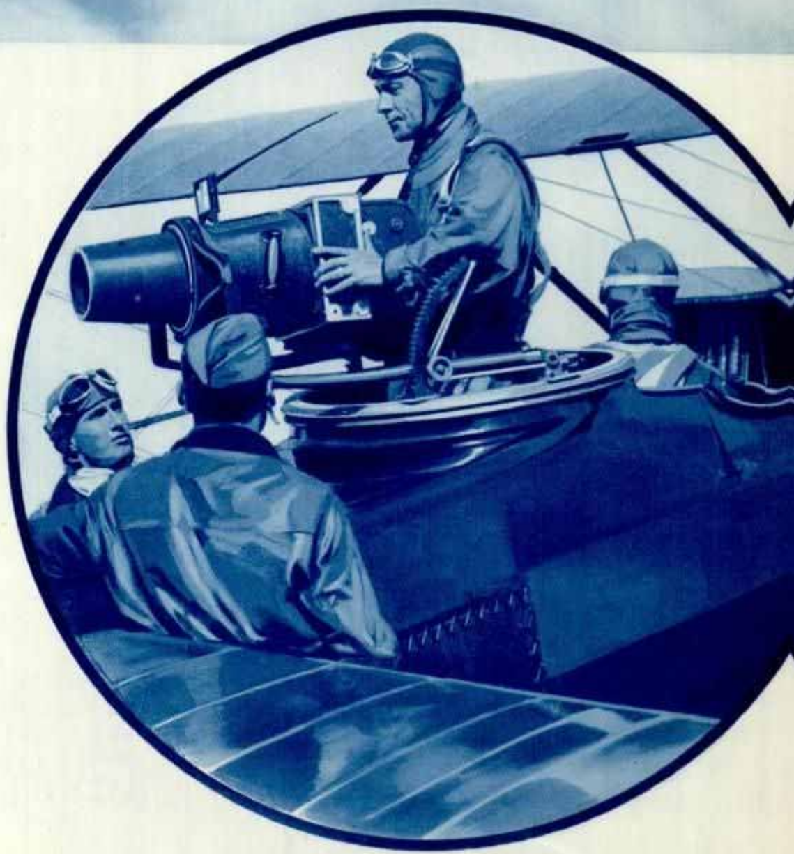
FOLLOW - the - leader, an example of close formation flying. Right, students learning how to mount and manipulate the aerial camera on an observation plane. This camera can take oblique views of strategic positions, and the record it makes is an invaluable aid to military strategists in time of war.
