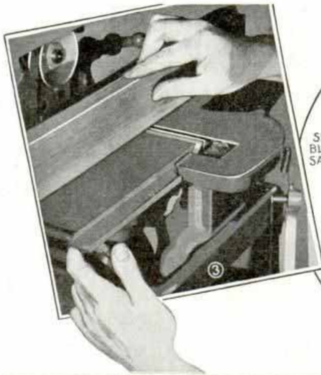
HOW MORTISING ATTACHMENT MAY BE USED TO GRIND JOINTER KNIVES
