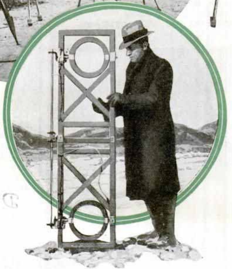
Two Observers Simultaneously Registering Electrical Currents at Right Angles; Below, Magnetic Gradiometer Used in Geophysical Exploration
