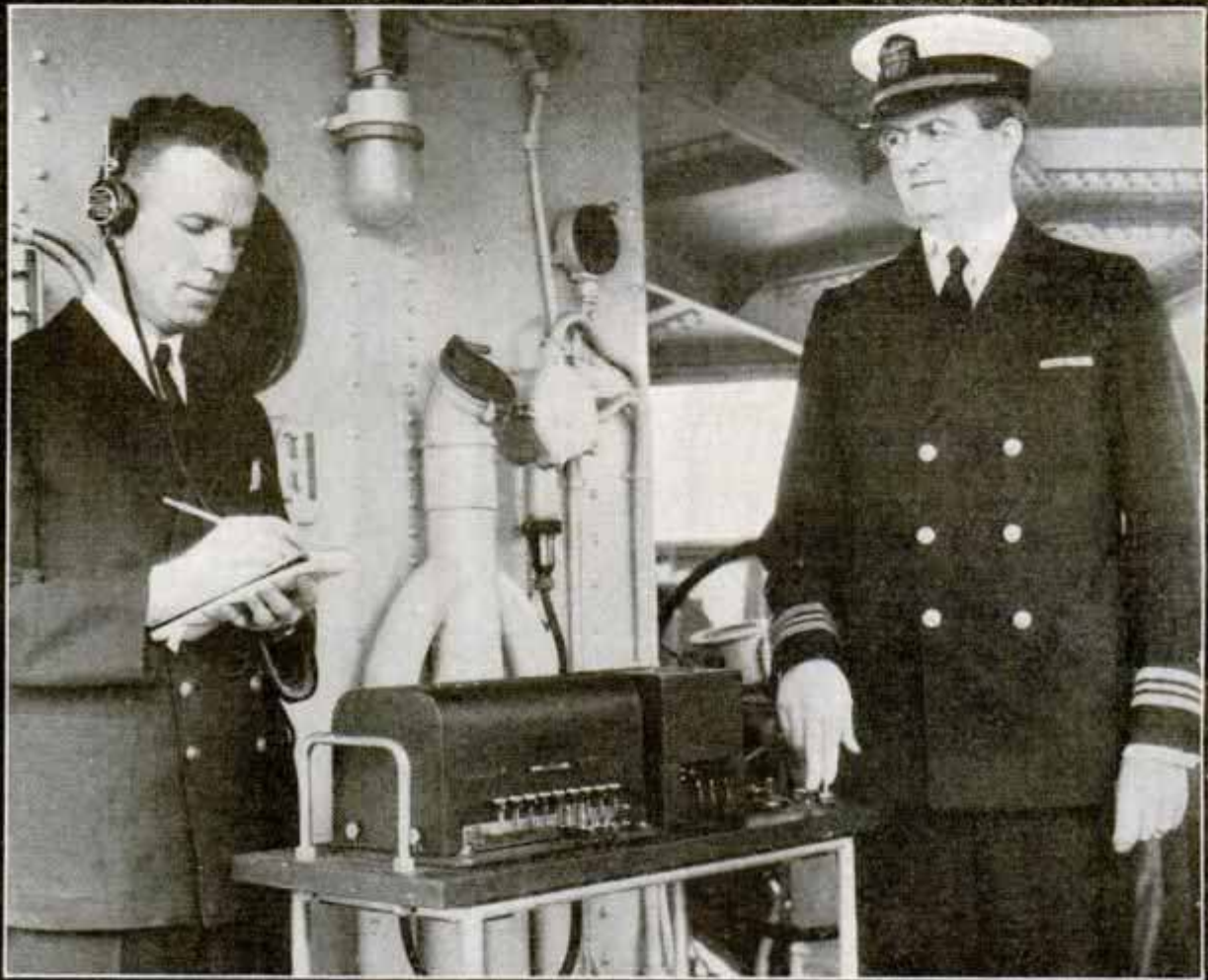
Control Box Which Governs the Operation of the Manless Warship Several Miles Distant; the Petty Officer Receives Radio Reports as Each Mechanism on Robot Ship Goes into Action
