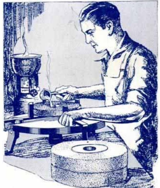
Drawing Shows How Grinding Wheels May Be Babbitted in Preparation for Mandrel
