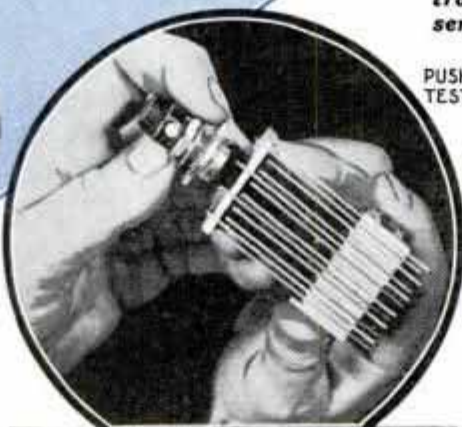
Above, Four-Circuit Double-Pole Double-Throw Jack Switch; Below, Fig. 1, Correct Method of Connecting Volume Control, Prevents Possible Loss of C-Bias
