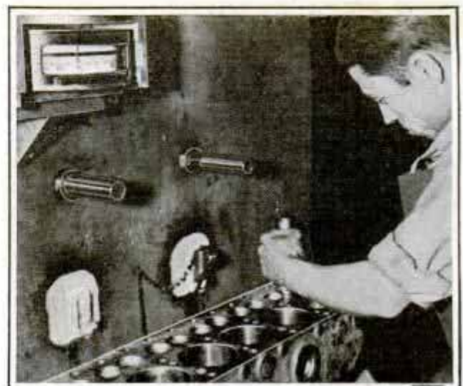
Note Frost around Valve Ring Outlets
