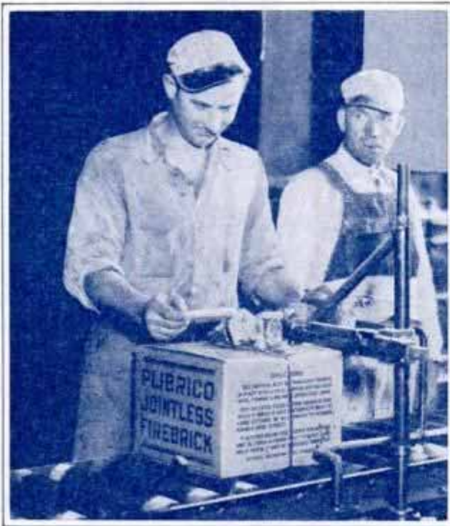
Packaging Is Speeded Up by This Strapping Tool with Mount Adjustable to the Package
