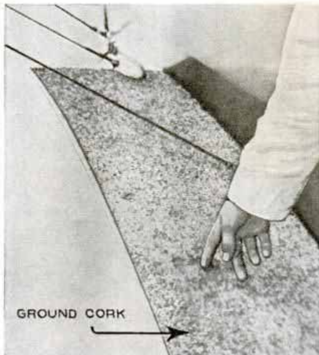
Ground Cork Applied to Step Area of Airplane Wing Prevents Slipping
