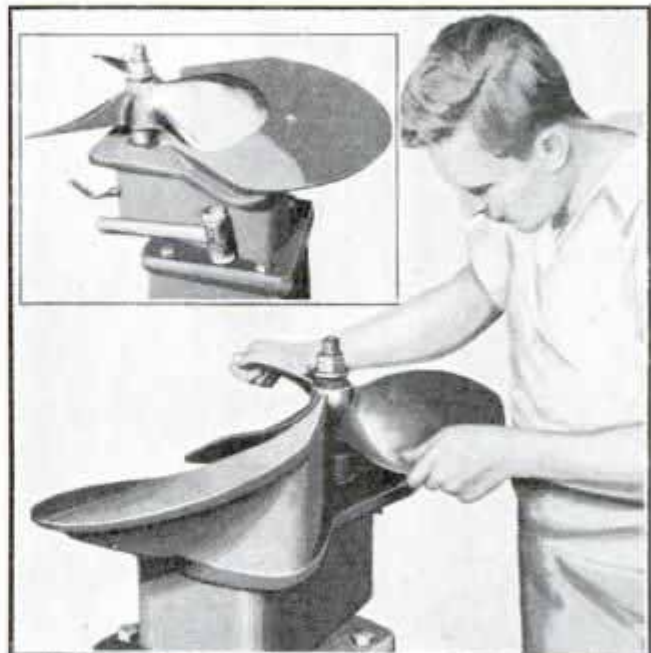
Fitting Boat Propeller Blade to Special Form Reveals Deviation from True Shape
