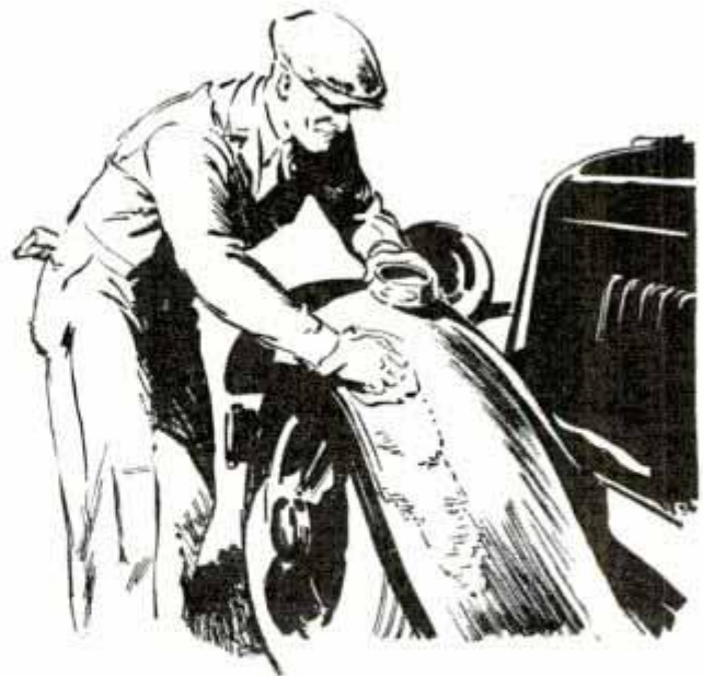
Wax Coating Prevents Exposed Metal of Car Fender from Rusting Until Repainted
