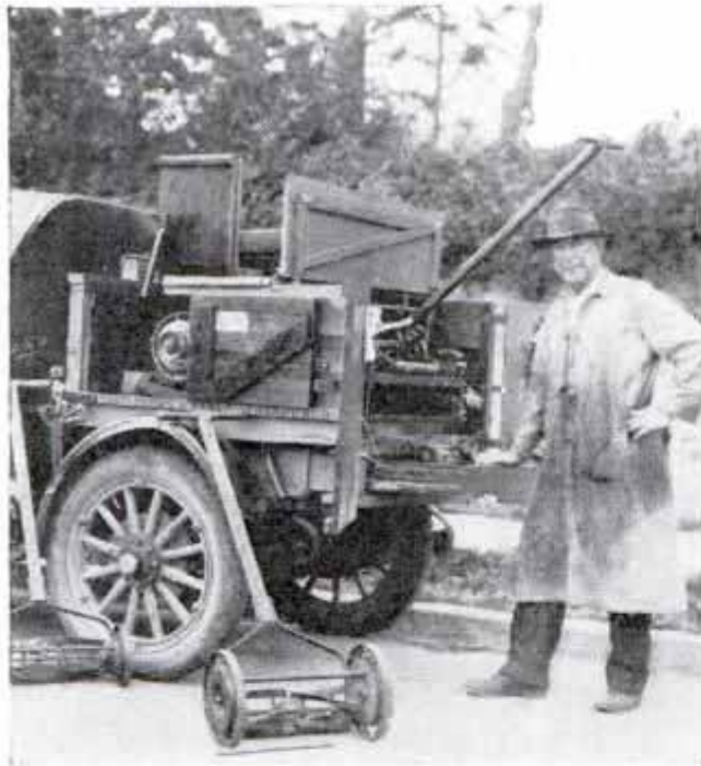
Traveling Shop Consists of Small Auto with Lawn-Mower Sharpener Built on Rear Deck
