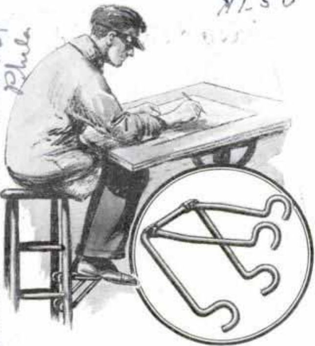
Bracket Which Provides Foot Rest for Stool When Attached to Rungs as Shown
