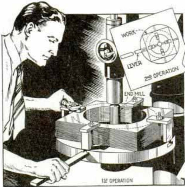
Large Rings Machined from Sheet Brass with End Mill in Drill Press
