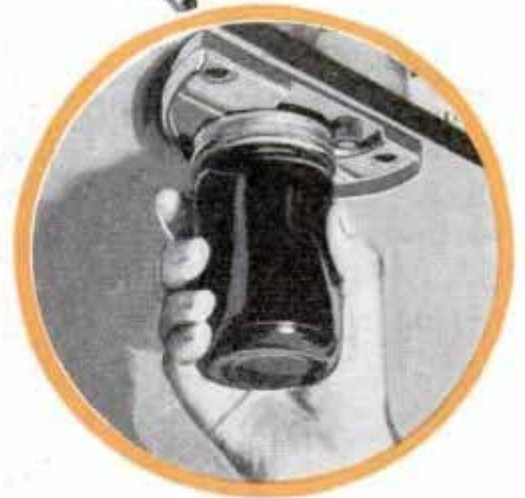
Above, Jar and Bottle-Top Opener Attached to Underside of Shelf; Top Is Wedged between Knurled Stud and Side of Groove
