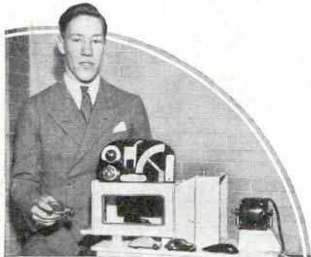
D 430 Small Portable Wind Tunnel for Testing the Stream-line Efficiency of Model Automobiles
