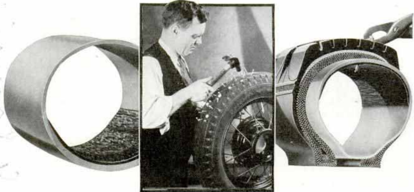
Left, Tube with Reinforcing Rubber to Prevent Damage When Tire Is Run Flat; Center, Driving Nails into Tire; Right, Removing Nail from Tube Which Is Self-Sealing, Keeping Air from Escaping
