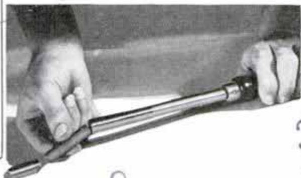
Electric Soldering Iron Employs Removable Cartridge-Type Heating Element; Suitable Wattage May Be Selected for Any Particular Kind of Work
