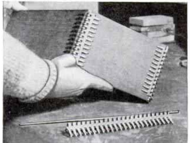
Metal Belt Lacing Makes Corner Fasteners for Boxes and Permits Them to Be Taken Apart
