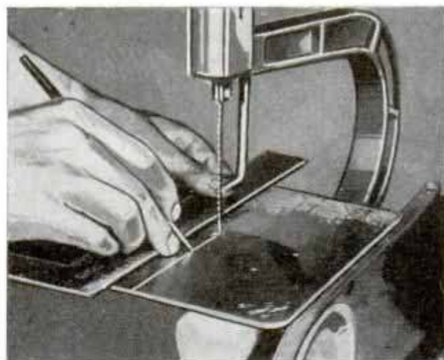
Line Scribed in Center of Jig-Saw Table Aids in Keeping Work Lined Up
