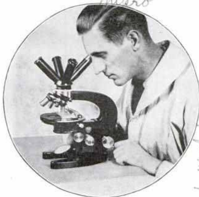
This Microscope Has Four Eyepieces so Arranged That Each Can Be Brought into Instant Use
