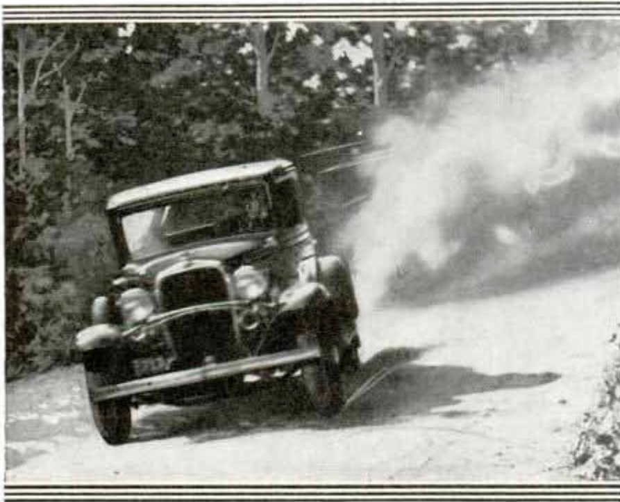
The Power Skid Is Newer Than the Side-Sway or Braking Skid, but Is Handled the Same Way—Steer in Direction Rear Wheels Are Sliding
