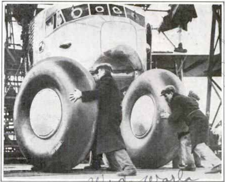
Landing Wheels of Great Britain's Biggest Passenger Plane Being Rolled into Position; the Ship Will Accommodate Forty Passengers
