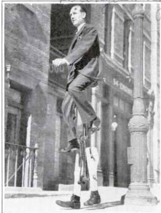
This Man Sits While Walking as He Propels a "Bicycle" Equipped with Legs Instead of Wheels
