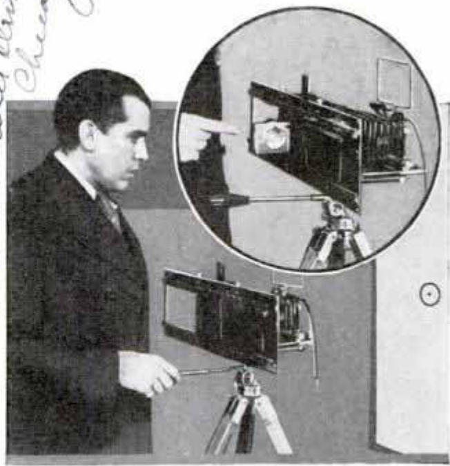
Focusing a Camera in the Dark Is Made Easy with This Flash Light in the Form of a Plate Holder
