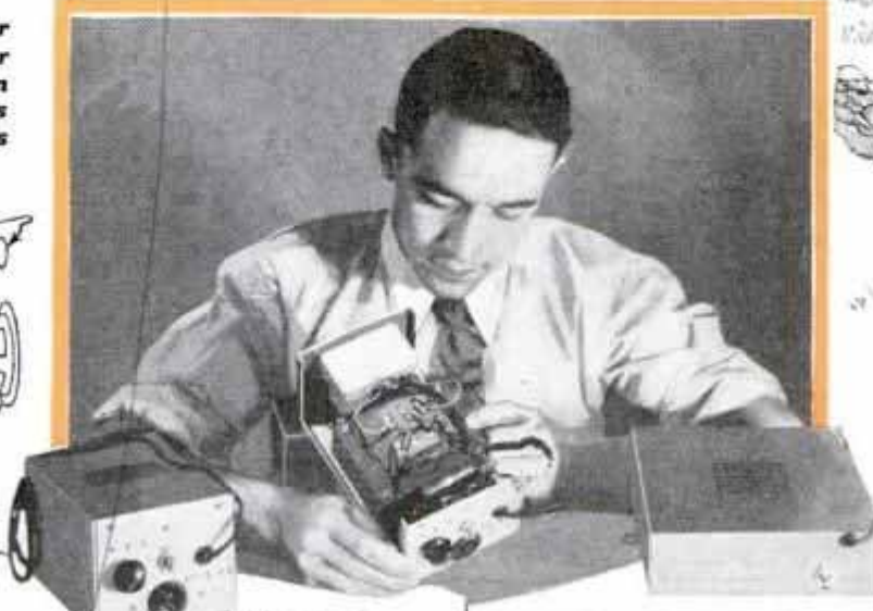
Above, Small High-Range Speaker, of Piezoelectric Crystal Type, Connected across Ordinary Loud Speaker Improves Tone Range; Right, D.C. Converter and B-Eliminator Now Available for Operating Any A.C. or Battery Receiver on 32-Volt Farm Lighting Plant; the Converter Supplies 110 Volts A.C. at 100 Watts and the B-Eliminator Has an Output of 200 Volts D.C. at 40 Mils.; Below, Plugs and Sockets for Heavy Inductance Coils
