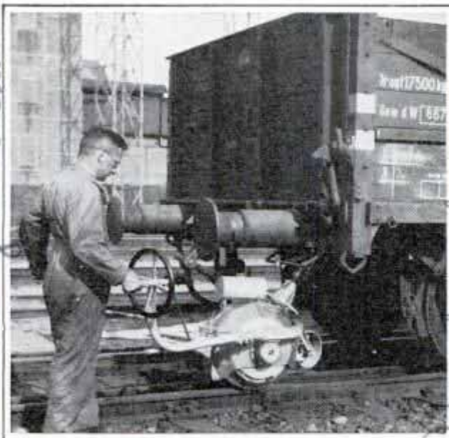
How Small Shunting Engine Enables One Man to Move a Loaded Freight Car
