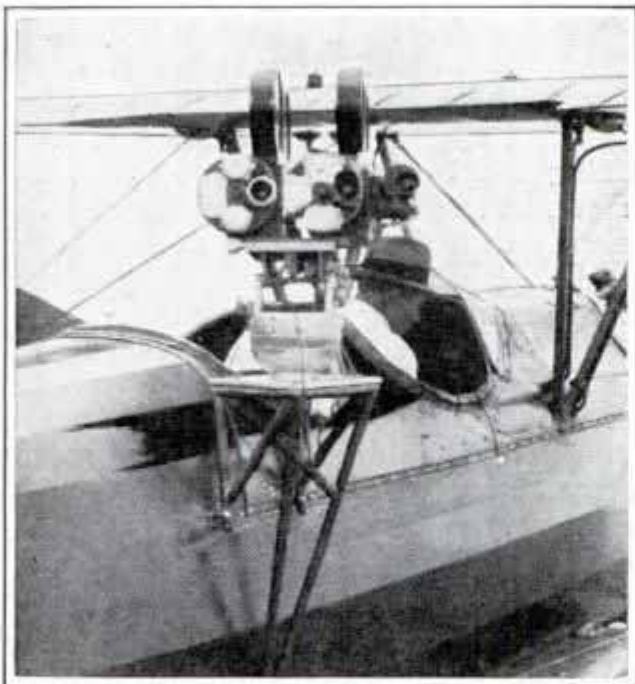
Two Movie Cameras Mounted on Plane for Taking Long Shot, and Close-Up of Same Scene
