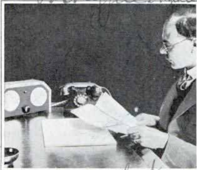
You Can Talk from Across the Room into This Telephone Containing a Microphone and Loud Speaker
