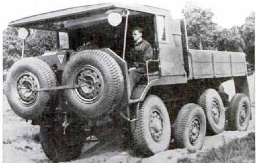
Flexibility Made Possible by Independent Wheel Suspension Enables This Truck to Travel the Roughest Roads without Jars or Bumps
