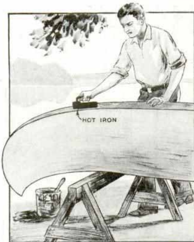
Hot Flatiron Run over Canvas Covering on Canoe Makes the Fabric Adhere Snugly
