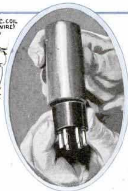
Upper Right, Slight Cuts on Tube Prongs for Better Contact in Old Sockets; Below, Fig. 1, Condenser Capacities Added by Parallel Connections; Lugs Used as Shown in Photo; Fig. 2, Noise-Filter Condensers in Series across Power Line
