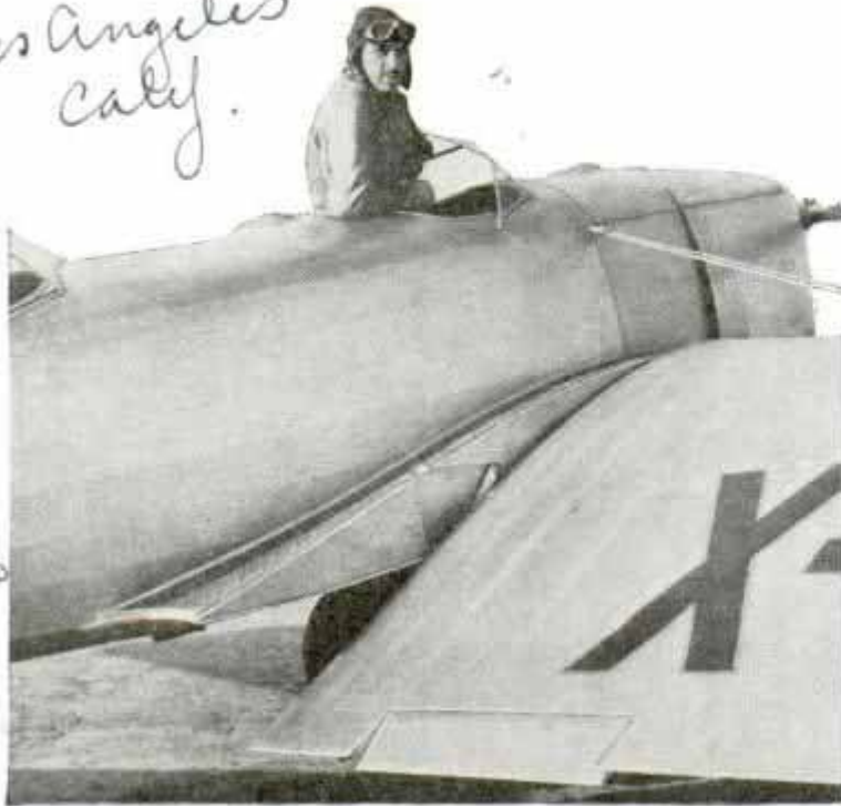
Showing Wing of Plane with Trailing Edge Much Lower Than Angle of the Ship; the Wing Is Controlled from Cockpit
