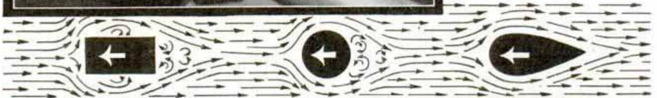
Top, Changing Shape of Wind-Tunnel Model with Clay; Below, Resistance Met by Three Shapes Passing through Air
