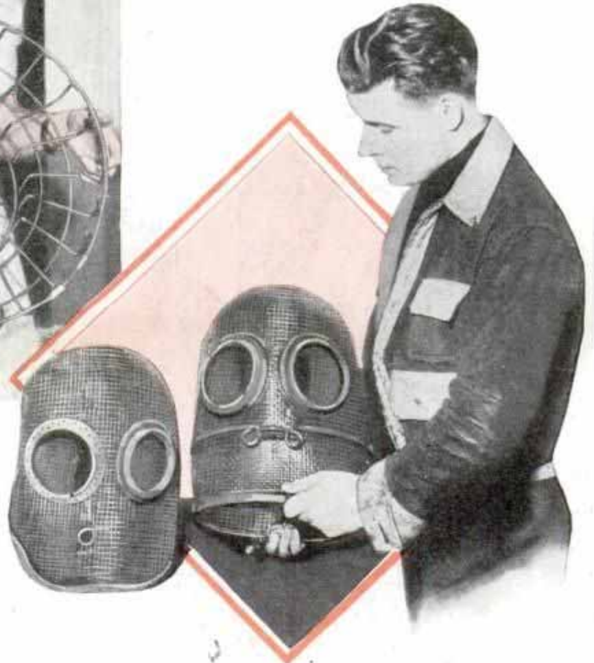
Left, Dish Rack Illustrates Intricate Forms That Can Be Covered with Rubber; Right, Sandblaster's Helmets; One at Right Is Rubber Covered
