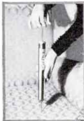
Left, Insecticide Gun with a Hollow Pointed Needle, Like the Surgeon's Hypodermic Syringe, for Injecting Moth-Killing Liquids into Upholstery
