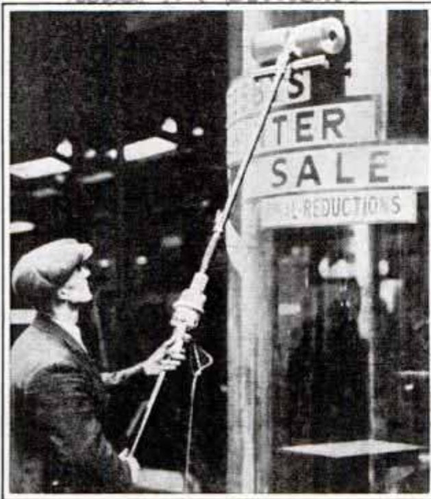
Window Cleaner and Polisher Operated by an Electric Motor Which Turns Rotary Felt Pads
