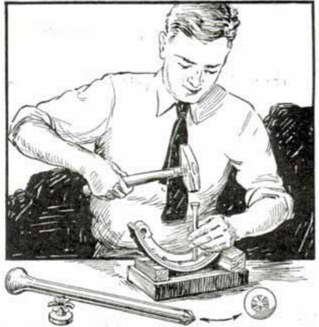
Tool Made from Old Valve Stem for Setting Rivets When Relining Auto Brakes
