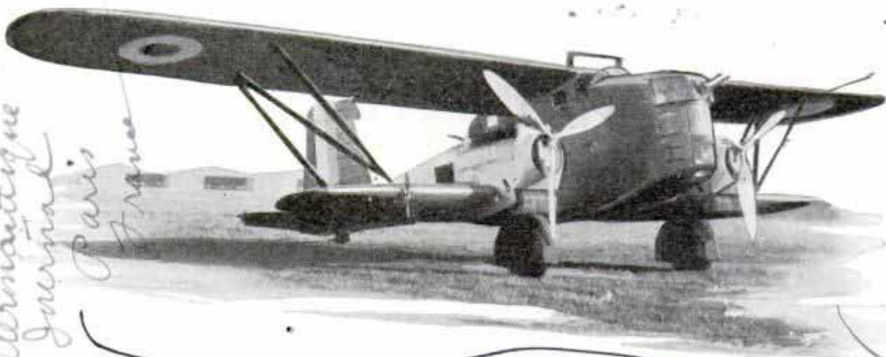
Courtesy l'Aeronautique Journal French War Plane with an All-Steel Armored Hull Inclosing Three Decks; Note the Battery of Machine Guns Mounted in the Nose of This Giant Flying Fortress
