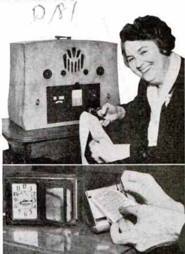
Top, Radio with Built-In Clock Control; Bottom, Desk Clock with Moving Schedule Tape
