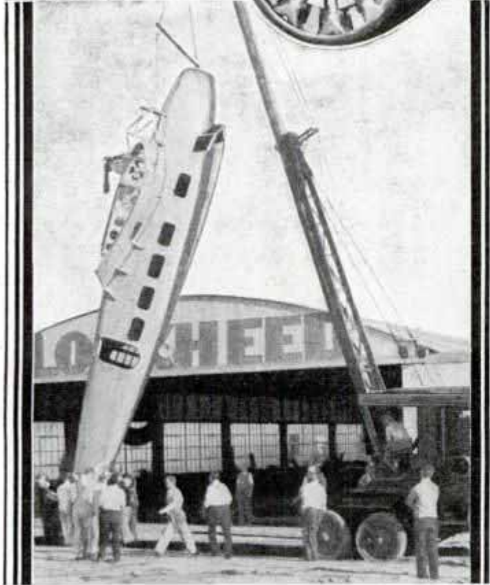
Above, Electrically Driven Motor and Dynamometer Inclosed in Metal Plane Fuselage Used for Studying Characteristics in Wind Tunnel; Below, Plane Being Turned Upside Down for Load Test
