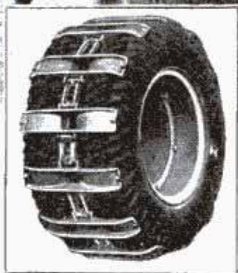
Steel Treads Applied over Dual Pneumatic Tires Like Tire Chains to Give More Traction to the Truck Either in Mud or Snow
