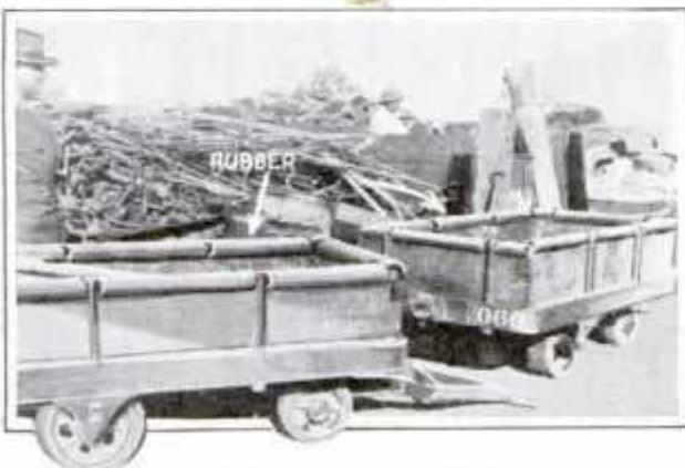
Rubber Hose or Auto Tires on Top Edge of Truck Bodies Prevent Wear
