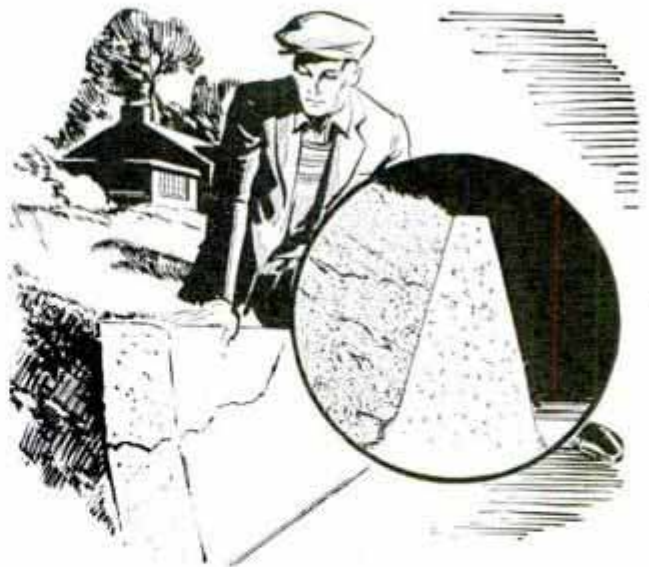
Tapered Terrace Wall Has Less Tendency to Be Cracked by Freezing and Thawing of the Ground
