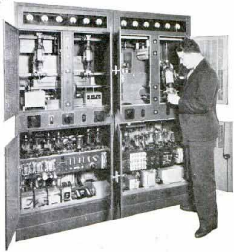
Above, Front View of Police Transmitter; Below, Dispatcher Handing Message to Police Radio Announcer
