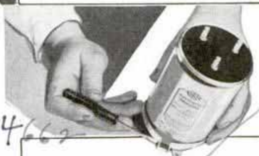
Electrolytic Condenser for Power Units Has Three 8-Mfd. Sections; Metal Container Is Common Negative; Left, Tin Can as Protection from Hot Resistors
