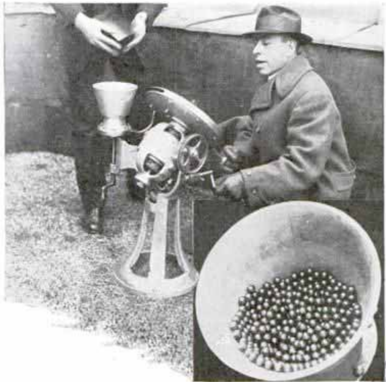
Motor-Driven Machine Gun and the Funnel-Like Arrangement through Which Ammunition Is Fed
