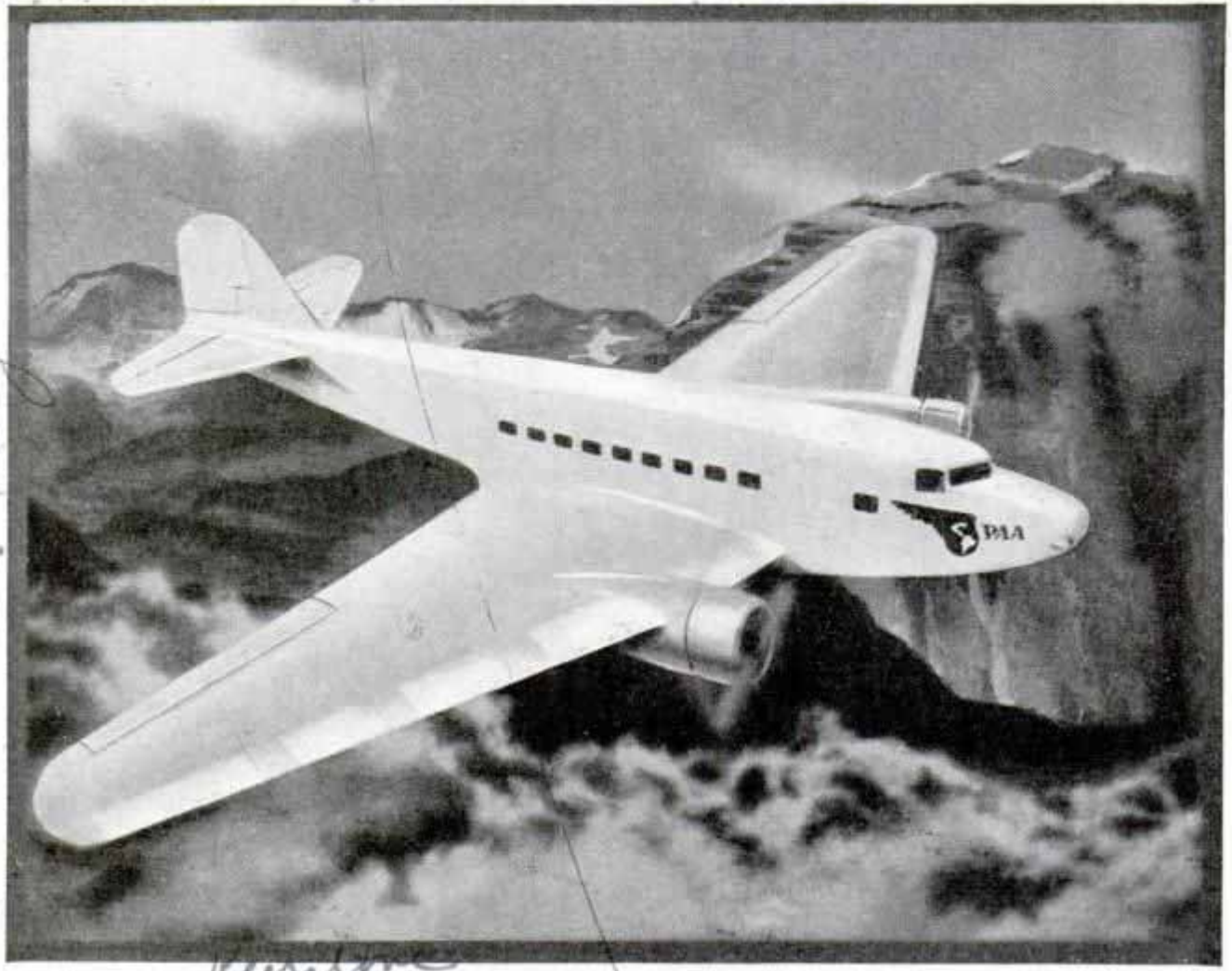
Fourteen-Passenger Transport Plane Which Will Speed Up Service over Pan-American Airways; Ships Like This Can Operate at Altitudes of 30,000 Feet at Speeds of 200 Miles Per Hour
