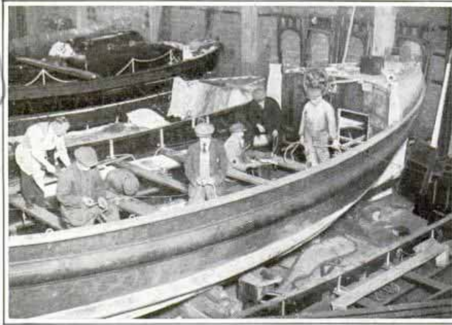
Overhauling and Repairing a Lifeboat at a Diminutive Drydock in London Where All Such Craft Are Constructed, Equipped and Repaired
