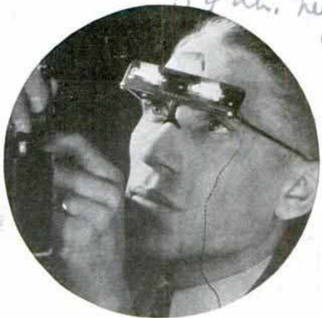
Double Spot-Light "Spectacles" Which Illuminate Close Work and Leave the Hands Free
