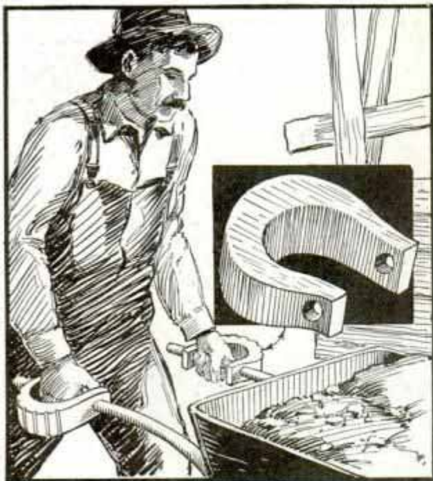
Short Sections of Old Auto Tire Protect Hands When Pushing Wheelbarrow in Tight Places
