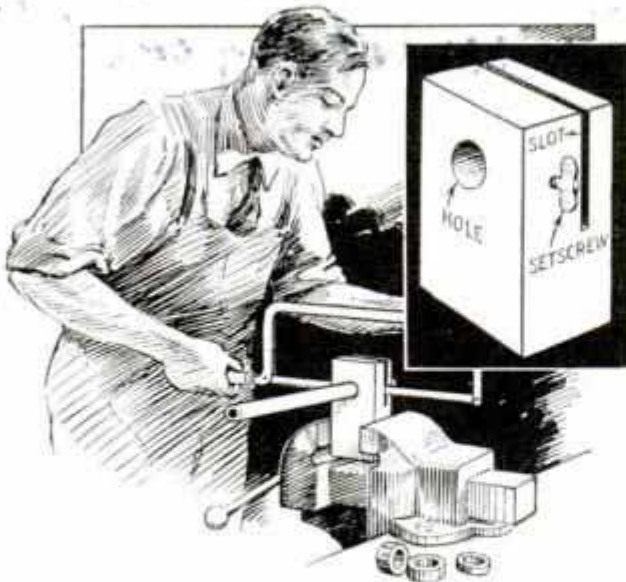
Jig Made from Steel Block Helps in Cutting Rings from Pipe with Hacksaw
