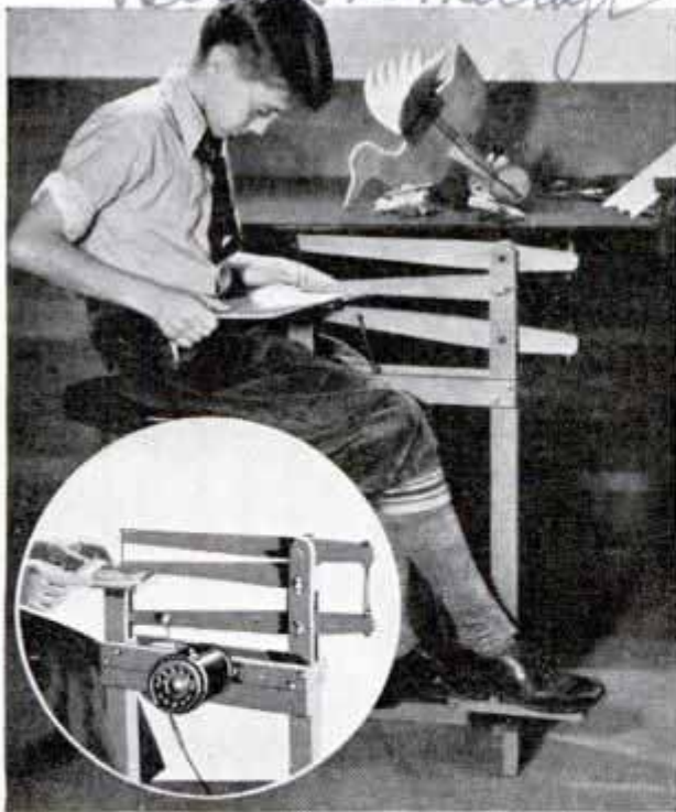
Foot-Operated Jigsaw Which Can Be Converted to Electric Drive by Attaching Small Motor
