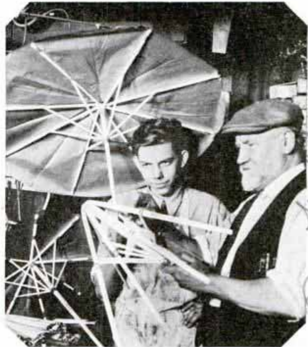
The Top of This Umbrella Is Made of Paper and the Stays, Ribs and Handle Are of Cardboard
