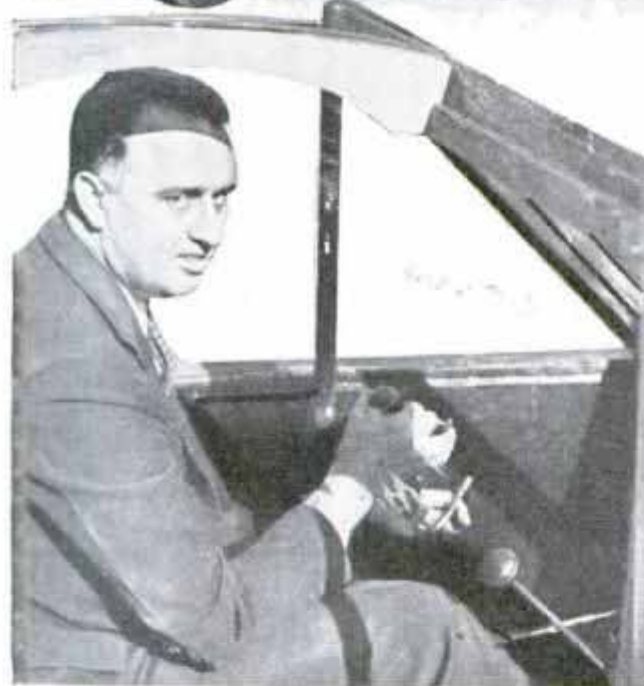
Interior and Exterior Views of a Two-Passenger Auto Built Like an Airplane; It Travels on Two Wheels and the Big Rudder Aids in Steering and in Balancing
