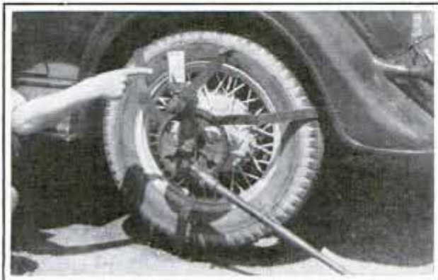
Brake Tester Shown in Place on Wheel: It Gives Quick Checkup on Condition of the Brakes
