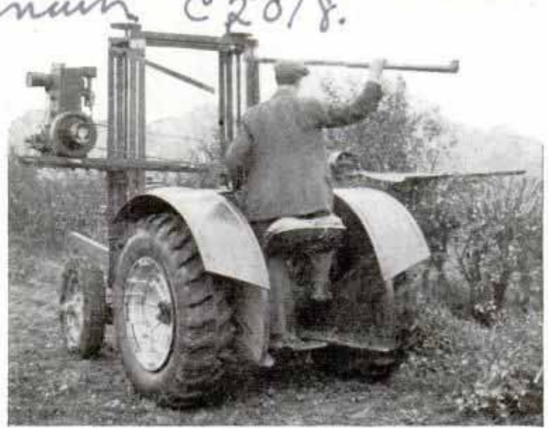
Hedge Trimmer Mounted on Small Tractor and Run by Gasoline Engine; It Cuts at a Uniform Height
