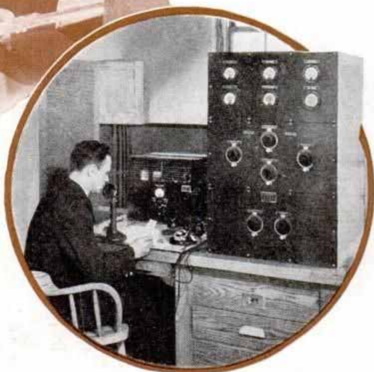
Above, New York Radio Squad Recording Alarm; Below, Left, Police Transmitter and Power Amplifier, at Right
