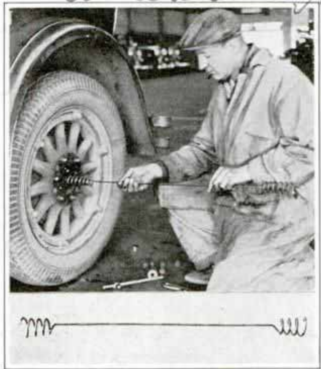
Spring Puller for Removing Broken Automobile Rear-Axle Shafts from the Housing
