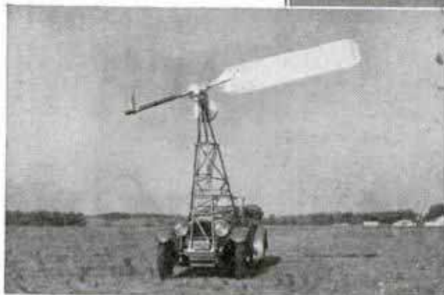
Top, Air Turbine on Sixty-Foot Tower; Center, Close-Up of Blade; Bottom, Power Plant Mounted on Auto for Tests in Wind Velocities up to Fifty Miles per Hour
