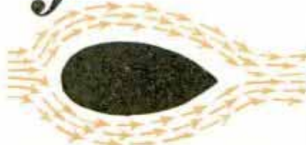
ILLUSTRATES THE EFFECT OF STREAMLINING IN REDUCING WIND RESISTANCE
