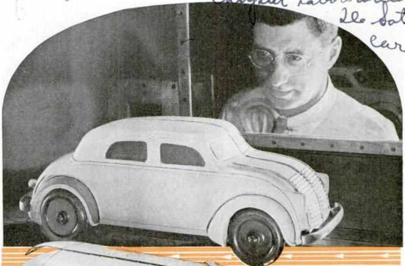
Above, Looking through Window of Wind Tunnel at Car Model under Test; Left, Streamlined Tank Truck with Rear Engine; Below, Air Flow as It Passes over Streamlined Car
