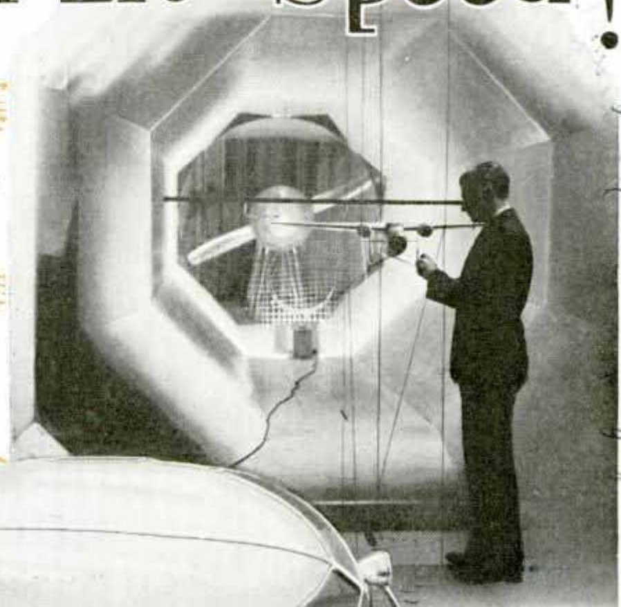
ILLUSTRATES THE EFFECT OF STREAMLINING IN REDUCING WIND RESISTANCE
