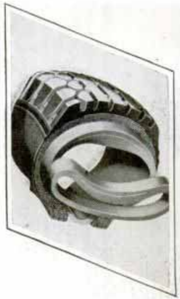
Below, Compression Inner Tube; Sliced Portion Shows Form Tube Tries to Take
