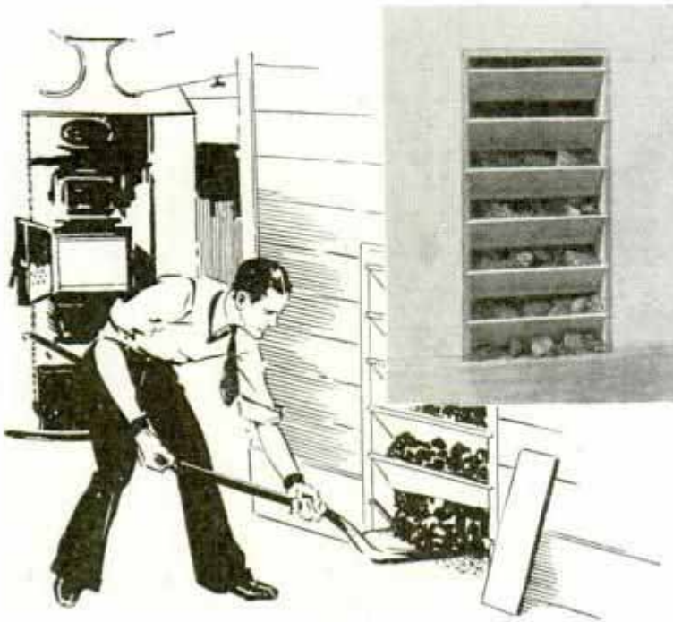
Louvers Fitted in the Door of Your Coal Bin Make It Easy to Remove the Coal
