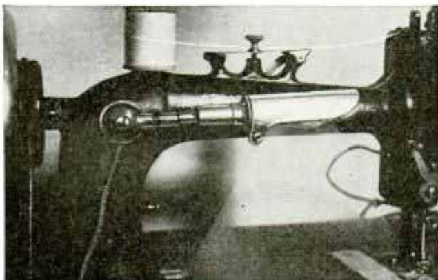
Light for Sewing Machine Made from Auto-Dash Light Socket and Sheet Aluminum
