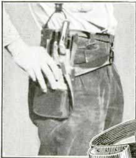
Above, Pipe Reel Holder, Fitted with Wheels and Back-lash Brake, Keeps Wire from Kinking and Tangling When Pulled through Conduit from Remote Point; Upper Right, Winch on Short Ladder Simplifies Job of Cable Pulling; Below, Leather Tool Holder Riveted to Belt Prevents Wear on Pockets; Center and Right, Small Reel Holder for Ladder Use When Dispensing Lampcord
