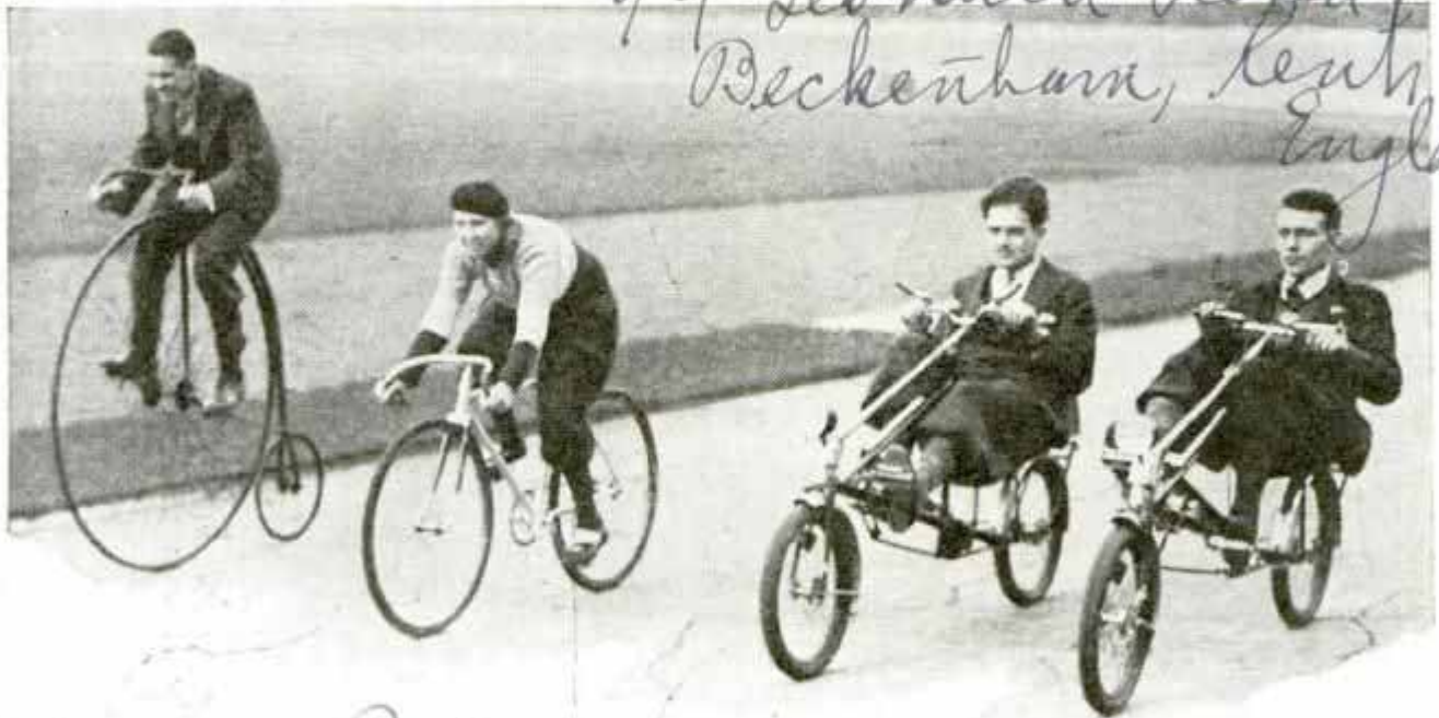
Riders on Ancient, Conventional and Newest Models in Bicycles; the Ones at the Right Have Comfortable Seats and Are Propelled by Pushing Forward on the Pedals
