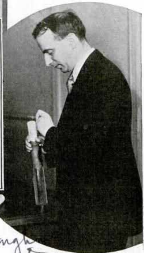
Top, Household Circuit Breaker; Insert Shows Inside of Device; Above, Inserting Boric-Acid Filler into Cartridge Fuse
