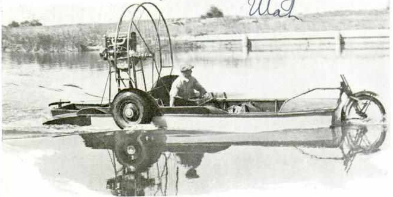
This Strange-Looking Craft Is Driven through the Water or on Land by Propeller Mounted at Rear; Note Wheels and Steering Arrangement for Use on Land; the Boat Is Particularly Useful to the Duck Hunter
