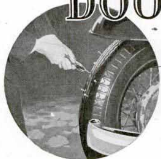
Driving Nails into a Truly Puncture-Proof Tire, Then Pulling Them Out without Losing Any Air; Running the Car around the Block Seals the Holes
