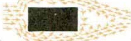
DEPICTS RETARDING FORCE SET UP BY NON-STREAMLINED CAR IN MOTION
