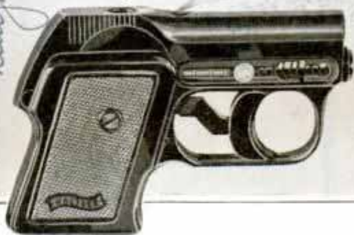
Pistol Which Fires Only Blank Cartridges; It Has an Automatic Ejector and No Magazine
