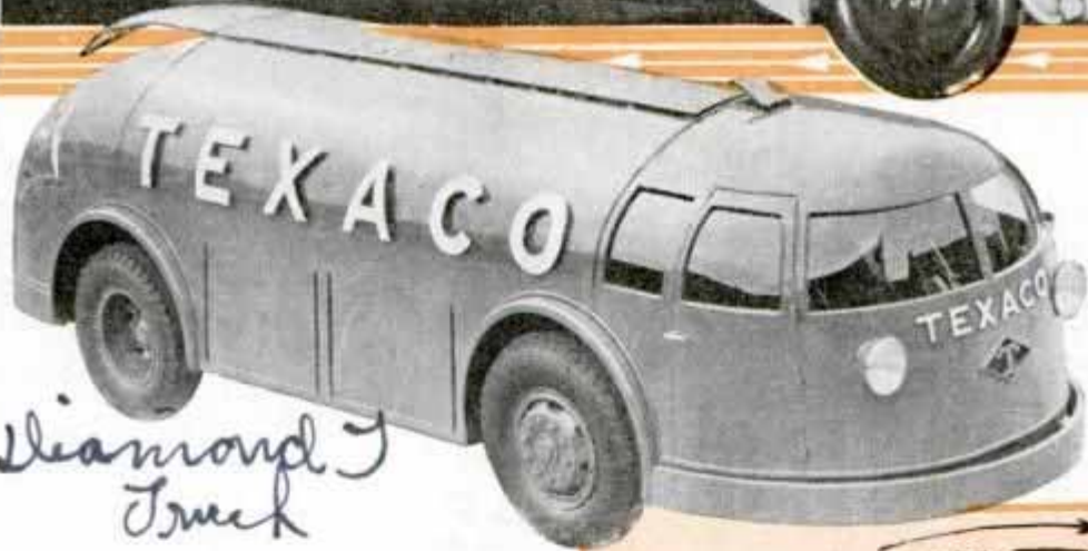
Above, Looking through Window of Wind Tunnel at Car Model under Test; Left, Streamlined Tank Truck with Rear Engine; Below, Air Flow as It Passes over Streamlined Car
