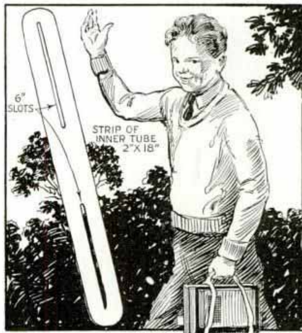
Slotted Ends of Rubber Strip Slipped over School Books Provide Good Carrying Handle
