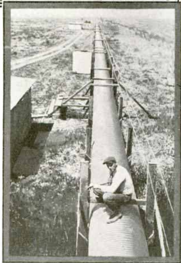
Top, Method for Sending Beam of Light through Mile-Long Tube Used in Making the Measurements; Below, a Section of the Tube
