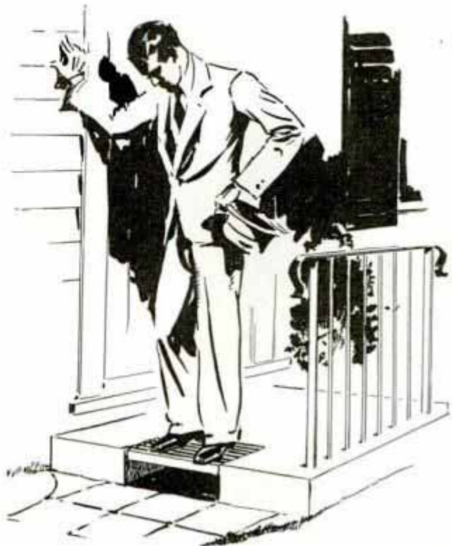
Sewer Ventilator Set in Recess in Porch Step Makes Handy Shoe Scraper
