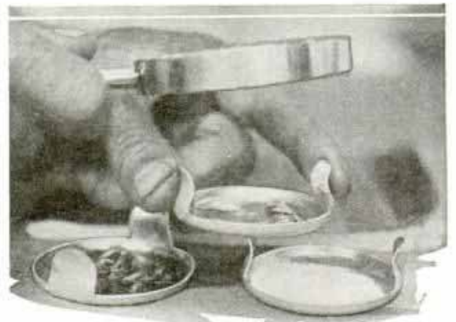
Milk-Bottle Caps of the Metal Type Hold Small Specimens While Studying Them under Magnifying Glass
