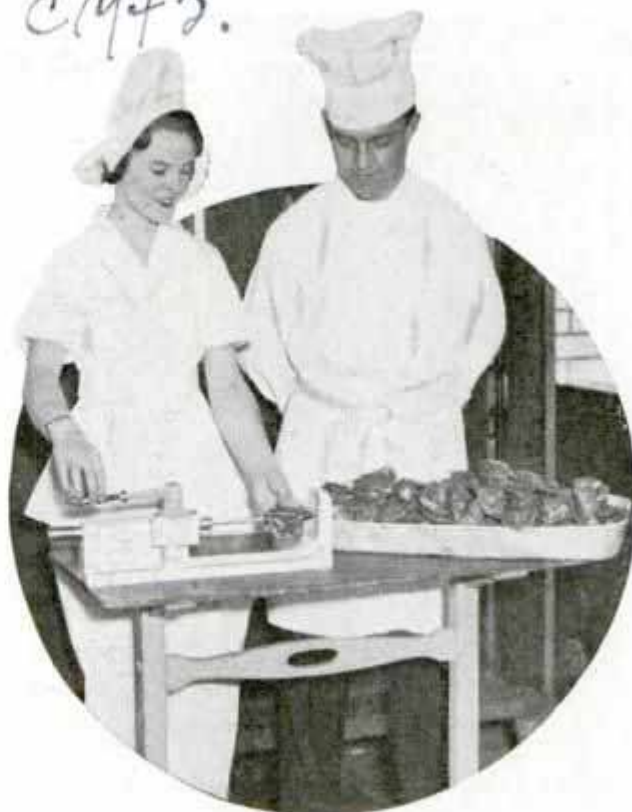
Twice as Many Oysters Can Be Opened Safely with This Device as with the Oyster Knife
