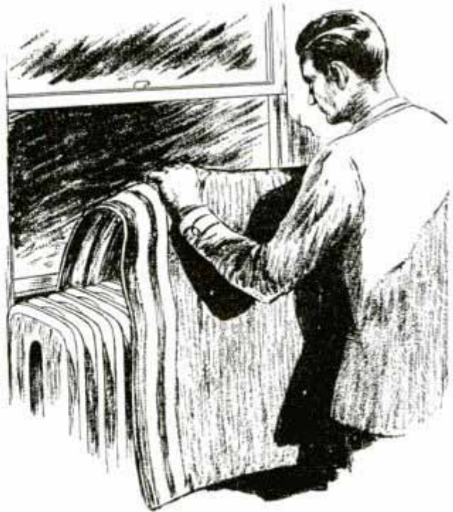
Covering Radiator in Cold Bedroom Prevents Rapid Cooling of Hot-Water Heating System
