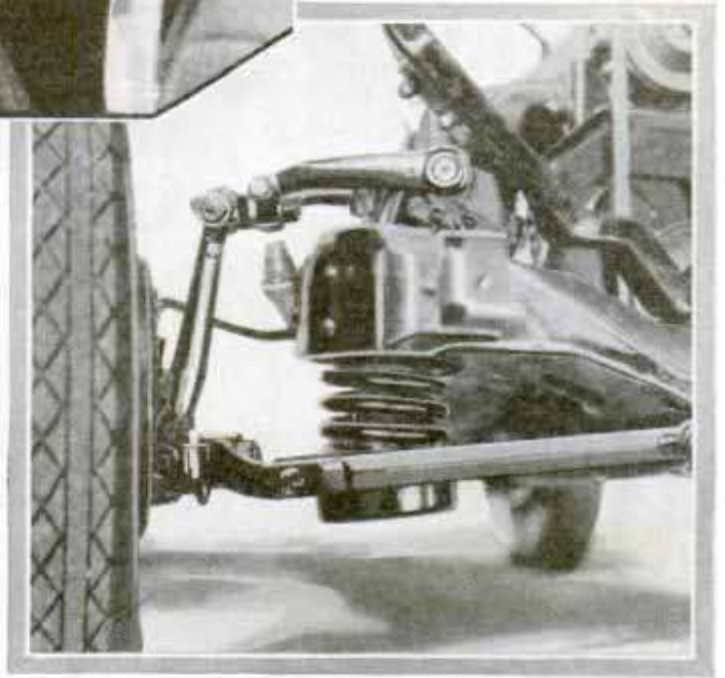
Top, Rear Seat of DeSoto; Note Tubing-Seat Frame; Bottom, Plymouth's Wheel Suspension
