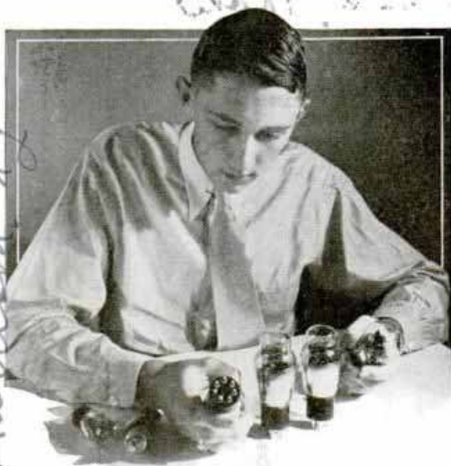
Triple-Grid Tube Showing the Seven-Prong Arrangement to Provide External Connections for Each Grid
