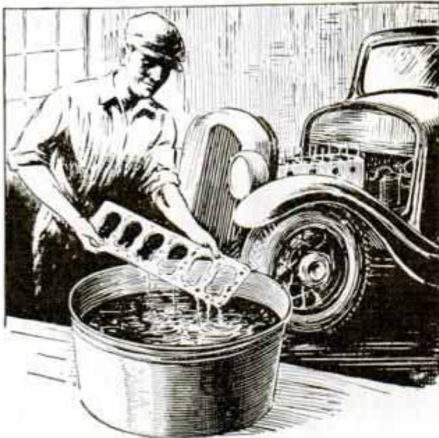
Soaking New Cylinder-Head Gaskets in Water Assures Effective Seal between Motor Head and Block
