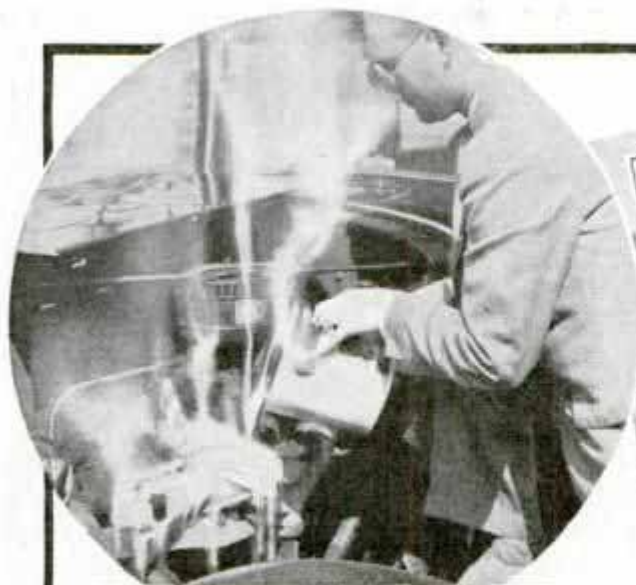
When Using Hot Water to Warm Up Intake Manifold to Make Starting Easier, Heat Can Be Retained by Wrapping Cloth on the Manifold
