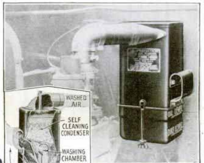
Photo and Diagram Show How Oil Device Cleanses Air before It Enters Auto Carburetor
