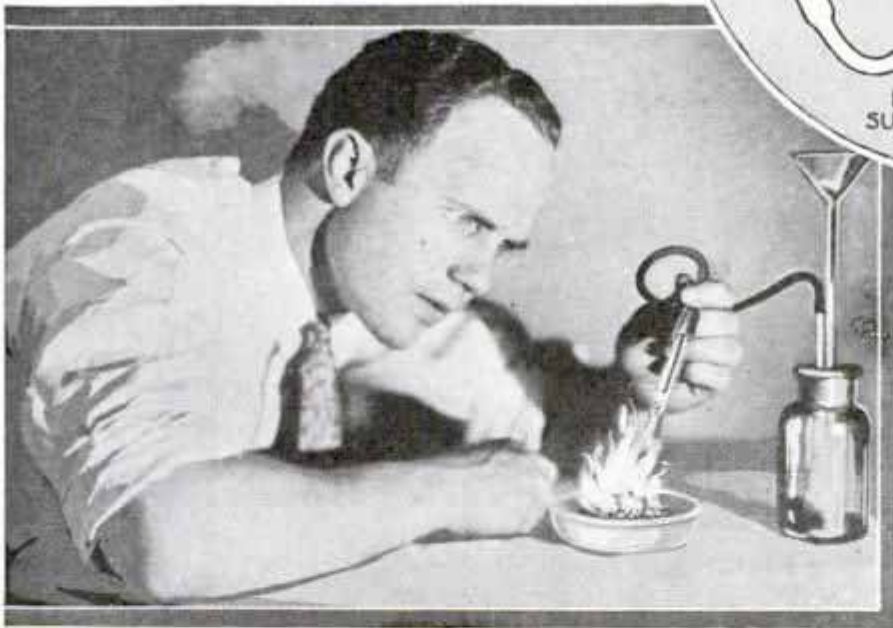
Above, Construction of a Homemade Hydrogen-Sulphide Generator; Left, When Directed against a Small Particle of Lead Peroxide, the Hydrogen-Sulphide Gas Will Take Fire and Give Off Odor of Burning Sulphur
