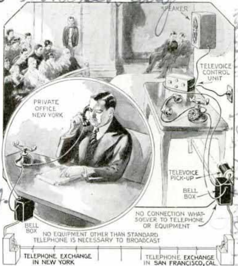
Diagram Shows Arrangement for Two-Way Conversation on Public-Address Scale by Means of Telephone Pick-Up
