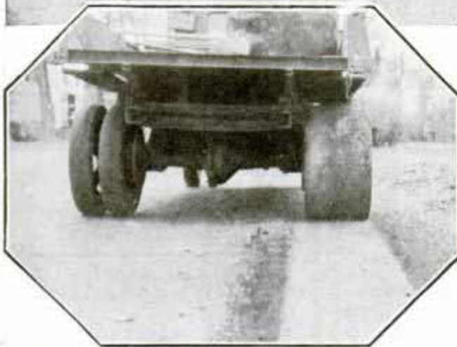
Top, Rim for Converting Truck into Roller; Bottom, Rim Shown in Use on Right Wheel
