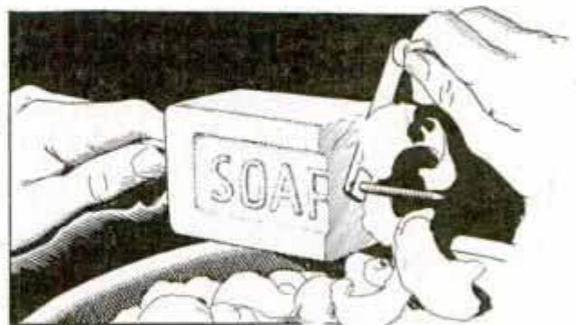
Soap and Vegetables Sliced with Tool Improvised from Iron Rod and a Strip of Sheet Metal
