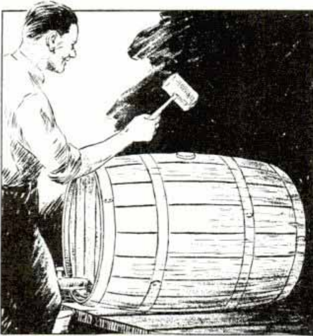
Striking Side of Barrel with Wood Mallet Quickly Removes Bung without Getting Splinters Inside
