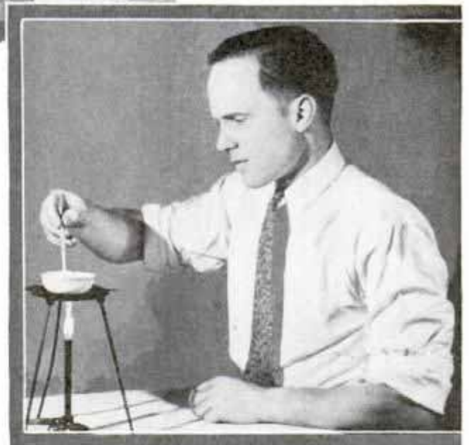
Drying and Dehydrating the Lead Tartrate in a Porcelain Dish Set over a Bunsen Burner
