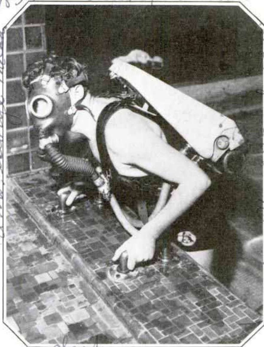
Oxygen Breathing Apparatus for Rescuing Drowning Persons; Visibility and Ease of Movement Are Not Hampered by Its Use
