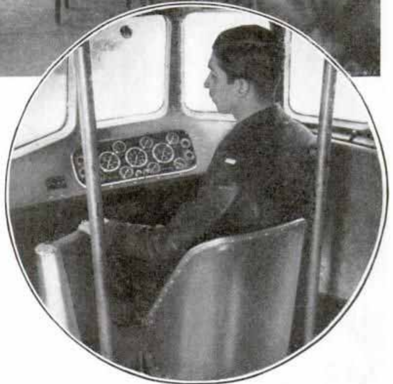
Top, Interior of Railplane Before Installation of Soundproofing, Insulating and Decorative Materials; Note Tube Construction; Bottom, Showing Neat Instrument Panel Resembling That of Airplane
