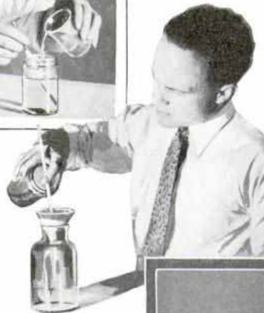
Above, the First Step in Making Pyrophoric Lead Is to Precipitate Lead Tartrate; Center, the Lead Tartrate Is Slowly Poured through a Filter
