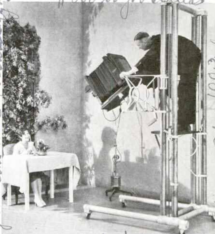
Stand Equipped to Place the Camera in Any Position for Photographing Commercial Scenes; Note Unusual Angle in This View
