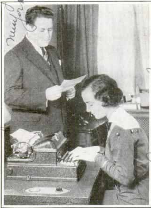
Operating the Radiotype, an Electric Typewriter with a Radio Transmitter Attached to It
