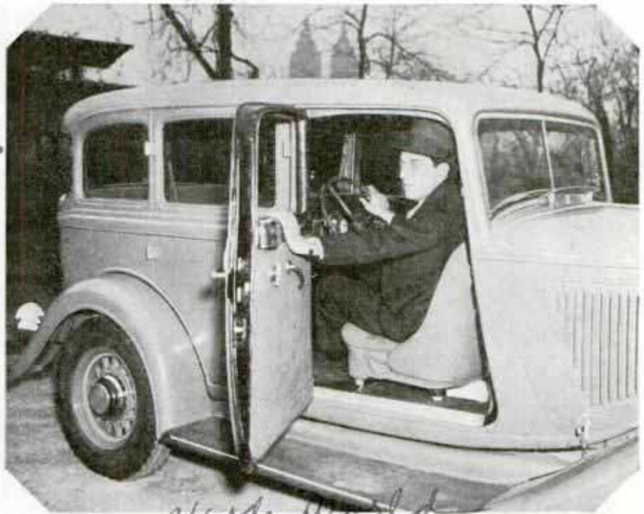
Body of Auto Reversed on Chassis; When It Is Going Forward, It Appears to Be Backing; This Demonstrates How Wind Resistance May Be Reduced
