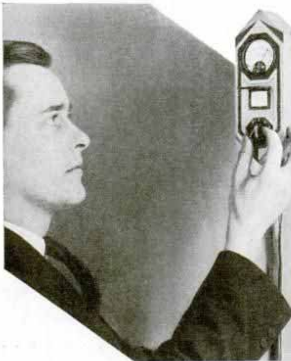
Indicator Which Shows Temperatures in Eight Separate Locations in Industrial Plant
