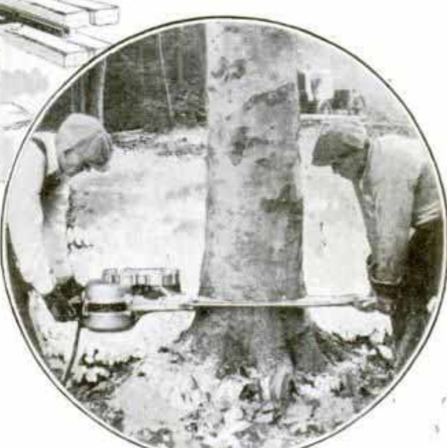
Left, Sawing Log into Boards After Equipment Has Felled Tree, Shown at Right
