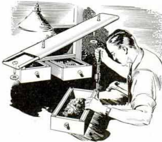
Lengths of Telescoping Curtain Rods Provide Easily Operated Slides for Drawers underneath Workbench
