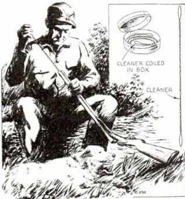
Doubled and Twisted Length of Piano Wire, Makes a Gun Cleaner That Is Easily Carried in the Pocket
