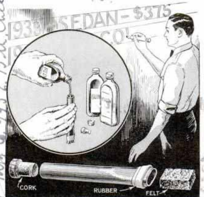
Circle, How Fountain Brush Is Filled; Bottom, Parts of the Felt-Tipped Brush
