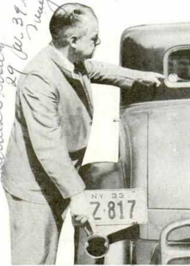
Circle on Rear Window Shows Location of "Electric Eye" Control for Parking Lights
