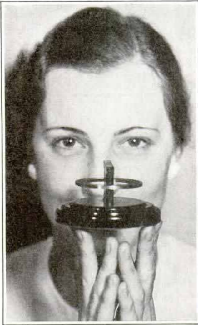
Small Ring Hovers Above Base in Demonstration of Magnetic Properties of Cobalt Steel
