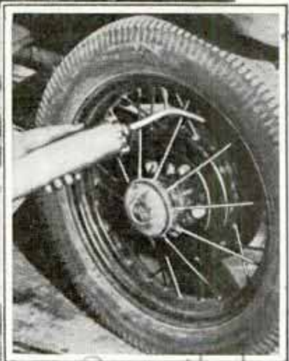
Top, Thawing Out Radiator with Hot-Air Gun; Bottom, Left, Warming Grease to Make It Flow Freely; Right, Thawing Brake Drum
