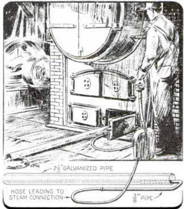
Suction Created by Steam Escaping from Small Pipe inside Large One Removes Water from Ash Pit
