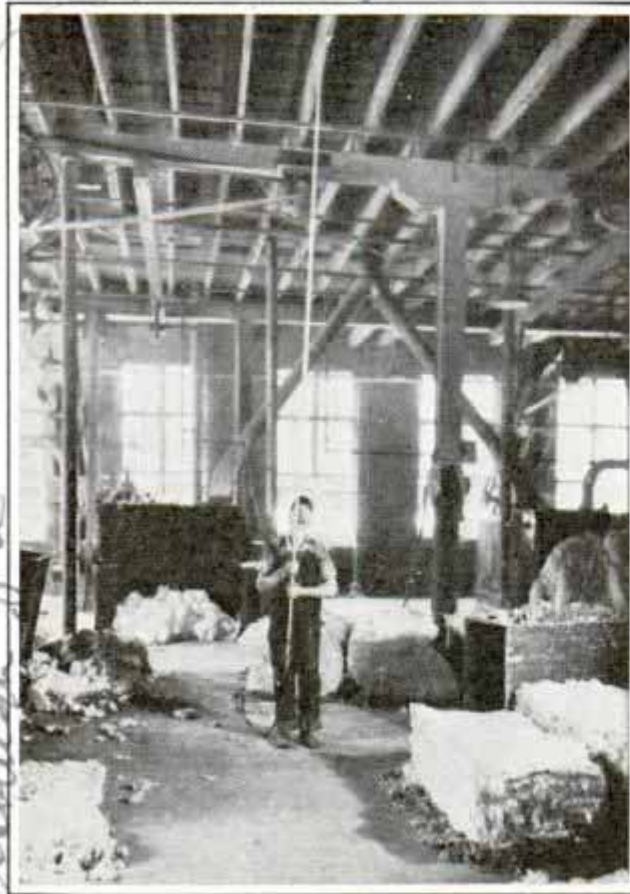
Using an Aluminum Pipe Attached to an Air Hose to Remove Lint from Ceiling of Cotton Mill
