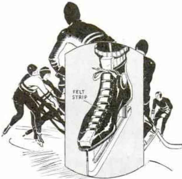
Strip of Felt between Laces and Tongue of Skate Shoe Gives Skater Foot Comfort
