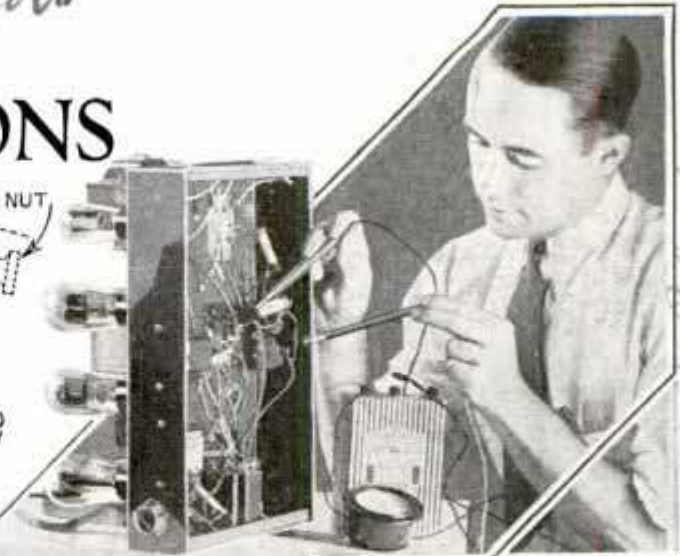
Using a D.C. Voltmeter in Series with a Small B-Battery to Check Wiring for Open Circuits; Shorted Condensers Are Also Easily Located by This Method; Left, Inexpensive Insulated Test Prods with Flexible Red and Black Leads for Easy Positive and Negative Identification
