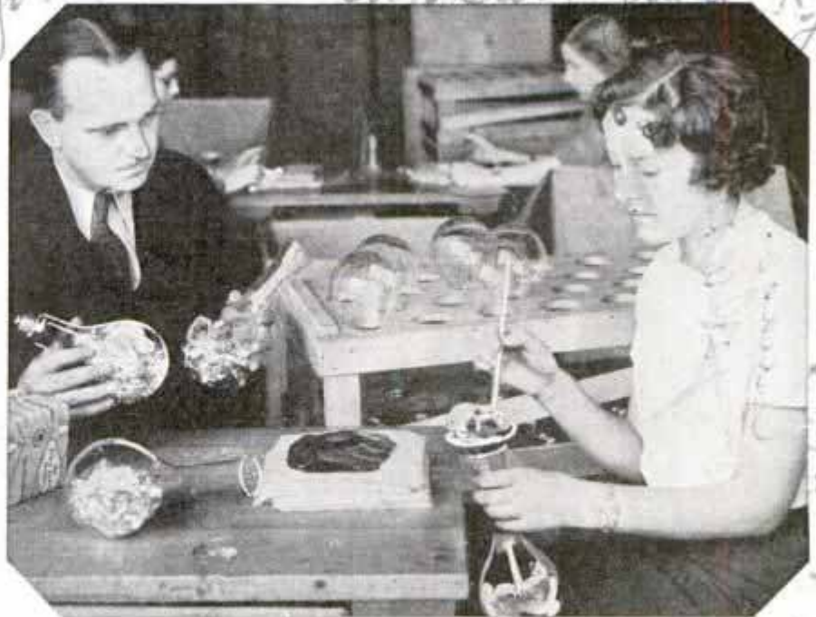
Inspecting Packing of Flashlamp Bulbs as the Foil is Carefully Inserted; These Bulbs Produce Brilliant Light for Photographic Purposes
