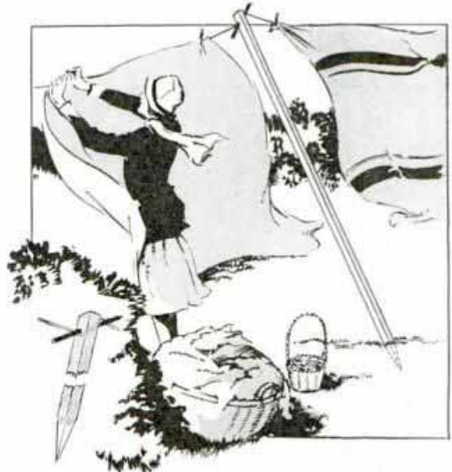
Dowel at Top End of Clothesline Prop Prevents It from Slipping Along the Line
