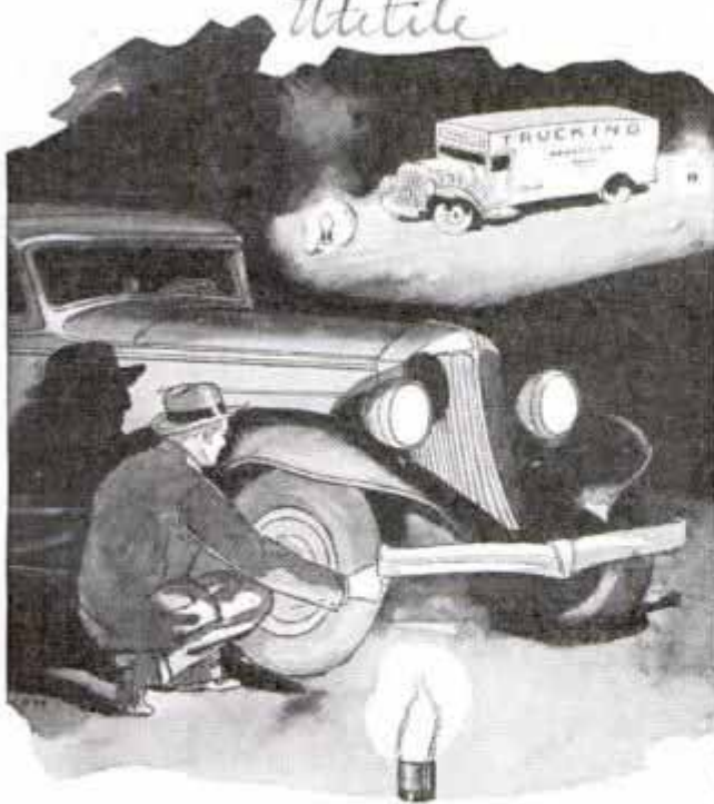
Repairing Tire on Roadway with Protection of Flare; Inset, Flare Guards Truck
