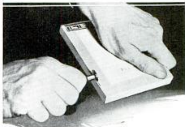
Empty Film Spool Used to Cut Paper Tape Sealing Boxes of Photographic Films and Print Paper
