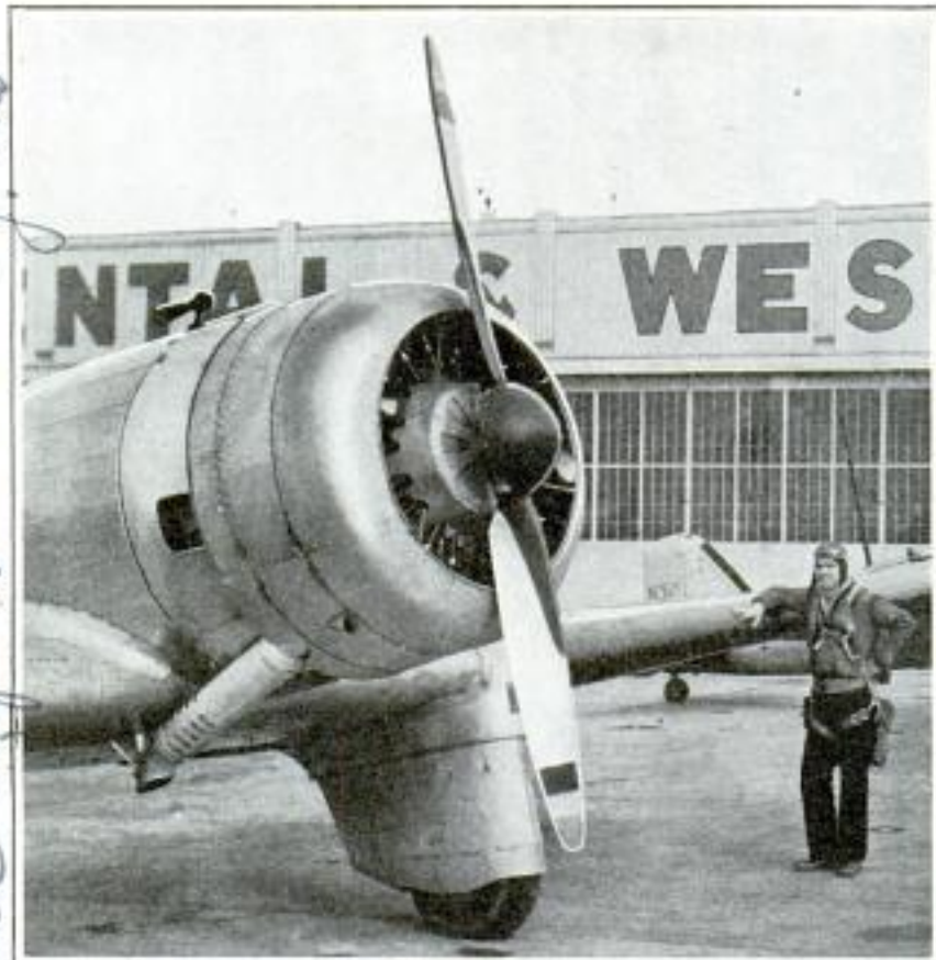
Note Rubber over Hub and Extending along Edge of Propeller; Arrangement Prevents Ice from Forming and Interfering with Flying
