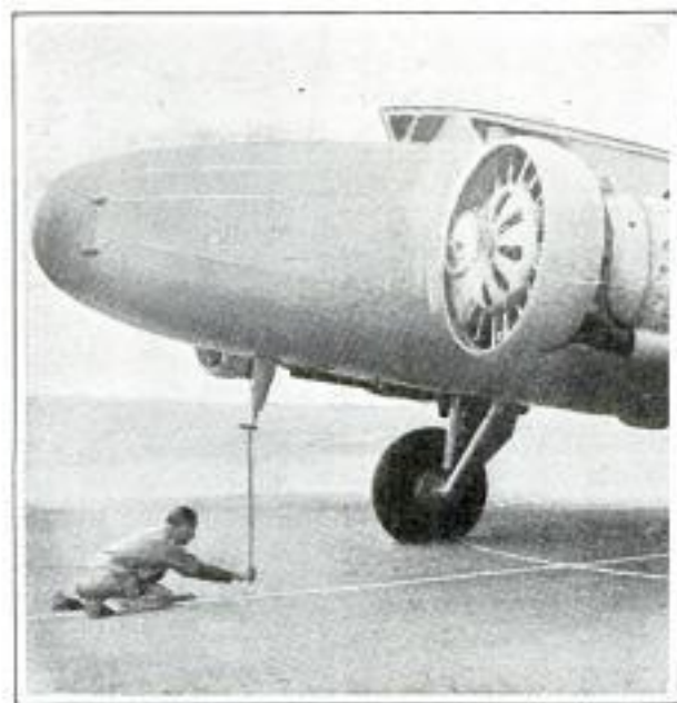
Using a Plumb Line to Test Compass of Airplane as Ship Is Turned in Segments of Circle
