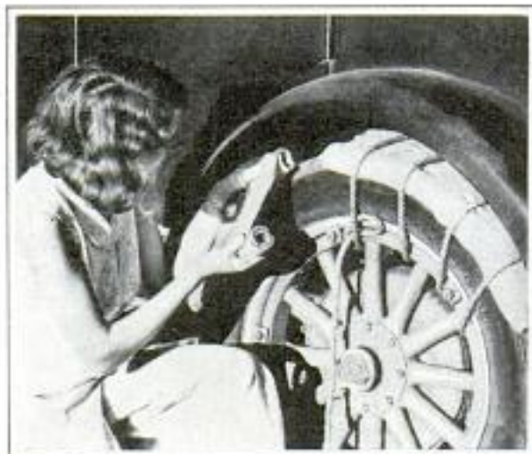
Sand "Shoes" for the Automobile Made by Tying Burlap Sacks around Front and Rear Tires
