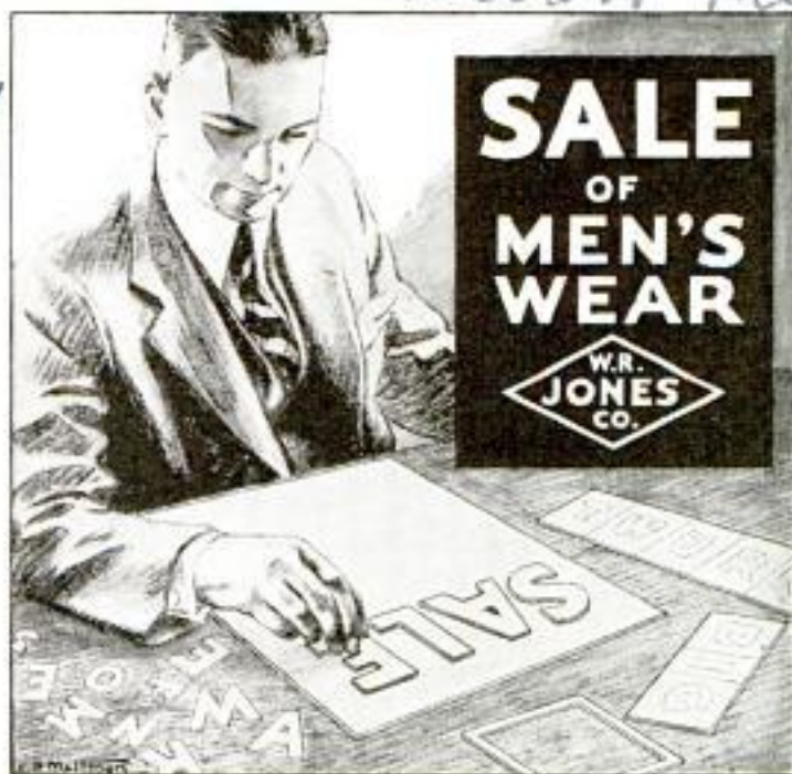
Gummed Letters Placed on Cardboard for Casting into Metal; Right, How Advertisement Appears after Printing
