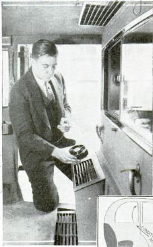
Top, Air-Conditioner Register in Rear of Auto; Center, How Unit Works; Bottom, Experimental Installation
