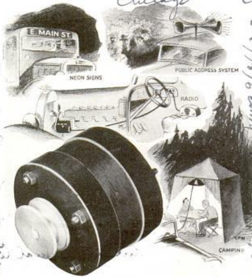
Generator for Supplying 110-Volt Current Is Easily Installed in Auto; Drawing Shows Some Uses of Electricity Generated by the Device
