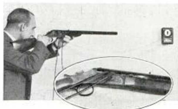
Shotgun Equipped to Fire a Ray of Light at Electric-Eye Target Which Lights Lamp to Show a Hit
