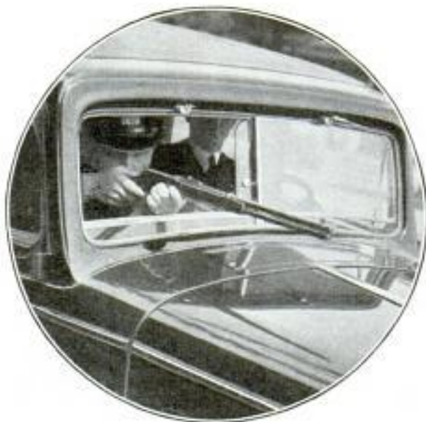
Sliding Windshield for Police Car Which Can Be Moved Back to Form a Port for Firing Gun
