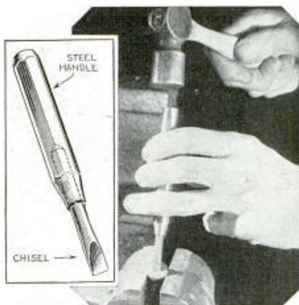
This Chisel Is Made of High-Speed Steel and Will Cut Through Most Materials Easily
