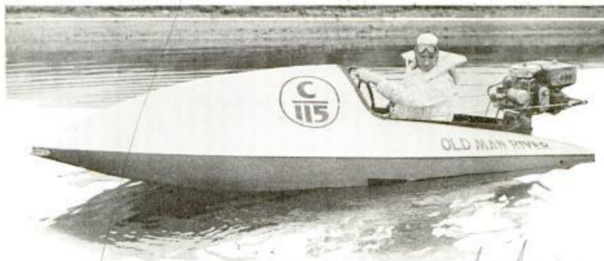
Here is the Latest Craft to Invade American Racing Circles; Judge Turnbull is Shown at the Wheel; Note Big Outboard Motor Which Drives the Boat; It is a Class X, 1,000-Cubic Centimeter Hydroplane
