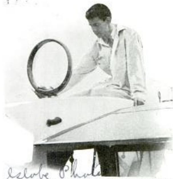
Hoop-Shaped Device Installed on Top of Plane Enables Pilot to Keep on Course
