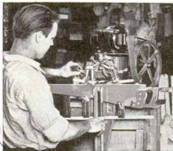
An Automatic Motor-Driven Saw Filer for Circular, Band and All Handsaws
