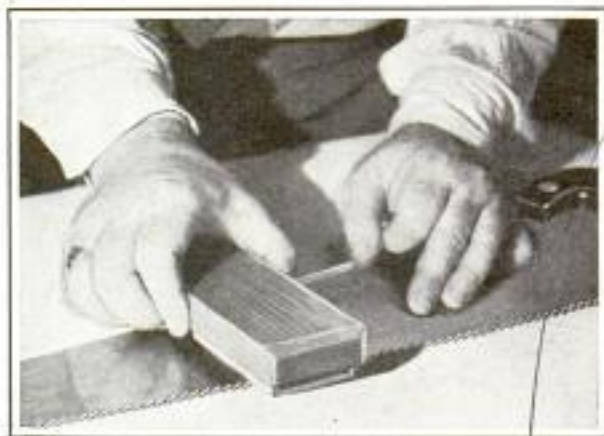
Fig. 14. Teeth of Both Hand and Circular Saws Should Be Lightly Dressed Down on the Sides
