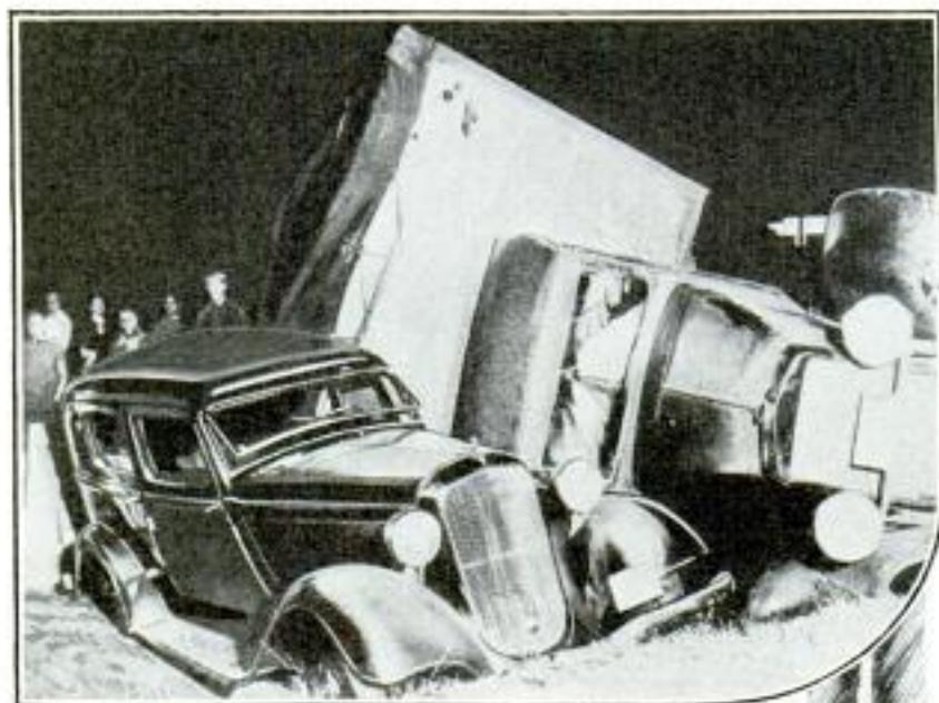
Photo of a Plymouth against Which a Truck Overturned; Note How Steel Body Resisted Impact
