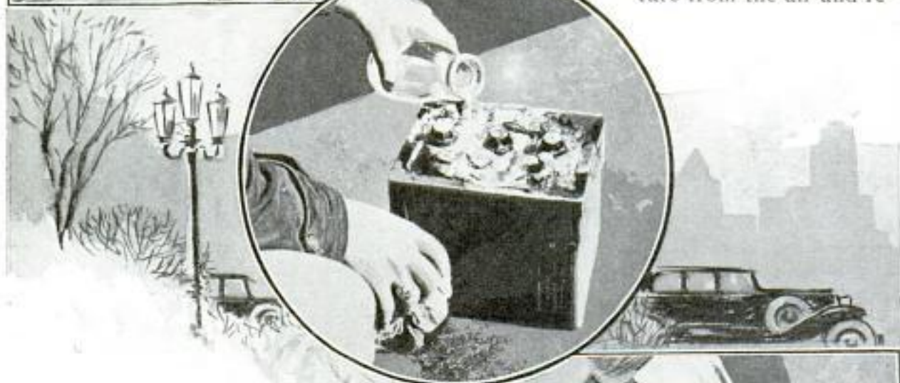
Above, Depressing Clutch in Cold Weather When Starting the Car Saves the Battery; in Circle, Cleaning the Battery with Soda and Water; Right, Polishing the Battery Terminal with Steel Wool
