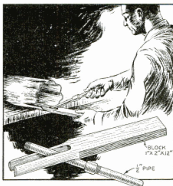
Corrugations in Conductor Pipe Straightened with Tool Made from Wood Block
