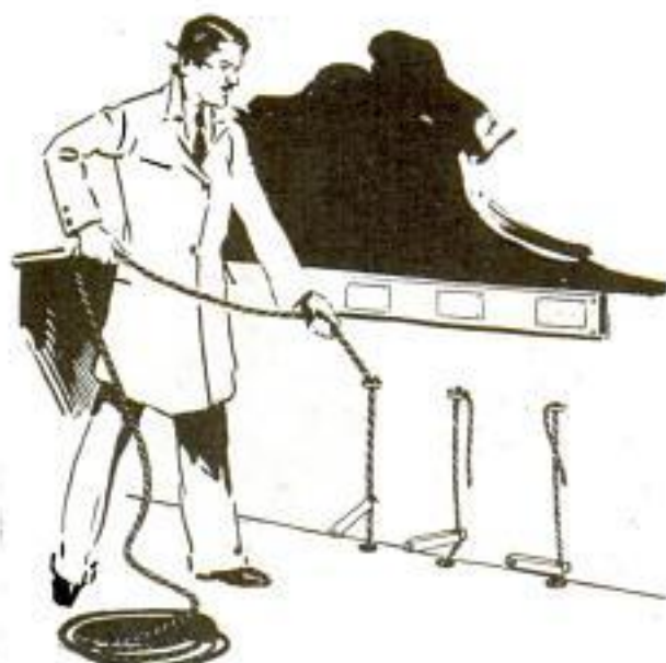
Wooden Stops Pivoted to Wall Hold Ends of Rope Pulled Up through Floor of Store
