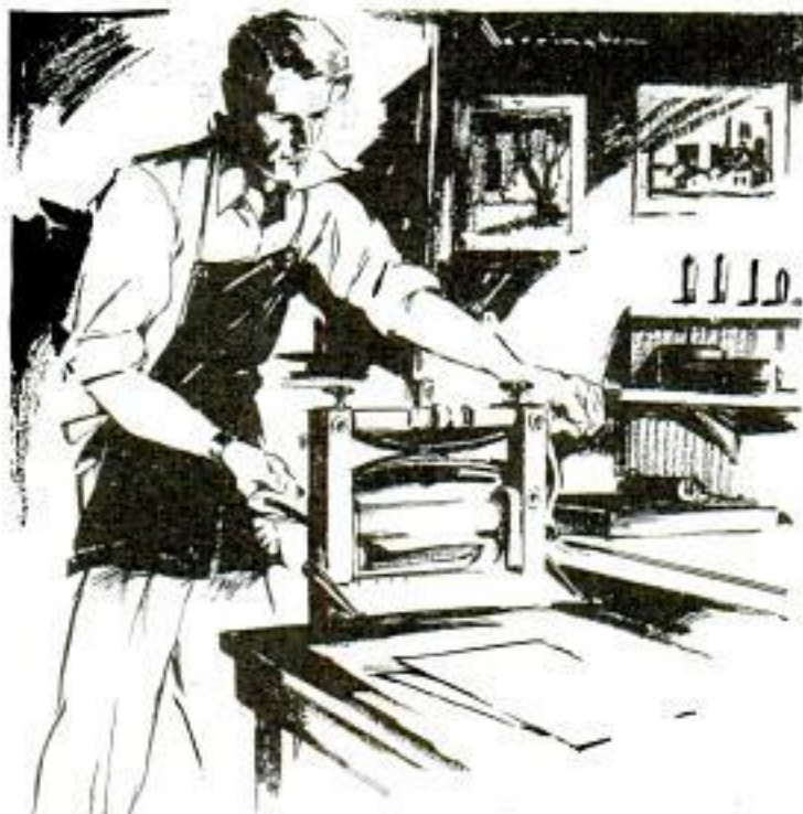
Fig. 12, Washing-Machine Wringer with Rollers Adjusted to Suit the Work Can Be Used as Press for Printing
