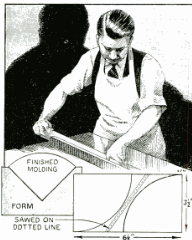
Simplified Method of Cutting Large Quarter Rounds, Using a Form and Only the Top Head of the Molder
