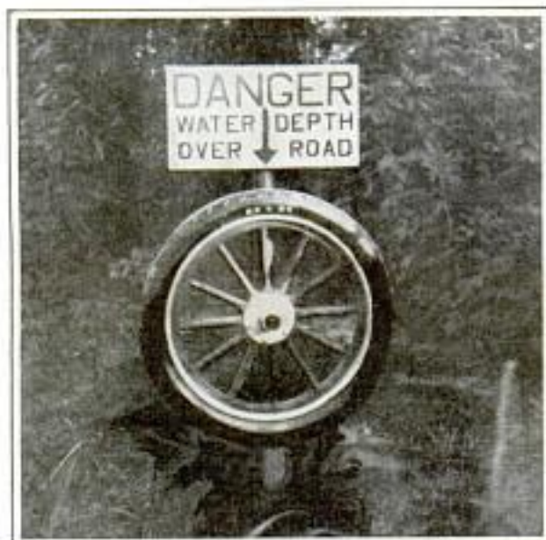
Auto-Wheel Water Gauge Which Shows Depth of Water over Road When Highway Is Flooded
