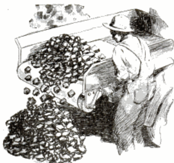
Heavy Canvas Fastened to Roller and Pulled over Truck Bottom Quickly Dumps Light Loads
