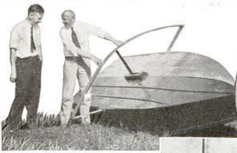
Left, Showing How Hydrofoil Is Attached to Boat: Circle, Inventor at the Wheel; Bottom, Boat Riding High and Almost Dry on Hydrofoils
