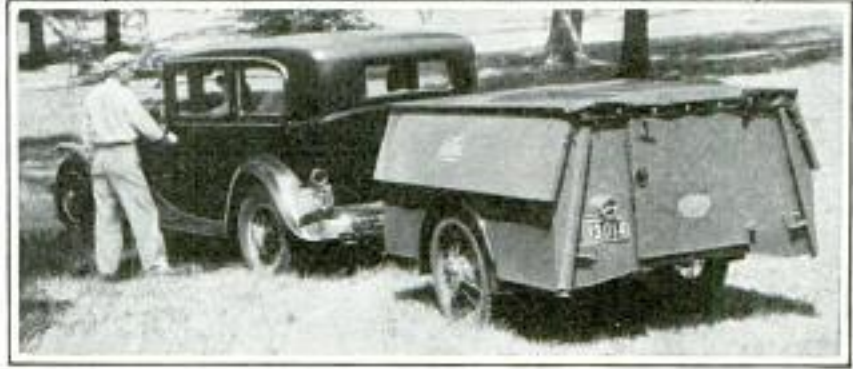
Auto Trailer Which Expands into a Small Home Accommodating Four Persons; a Kitchenette and Ice Box Are Built into the Unit
