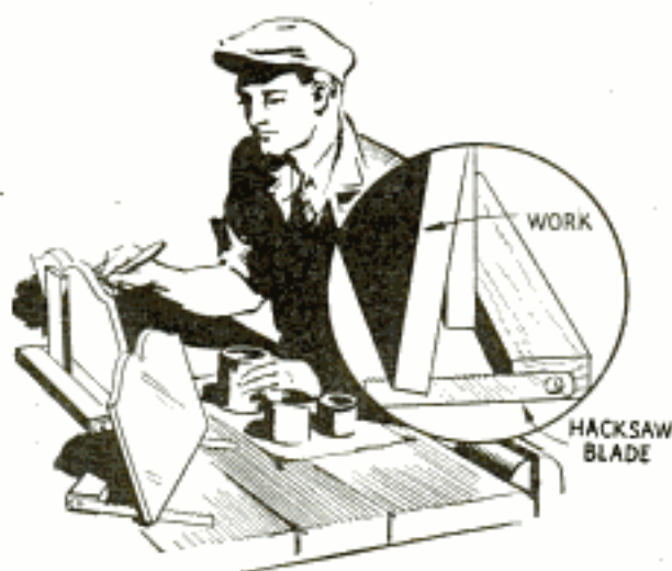
Rack Consisting of Wood Blocks and Hacksaw Blades Holds Freshly Painted Work While It Dries
