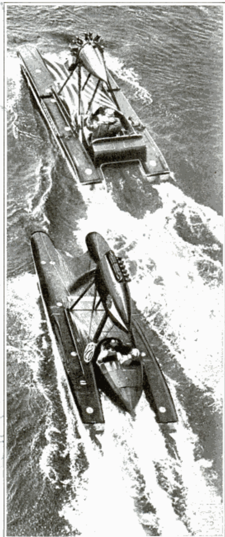
Streamlined Racing Boats of Italian Design Powered with Airplane Motors Which Drive Air Propellers
