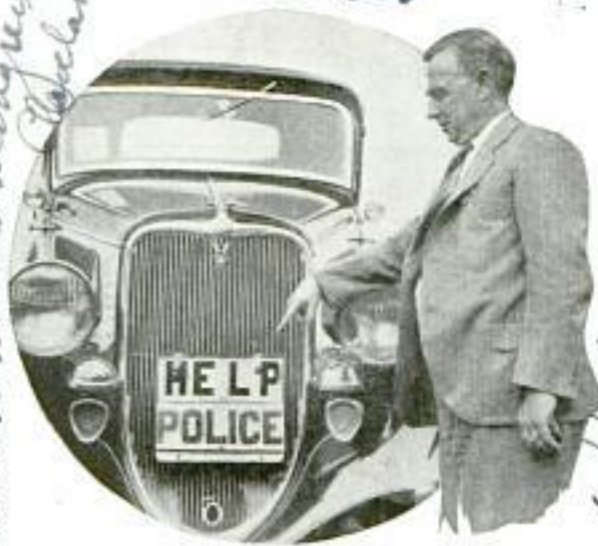
Burglar-Alarm Sign Which Tells Police Car Is Stolen; It Is Exposed When Starter Is Pressed
