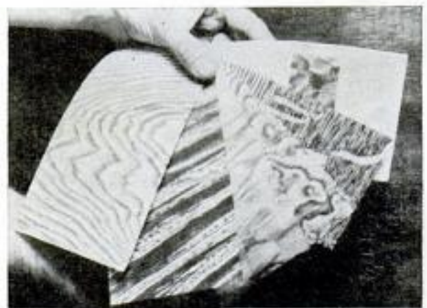
Transfer Paper Used to Impart Artificial Grain Designs to Various Kinds of Wood or Marble
