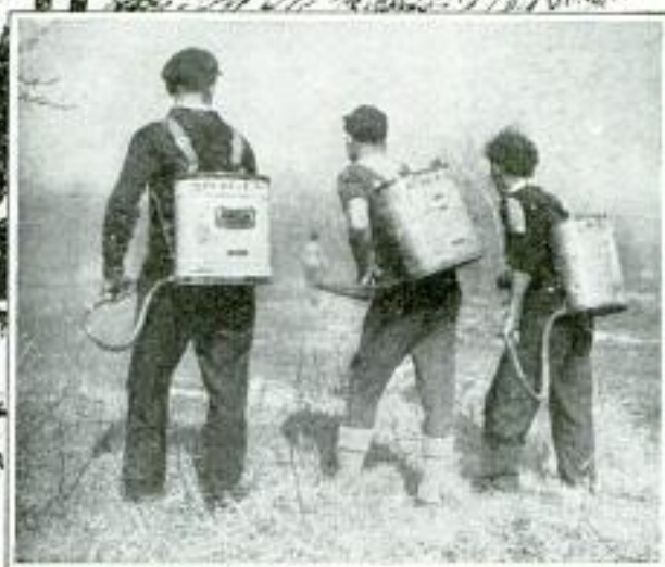
Individual Water Tanks for the Use of Rangers in Fighting Forest Fires Are Refilled by Carriers When the Supply Becomes Exhausted
