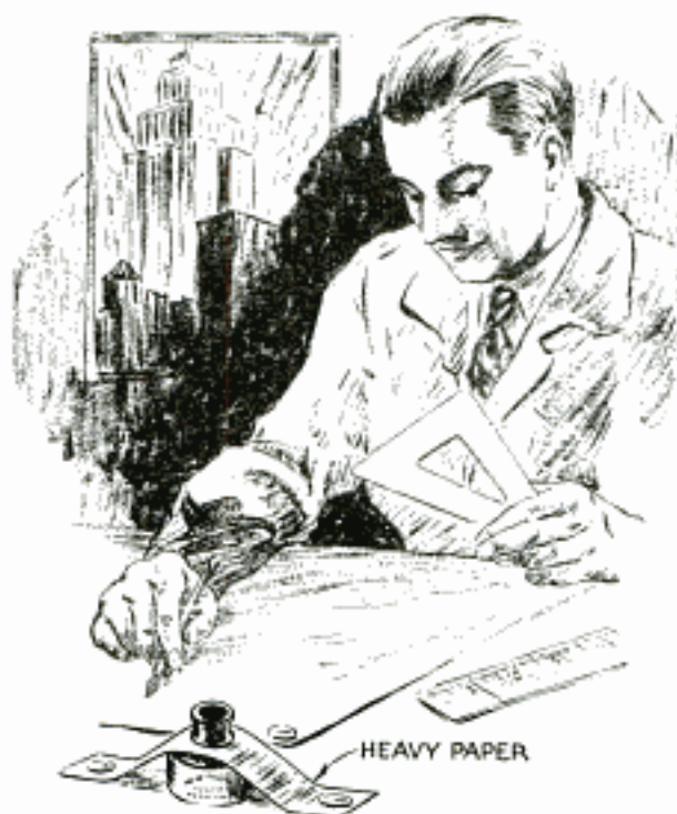
Ink Bottle Held Securely with a Strip of Heavy Paper Tacked to the Drawing Board
