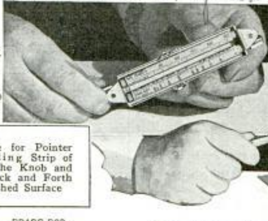
Above, Small Wooden Wedge between Core and Winding Stops Power Transformer Hum; Left, Master Die Fits across Face of D.C. Milliammeter to Supply Extra Scales for Many Readings
