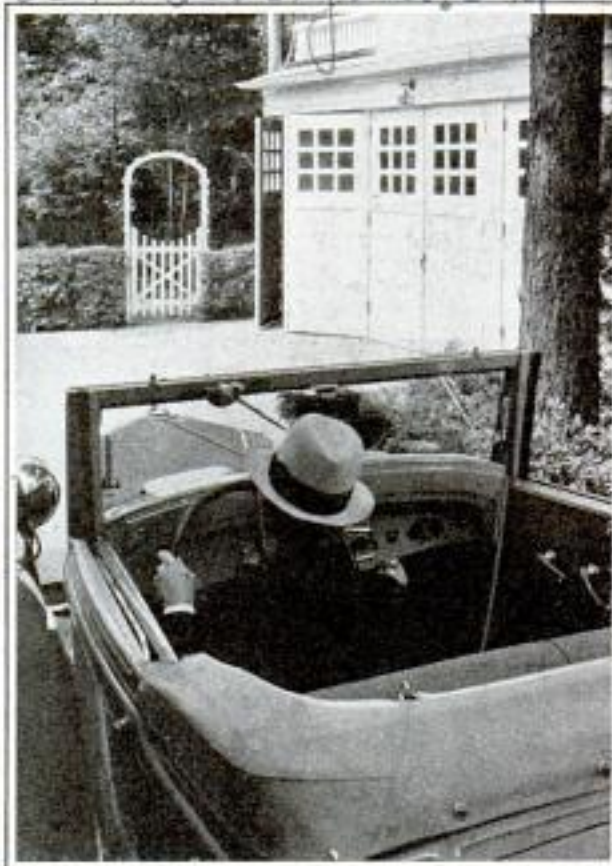
Driver Touches Button on Radio Control to Set in Motion the Apparatus for Opening Doors
