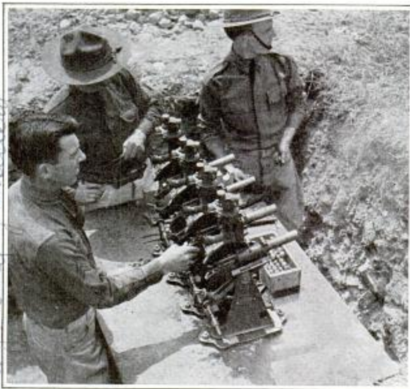
Artillerymen Firing Miniature "Cannon" Which Simulate the Action of Big Guns; They Are Made by Attaching Tubes to Sawed-Off Rifles
