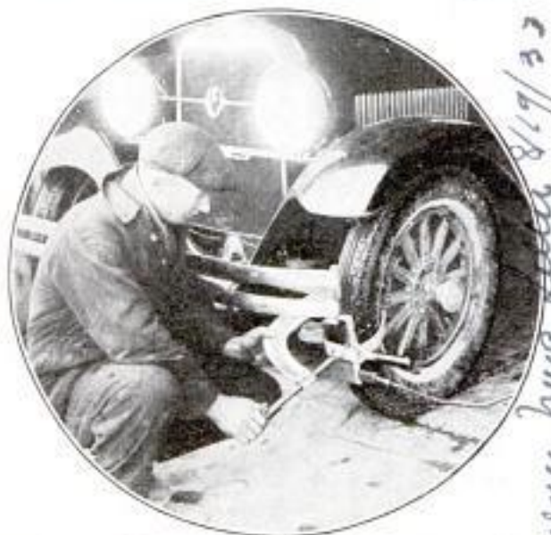
Vulcanizer Shown Applied to Tire on Wheel; Note That Tire Has Not Been Deflated
