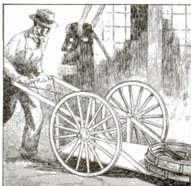
Cart for Handling Heavy Articles, the Load Being Raised Only a Short Distance from the Floor
