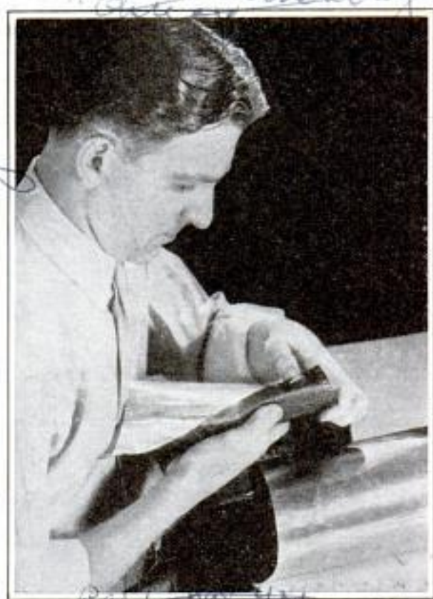
Building Paper Coated with a Thin Layer of Copper to Make It More Durable and Weatherproof
