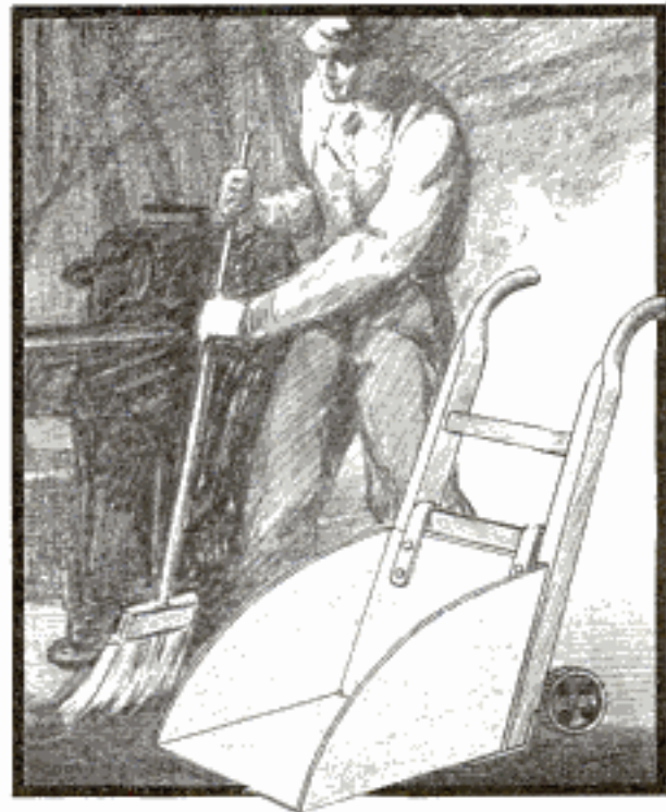
Sheet-Metal Scoop Attached to Hand Truck for Gathering Sweepings around Shop Machines
