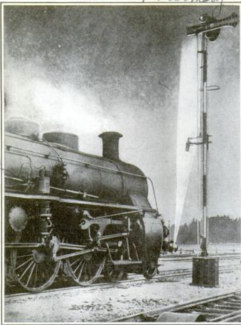
Light on Locomotive Is Reflected by Mirrors on Signal Tower Back to the Engine and Strikes Selenium Cell, Which Applies Brakes
