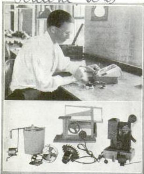
Above, Winding and Assembling Small Motor for Light Work. Below, Some of Its Applications
