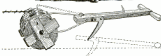
Fence Wire Can Be Strung and Stretched for Stapling to Posts with This Homemade Device
