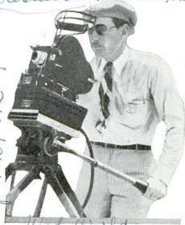
Wedge World Moving-Picture Camera for Timing Air Races to One One-Thousandth of a Second
