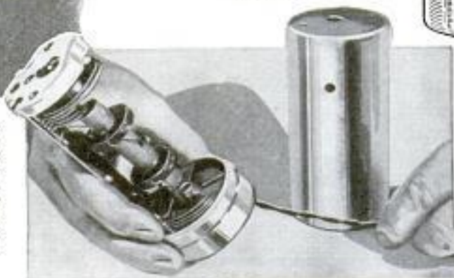
Plug-In Coil Winder from Discarded Pencil Sharpener; Cutters Are Removed and Tapered Wooden Block Is Drilled and Screwed to Shaft
