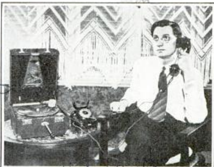
Using the "Teleskriptor," Which Records Both Ends of a Telephone Conversation on an Unbreakable Record
