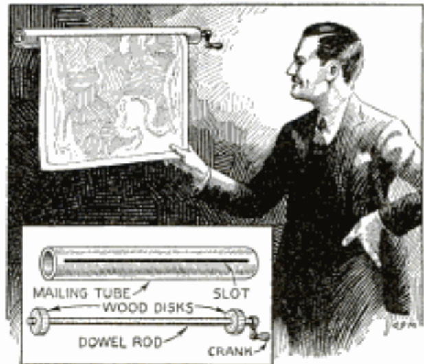
Large Charts in Shop Wound on Rod Inside Mailing Tube Protected from Being Soiled
