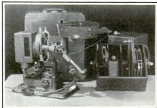
Cylinder on Top of Projector Contains Apparatus Which Automatically Rewinds Movie Film
