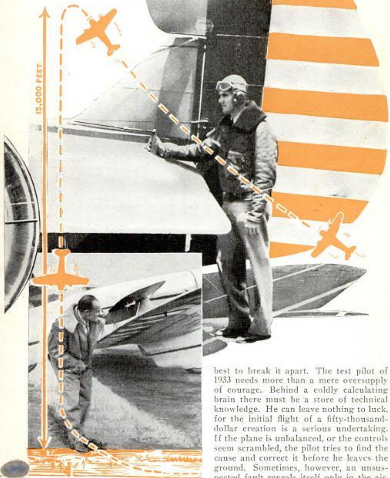
Above, Play in Elevator Fittings May Cause a Disastrous Flutter in Tests; Below, Eddie Allen, Test Pilot, Examining Offset Ailerons He Tested
