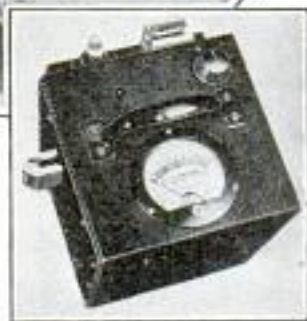
Above, Making a Test with the Oil-Sediment Meter and Allowing Motorist to See Result; Below, the Compact Instrument for Testing the Motor Oil
