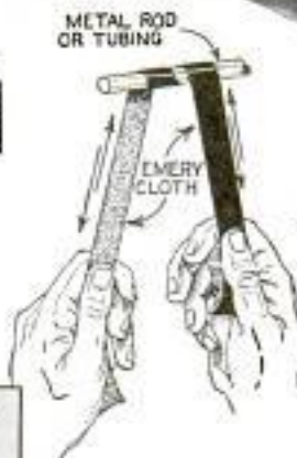
Upper Left, Hook-Up for Using Phones with A.C. Receiver; .001 Mfd. Condenser Prevents Hum; Switch Cuts Out Speaker; Below, Removing Insulation from Litz Wire for Soldering
