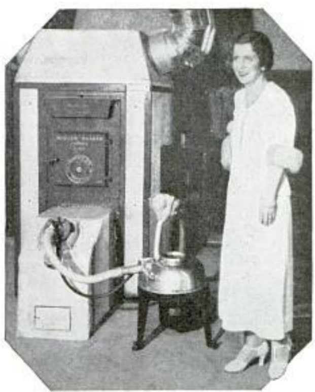
Furnace Hopper Which Grinds Up the Coal as It Is Fed Automatically into the Heater
