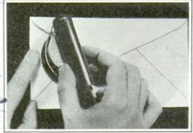
Envelope Sealer Which Moistens Flap at One Stroke and Seals Container on Return Stroke
