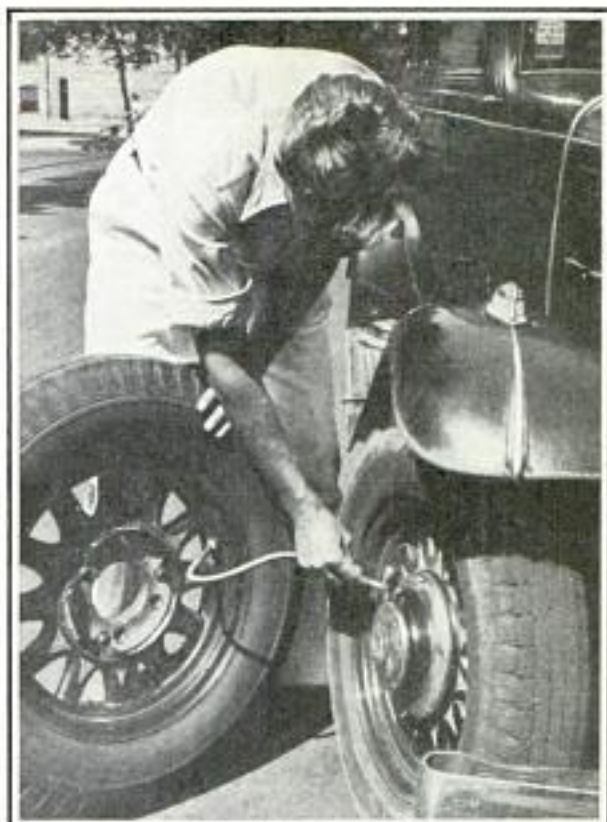
Using Air-Transfer Tube to Divert Part of Air from an Inflated Tire to a Flat One
