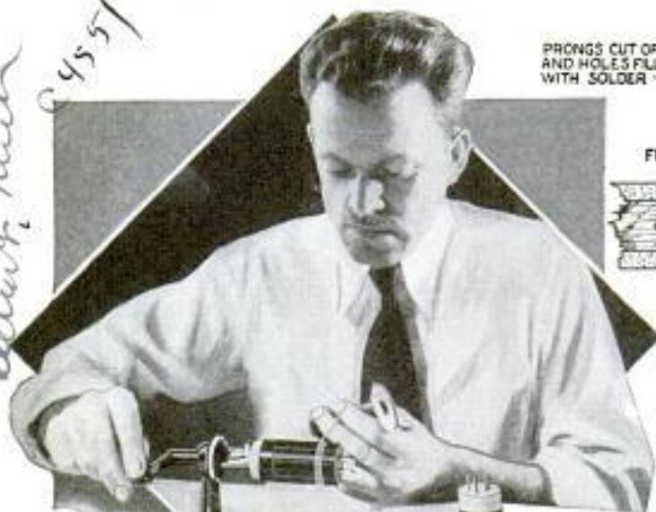
Plug-In Coil Winder from Discarded Pencil Sharpener; Cutters Are Removed and Tapered Wooden Block Is Drilled and Screwed to Shaft
