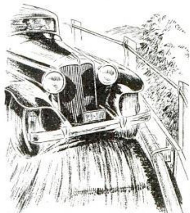
Highway Guard Consisting of a Revolving Pipe Which Tends to Shunt Car Back into Road
