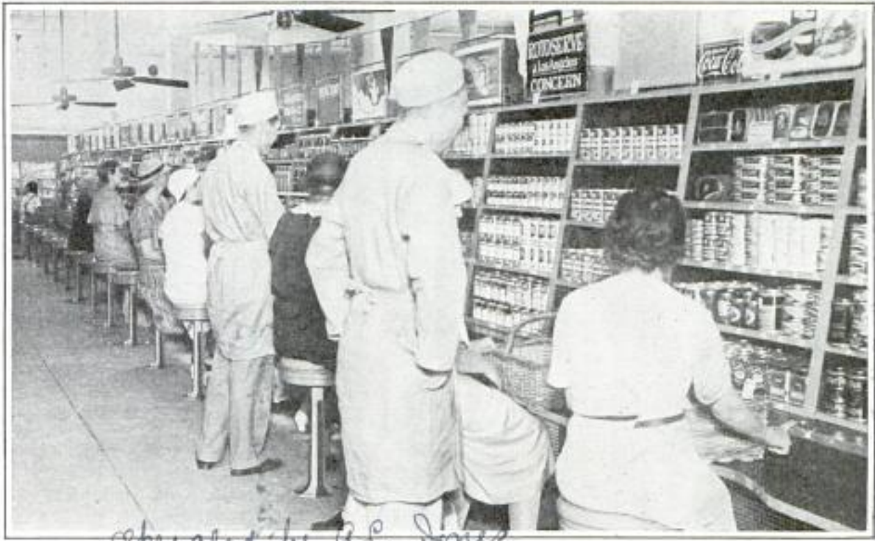
"Merry-Go-Round" Grocery Store with Revolving Shelves Which Move the Entire Stock Past the Customers Every Few Minutes; the Shelves Are Moved by a Small Motor
