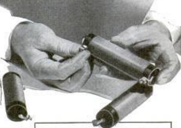
Above, Heavy-Duty R.F. Choke Coils for Amateur-Wave Bands; 235 Turns of No. 30 D.S.C. Wire Is Wound on Form 1 In. in Diameter and 4 1/4 In. Long; Left, Using Emery Cloth to Remove Scores from Condenser Shaft or for Polishing Copper Tubing
