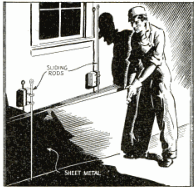
Stocks of Sheet Metal Stacked on Edge Along Wall and Held by Sliding Rods
