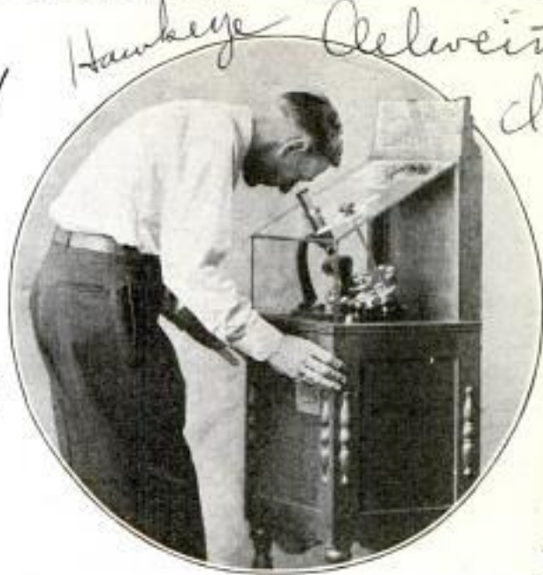
Coin-in-Slot Microscope Which Exposes One of Ten Subjects When Money Is Deposited
