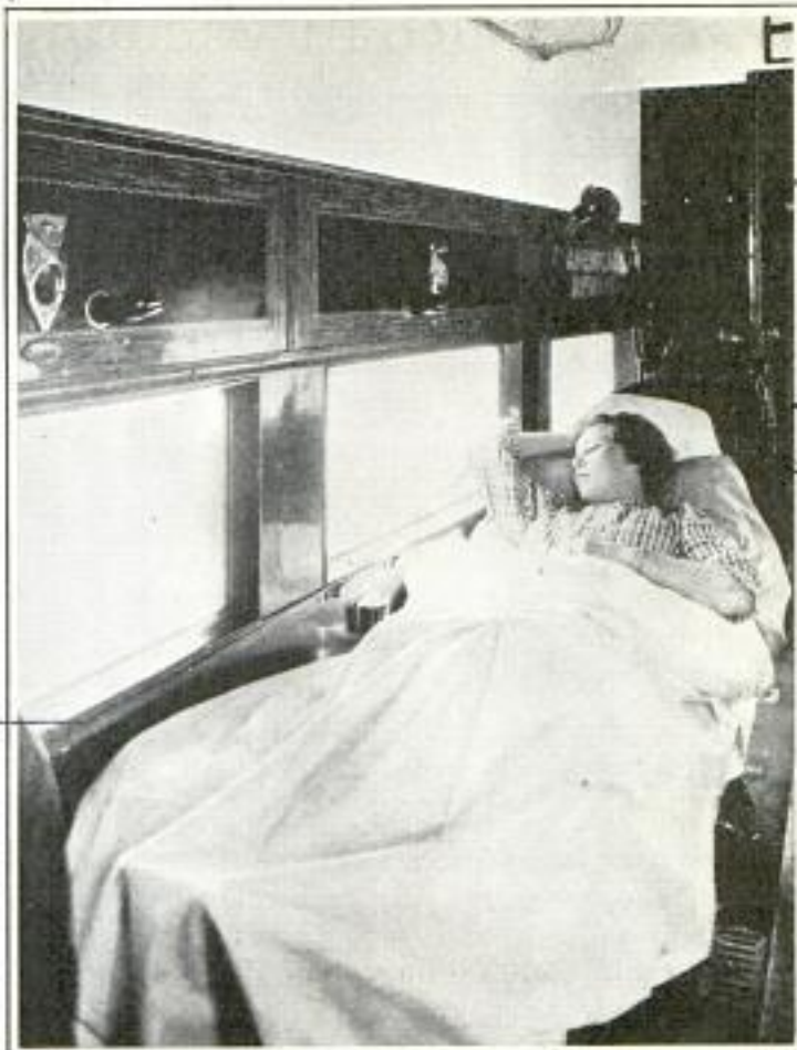
Two Seats of Modern Transport Plane Are Folded Together to Make This Comfortable Berth for Night Flyers
