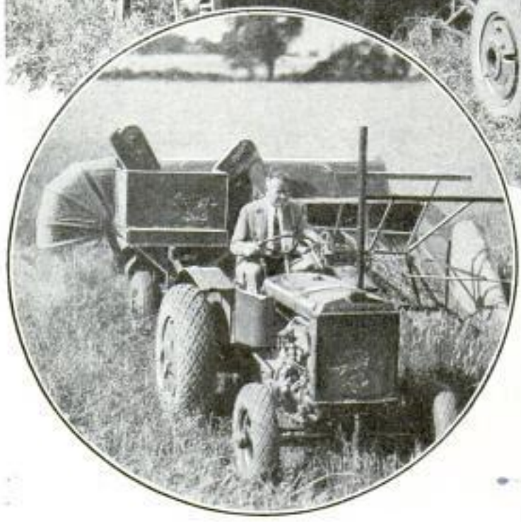
Two-Wheeled Baby Combine Being Operated by Tractor with Pneumatic Tires; It Cuts a Five-Foot Swath
