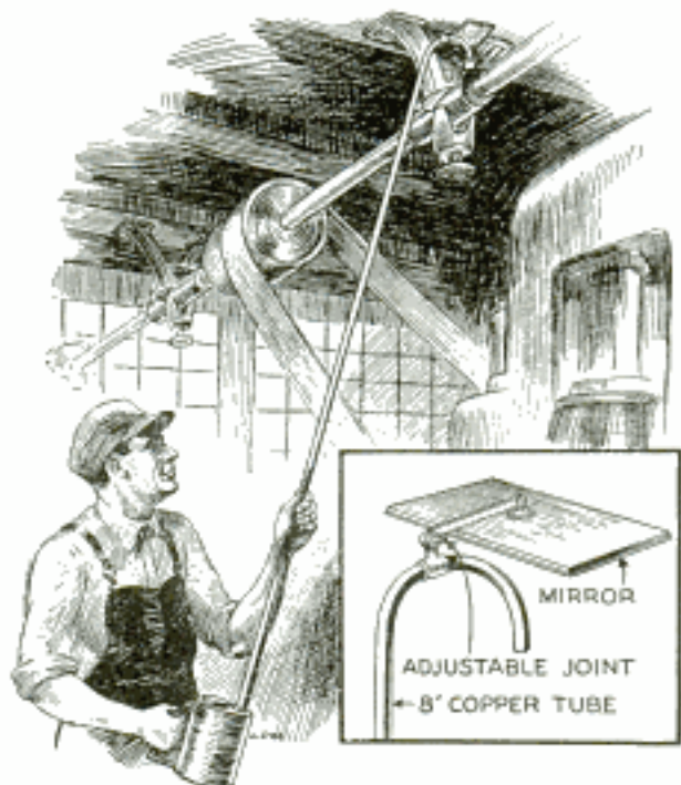
Overhead Bearings Oiled from Shop Floor by Means of Long-Spouted Oilcan and Mirror
