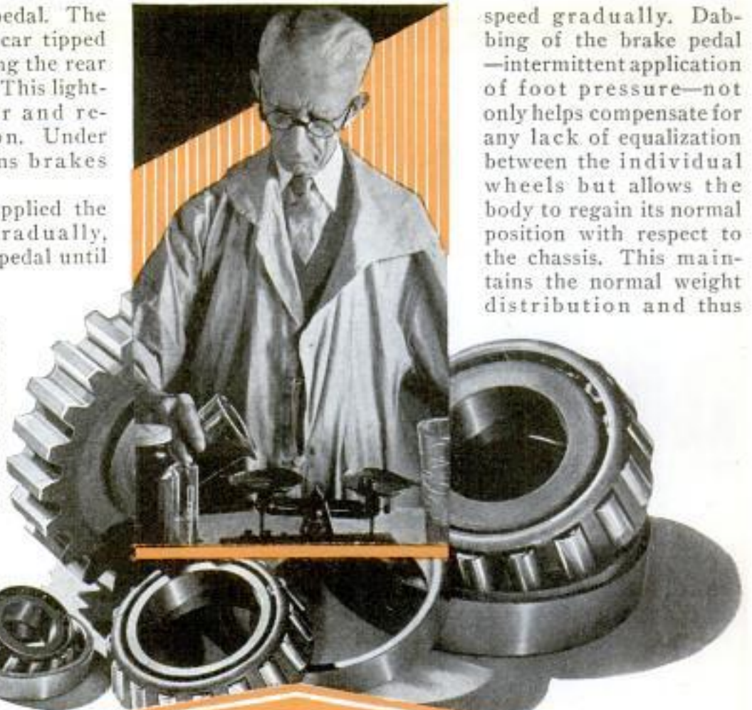
Right: Testing Properties of an Automotive Lubricant Which Deposits a Thin Film of Metal on Bearings and Other Surfaces, Protecting against Wear and Corrosion; Below: Point Chart for the Metal-Plating Lubricant
