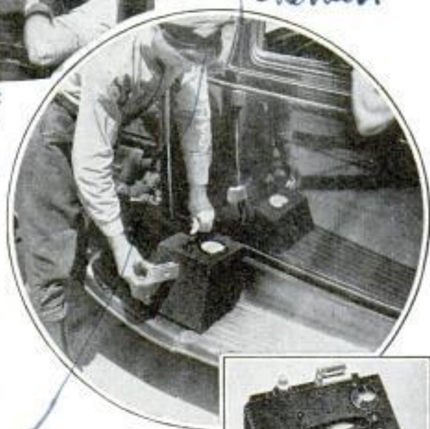
Above, Making a Test with the Oil-Sediment Meter and Allowing Motorist to See Result; Below, the Compact Instrument for Testing the Motor Oil
