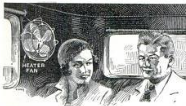
Heater Fan Removed and Fitted with Wire Guard Used to Circulate Air inside Closed Car
