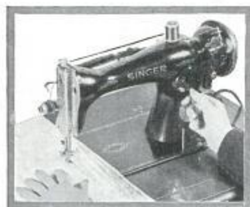
Above, Small Shift Lever Controls Machine so That Operator May Sew Forward or Backward, Eliminating Turning the Cloth to Reverse the Line of Sewing; Below, Self-Starting Siphon Removes Cream from Milk; Siphon Is Inserted into Bottle of Settled Milk to Withdraw the Cream Suitable for Whipping; When the Cream Is Off, the Device Stops Working
