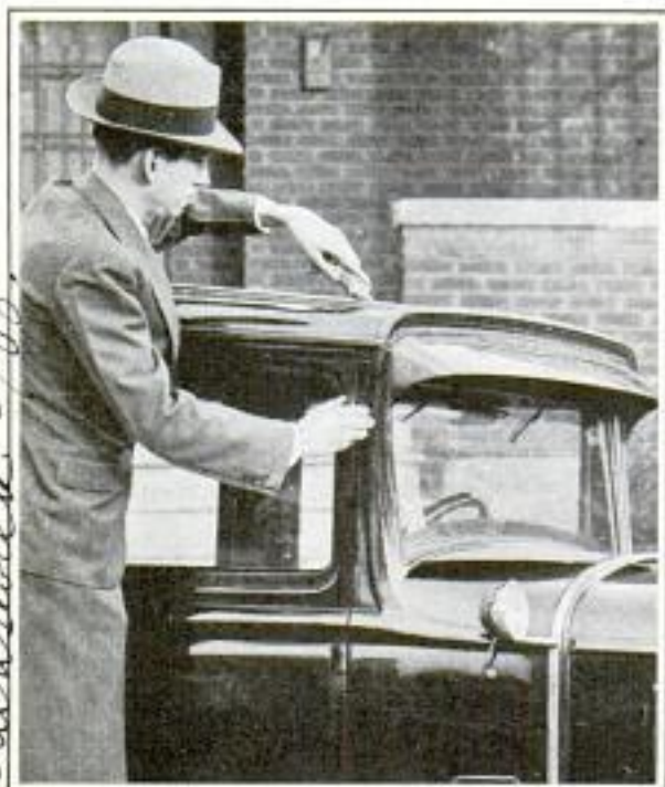
Easy to Apply. This Waterproof Cement for Sealing Cracks in Auto Top Comes in Handy Tube
