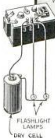
Fig. 10. This Homemade Light-Sensitive Unit Can Also Be Installed in the Alarm System
