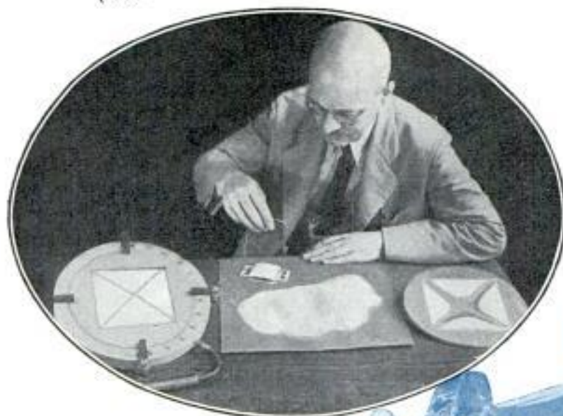
Top, Left, Fine Dry Sand Helps Scientist to Find Out What Goes on Inside a Piece of Steel When It Is Stressed Beyond Its Elastic Limit; Top, Right, Cutting Natural Quartz Crystals in New Way to Improve Control over Radio Station's Wavelength; Bottom, Left, Power Grid Tube That Handles 900,000 Watts, the Power of a Locomotive
