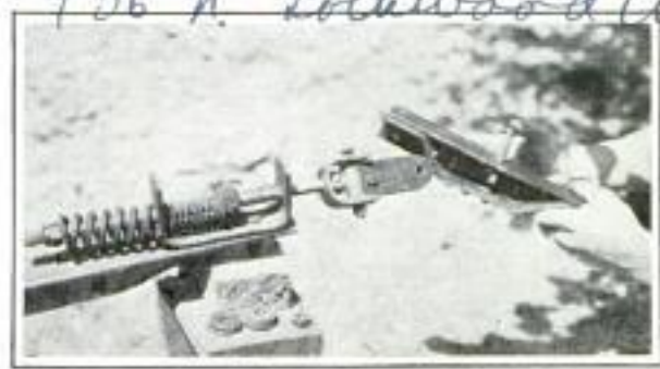
Hookup for Trailer Is Absorber for Road Shocks; Auto Is Connected at the Right
