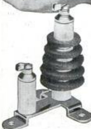
Left, Heavy-Duty R.F. Choke Has Continuous Universal Winding Divided in Five Tapered Sections, Base Insulated for High Voltage; Right, When Suitable Tube Sockets Are Not at Hand for Experimental Hook-Ups, Dry Plywood May Be Drilled for Tube Prongs; Sub-panel Connections Are Soldered Directly to Tips
