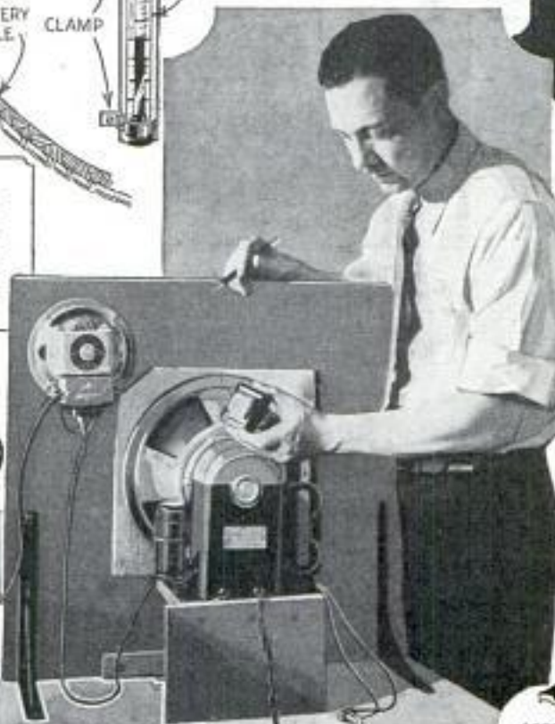
Upper Left, Insulating Small Resistor in Portable or Auto Receivers; Right, Universal Output Transformer Replaces Transformer in Any Dynamic Speaker; It May Be Used to Match High and Low-Range Speakers for Dual Operation
