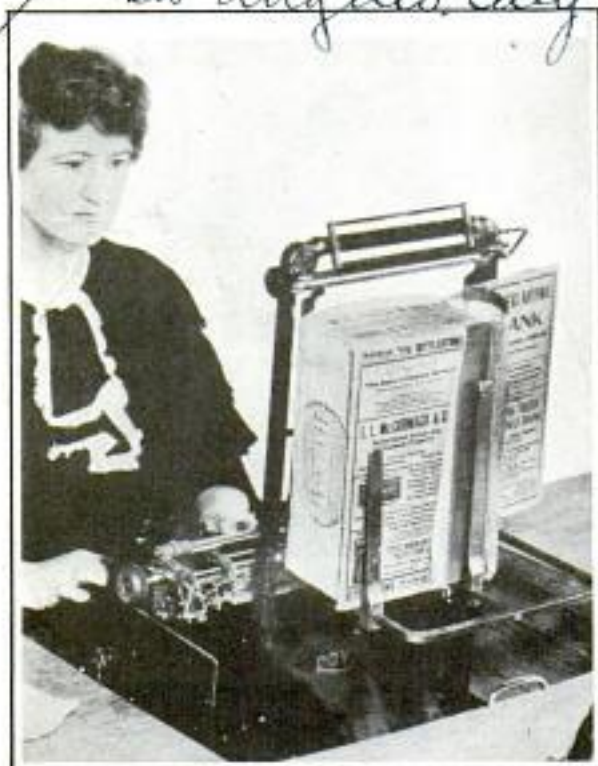
Here's How New Copy Holder for Typewriter Handles City Directory or Other Heavy Book
