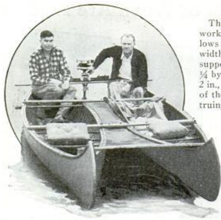
Consisting of Two Canoes Bolted Together, This Outboard Craft Was Used on a 1,000-Mile River Tour
