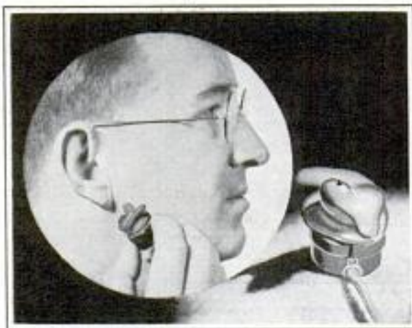
Made to Fit the Average Ear. This Inexpensive Earpiece Is an Aid to the Hard of Hearing
