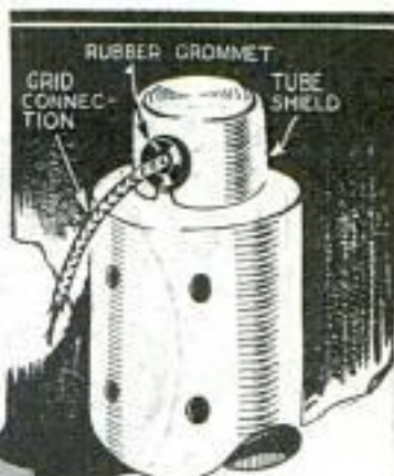
Above, Rubber Grommet Insulates Screen-Grid Lead to Prevent Vibration Noises; Below, a Handy Mounting Strip for Small Fixed Resistors
