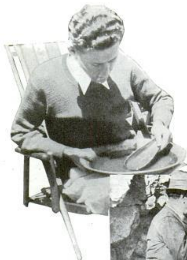
Above, When Concentrates from Panning Contain Gold, a Trail of Colors Is Exposed by Dribbling Material from Horn Spoon into Pan of Water
