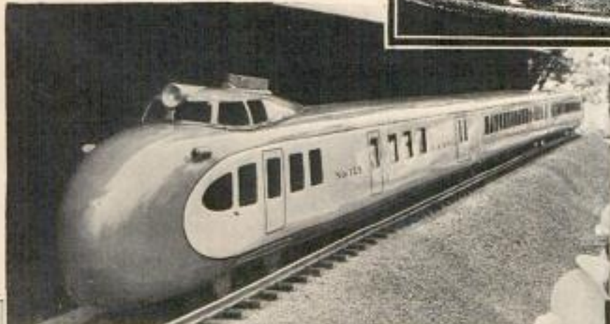
Above, Drawing of Driver at Controls; Left, Model Shows How Super-Train Will Appear; Note the Flowing Lines That Reduce Wind Resistance
