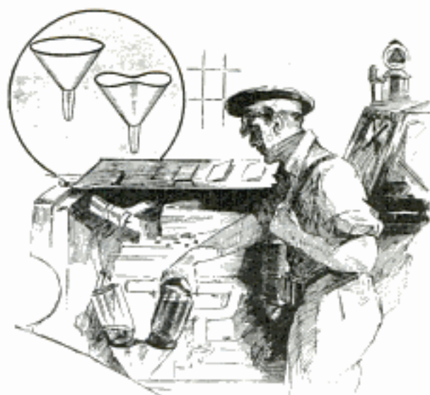
Funnel Bent to Take Two Bottles of Oil Saves Time in Filling Auto Crankcase
