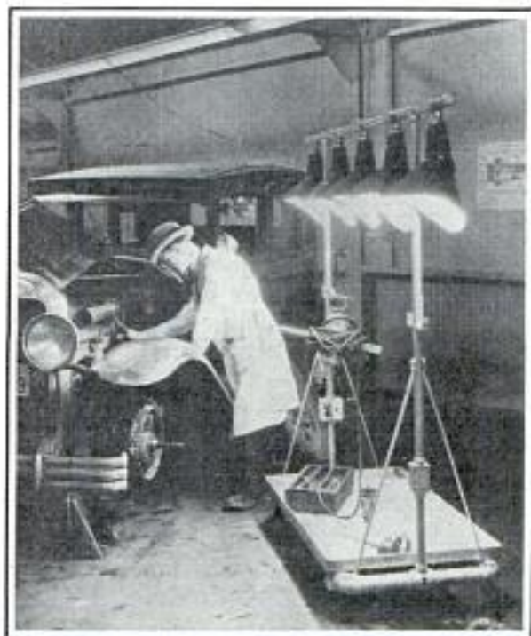
Rack Holding Battery of Lights for Repair Work Also Has Space for the Mechanic's Tools.
