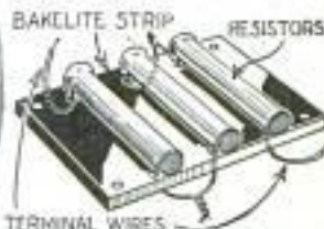
Above, Rubber Grommet Insulates Screen-Grid Lead to Prevent Vibration Noises; Below, a Handy Mounting Strip for Small Fixed Resistors
