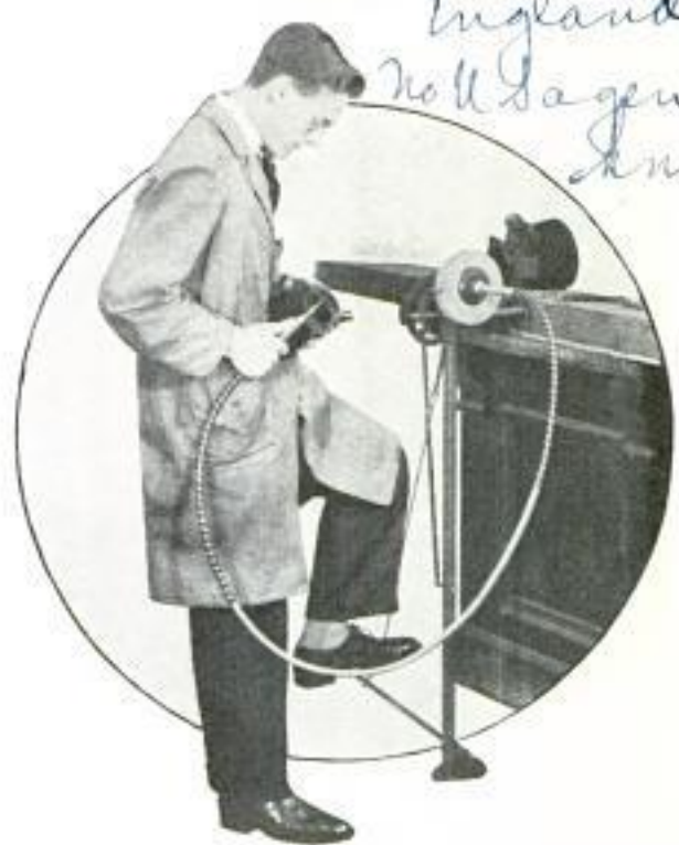
Grinder in Combination with Grindstone Is Shown in Operation; Note the Foot Drive
