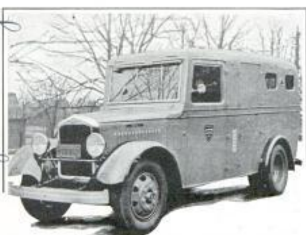
Armored Car Covered with Aluminum Shell and Insulation Material to Keep Bullets from Rebounding
