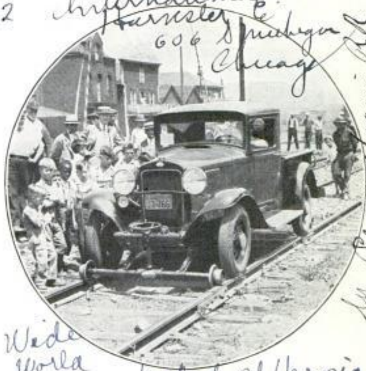
Flanges in Front and Behind Keep Pneumatic-Tired Truck on Rails; Flanged Wheels Can Be Elevated for Operation on Road
