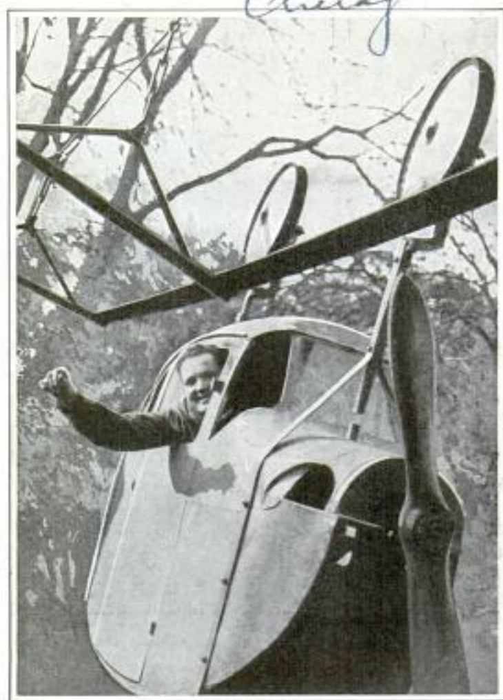
Inventor Is Shown in Overhead Rail Car That Attains High Speed; It Is Driven by a Propeller on Power from the Rail
