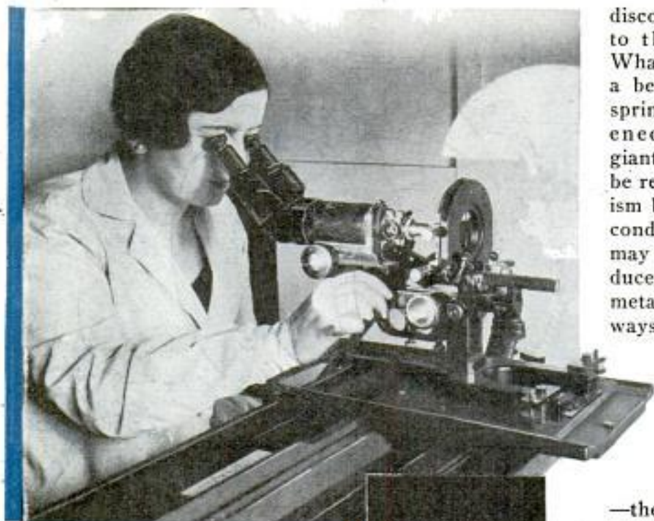
Metals Tell All About Themselves under This Photo-Micrograph Apparatus
