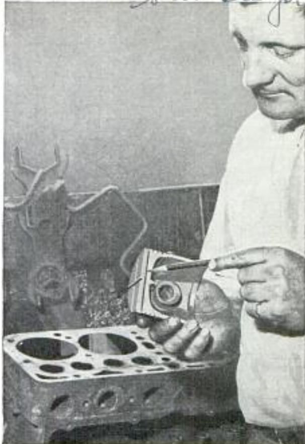
Piston Insulated with a Layer of Asbestos to Reduce Heat and Improve Motor Performance
