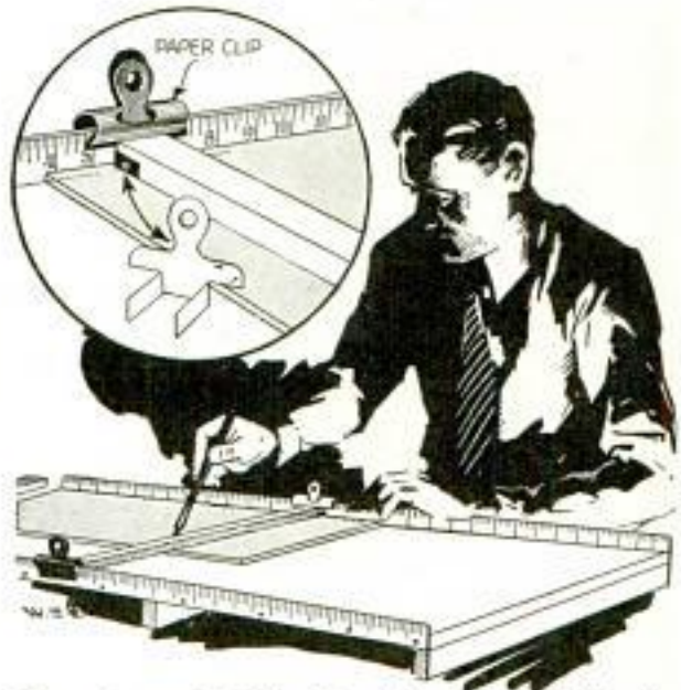
Glass Cutters' Table Has Adjustable Straightedge Which Is Clipped to Graduated Guides along Edge
