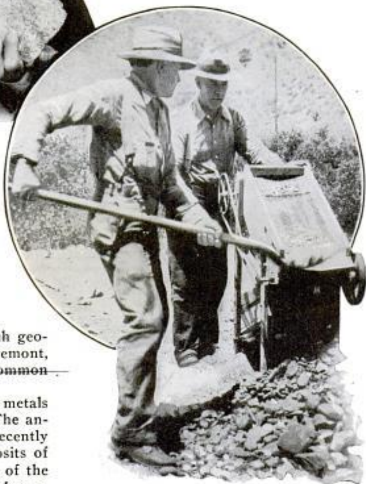
Top, Piece of Lepidolite Containing Five Rare Metals; Below, Screening Method of Prospecting for Gold Which Cannot Be Used with the Rarer Metals
