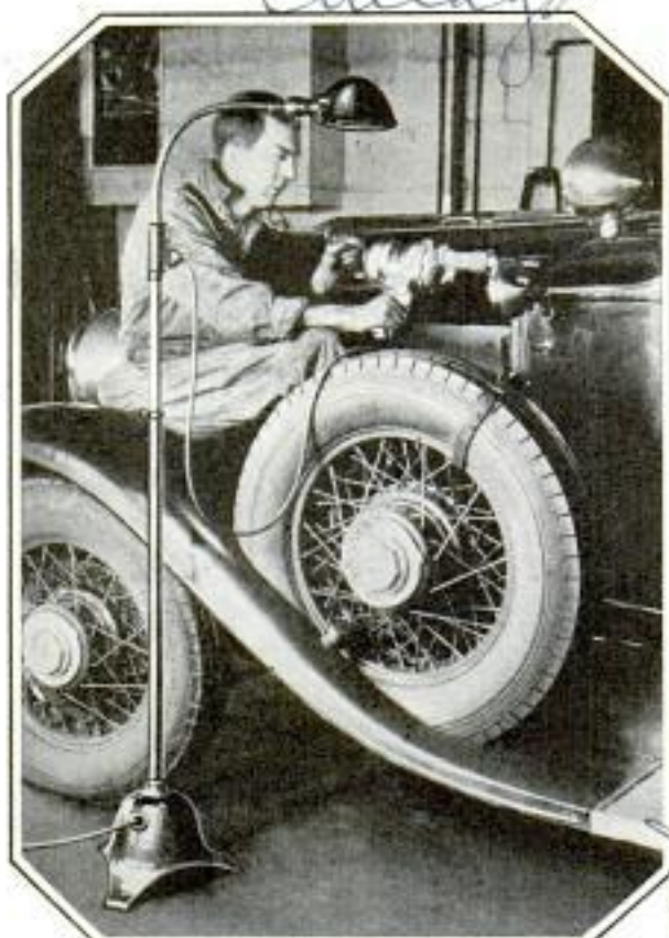
This Convenient Stand Provides Illumination for Auto- Repair Work; It Can Be Adjusted Easily
