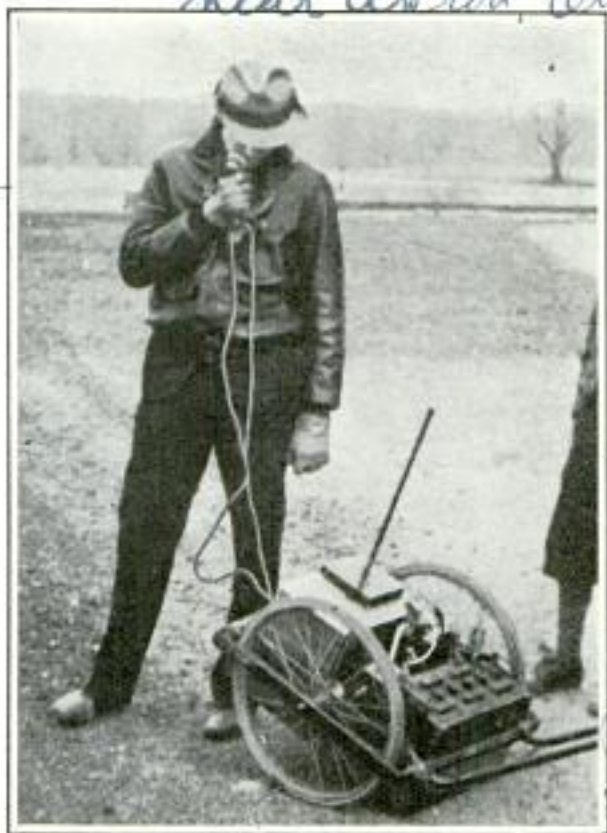
Small Broadcasting and Receiving Set on Wheels Used for Communicating with Airship in Flight
