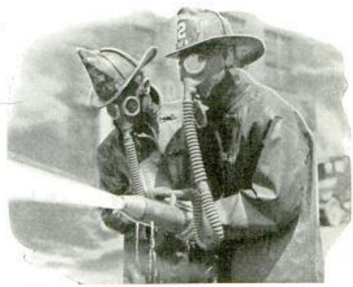
Firemen Are Shown Wearing Masks to Which Washed Air Is Supplied by Two-in-One Nozzle on the Hose
