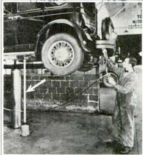
Arrow Points to Auxiliary Jack Which Rocks Car While It Is Greased, and Locates Squeaks
