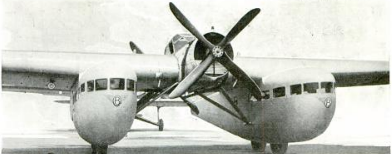
Latest Air-Transport Plane in Europe; Note How the Twin Cabins Are Constructed under the Wings, with the Cabin Roof as Part of the Wing; Each Cabin Has Two Wheels
