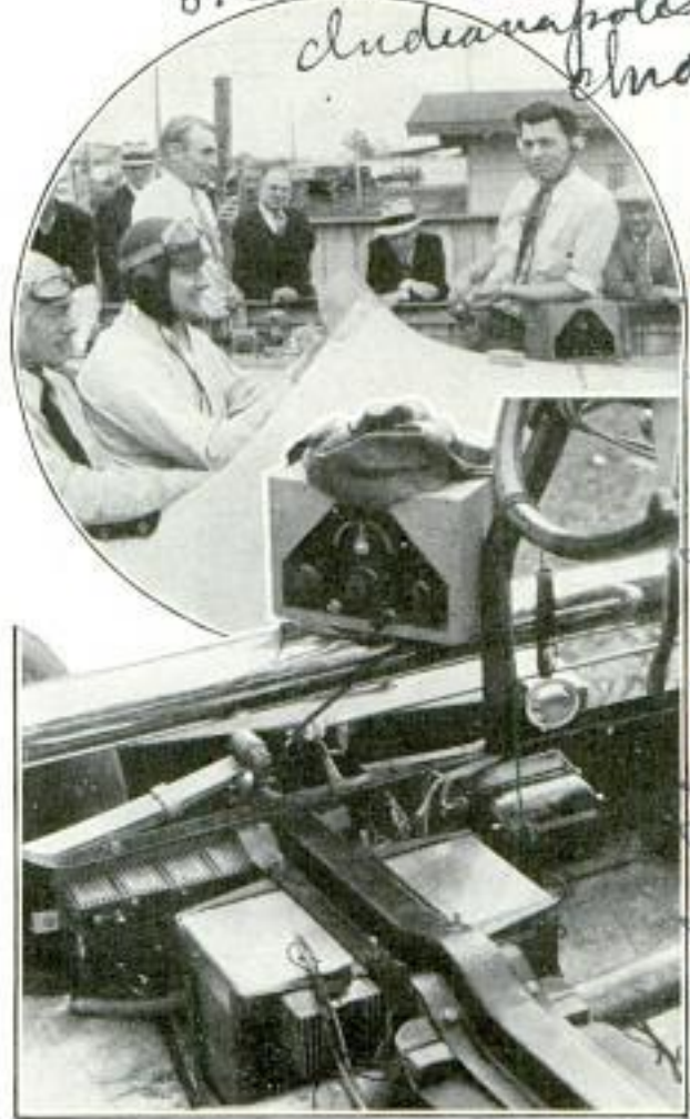
Top, Racing Driver Wears Headphones; Bottom, Two-Way Radio in Car for Talking to Pits
