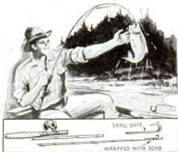
Small Gaff on End of Casting Rod Helps in Landing Large, Fighting Fish
