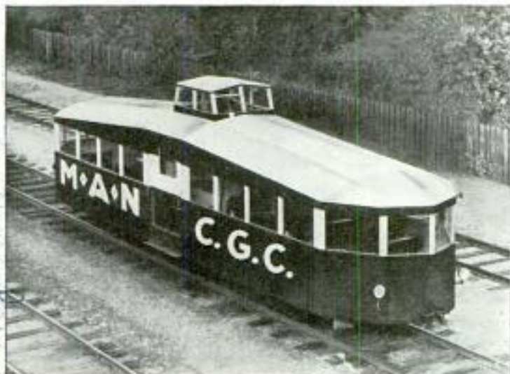
Diesel Railway Car with Control Cabin Mounted above the Roof and in Center of the High-Speed Vehicle
