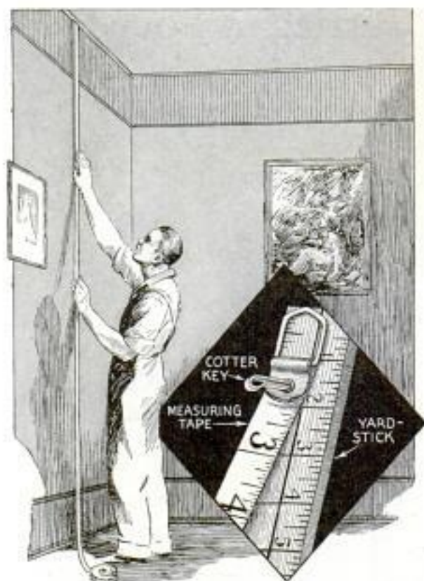
Height of Walls Quickly Measured by Using Measuring Tape Attached to Yardstick
