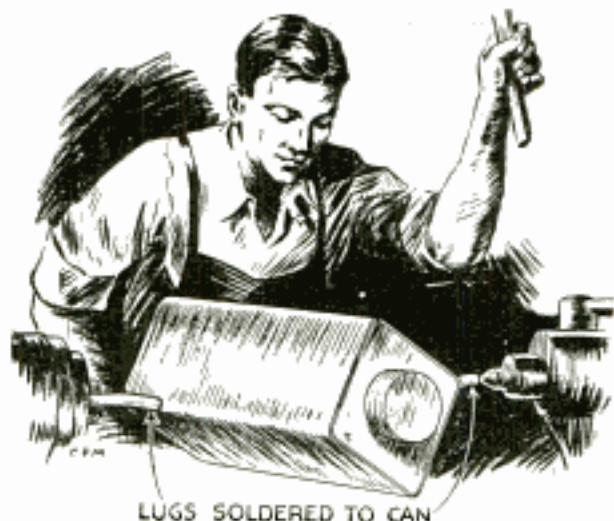
LUGS SOLDERED TO CAN Large Tin Can with Lugs Soldered to Two Corners Used as Tumbling Barrel in Your Lathe
