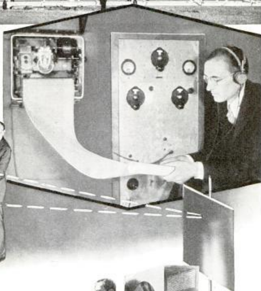
Top, Rotating Directional Antenna Used by Karl Jansky in Seeking Causes of Static Interfering with Short-Wave Communication; Right, Mr. Jansky Listening in as Static Recorder Operates on 14.6-Meter Wavelength
