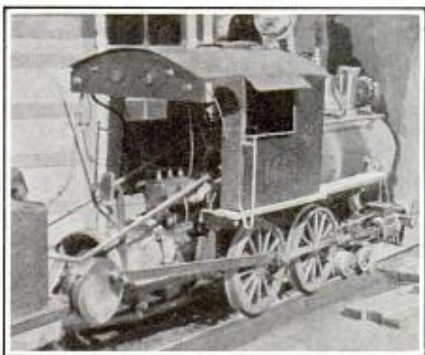
How Gasoline Engine Was Installed in Amusement-Park Locomotive When Steam Power Failed
