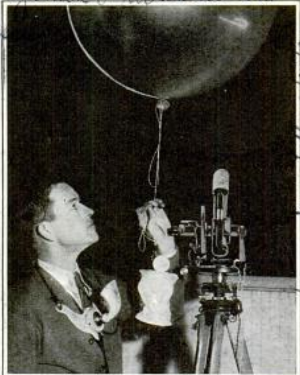
Night Observations Are Made by Attaching Paper Lantern Containing Candle to Weather Balloon
