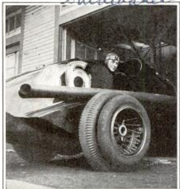
Extra Wheel on Racing Car Which Protects Driver Testing Tires in Case of a Blowout
