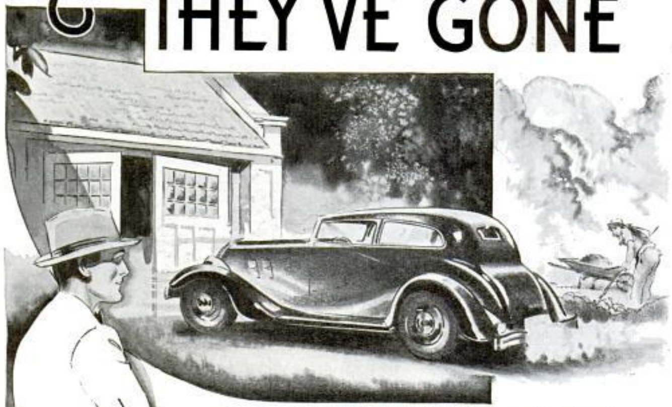
Car Driving Itself Out of Garage after Motor Has Been Started and Doors Opened Automatically
