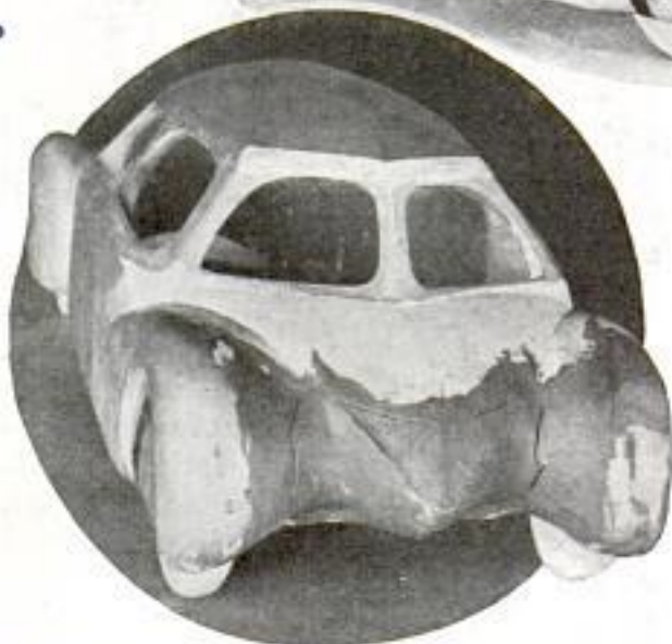
These Models Show How Streamlines Will Help Reduce Wind Resistance in Future Automobile
