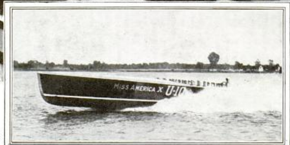
Here is Gar Wood's "Miss America X" in Action: Her Thirty-Eight-Foot Hull Carries Four Huge Motors Delivering More Than 6,000 Combined Horsepower to Drive Her Forward
