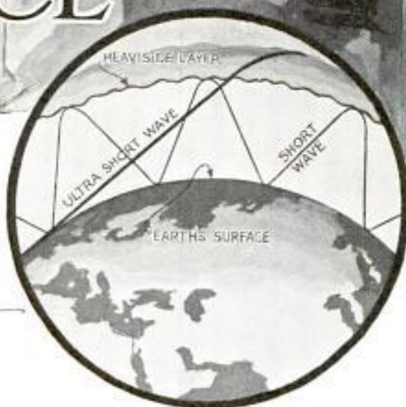
Top, Drawing of Possible War-Time Scene Showing "Beam-Casting" Station; Inset, How Ultra-Short Waves Fly into Space, Never Returning to Earth
