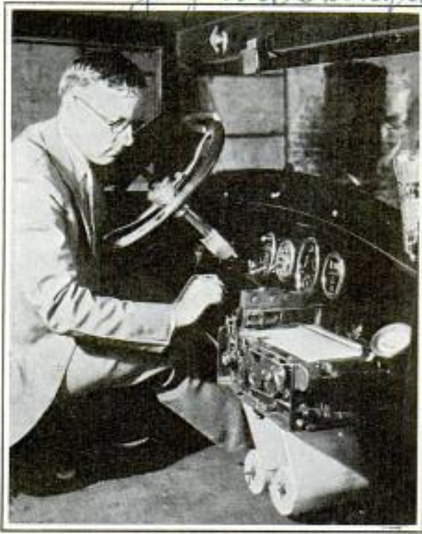
As Auto Moves Along, Moving Pencils Write the Road's Condition on Paper Shown in Recorder
