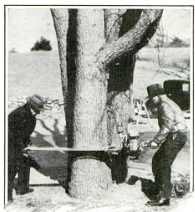
Tree-Felling Saw in Operation; Note Small Motor at Right Controlled by Cycle-Type Handle
