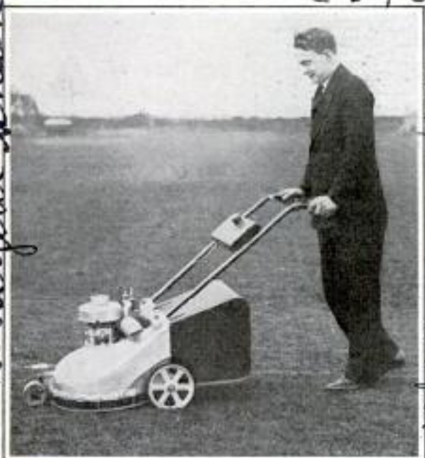
Grass Is Sucked into Basket as It Is Cut; Small Motor Does All the Work
