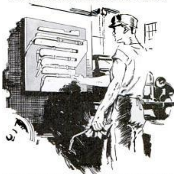
Welding Torches Are Always at Hand When Needed if They Are Kept in This Holder
