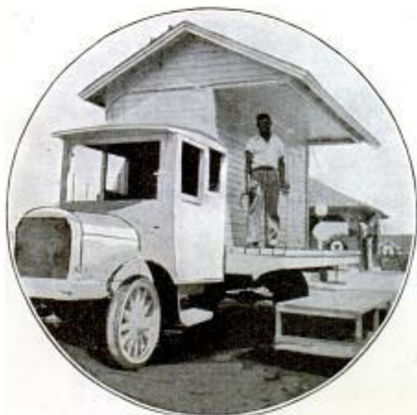
Small Insulated Ice House Mounted on Old Truck Provides Portable Ice Station
