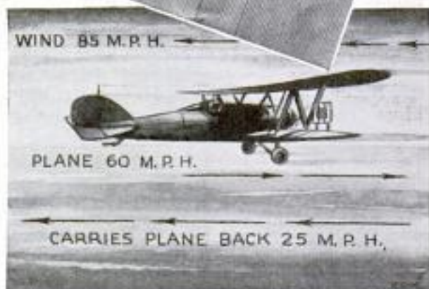
Top, Left, Ready for Flight into the Clouds; Right, Weather Record Made by the Aerograph; Bottom, How Strong Wind May Drive Plane Backward
