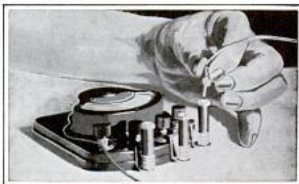
Some of Tiny Fuses Containing a Platinum Filament One-Thirtieth the Diameter of Human Hair
