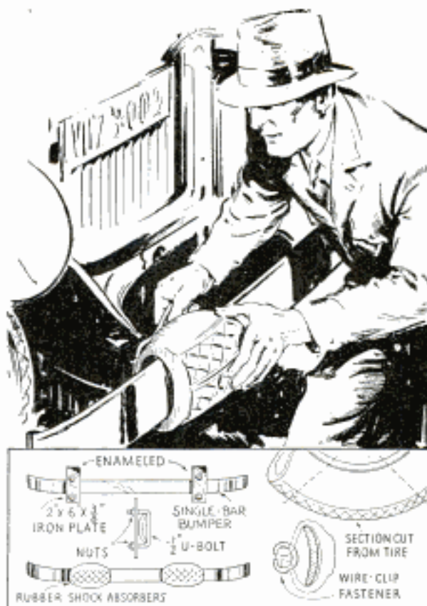
Guards of Rubber or Metal Help to Prevent Locking of Car Bumpers
