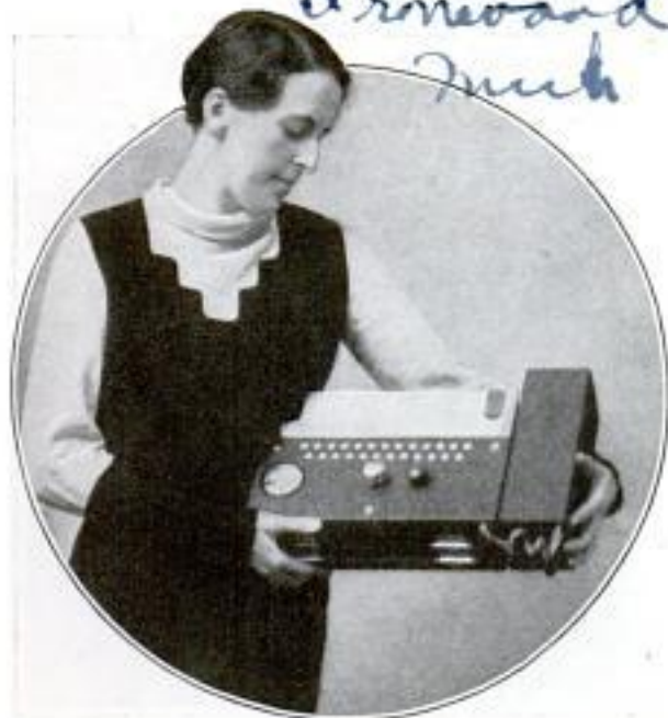
Showing How Machine Grades Student's Test Paper; Light Flashes if Answer Is Right
