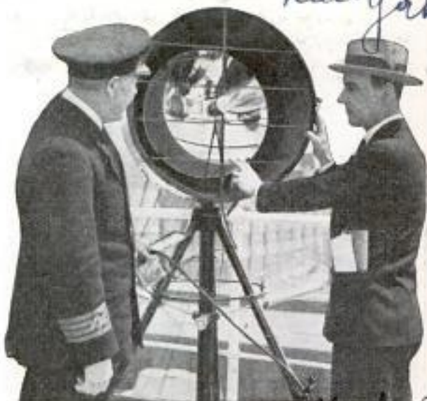
Demonstrating the "Fog-Eye" Which Reveals Obstacles in Ship's Path When Weather Is Murky
