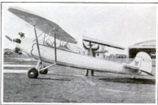
Monoplane with Removable Cover Back of Cockpit, Thus Providing a Space for Baggage
