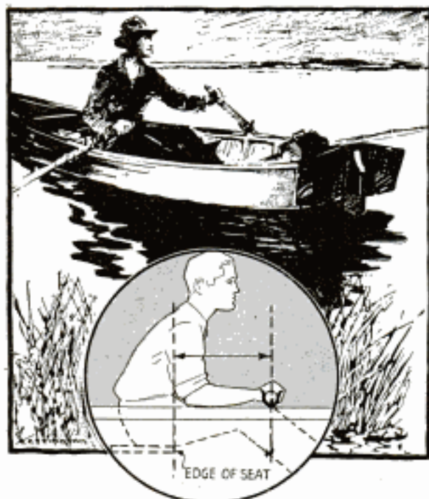
Location of Oarlocks Determined by Measuring from Edge of Rowing Seat with Forearm
