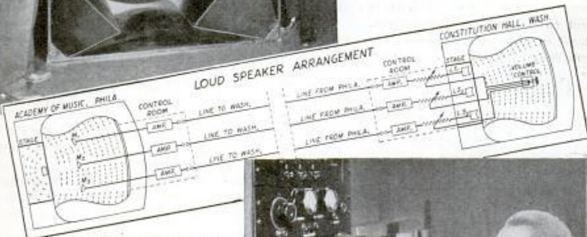
Above, Low and High-Frequency Loud Speakers for Transmission System, and Diagram of Speaker Arrangement; Right, Doctor Stokowski at Control Board
