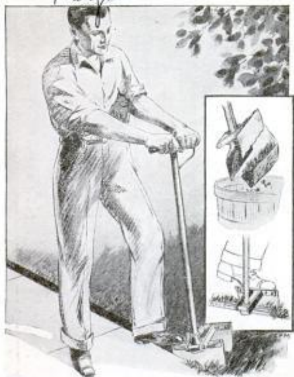
Lawn Edger with Cutter Operated by Foot; the Tool Eliminates Stooping and Sweeping Up Cuttings
