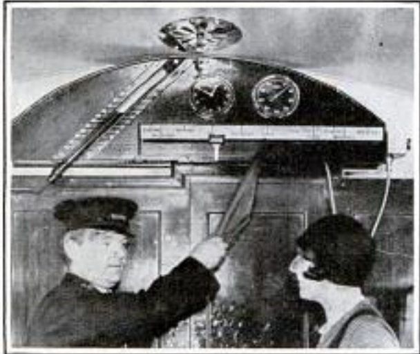
Indicator in Railway Coach Which Shows Passengers the Next Station as Train Approaches It
