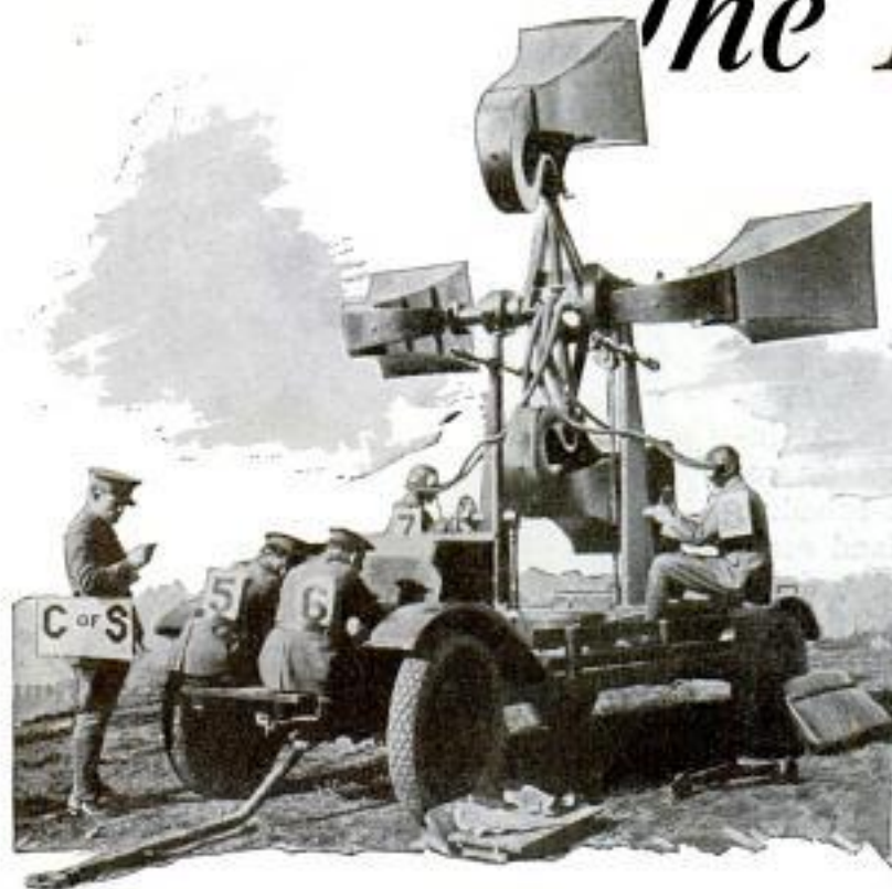
Left. Sound Locator for Determining Position of Hidden Plane; in Circle. Two Boeings Used by Army Lower Photo Courtesy U. S. Army Air Corps
