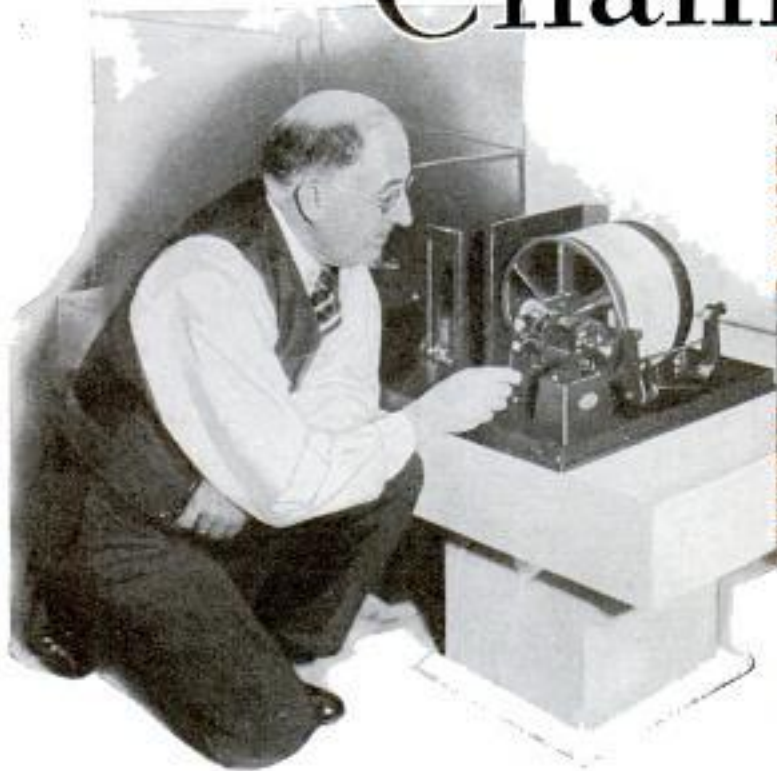
Left, Accelerograph Ready to Be Installed to Record Earthquake Shocks; Top, Two Accelerograms Showing Violence of Recent California Disturbance; Upper Record Was Made at Los Angeles, Where Shocks Were Not Severe, and Lower Record at Long Beach, Where Tremors Were Severe
