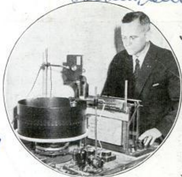
This Apparatus Can Read Your Newspaper to You; It Changes Printed Writing into Sound
