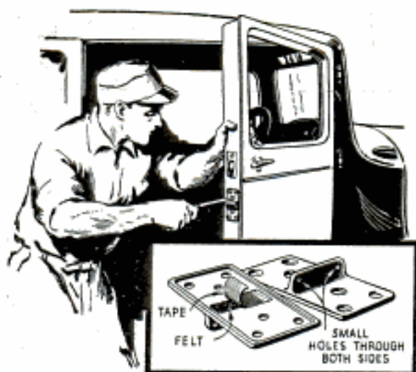
Oil-Soaked Felt in Hollow Part of Antirattler Eliminates Squeaks in Car Door
