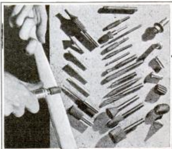
Using Rotary File to Shape Hammer Handle, and Various Types Employed for Carving or Engraving
