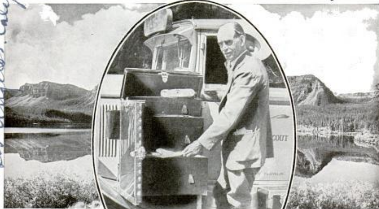
In Oval, Drawers for Clothes; Below, Stove Slides Out Ready for Instant Use
