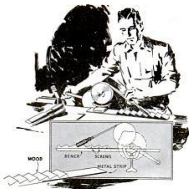
Simple Device Aids in Holding Tools at Proper Angle to Grind Bevel on Cutting Edges
