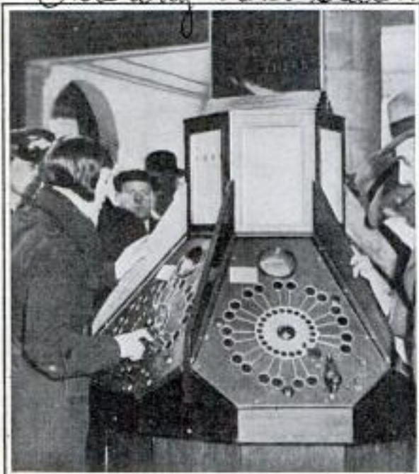
By Operating Dial, Travelers Are Given Information on Subway-Train Schedules and Fares
