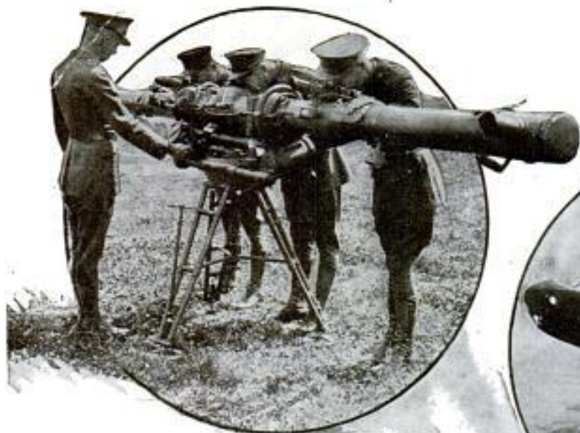
Above, This Instrument Measures the Height of Plane from Ground
