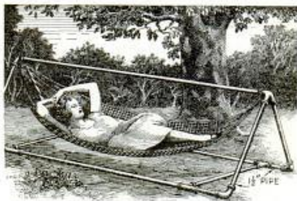
Hammock Support Made of Pipe and Fittings Is Light and Rigid, and Easily Moved
