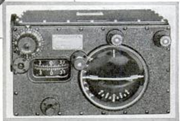
Sperry Automatic Pilot on Instrument Panel, and Sketch Showing How It Controls the Plane
