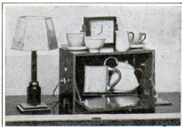
Clock on Cabinet Turns on Light and Rings Alarm When Coffee Is Ready
