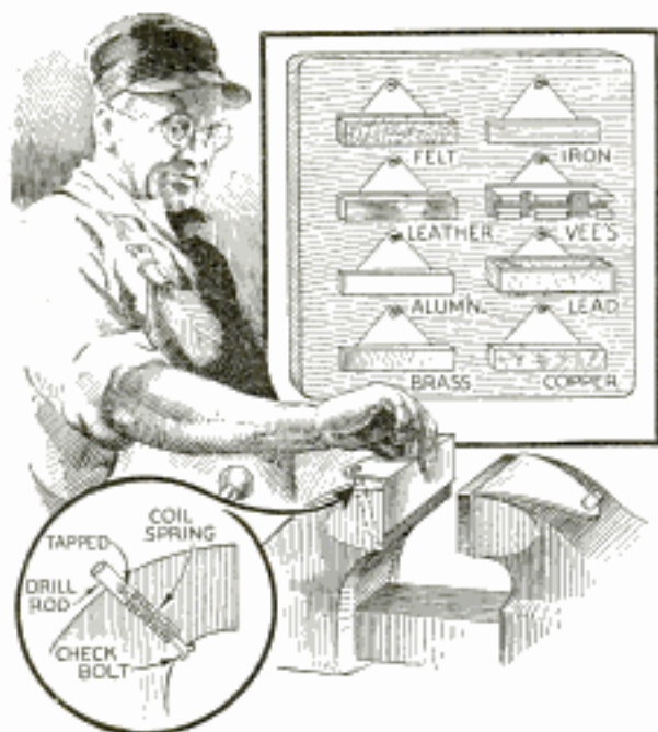
Interchangeable Pads of Varying Hardness Enable All Kinds of Work to Be Clamped in Vise
