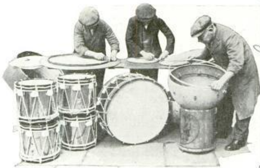
© Fox Photos Making Drums for the Use of the British Army; the Men Are Stretching Vellum on the Drum Hoops, Preparatory to Installing the Heads
