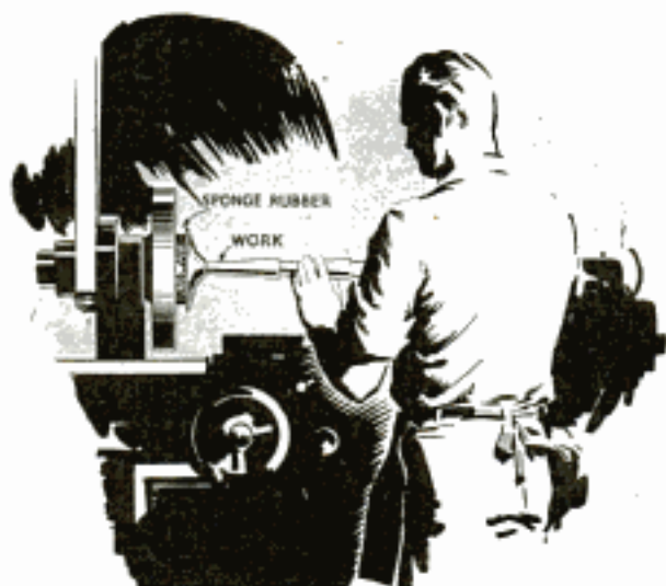
Sponge-Rubber Disk between Lathe Faceplate and Work Holds It for Light Turning and Polishing
