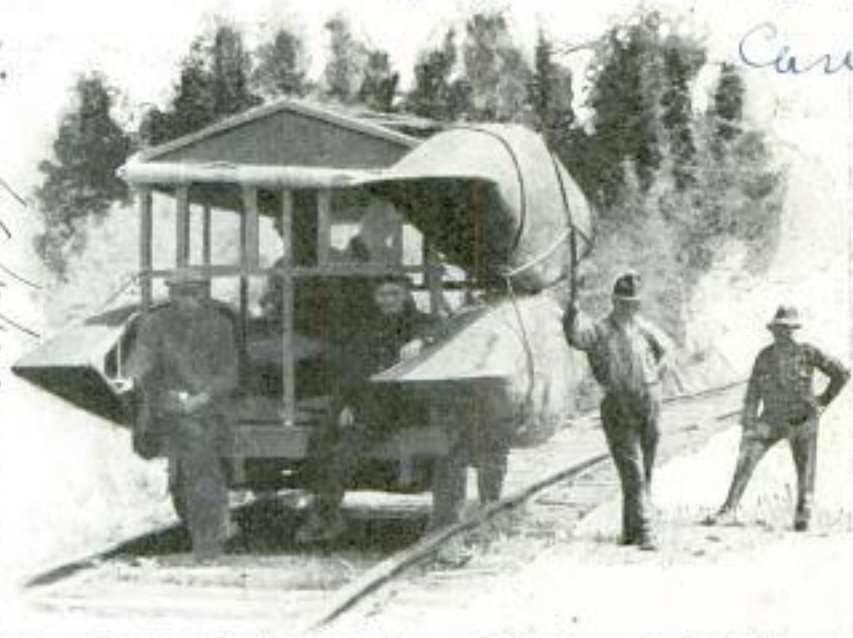
Canoes Used by Canadian Fire Rangers Lashed to a Small Rail Car on Which the Boats Are Often Carried on Long Overland Trips
