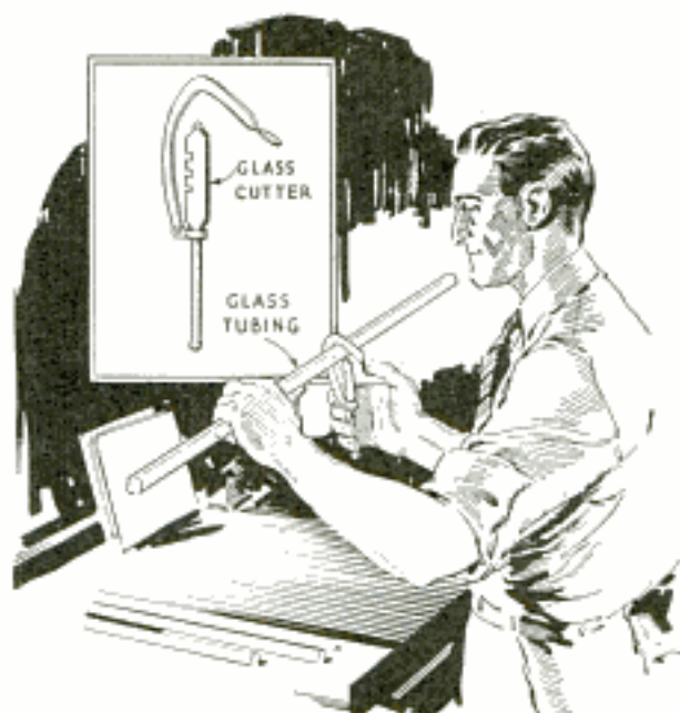
Simple Attachment Holds Glass Tubing to Permit Quick Parting with Ordinary Glass Cutter
