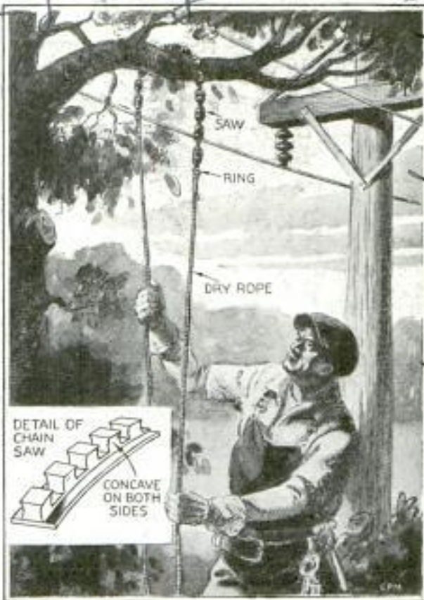
This Unusual Saw, Operated from the Ground, Makes It Easier to Cut Tree Branches
