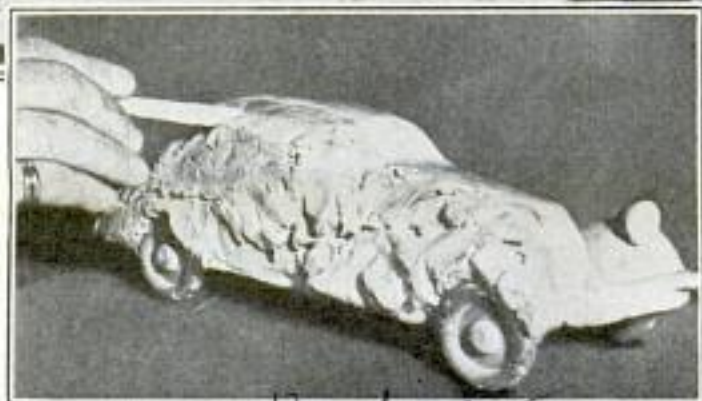
Below, Shaping an Auto-Body Model in Dough Preliminary to Creating Tiny Replica of Design for a New Car
