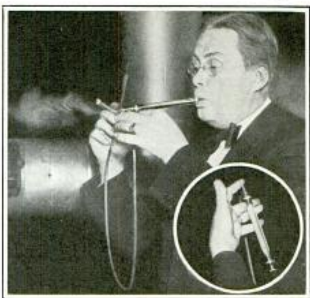
Testing the Draft with Cigar Smoke; Inset, Small Gauge Which Shows Condition of Chimney
