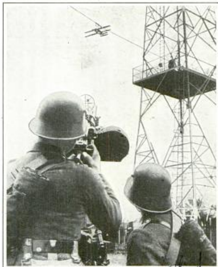
Army Gunners Aiming at Dummy Airplane on Cable; Small Model Is Used to Give Effect of Distance from the Ground
