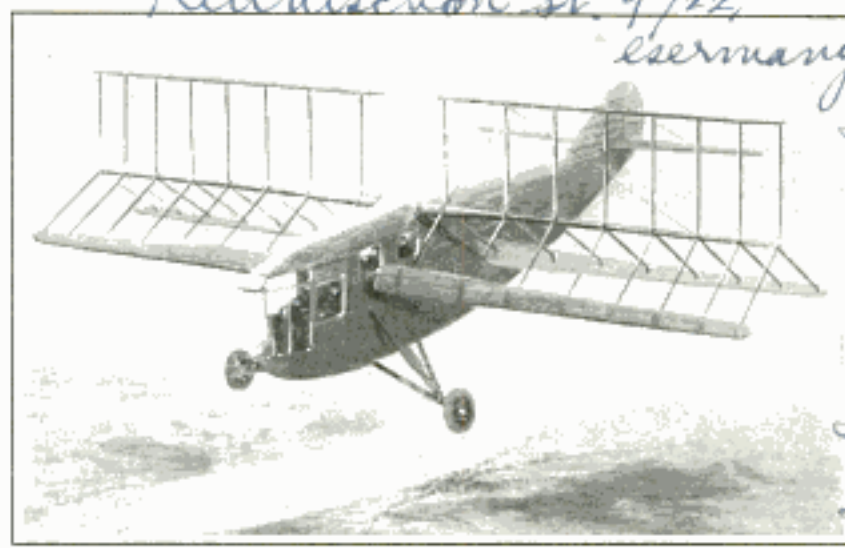
Paddle Wings Replace the Conventional Wings and Propeller on This Plane That Is Expected to Fly Backward or Forward and to Hover in the Air
