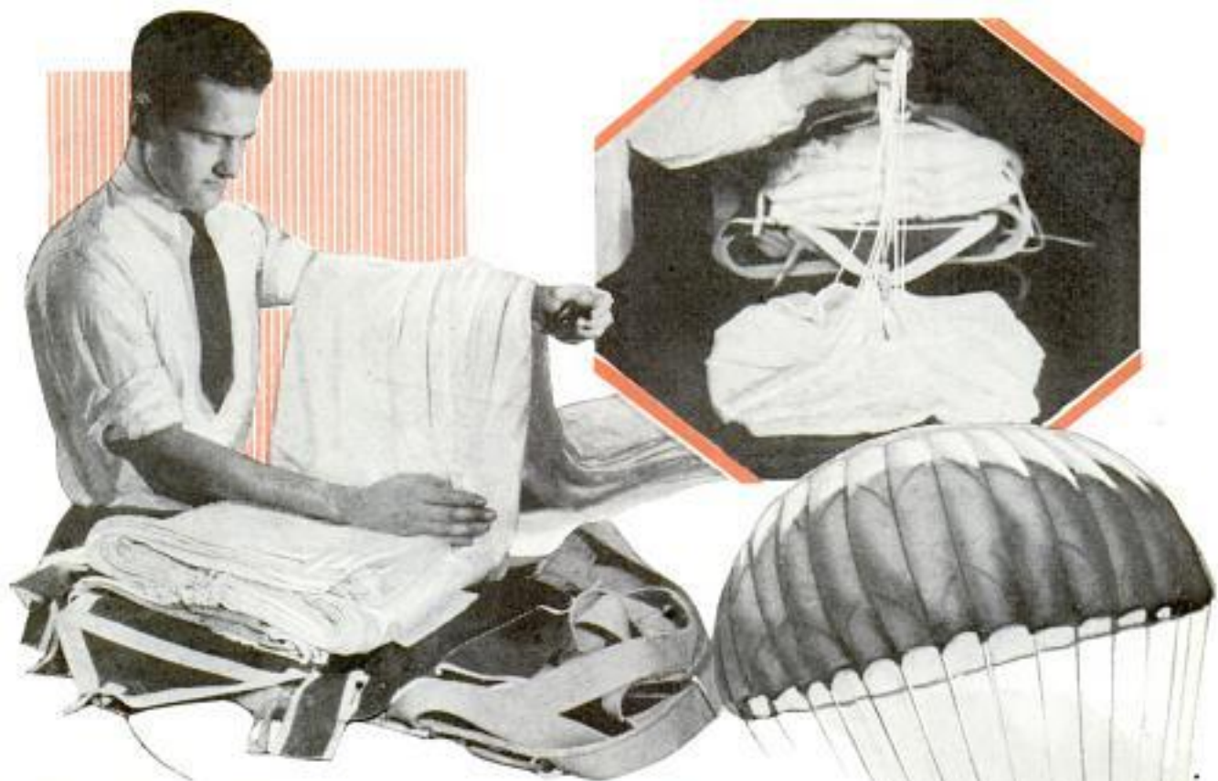
Above, Packing a Parachute; Insert, Folding the Pilot Chute; Right, Showing How Two Parachutes Can Be Used Simultaneously
