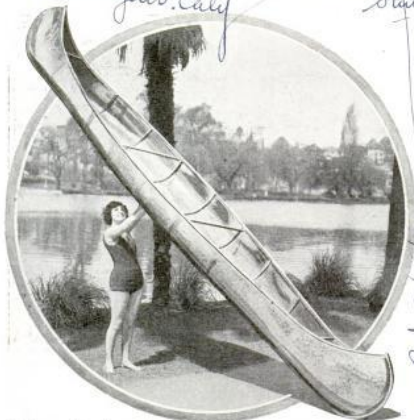
Aluminum Alloy Canoe Eighteen Feet Long and Weighing Only Thirty-Five Pounds; It Is Intended to Carry a Load of 700 Pounds
