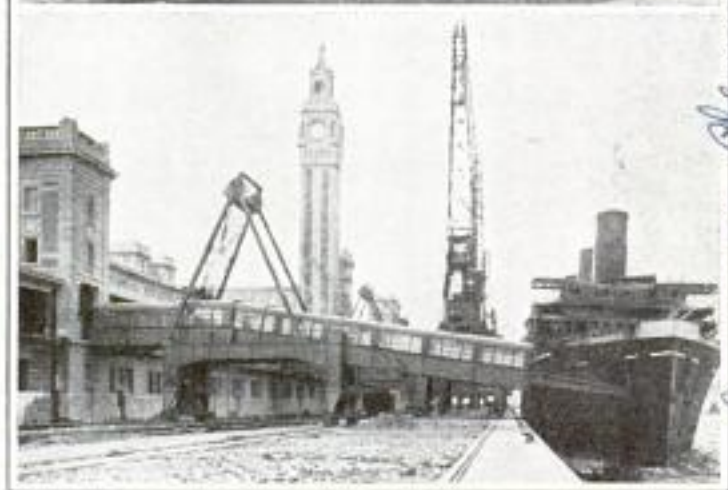
Interior and Exterior Views of Mechanical Gangway on Rails Which Can Be Moved from One Ship to Another
