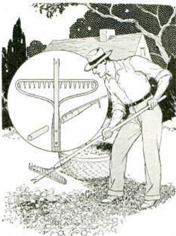
With This Tool You Can Cut Out Dandelions as the Lawn Is Raked
