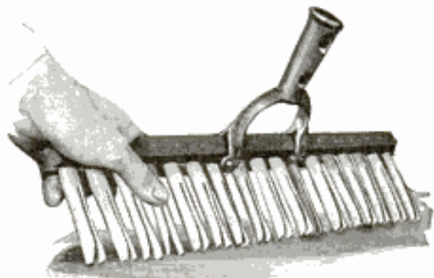
Lawn Rake, Fitted with Clothespins for Teeth, Is Not Easily Clogged by Grass and Leaves
