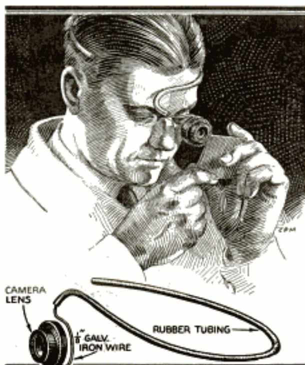
Magnifying Glass Held by Wire Headband Helps in Examining Fine Model Work
