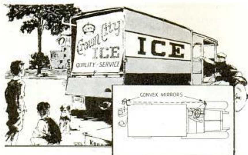
Two Rear-View Mirrors and a Canvas Curtain Aid the Driver in Keeping Children off Rear of Large Truck
