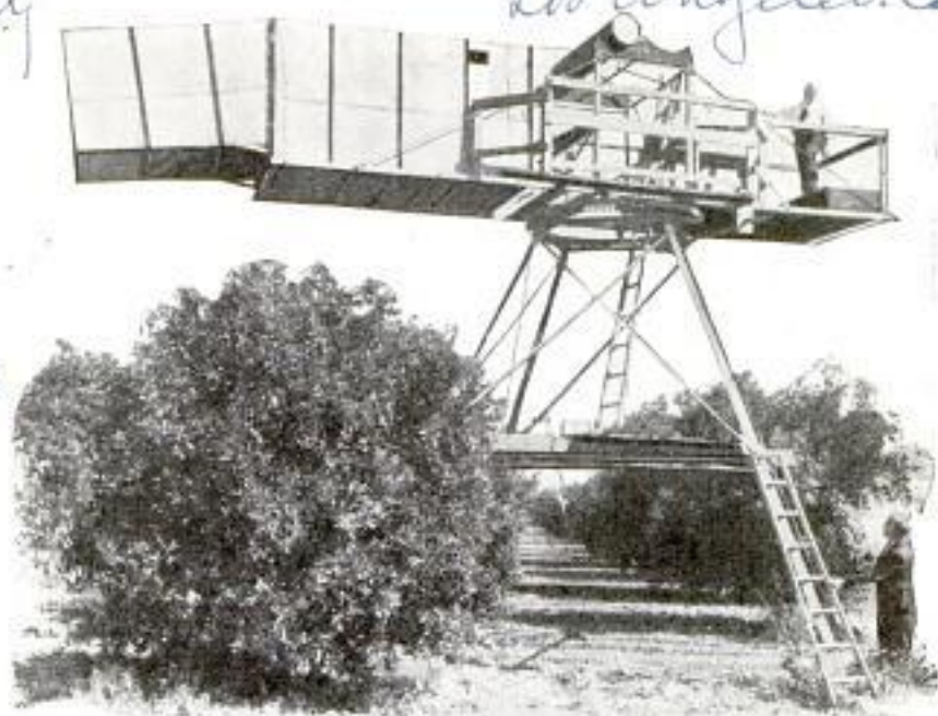
Blower "Gun" for Use in Orchards Keeps Air Circulating and Prevents Formation of Frost; Hood "Shoots" Air in Desired Direction
