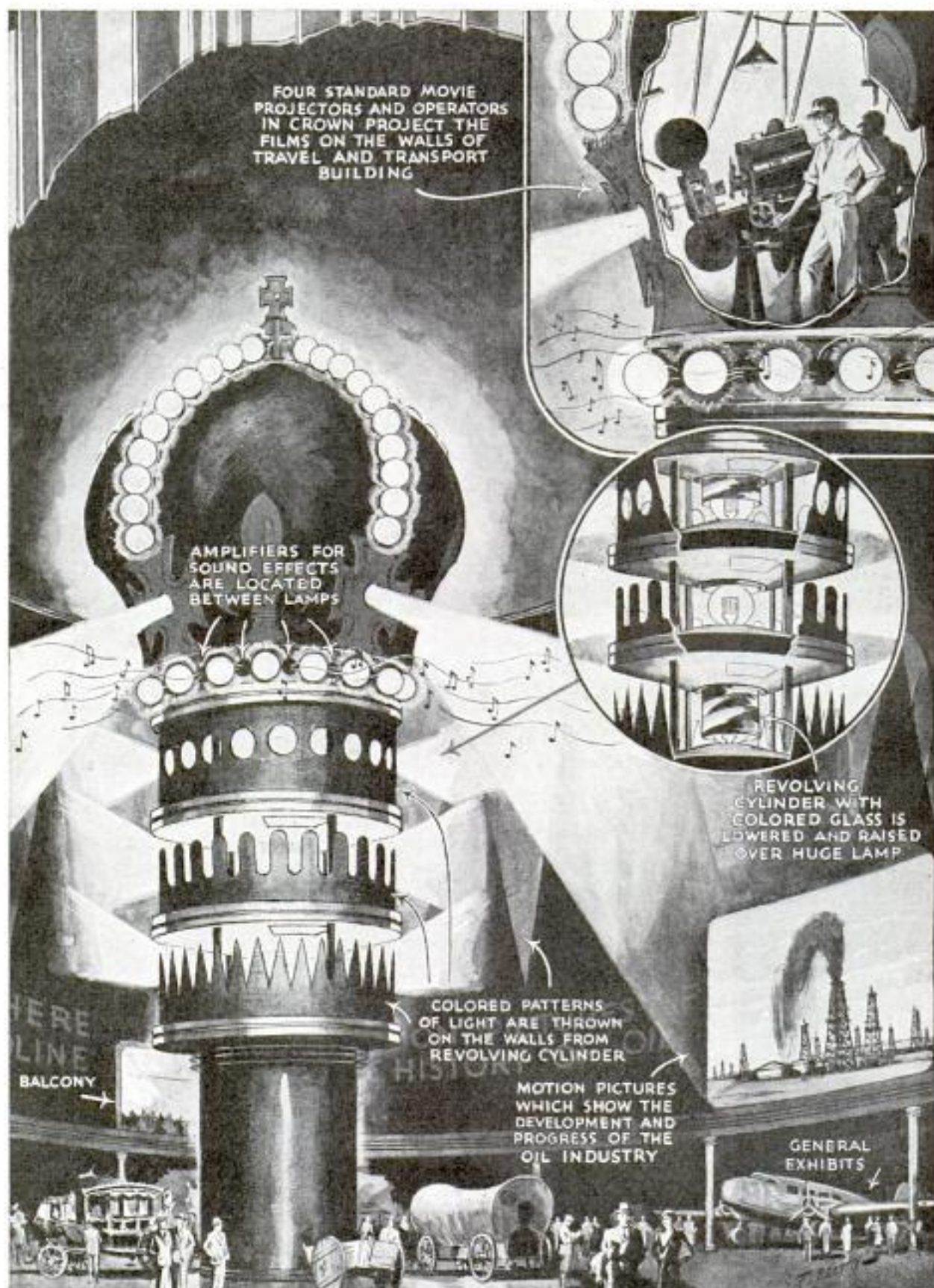
Artist's Representation of Twenty-Eight-Ton Crown That Will Give an Entire Show; Insets Show Some of the Interior Construction of the Robot
