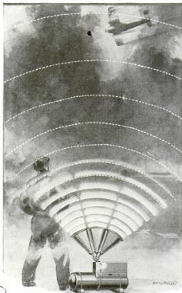
How Sound Beam Guides Airplane to Earth; Note Three-Horn Arrangement on the Sender
