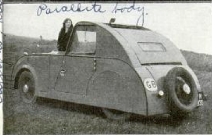
Luggage Is Carried in This Car in Compartments in the Fenders Provided with Doors; Note Open Top
