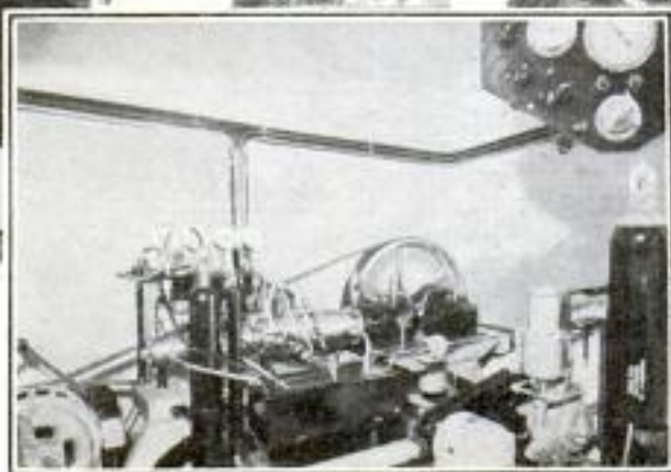
Compressor Unit in the "Cold" Laboratory at California Institute of Technology Applies Pressure of 8,000 Pounds per Square Inch; Gases So Compressed Are Explosive, so Electric Switches Are Sealed in Glass to Prevent Sparks from Escaping
