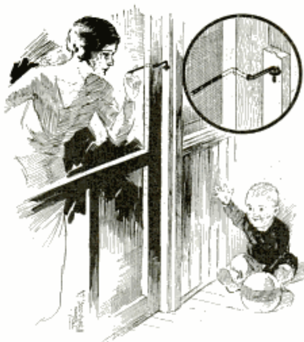
This Screen-Door Hook Can Be Locked or Unlocked from Either Inside or Outside
