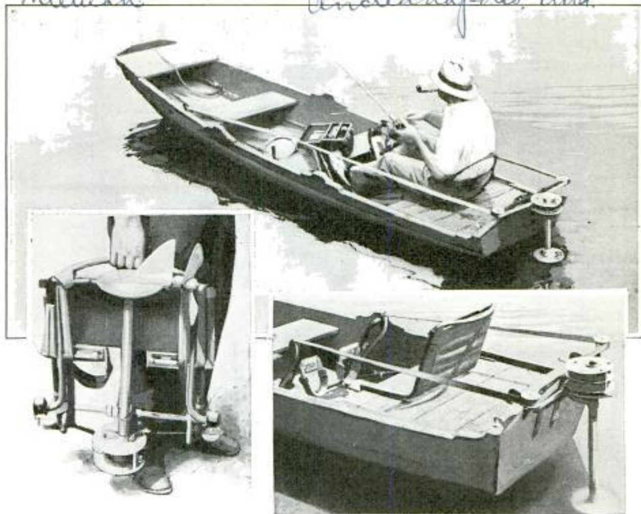
Top, Casting Is Easy in Boat Controlled and Propelled by Foot-Operated Oars; Bottom, Pedal Oars Folded for Carrying, and Close-Up of Arrangement in Boat, Showing Pedals and Means of Turning the Propeller
