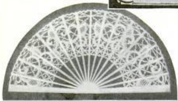
Samples of New Art Showing That Extremely Thin Metal Can Be Etched in Intricate Designs
