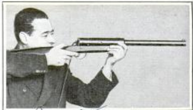
Resembling the Regulation Army Rifle, This Gun Shoots Light Beam That Registers on Target
