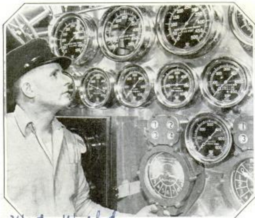
Cluster of Dials That Help to Operate a Modern Cruiser: Photo Shows Part of the Control Board of the "Indianapolis"
