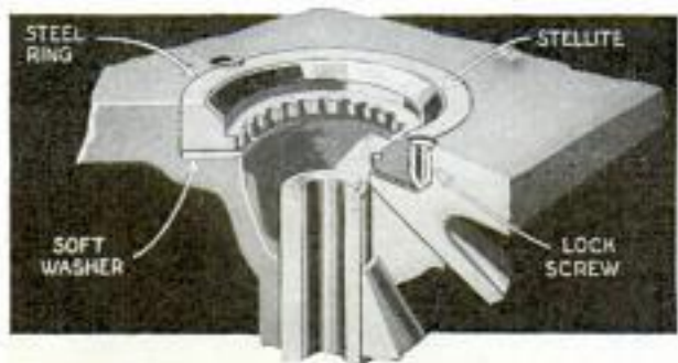
View of Auto Valve Seat That Resists Heat; Special Alloy Eliminates Frequent Regrinding
