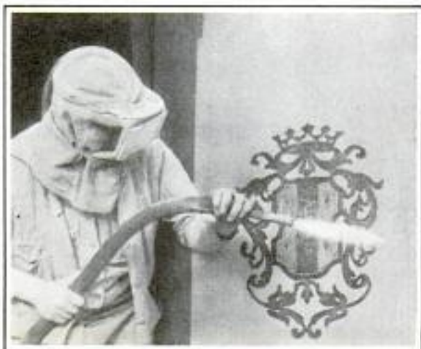
Designs Are Easily Cut in Wood by Using a Rubber Stencil and Sand-Blasting Equipment
