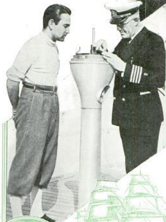
Top, Old Sailor Inspects Fathometer That Replaces Lead-Heaving in Determining Depth; Left, the "Mariposa's" Gyro-Compass Repeater and the Polaris
