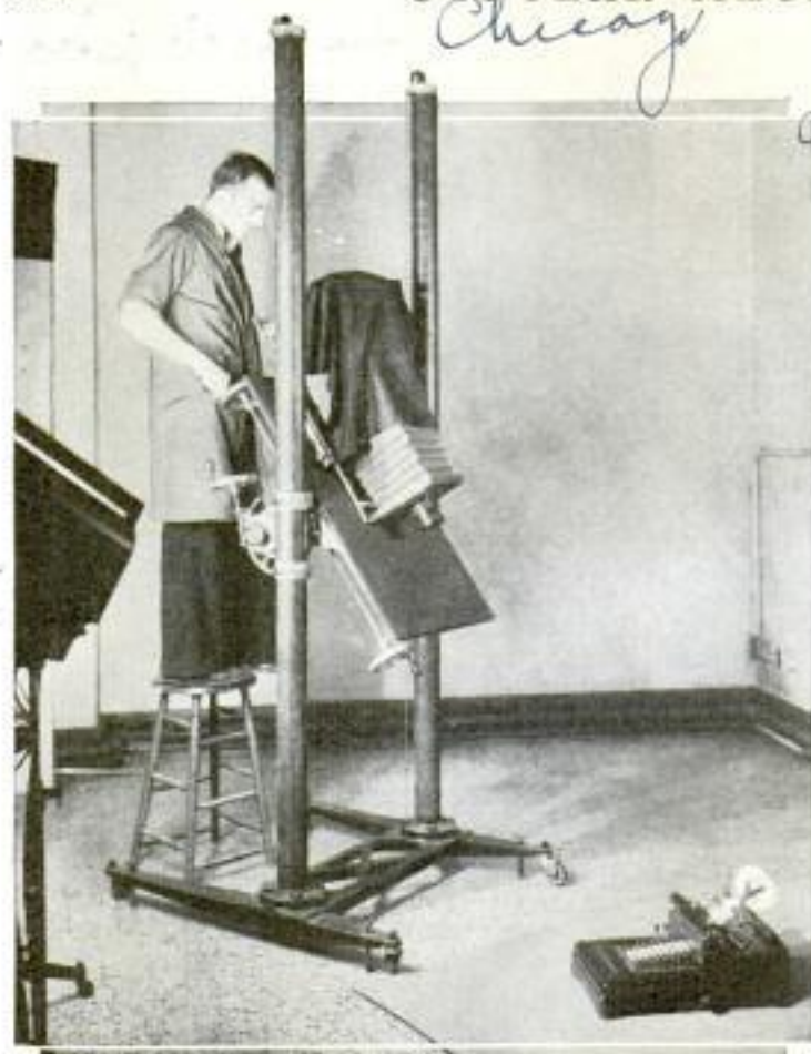
Photographing an Object at an Angle Is Made Easier by This Camera Mount That Has Numerous Adjustments
