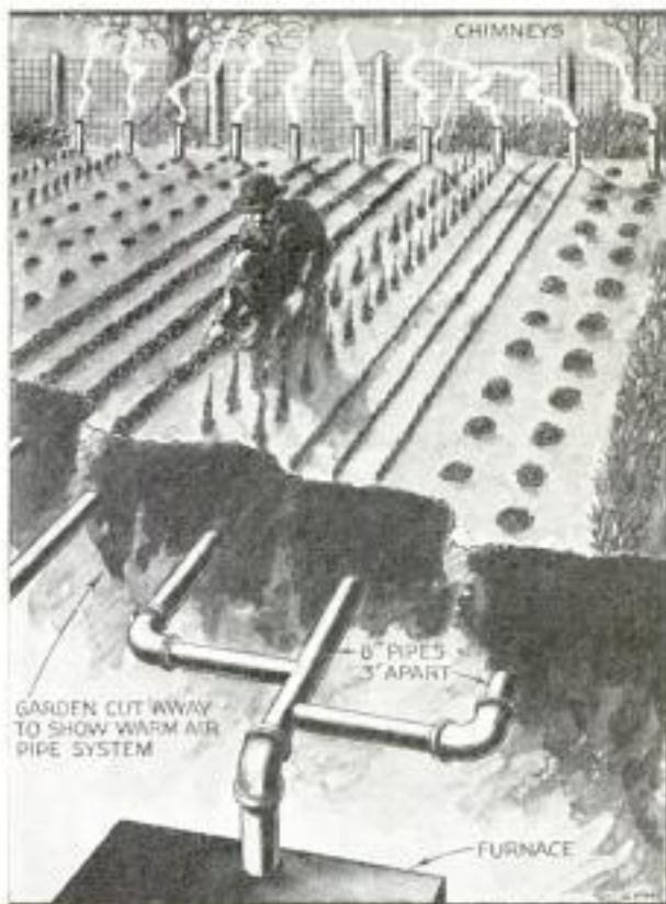
Garden Heated by Furnace Ovens, the Heat Passing through Tile Laid beneath the Surface
