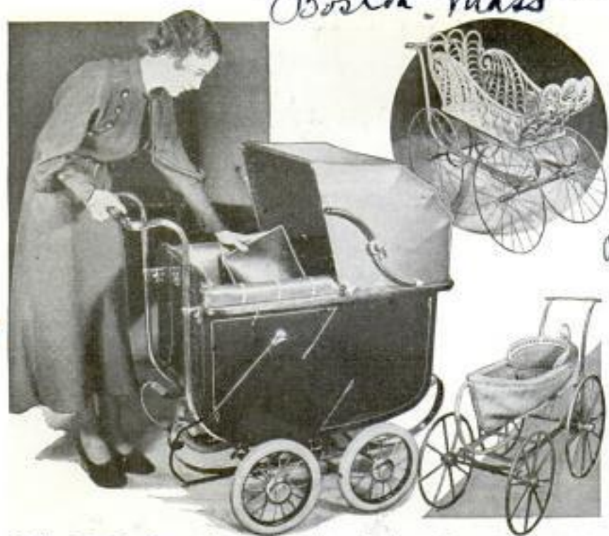
Modern Baby Carriage with Air-Filled Tires, Brake and Easy Springs; Right, Two Models of Earlier Date
