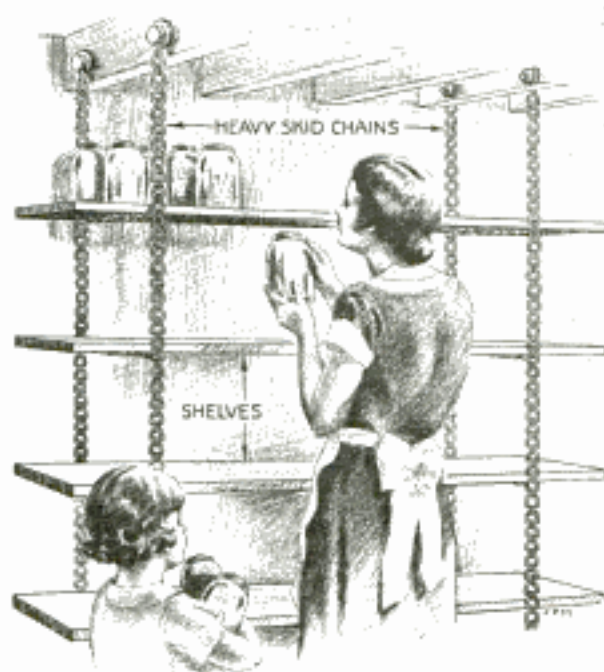
Auto Skid Chains Suspended from Floor Joists Support Shelves in Basement
