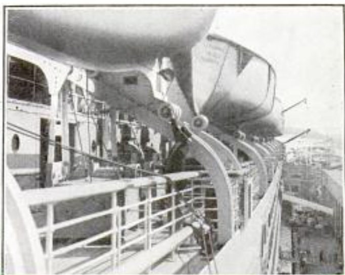
Quadrant Gravity Davits Operated by One Man Swing the Lifeboats Clear on New Vessels Operating in Pacific Service
