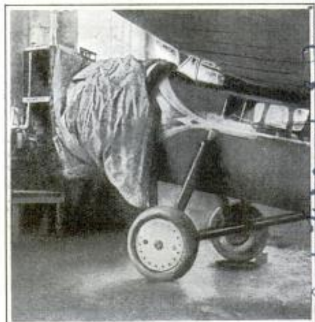
Hood Covering Plane's Nose Helps to Transmit Warmth from Wall Heater to Aid in Starting
