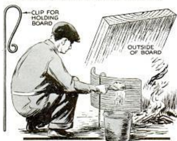
Board Dampened with Water Is Easily Bent When Held Close to Fire
