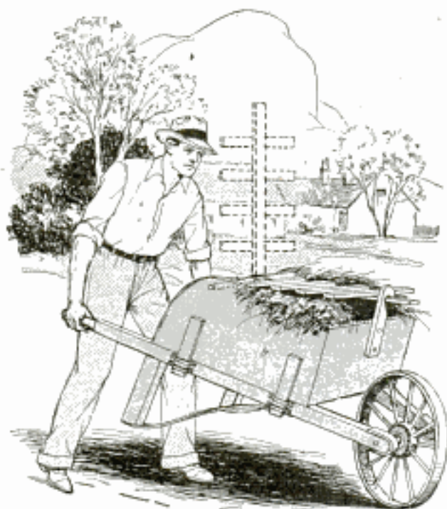
Pivoted between Sides of Wheelbarrow, This Rack Keeps Wind from Scattering Load of Light Material
