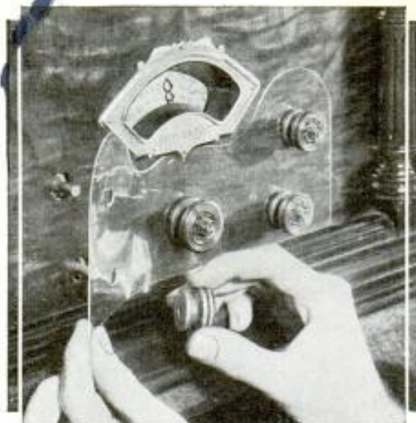
Celluloid Shield behind Control Knobs Protects Panel from Fingernail Scratches
