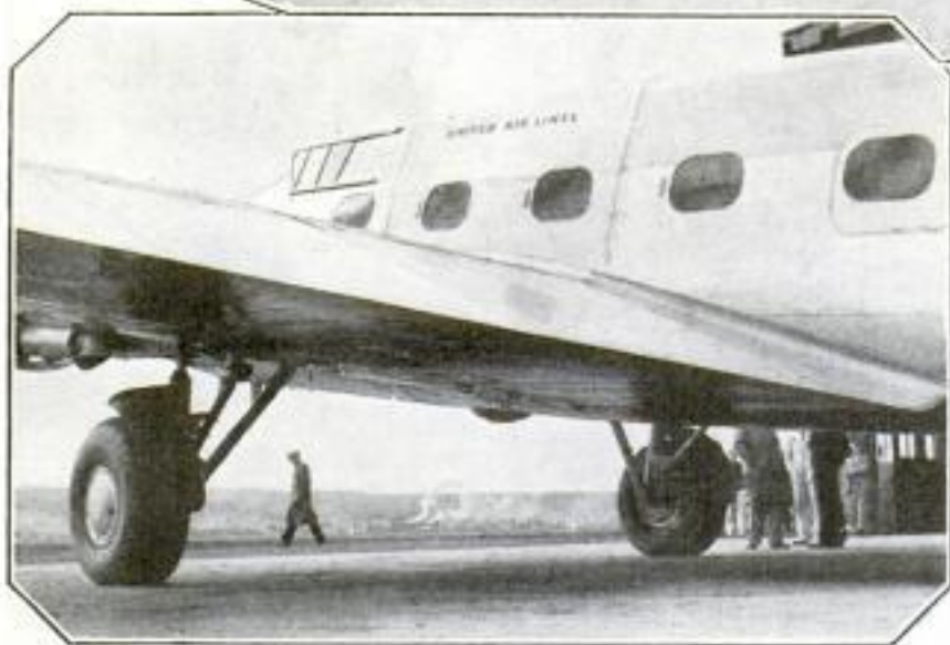
Two Views of Boeing Plane; Note Retractable Landing Gear
