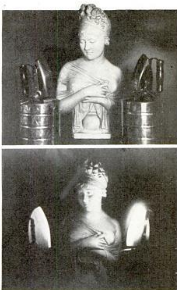
Arrangement of Irons and Statue for Invisible-Ray Photograph; Bottom, Finished Picture
