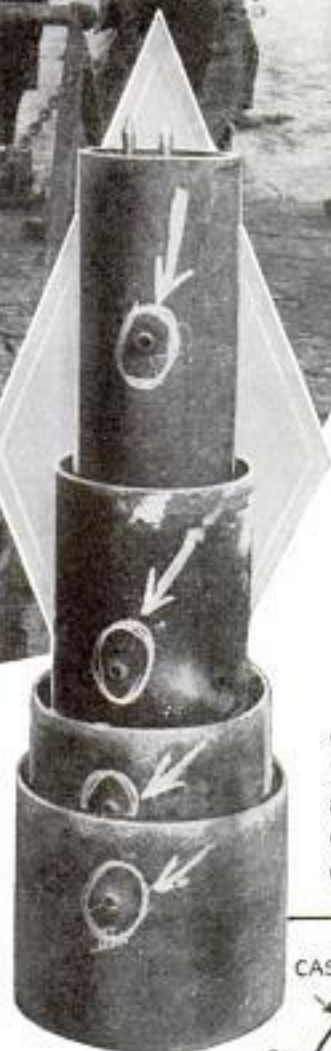
Top, Withdrawing Gun after Firing Charge Far Below Surface; Center, Bullet Holes in Four Casings Encircled in White; Bottom Diagram Shows How One Bullet Penetrated Four Casings
