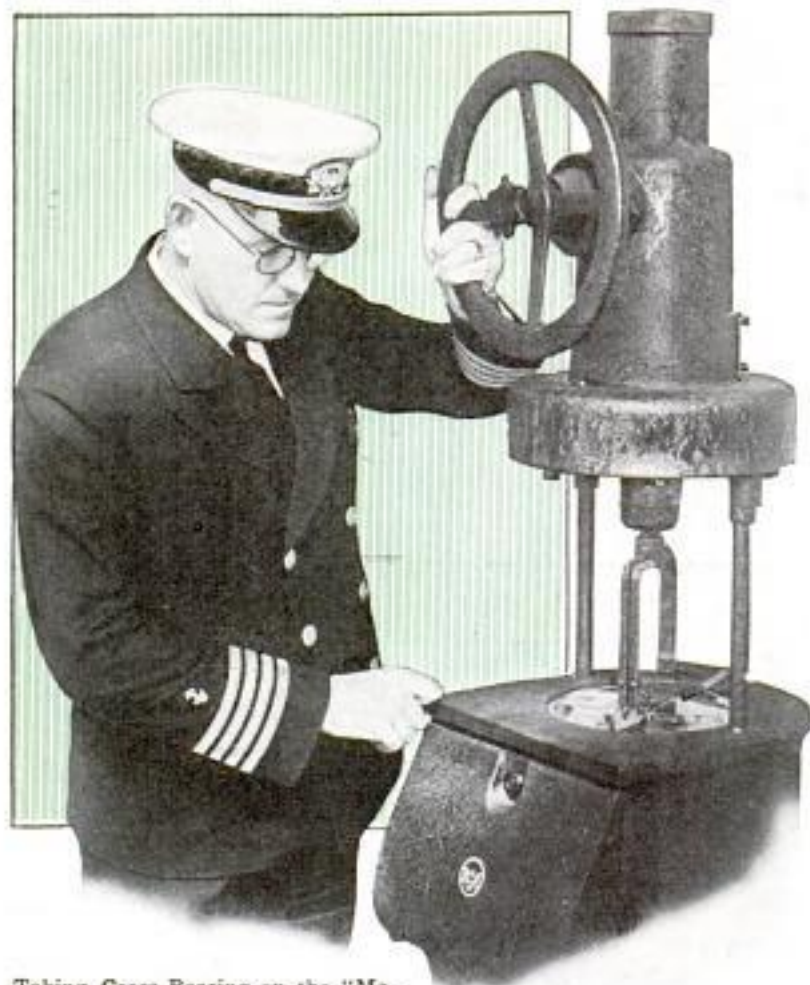
Taking Cross-Bearing on the "Mariposa's" Radio Direction Finder
