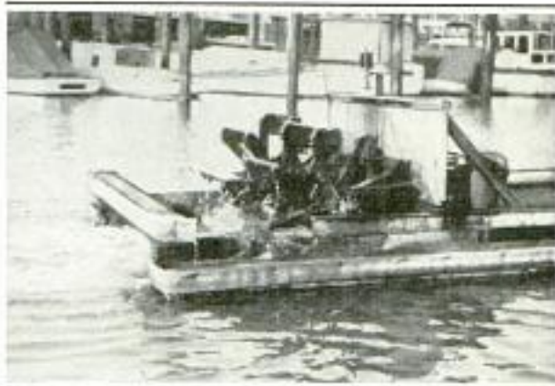
Paddle Wheels Mounted on Float Keep Oil and Drift Out of Yacht Harbor
