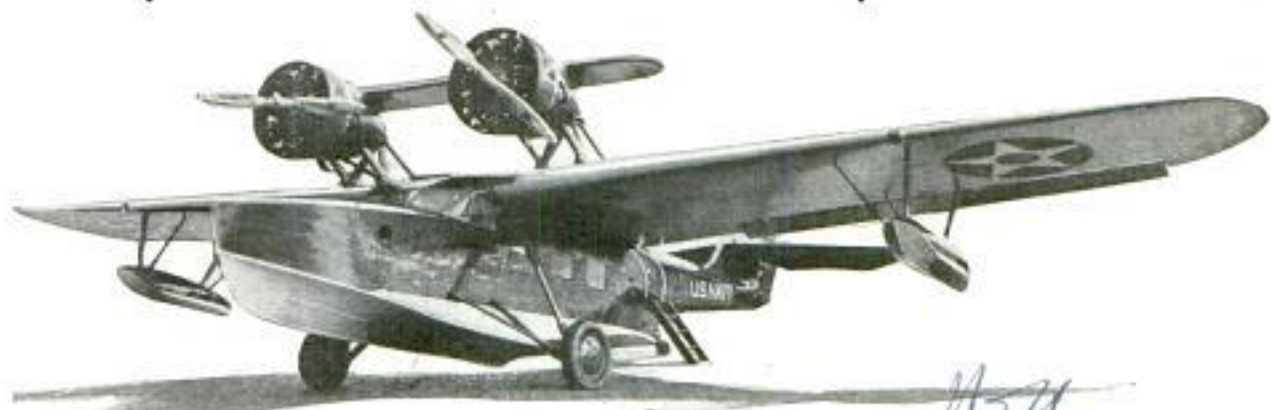
© U. & U. Big Amphibian Monoplane in Which the President May Make Business or Pleasure Trips; It Can Alight on Land or Water and Has a Cruising Range of about 650 Miles
