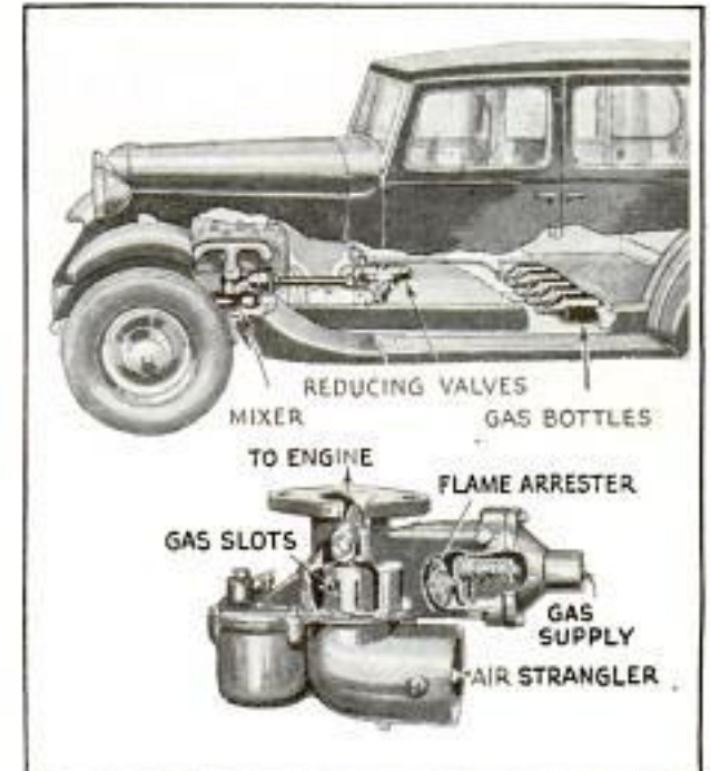
View Showing How Bottled Gas Is Used as Auto Fuel; Below, Carburetor Connections
