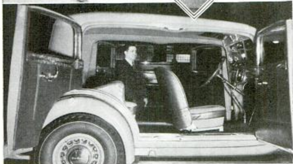
Above, "Straight Through" View of the Pillarless DeSoto; Note That Center Columns Have Been Eliminated; Door Catches and Locks Are at Top and Bottom of Body; Right, Pointing to Divided Bumper at Front of the Graham; This Innovation Makes the Bumper Conform to Flowing Lines of the Modern Auto, Adding to Its Beauty without Loss of Strength
