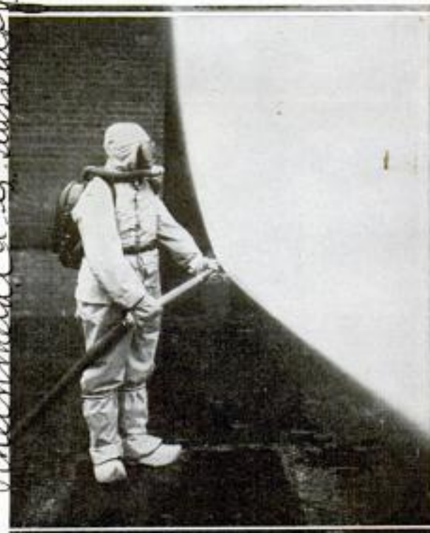
Fire Hose Which Throws a Fine Spray, Thus Smothering a Blaze by Excluding Air from It
