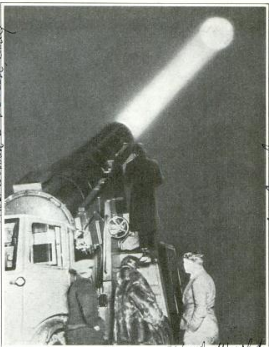
This Huge Projector Puts a Second Moon in Sky by Throwing Picture on Clouds; the Beam Has a Range of Fifteen Miles
