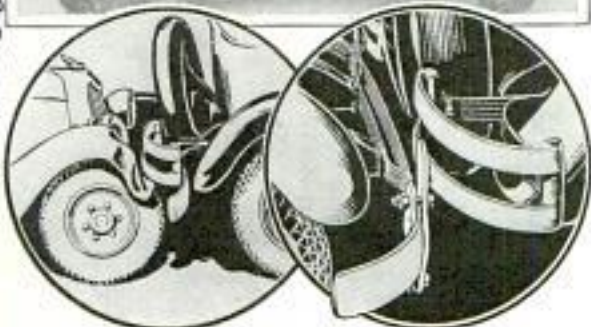
Bumper Stops Installed; Insets, How the Guards Prevent Accidents by Equalizing Bumpers
