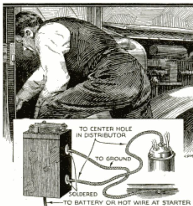
Old Model-T Ford Coil Temporarily Substituted for Regular Coil on Car
