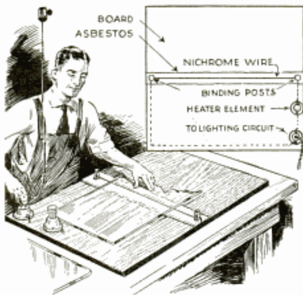
Hot Wire Softens Binding Substance in Non-Shattering Glass so It Can Be Easily Parted
