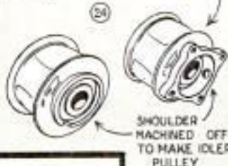
V-PULLEY WELDED TO SMALL ELECTRIC-FAN BLADES
