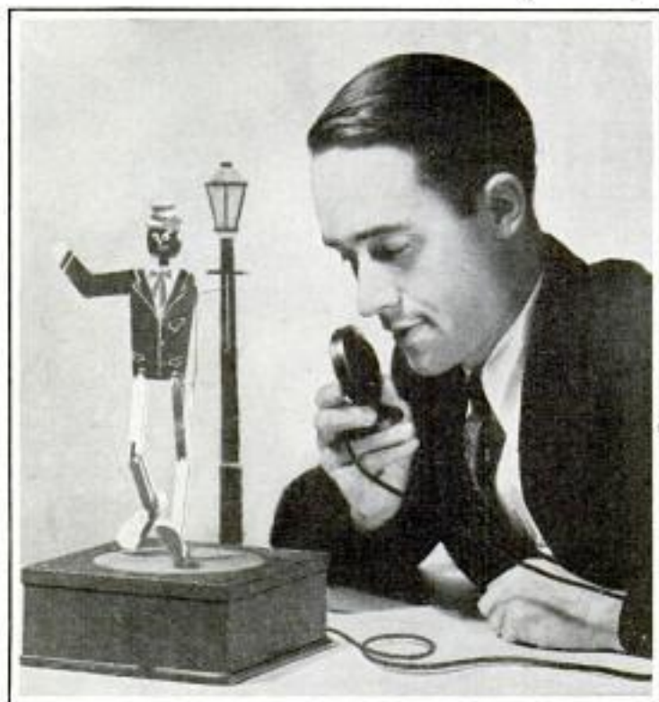
This Dancing Figure Responds to Voice or Radio Music Picked Up by a Miniature Microphone
