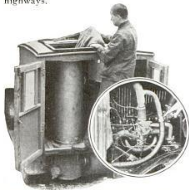
Filling Up Burner of Auto That Runs on Coal Gas; Inset, Pipes Carrying Gas to Engine
