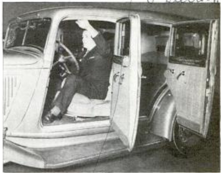
Driver Pushing Button in Car Top to Lower the Curtain over Back Window; Device Is Aid in Night Driving
