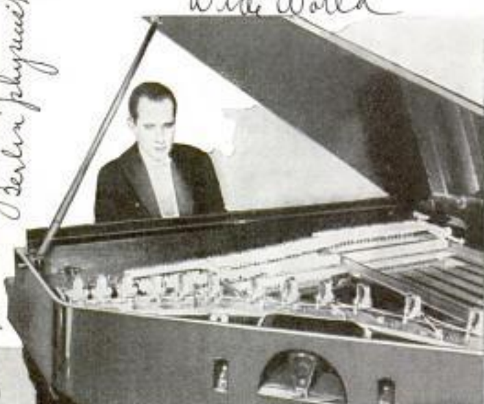
This Instrument Is More Radio Than Piano; It Has Microphones, Amplifiers and Even a Receiving Set in the Case
