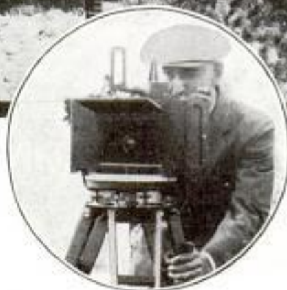
How Fire May Be Located by Meter Card, and, Inset, How Records Are Produced by the Camera-Transit
