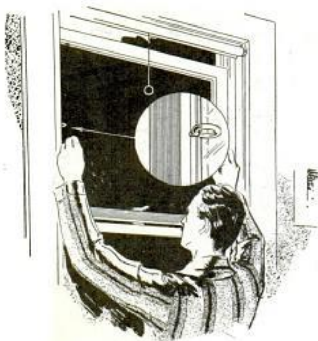
Screweyes Driven into Sash Serve as Fingerholds for Raising and Lowering Upper Window Sash
