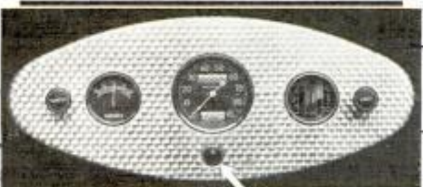
Arrow Points to Signal That Tells Driver When Something Goes Wrong in Auto's Oiling System
