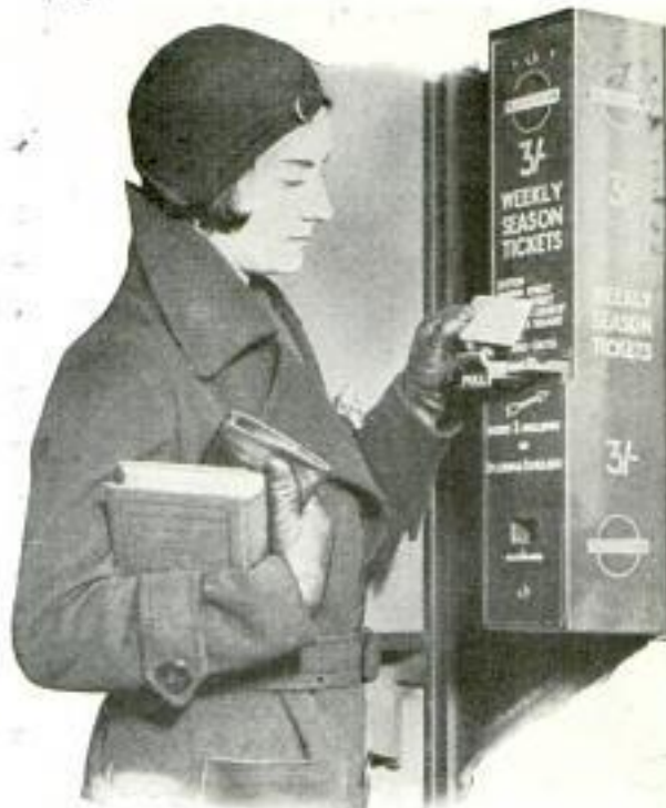
Vending Machine Which Sells Railroad Tickets to London Commuters and Makes Change
