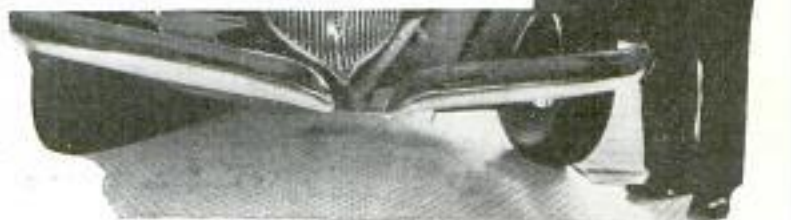
Above, "Straight Through" View of the Pillarless DeSoto; Note That Center Columns Have Been Eliminated; Door Catches and Locks Are at Top and Bottom of Body; Right, Pointing to Divided Bumper at Front of the Graham; This Innovation Makes the Bumper Conform to Flowing Lines of the Modern Auto, Adding to Its Beauty without Loss of Strength
