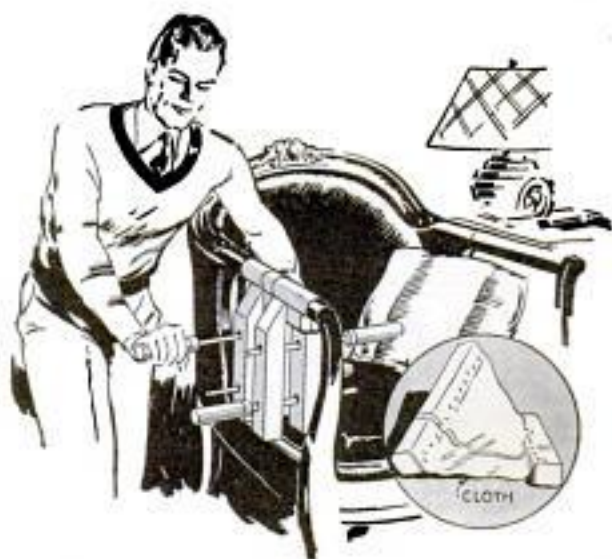
Veneer Can Be Held Firmly on Curved Surfaces While the Glue Dries by This Method
