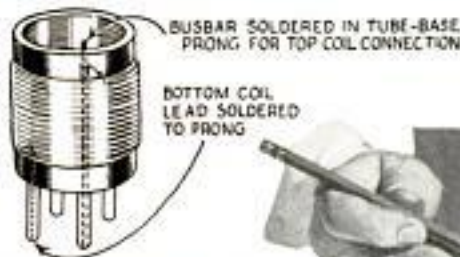
Homemade Choke Coil on Tube Base; Busbar Soldered in Prong for Easy Cut-and-Try Connection to Determine Correct Number of Turns
