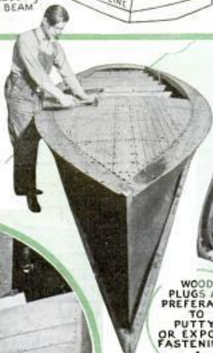
SOME FORM OF FASTENING SHOULD BE USED EVERY 3 INCHES
