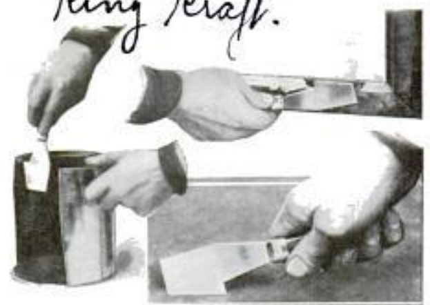
Putty Knife with Sharpened Offset on Side; It is Also Useful as Scraper and for Glazing
