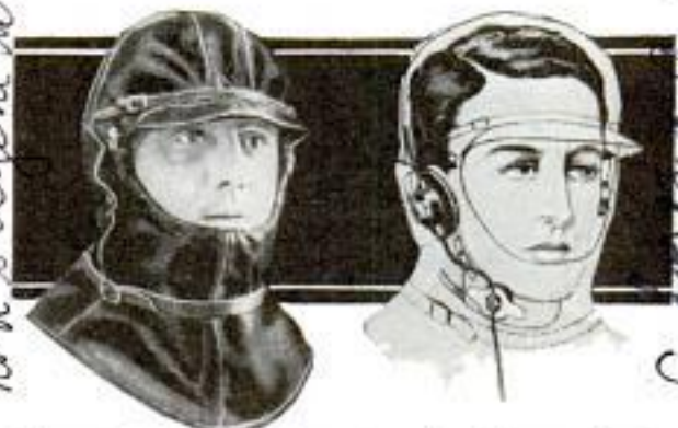
Microphone That Is Strapped against Throat for Use of Aviators or in Noisy Factories
