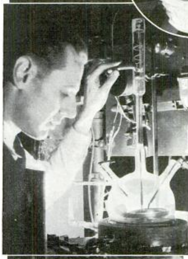
Top and Center, Views of Mercury Tube in Which a Tiny Current Controls Electricity a Million Times Greater; Bottom, Demonstration of Pencil-Lead Control for Powerful Electrical Arc
