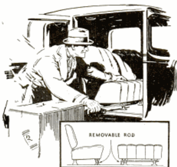
Front Seat in Coach-Model Car Easily Removed by Substituting Rod for Pins
