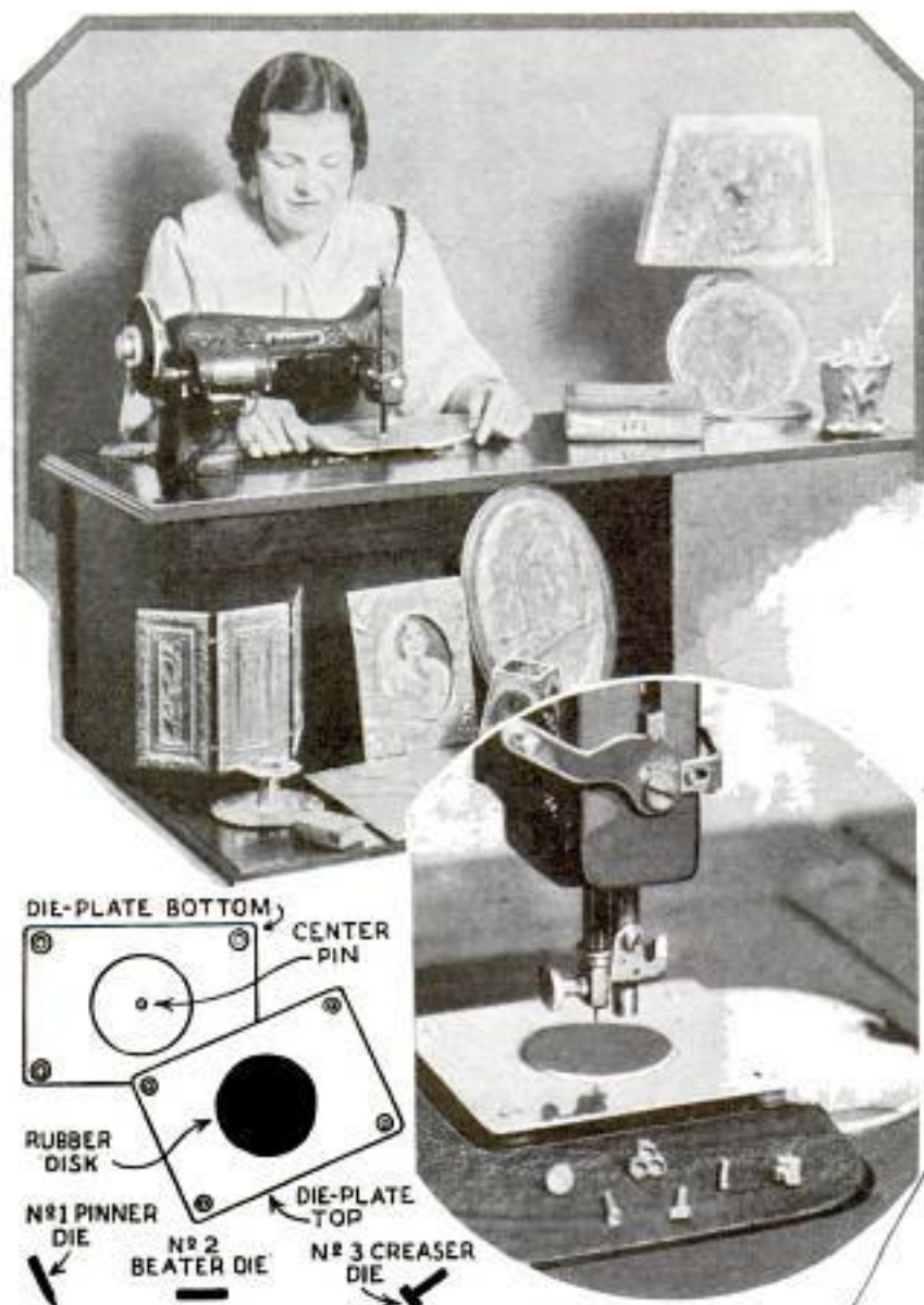
Top, Metal Working on Sewing Machine; Below, Left, Some of the Dies; Right, Close-Up Showing How Work Is Done
