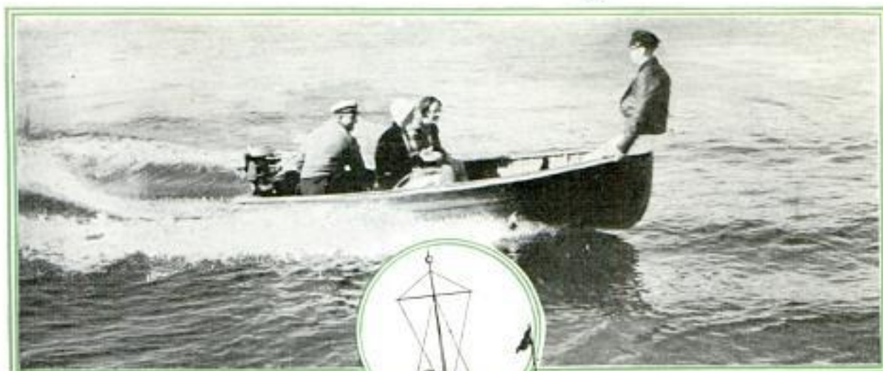
Above, Yachting Tender, a Fast Boat When Powered by Motors of from Twelve to Eighteen Horsepower, and Very Comfortable and Seaworthy; Below, Cross Section of a Single-Cabin Thirty-Foot Cruiser; Note the Immense Amount of Usable Space on This Boat, Due to Well-Planned Interior Arrangement
