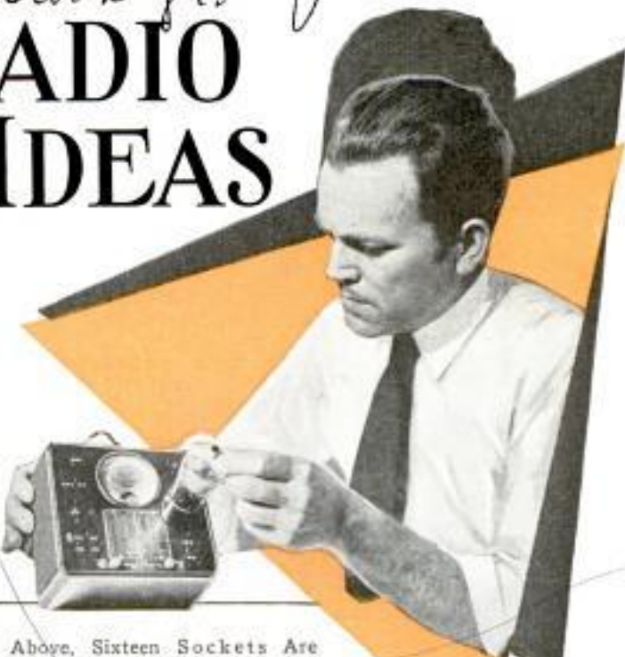
Above, Sixteen Sockets Are Provided in This Tube Checker to Include the New Tubes; Below, Dry-Electrolytic Filter Condensers That May Be Mounted in Any Position and Also Permit the Use of Higher Capacities in Less Space
