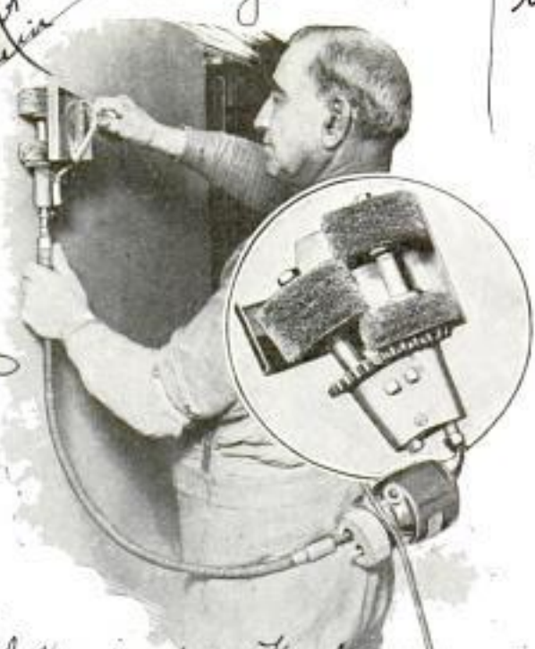
Illustrated Features Electric Motor Carried on Operator's Back Runs This Brush for Removing Wall Paper
