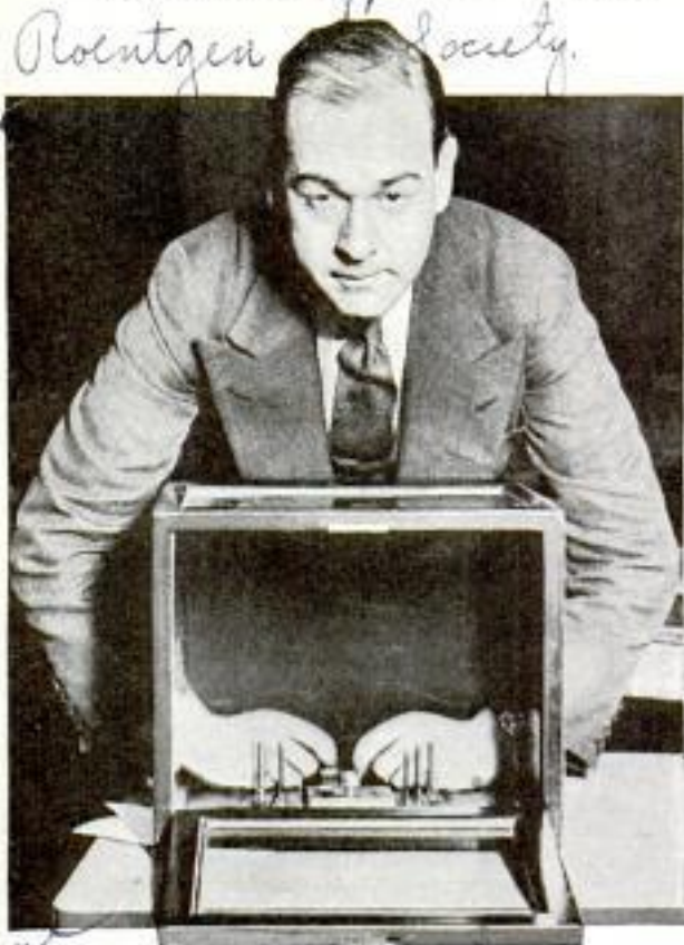
How Radium Needle Filler Is Protected; Only His Hands Enter the Lead-Lined Case
