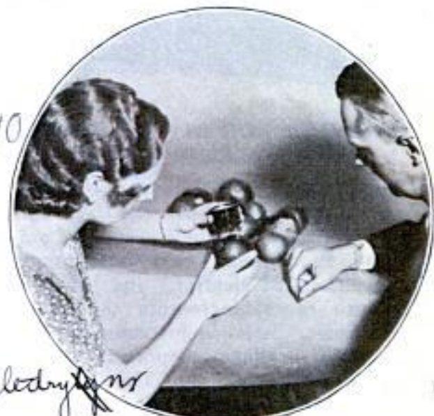
How the Electric Taster Is Applied; the Prongs Are Thrust into the Fruit
