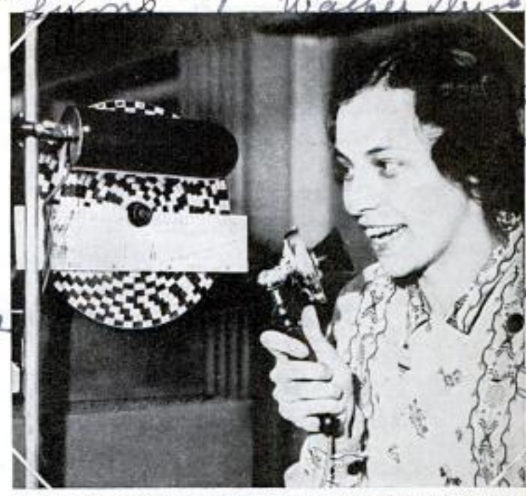
As Young Lady Sings, the Disk Revolves; the Line Appearing at Standstill Indicates Voice Pitch
