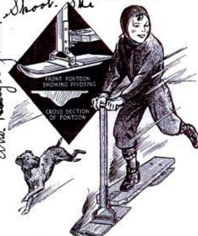
Scooter Mounted on Pivoted Steel Snow Runners to Permit a Modified Form of Skiing
