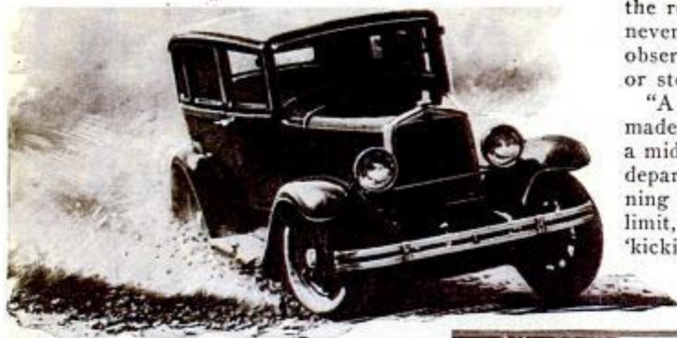
Above, Wrong Way to Get Out of Skid; Right, the Proper Way—Wheels Turned in Direction of Skid
