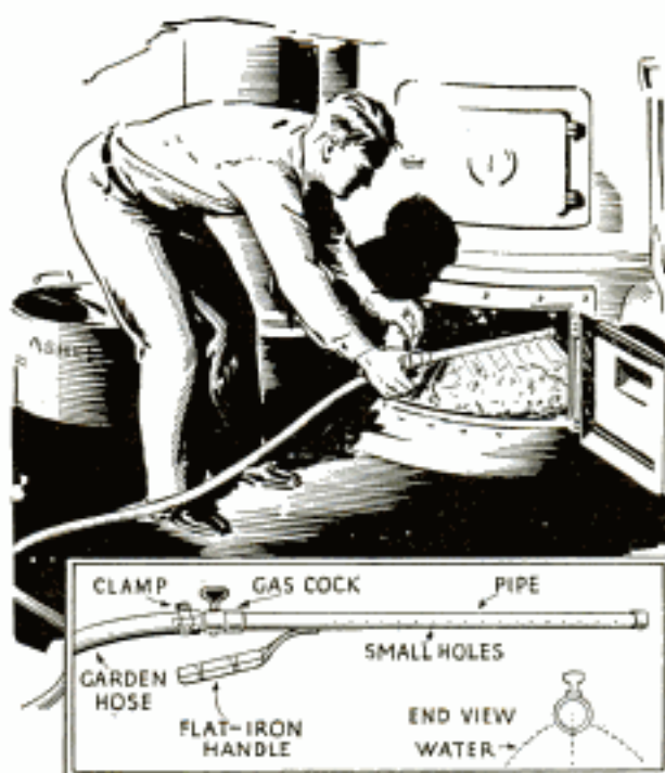
Improvised Nozzle for Wetting Ashes and Coal or for Sprinkling Requiring a Gentle Spray
