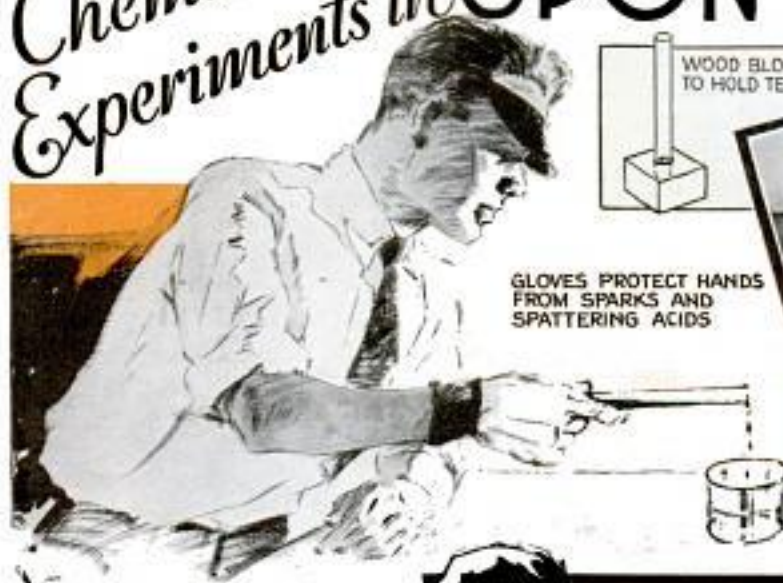
SULPHUR BURNS SPONTANEOUSLY IN OZONE. GLOVES SHOULD BE WORN & SULPHUR DROPPED FROM A PEN KNIFE
