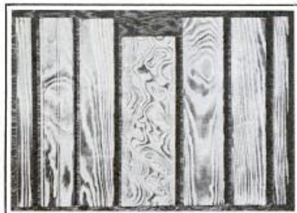
Samples of Pine after a Special Heat Treatment That Emphasizes the Grain
