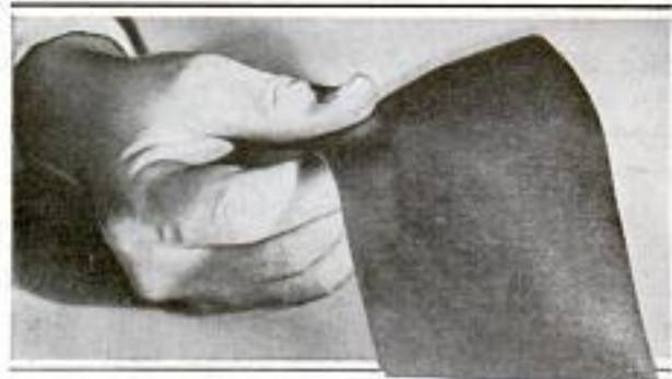
Glue in Sheets Is Useful for Bonding; It Is Applied by Hot-Plate Press
