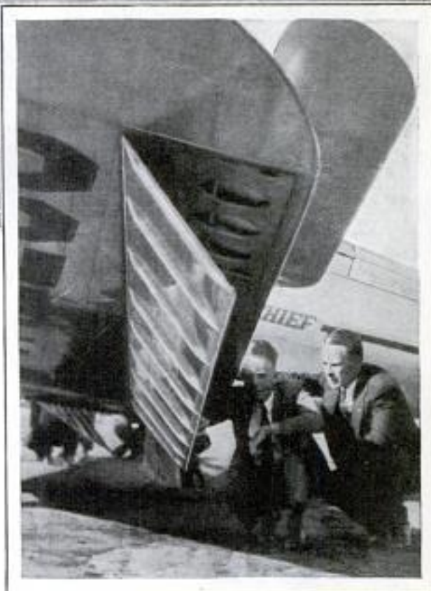
Frank Hawks' Latest Ship Intended for High Altitudes; Right, Wing Flaps to Reduce Landing Speed
