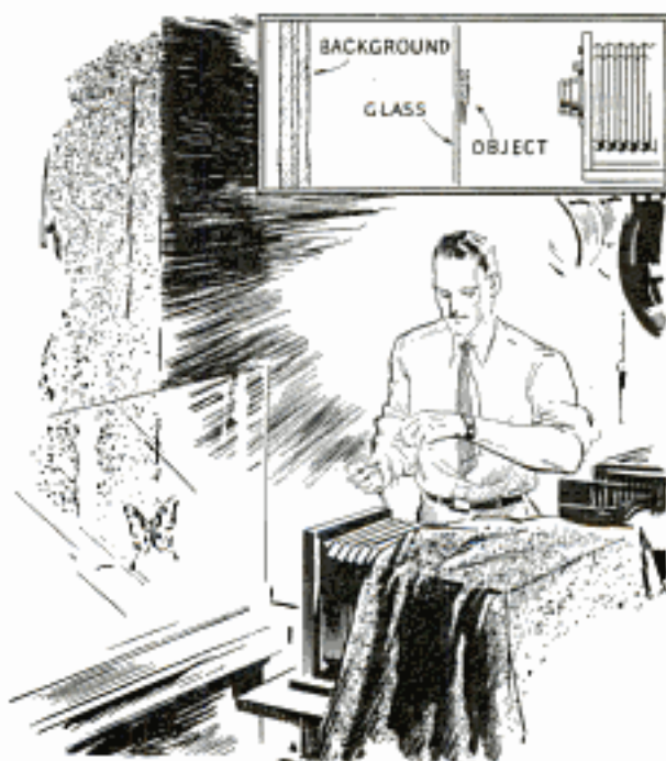
Shadows in Photographic Copy Work Are Avoided by Attaching Specimen to Clear Plate Glass
