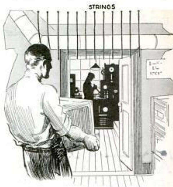
Row of Strings Suspended from Ceiling Warns Persons of a Low Doorway
