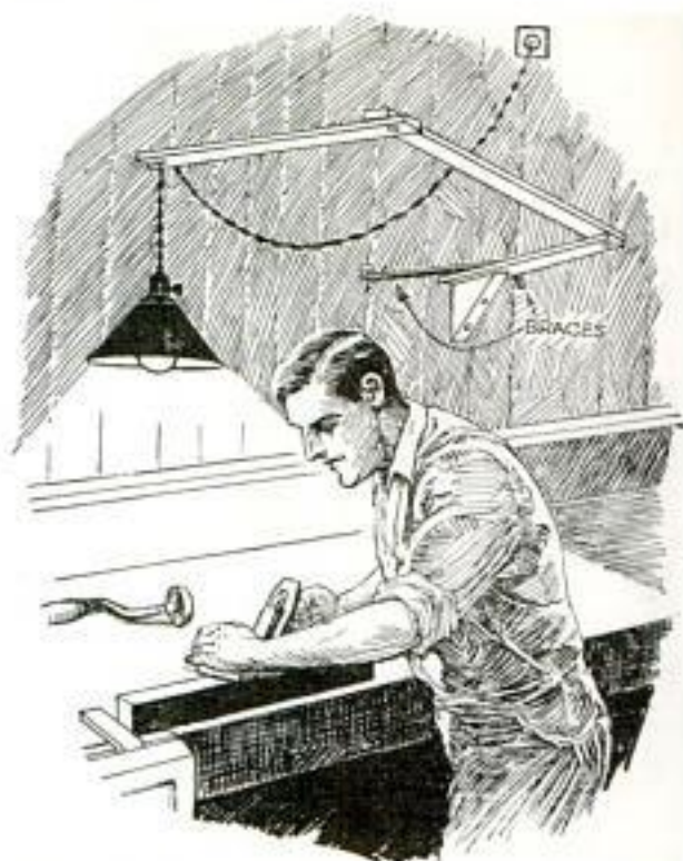
This Adjustable Arm Holds Electric Lamp Directly above Work on Any Part of Bench
