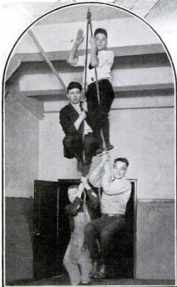
Top, Applying Copper Sheets to Roof; Below, Jute Fiber Expanded by Steel Screw, Holding Four Men
