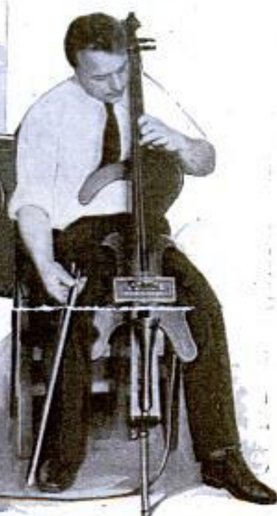
This Device Enables Stringed Instruments to Hold Their Own, Increasing the Sound Twenty Times without Distortion; Photos Show How the Amplifier Is Attached to Three Instruments
