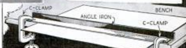
Clamps for Forming Shields and Receiver Bases; Light Aluminum or Eraydo Sheets Are Easily Bent as Shown
