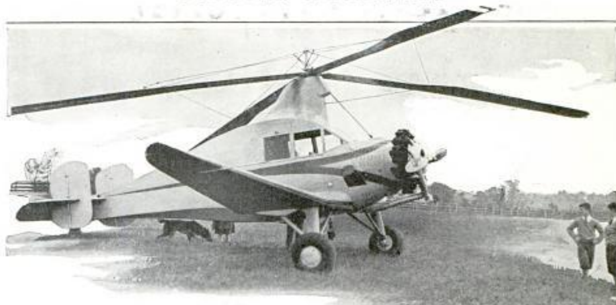
This Cabin Autogiro Is the Largest Ever Constructed in This Country; Note the Unusual Mounting of the "Windmill" Blades on Top of Cabin; This Feature Is Said to Increase Stability
