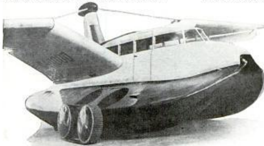
Wide Work Chain Treads on This Amphibian Plane's Wheels Help Pilot in Landing and Taking Off from Marshy Ground
