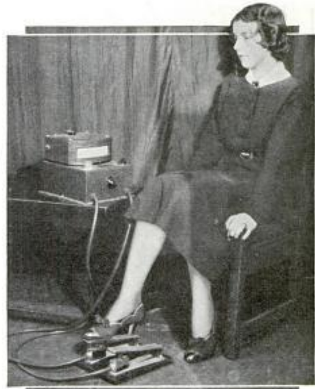
Testing Mental and Physical Response of Motorist to Danger by Electrical Timing
