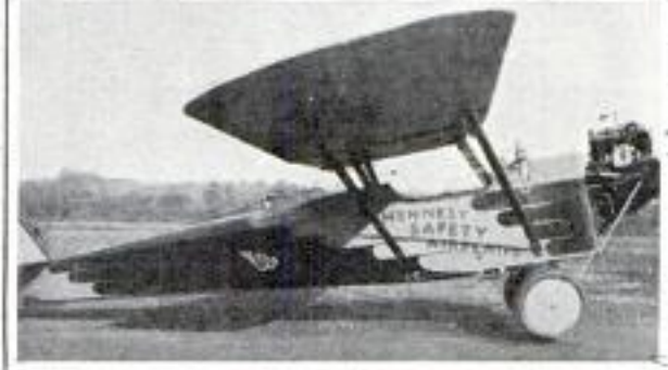
Monoplane with Adjustable Wing Which Enables the Pilot to Change the Angle of Incidence at Will
