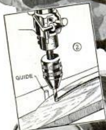
② GRINDING THE ROUTER BIT ON AN EMERY WHEEL
