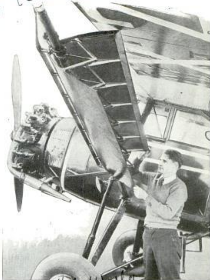
By Opening Out Panel-like Surfaces, the Pilot Can Apply Brakes to Ship Gliding to a Landing
