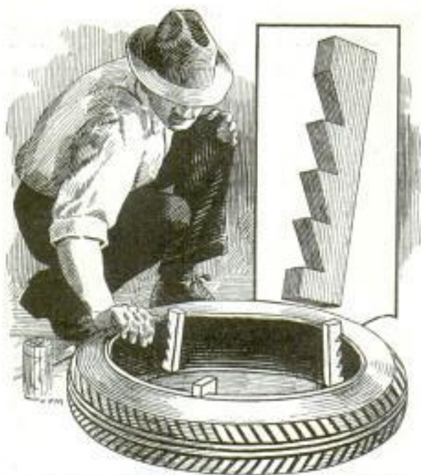
Spaced at Equal Intervals, Three Wooden Blocks Hold Auto Casing Open When Examining Inside for Tacks
