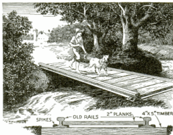
This Foot Bridge across a Small Stream Is Made from Old Steel Rails and Planking
