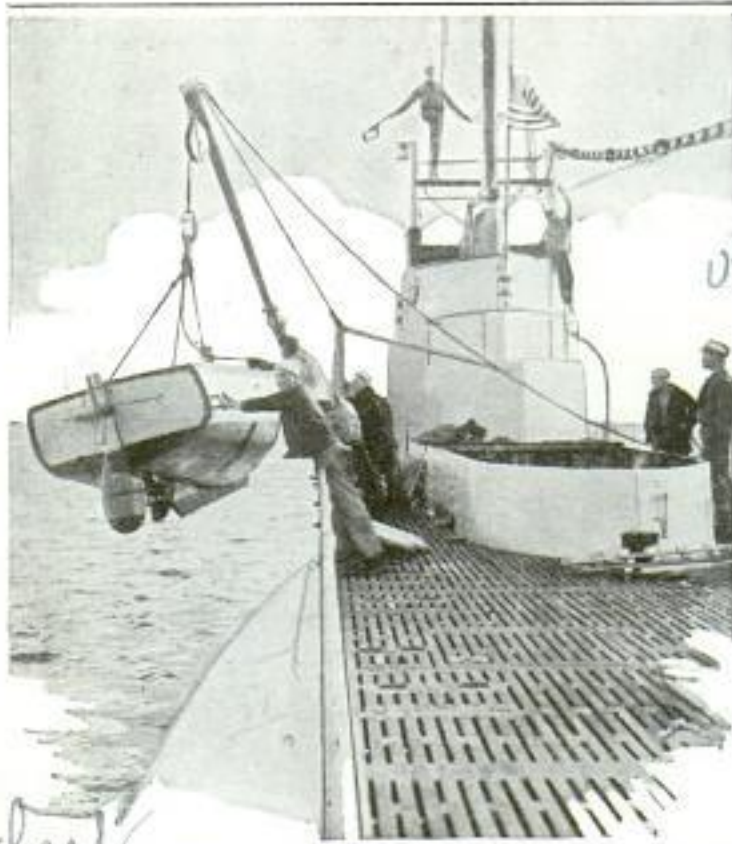
Launching Motorboat from Deck of Submarine; the Craft Is Waterproof and Submersion Does Not Damage It
