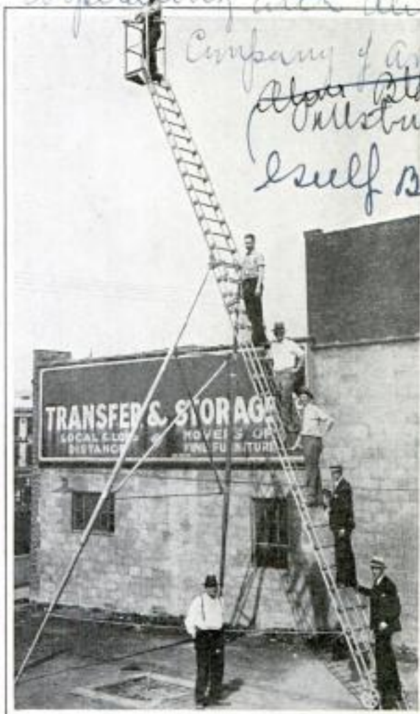
Weighing Only Half as Much as Wood, This Aluminum Ladder Has Wheels for Easy Moving
