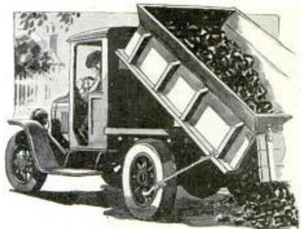
Rope Attached to Rear Wheel and Body of Truck Provides Self-Dumping Arrangement
