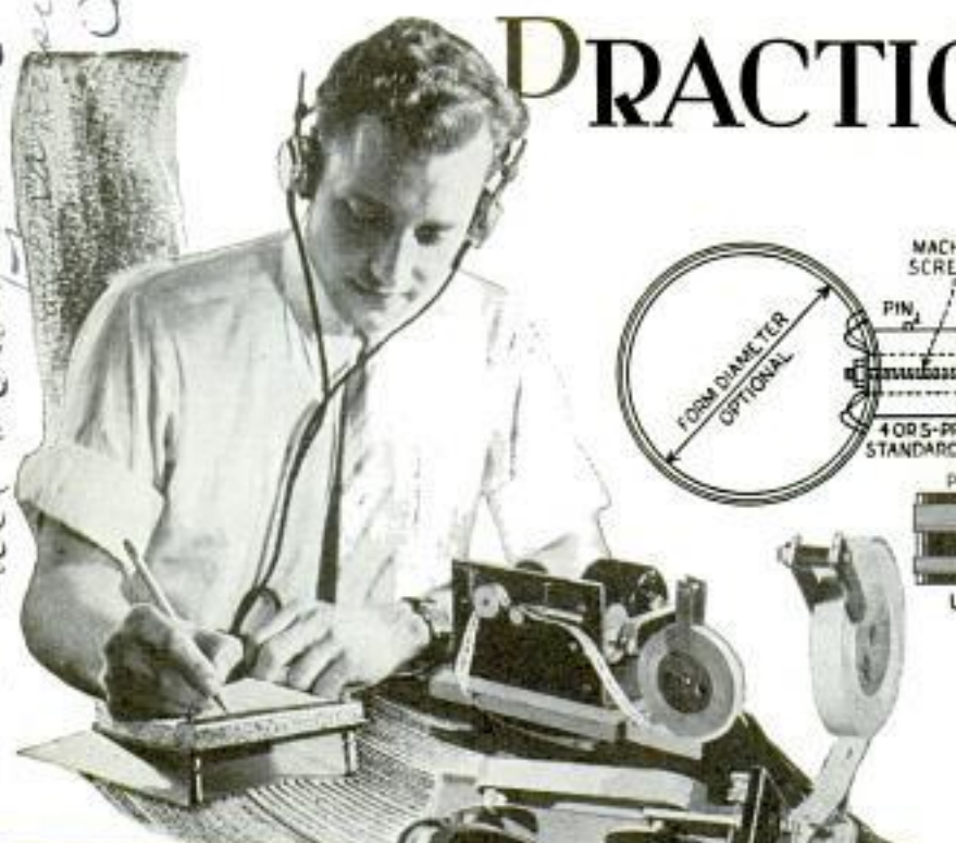
This Handy Plug-In Coil Form Provides Ample Winding Surface for All Short-Wave Coils; the Bakelite or Fiber Tubing Is Fastened to an Old Tube Base by Means of a Brass Machine Screw as Detailed Above
