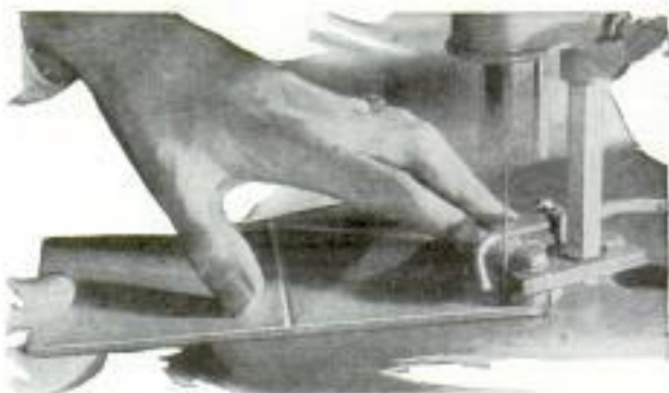
Fitting This Tile Is a Simple Task Since the Material Can Be Sawed and Drilled
