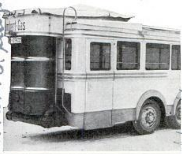
Tanks on Rear of Bus Are Part of the Vehicle's Wood Gas Manufacturing Plant
