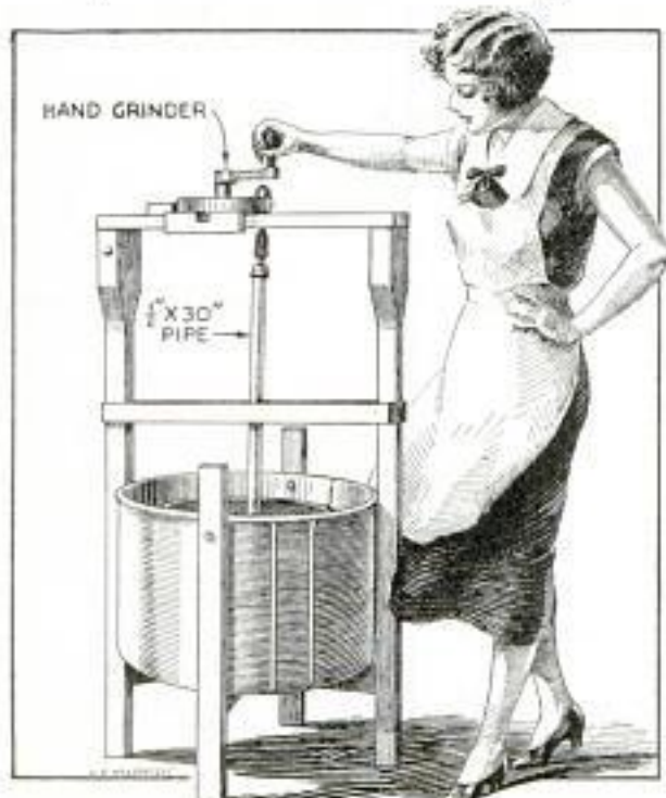
Whirling Clothes a Few Minutes in This Machine Makes Them Dry Enough to Be Ironed
