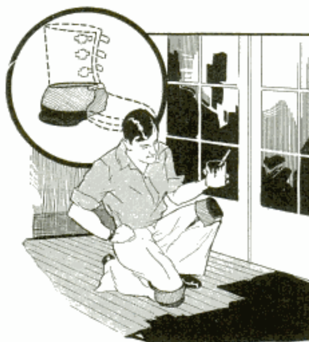
Comfortable Knee Pads Made by Cutting Out Heel Portion of Old Overshoes
