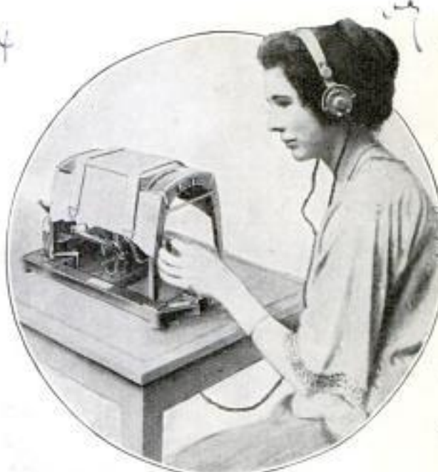
Courtesy American Braille Press Device for Turning Printed Letters into Sound Being Used by Blind Girl
