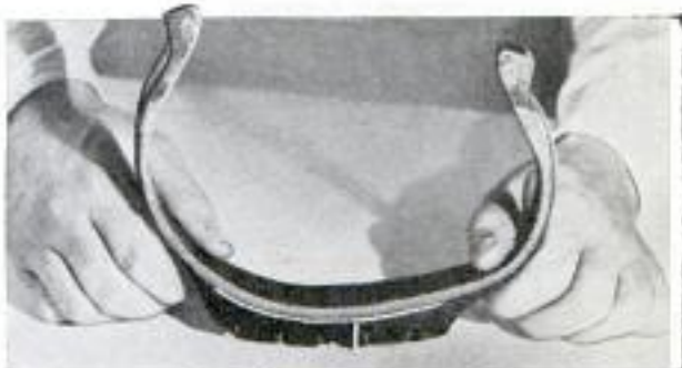
The Tread of a New Tire Is Heavy Enough to Withstand Tacks without Puncturing Tube
