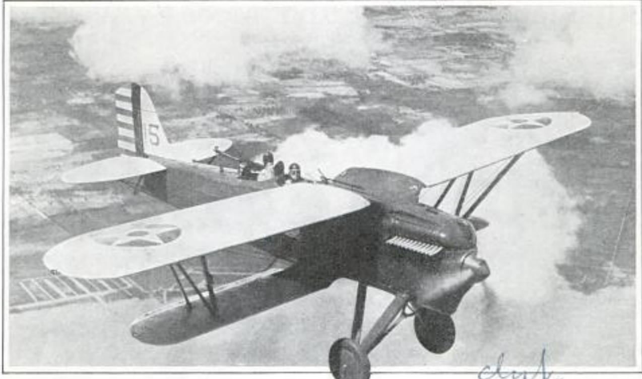
Two-Man Pursuit Plane Recently Developed for the Army; It Is as Fast as a Single-Seater and Has the Added Advantage of a Gunner in the Back to Protect Craft from a Rear Attack
