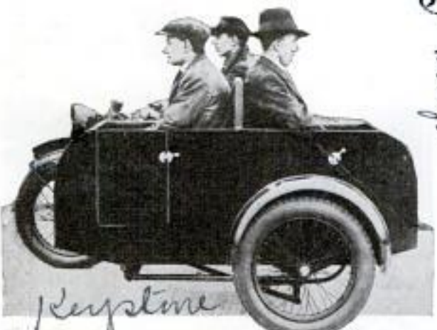
This Police-Patrol Motorcycle Has Sidecar for Two with Seat Arrangement as Shown
