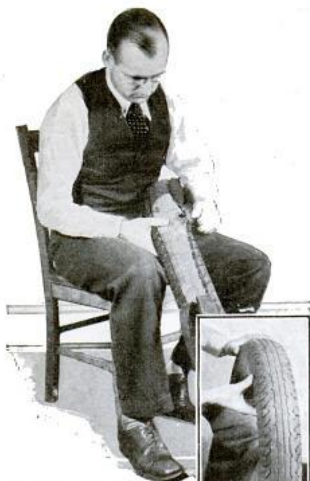
Tire Injuries Are Not Always Apparent: This Casing Seems Good for Many More Miles, but When Torn Down, Reveals Serious Carcass Injuries
