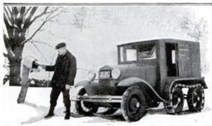
Runners, Attached to Front Axle, and Two-Extra Wheels with Tractor Drive Convert This Car into an Auto Sled
