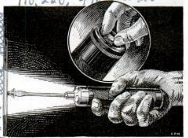
Screwdriver with Flashlight in Handle to Illuminate Work; Button in Handle Controls Light
