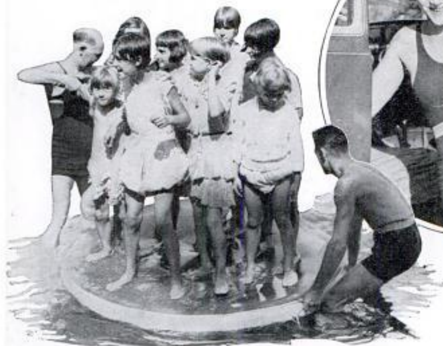
Collapsible Rubber Boat Resembling an Inflated Auto Tube with a Double Cover; It Can Be Used as a Raft or Propelled by Rocking
