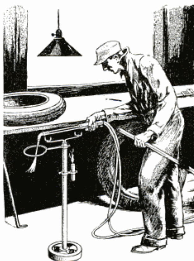
Sturdy Rack for Welding Torch Is Fitted with Pilot Light and Flame Guard
