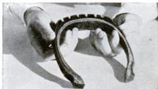
Cross Section of "Retreaded Tire" Turned Out by Slipshod Methods May Look Serviceable...
