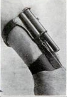
Tear-Gas Gun for Wrist Which Is Fired by Wire Leading from Trigger to Ring on Middle Finger
