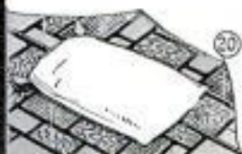
20 WHEN LINOLEUM IS CEMENTED IN PLACE, SAND BAGS OR OTHER WEIGHTS ARE LAID OVER SEAMS UNTIL CEMENT IS DRY
