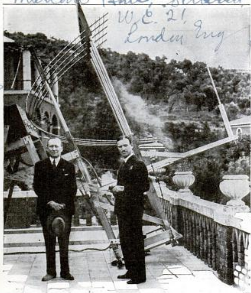
Equipment for Overcoming Curvature of Earth Is Used by Marconi in Successful Transmission by Ultra-Short-Wave Radio
