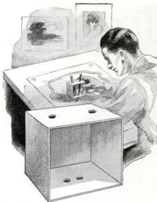
Emergency Double-Line Ruling Pen Made by Inserting Ordinary Ruling Pens in Side of Box
