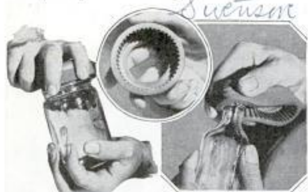
Rubber Wrench for Removing Screw Caps from Jars and Bottles with a Twist of the Wrist
