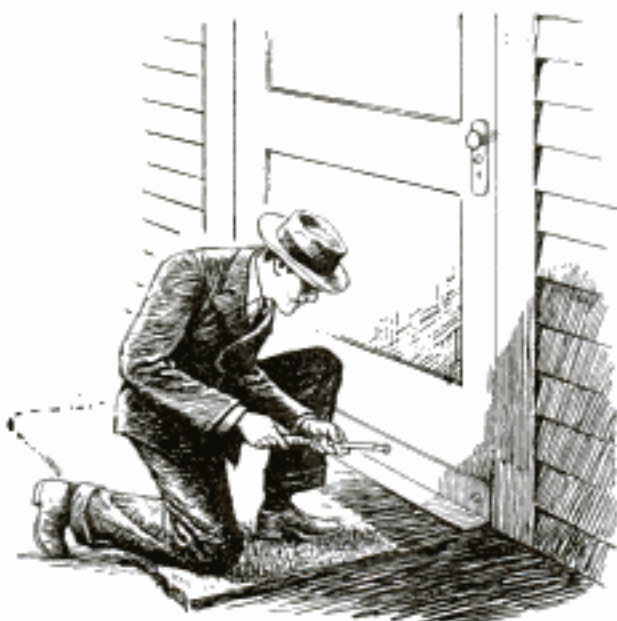
Sheet-Metal Scraper Prevents Accumulation and Packing of Snow in Front of Door
