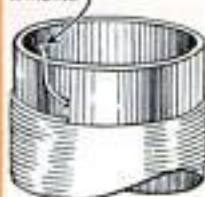
WIRE THRUST THROUGH HOLES IN TUBE TO SECURE WINDING
