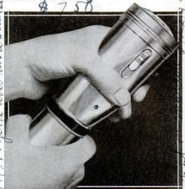
Flashlight without a Battery; Twisting Small End Winds a Spring Which Operates a Generator
