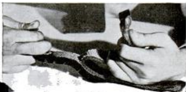
but, in This Case, Vulcanizing Was Improper and the Tread Easily Separates from Body
