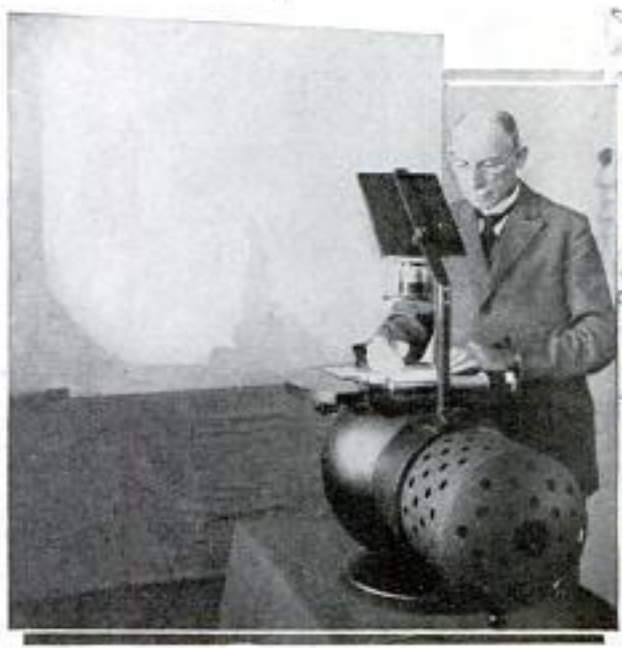
Drawings and Notes Made by Lecturer Are Flashed on Screen as He Writes and Talks
