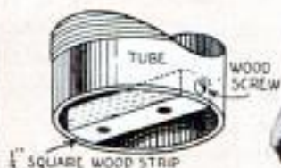
Above, a Simple Method of Mounting Coils Wound on Bakelite or Cardboard Tubing; the Mounting Strip May Be Fastened to the Form with Thumb-tacks or Wood Screws
