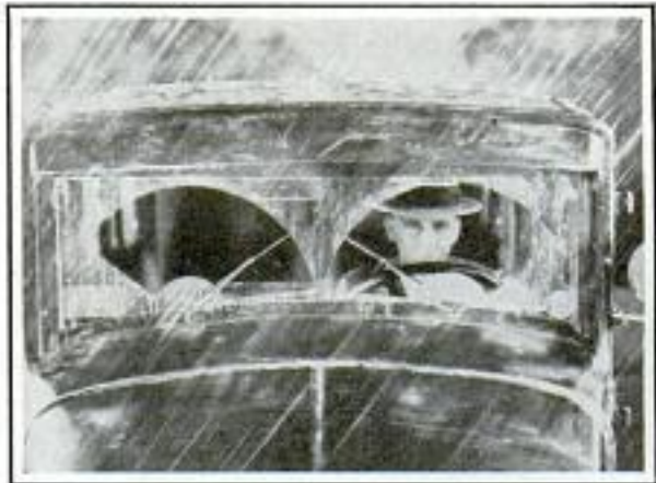
New Windshield Wiper, Fastened at the Bottom, Keeps Rain from Running into Cleaned Area
