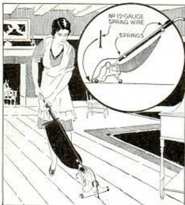
Spring-Wire Attachment on Vacuum Cleaner Loosens Dirt Accumulations in Cracks of Old Floors
