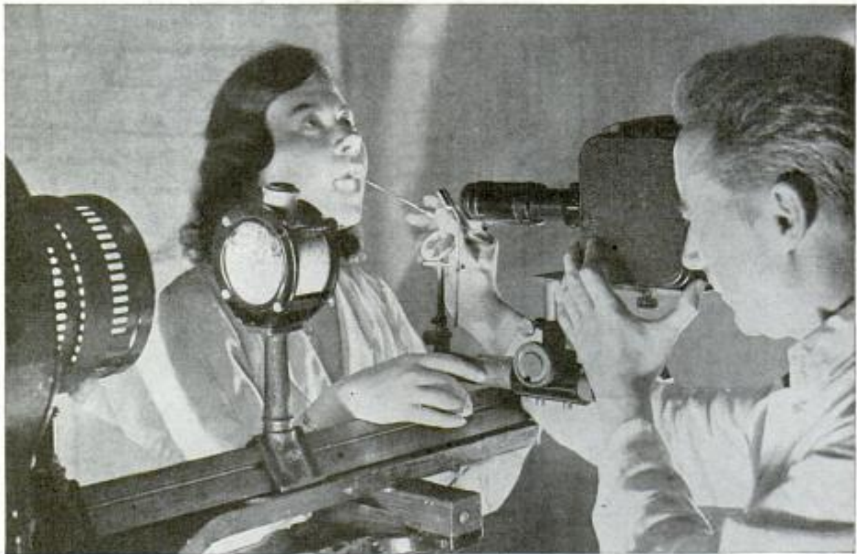
As a Guidance in Teaching Mutes to Speak, German Scientists Are Using Moving Pictures Showing the Pupils the Oscillations of the Vocal Organs, Which the Mutes Then Try to Imitate © New York Times
