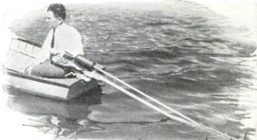
Rowboat Equipped with Electric Oar Operated from Storage Battery; the Outfit Is Silent, Thus Being Suitable for Fishermen
