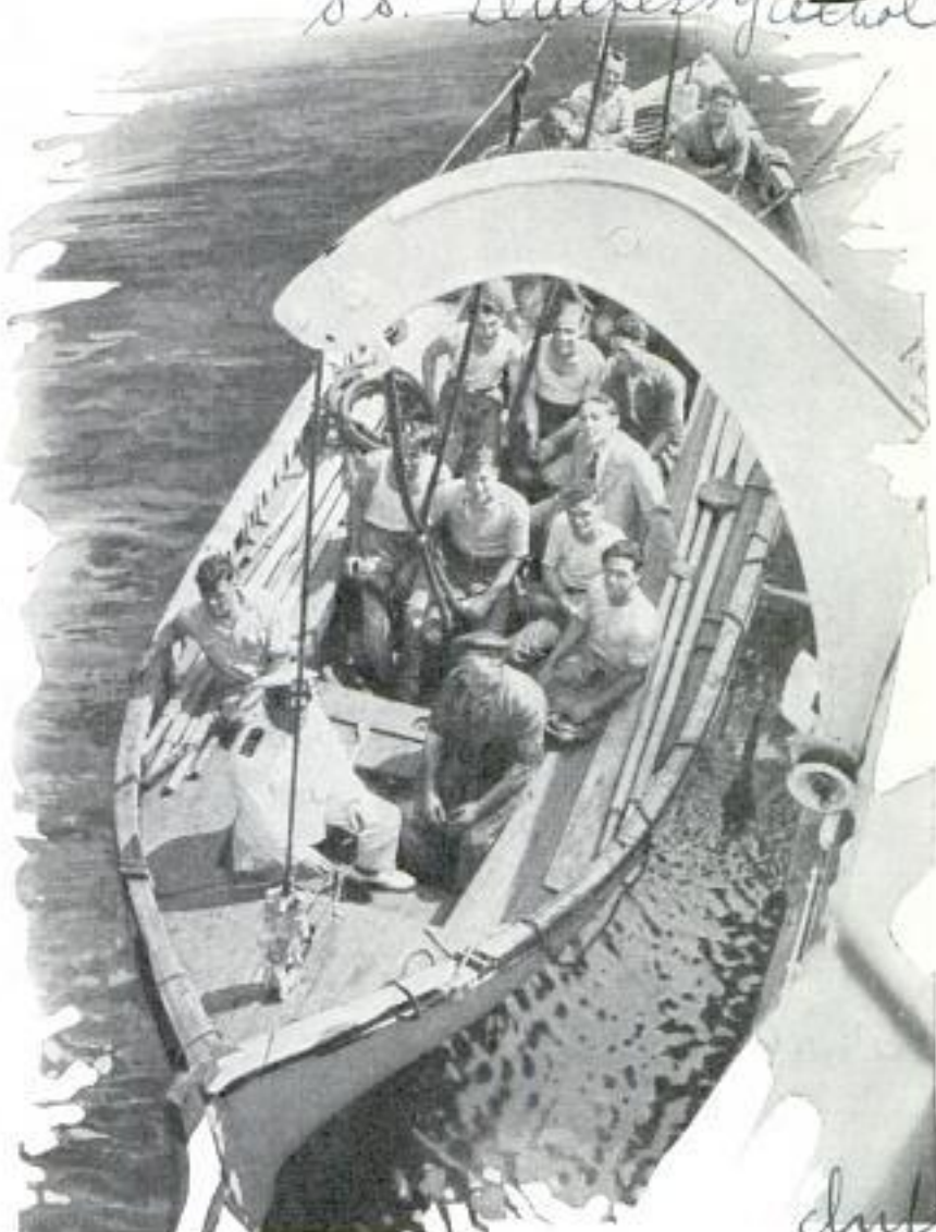
This New Davit and Release Detaches Both Ends of the Lifeboat at the Same Time, Preventing "Snaking" or Capsizing
