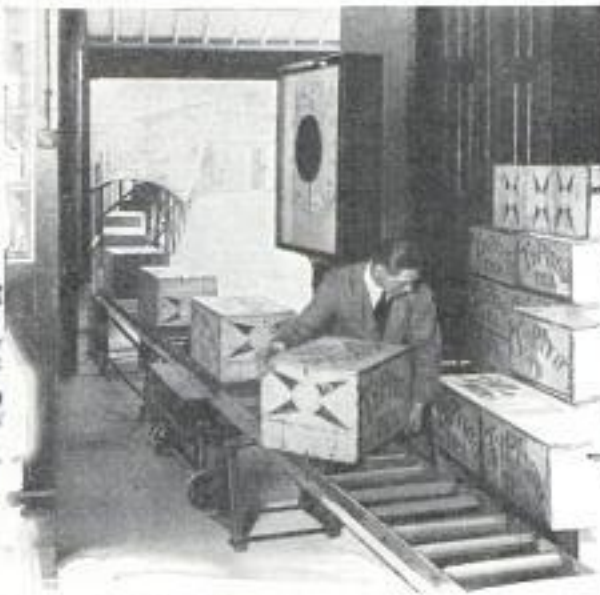
Courtesy Merris Loughboro Boxes Being Weighed and Counted Automatically as They Move along a Conveyor System
