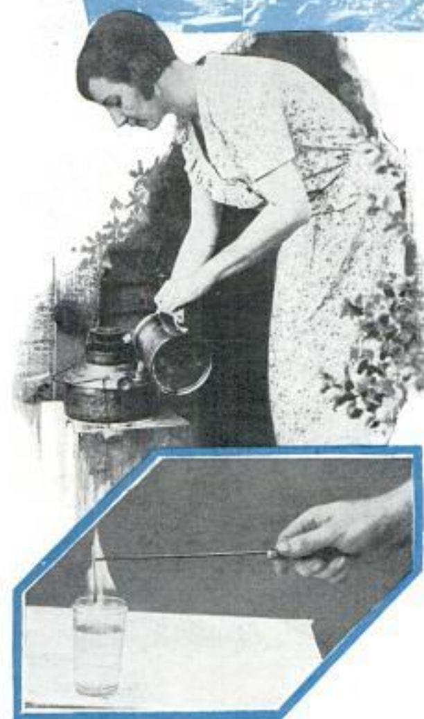
Center, Handling Kerosene Out of Doors; Below, Gasoline Vapors Ignite at Ordinary Temperatures
