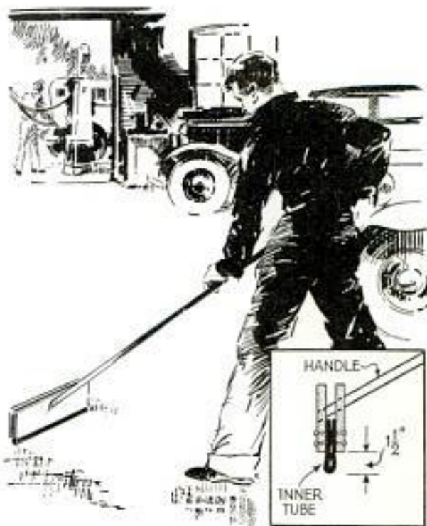
Piece of Inner Tube Nailed between Two Boards and Fitted with Handle Makes Floor Squeegee
