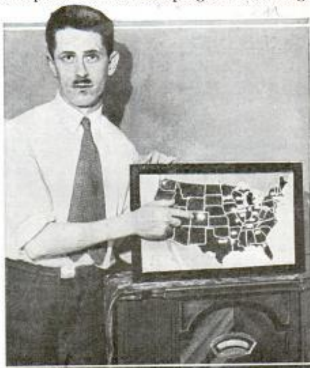
When Dial Is Turned to Wavelength of Radio Station, Map Shows Its Location
