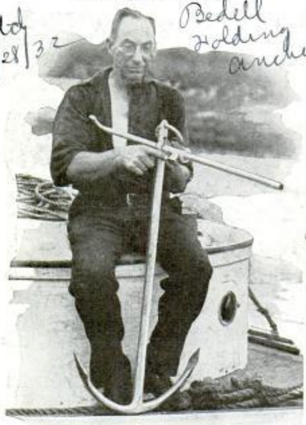
Cross Rod at Top Hangs at an Angle, Helping to Force Anchor into the Bottom
