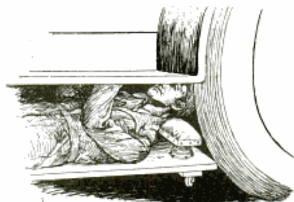
Springs under the Head Cushion Improve Garage Creeper
