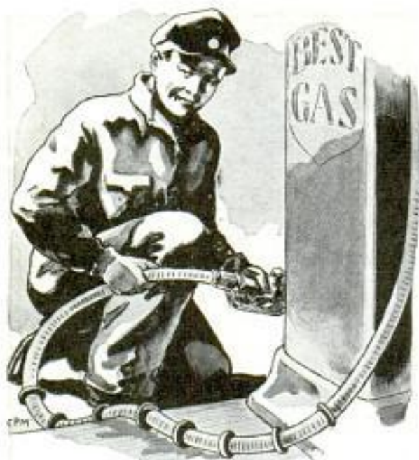
Rubber Washers Spaced Evenly on Gasoline-Pump Hose Protect It against Wear
