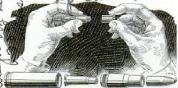
Reload Chamber to Give Reduced Power to High-Power Rifles; Note the Method of Assembly
