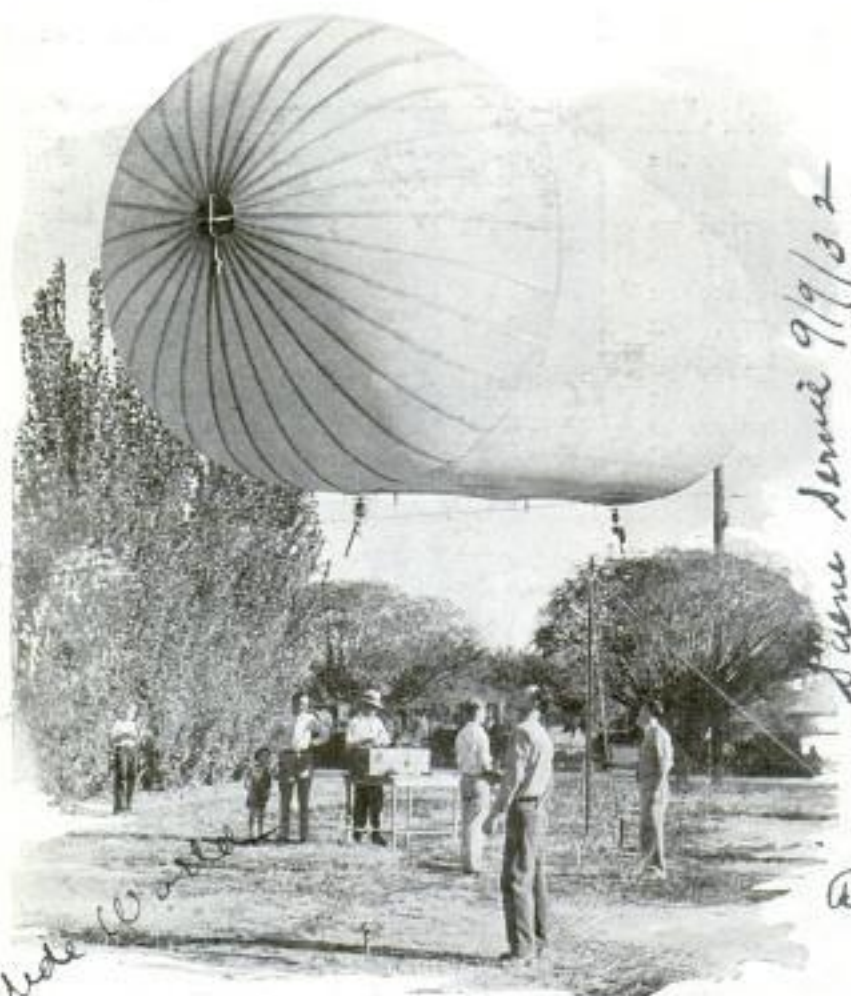
Small Dirigible of Semirigid Type Which Is Able to Land under Its Own Power without the Assistance of a Ground Crew
