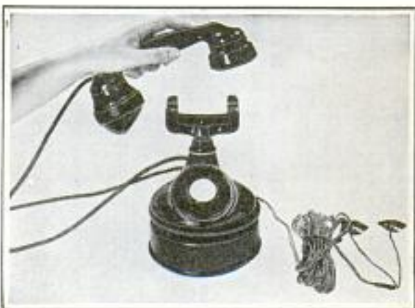
Platform Switch Turns Off Set When Phone Is Removed from the Hook
