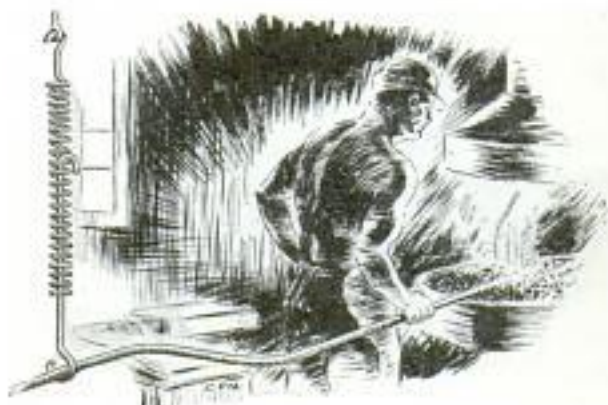
End of Long Work Conveniently Held for Drilling or Heating by Means of an Adjustable Hook
