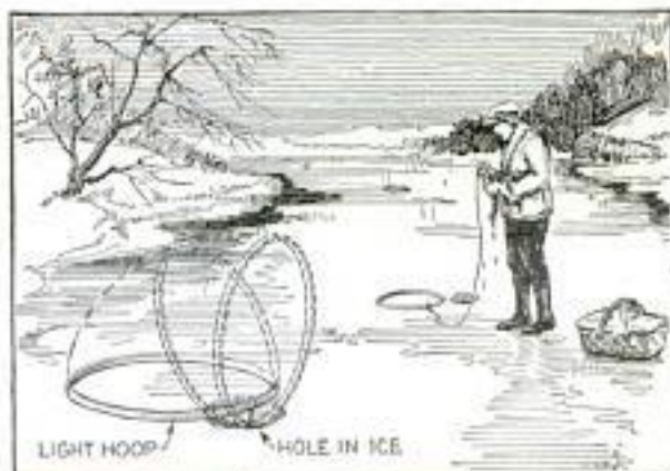
Signal Made from Barrel Hoop Gives Warning of Catch When Fishing through Ice
