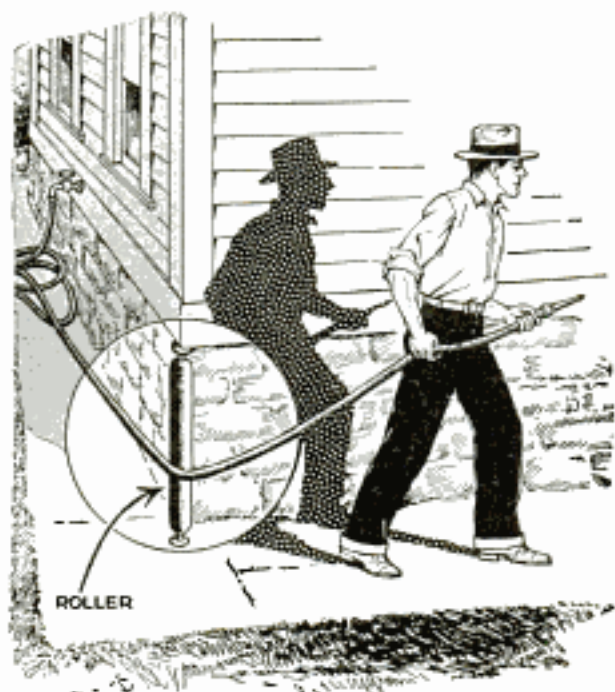
Hose Protected against Sharp Edges of House Corner by Vertically Mounted Roller
