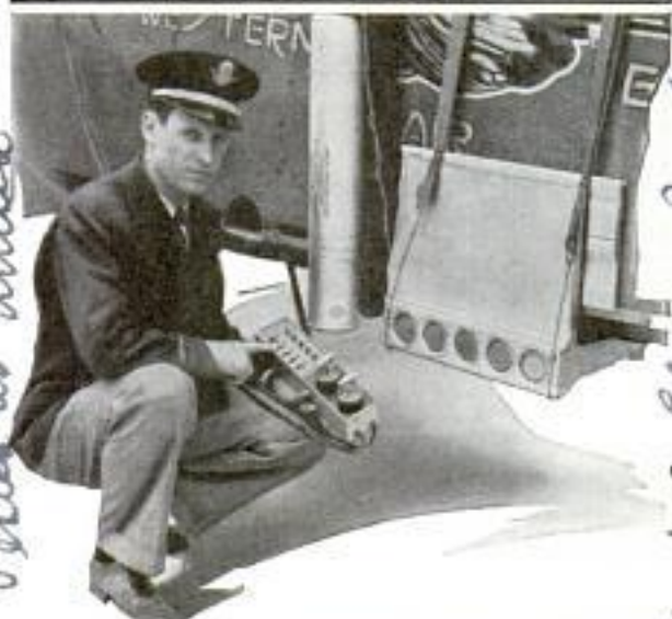
Set in a Special Frame, Electric Flares Are Discharged from Plane to Aid Night Landings
