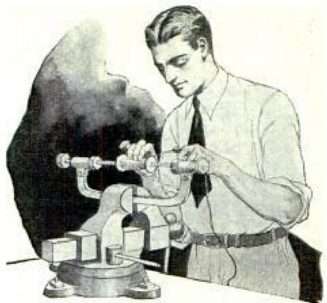
Fitted with Centers and Clamped in a Vise, Hacksaw Frame Holds Core for Winding Coils
