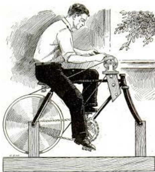
Old Bicycle Used as Power Supply for Driving Grinders and Other Rotary Tools
