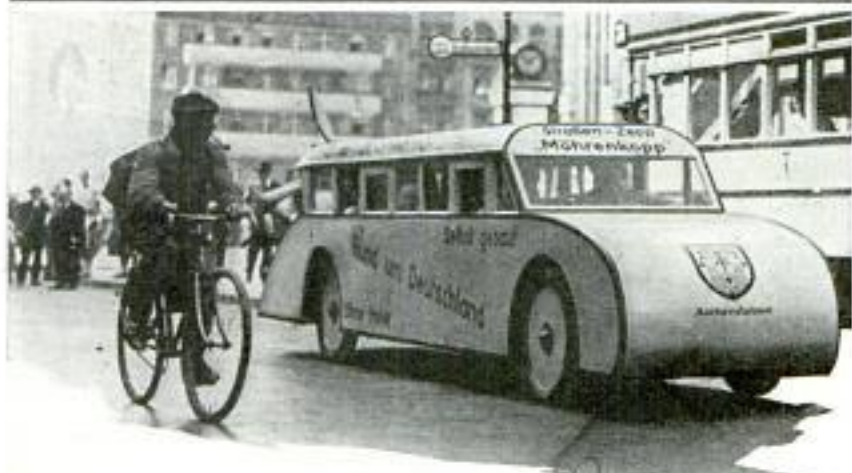
This Zeppelin-Like Vehicle Is Driven by Foot Power; Its Operators Pedaled the Car along Berlin Street on Tour of Germany
