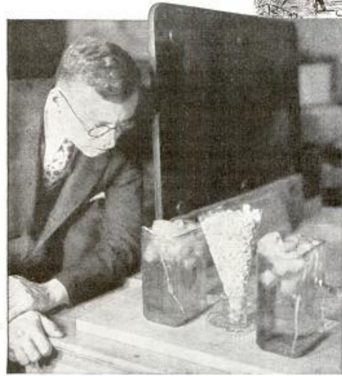
Popping Corn between Iced-Water Electrodes, Which Are Connected to a High-Frequency Heater
