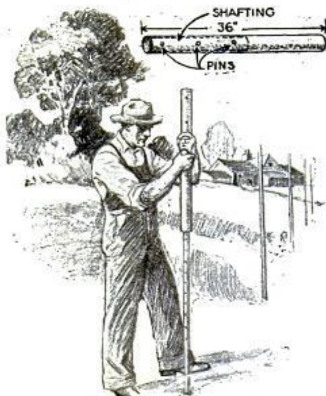
Steel Fence Posts with the Aid of a Pipe Containing Steel Shafting
