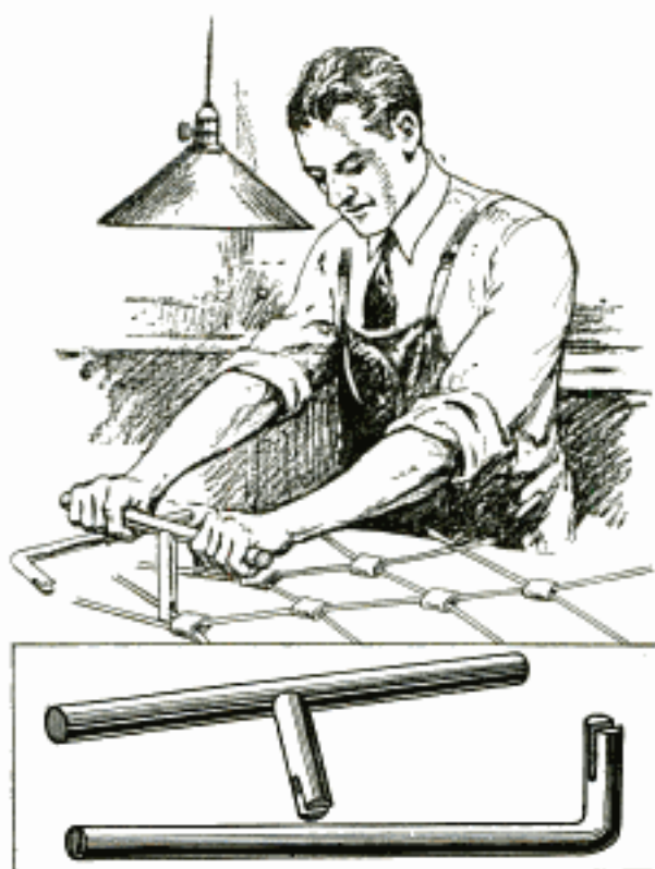
Wire Novelties Made in the Home Workshop with Aid of These Two Simple Bending Tools
