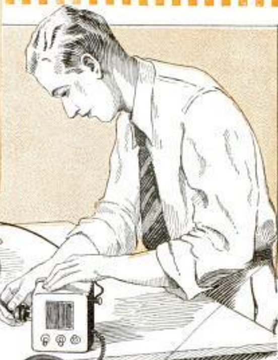
Interference Analyzer Contains Several Standard Filter Circuits Any of Which May Be Switched In or Out to Determine the Proper Filter to Use
