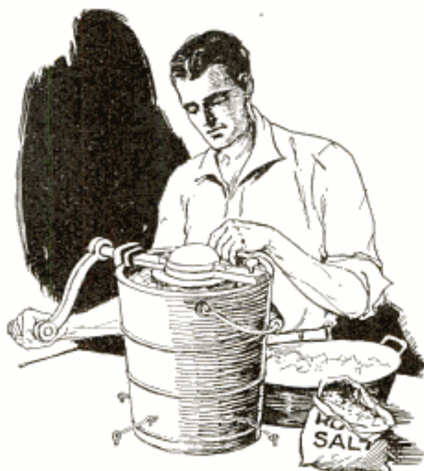
Turning the Ice-Cream Freezer Made Easier by Anchoring It to the Floor or Table
