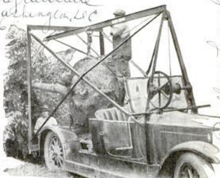
Whole Trees Are Picked Up and Moved by a Nurseryman Who Built This Windlass and Frame on a Truck
