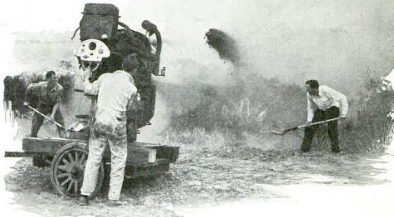
Wind Machine Developed for the Movies Being Used to Blow Out a Brush Fire; Dirt and Sand Are Shoveled into the Air Stream from the Propeller to Smother the Flames
