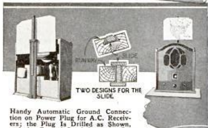
Completely Enclosed Heater Transformer Will Deliver Up to 10 Amp. at 2.5 Volts with Good Regulation for Experimental Multi-Tube Receivers
