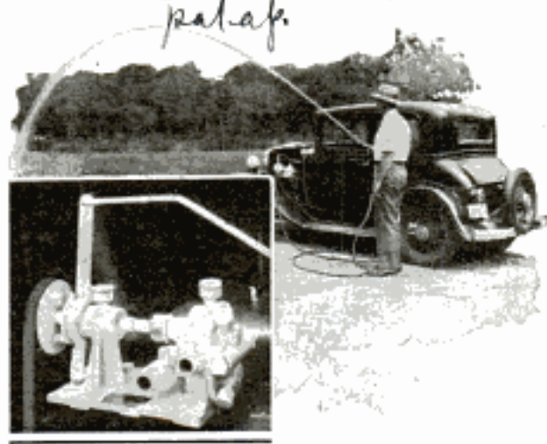
Bolted on Auto Engine, Water Pump and Hose Help in Fighting Forest and Home Fires
