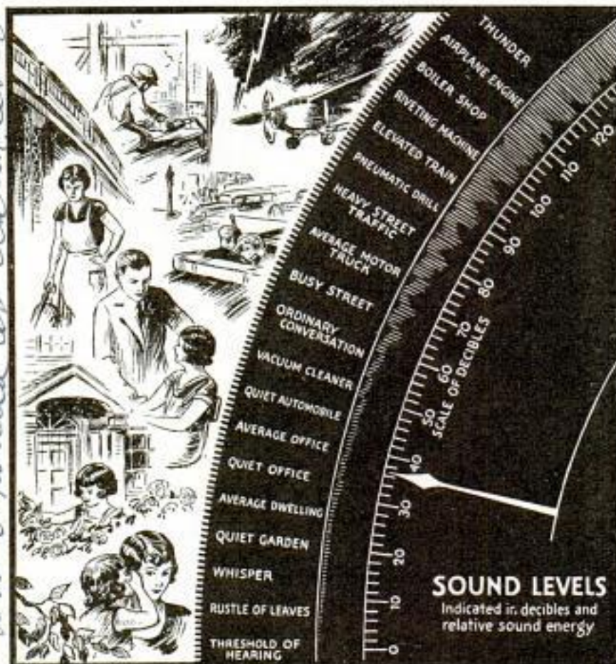
Chart Shows Relative Measurements of Noises; Right, Apparatus Used in Reducing Sound of Auto Tires
