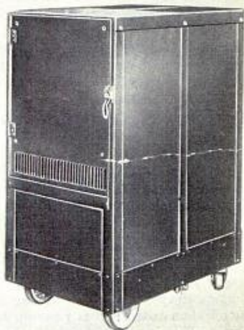
Left, Duster with Extension Tube to Reach High Fixtures; Right, Air-Cooling Unit That Holds 300 Pounds of Ice; Small Fan Draws Air through Front and Forces It Out through Controlling Damper Openings at Top; Capacity, 400 Cubic Feet a Minute
