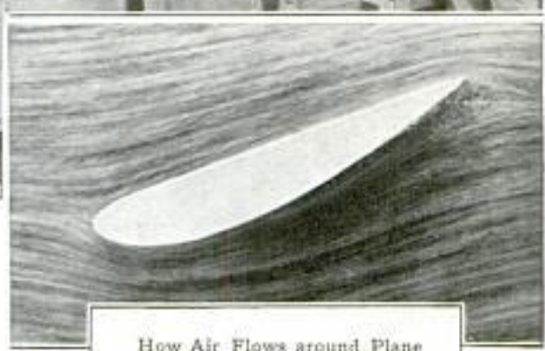
Camera on Moving Carriage over Tank Photographs Flow of Liquid around Objects Tested for Streamlining
