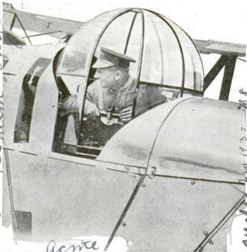
Glass Cage over Gunner's Cockpit of British Fighting Plane; the Dome Protects the Occupant and Increases Accuracy of Fire
