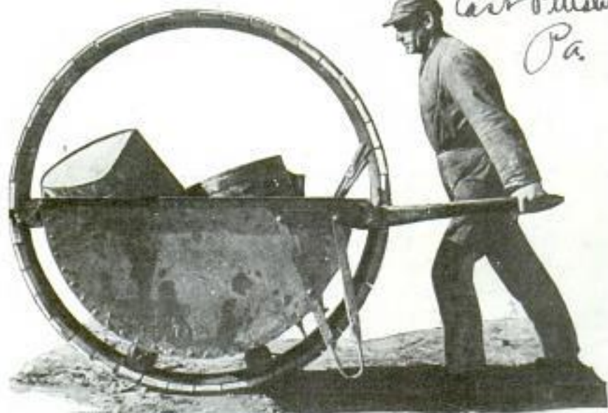
Rolling on the Inside of This Big Wheel, a New-Type Wheelbarrow Is Designed for Hauling Larger Loads with Less Effort
