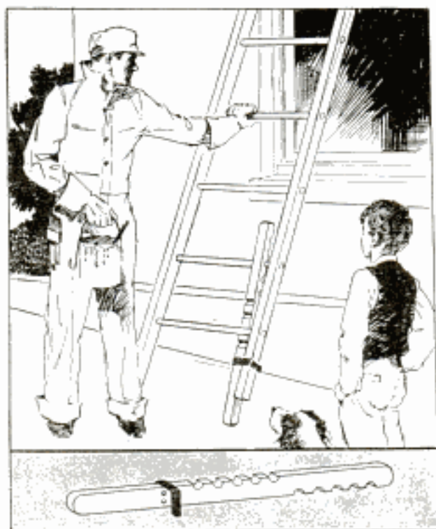
Adjustable Extension Leg Keeps Ladder from Sliding Toward One Side on Uneven Ground
