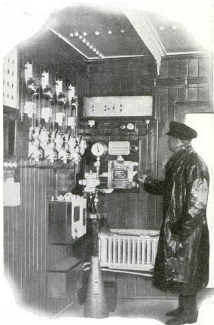
Junior Officer Turning the Small Brass Handle That Closes the Hydraulically Operated Watertight Doors during a Storm
