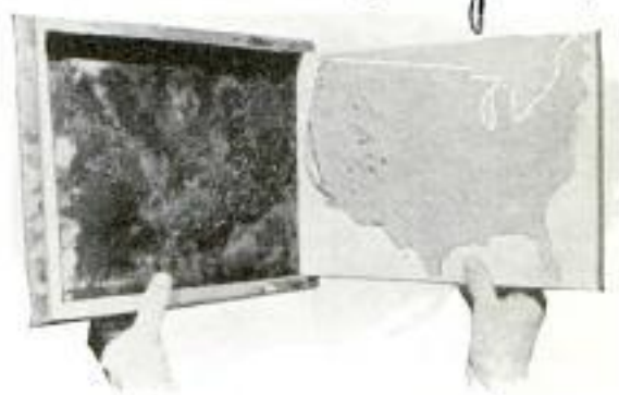
Packed with Plastic Material, These Molds Produce Relief Maps for the Classroom
