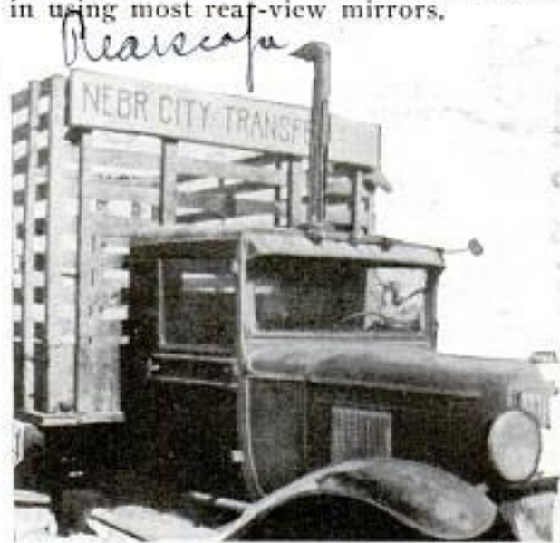
Truck Equipped with a Periscope Which Can Be Elevated to Permit Driver to Obtain Rear View
