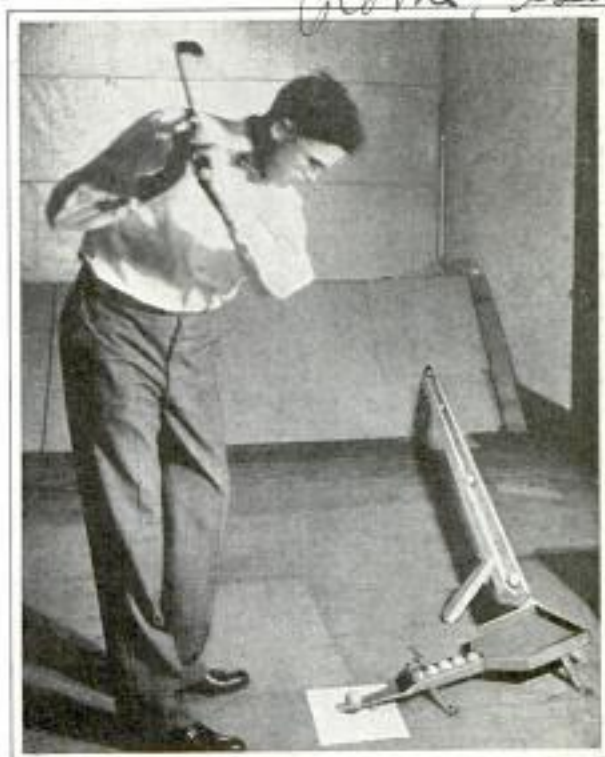
When Golf Ball Is Driven against Backstop, Trough Returns It to Tee-Up Position
