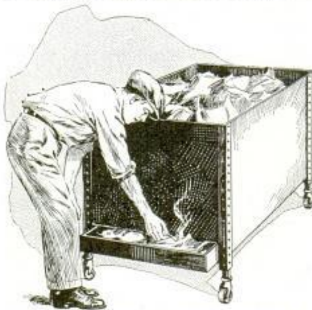
Old Sheet-Metal Tank, Fitted with Casters and a Sliding Ash Pan, Forms This Wheeled Incinerator
