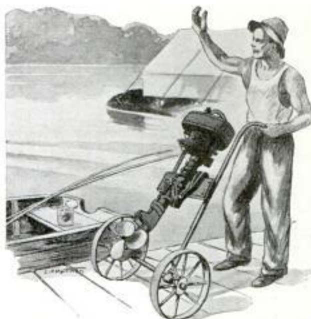
Wheeled Truck, Made of Pipe and Fittings, for Transporting Heavy Outboard Motors
