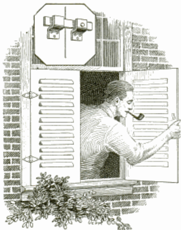
Window Shutters Made from Auto Hoods Permit Adequate Ventilation and Safeguard against Intruders
