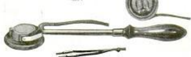
Headphone on Extension Handle as an Aid to the Partially Deaf
