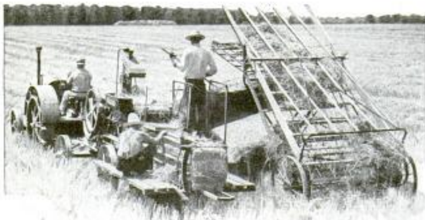
Machine Fed by Hay Loader Bales Scattered Straw Left in Field by Combined Harvester and Thresher
