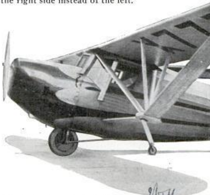
Note the One Large Landing Wheel on This Plane; Small Wheel Helps Steady the Ship in Standing Position
