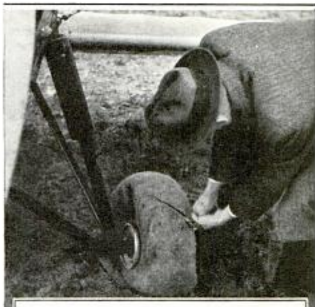
Slashing Hole in an Airwheel Tire to Test the Effects of a Blowout of Such a Tire
