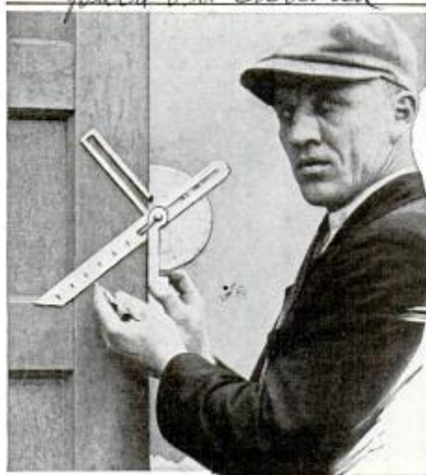
This Adjustable Square Saves Four-Fifths of Time Carpenter Usually Needs for Measurements
