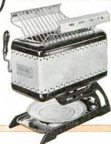
Above, Gas Broiler Which Applies Heat to Both Sides of Food Simultaneously; the Grid Automatically Adjusts Itself to Thickness of Meat; Plates Are Warmed Underneath While Meat Cooks
