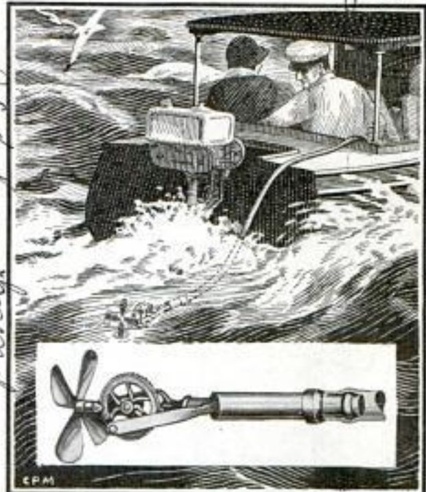
Literally Pulling the Water Out of a Boat, This Bailer Is Propeller Driven
