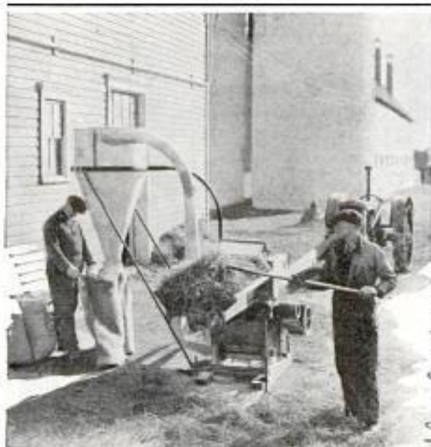
This Mill for Grinding Feed Is Operated by Tractor or Farm Engine
