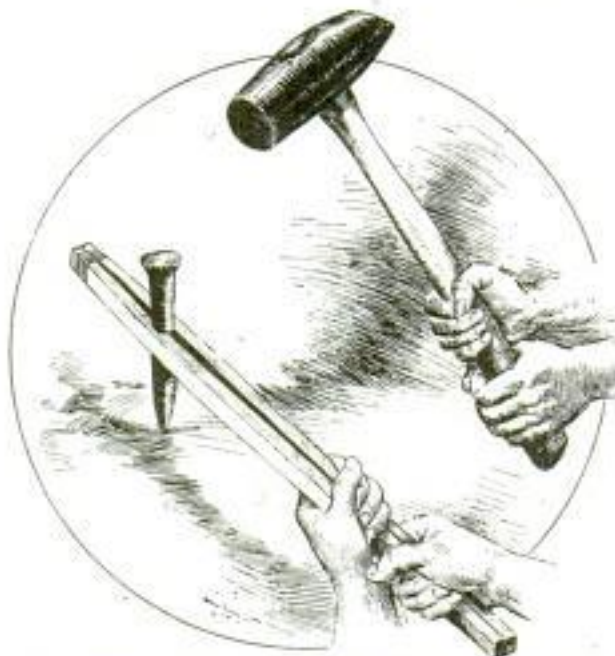
Two Wooden Sticks Hold Chisel Firmly without Danger of Injuring the Hands
