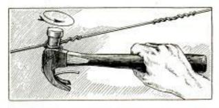
Emergency Repair on Your Wire Fence Can Be Quickly Accomplished with Aid of a Claw Hammer
