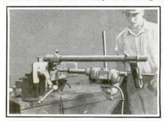
Improvised Mount Holds Electric Drill in Either Vertical or Horizontal Position
