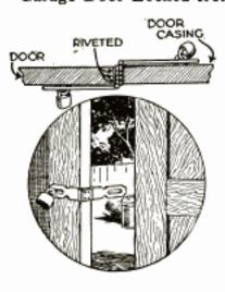
In order to be able to lock or unlock his garage from either the inside or outside, a car owner riveted the short ends of two hasps together as shown. When attached in this way, the longer ends of the hasps can be slipped over staples in the door and the casing, and both sides can be padlocked.
