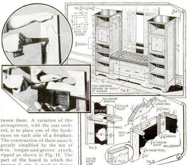
part of the board in which the groove is cut, is used to house the panel, while the other portion holds the shelf cleats, etc. Tenons
