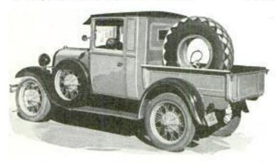
Large Truck Tire Mounted on Dealer's Service Car Forms Portable Air Tank for Inflating Smaller Tires
