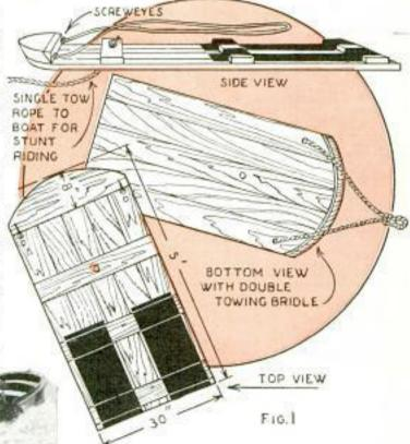
jointed with a plane, and crosspieces of the same stock are then screwed on securely, after which a semicircular bow is marked and sawed off. It is advisable to use 134-in, screws to join the component pieces, the screws being driven in from both sides to obtain additional strength. All edges of the crosspieces should be bev-
