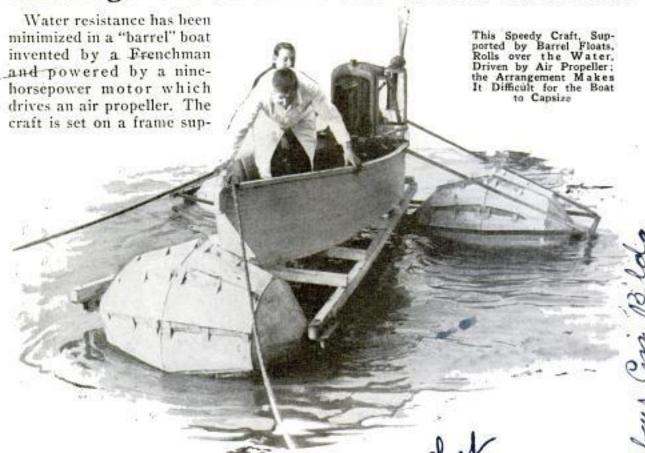
ported by three barrel-shaped floats, and the air propeller tends to decrease the draft until the boat skims over the surface. It is virtually impossible to capsize the craft which has a speed of more than eighty-five miles an hour, according to the inventor.
