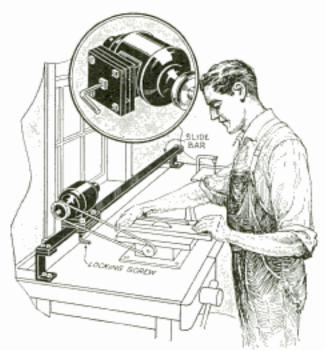
Here's a Simple Method of Using One Motor to Drive a Number of Home-Workshop Machines
