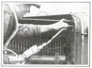
Angle Bit Set in Steel Casing Which Enables Operator to Drill at Any, Angle Necessary
