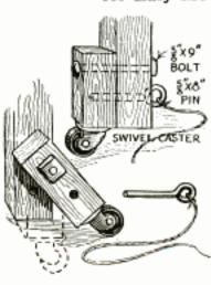
Having a heavy work-benchthat had to be moved around in the shop frequently, I made the illustrated caster attachment. The casters are fastened to short blocks pivoted to the
