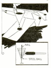
Sealing wax is easily melted with a soldering iron when this attachment is used. It consists of a sheetmetal cone with a length of tubing soldered to one side for the insertion of a soldering or
