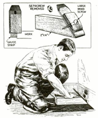
Bull-Nose Plane for Scraping Floors Improvised from Wooden Block and Plane Iron
