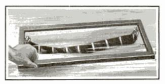
Roll Films Held on Floating Frame Can Be Washed in Running Water without Scratching
