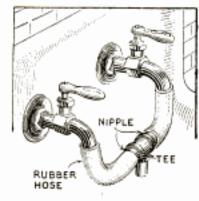
and joined in the middle by a nipple screwed into the tee.
