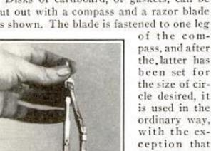
Razor Blade Attached to Compass for Cutting Gaskets
