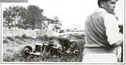
Wreck of Arnold's Car in 1931 Indianapolis Race; Upper Left, Hitting the Concrete Wall Crushed the Wheel, but the Tire Stood the Shock
