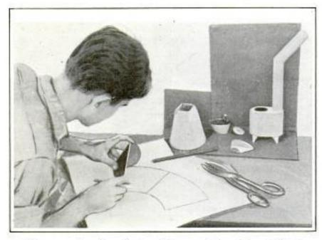
on the round end, and to roll up on the corners of the attached rectangle or square as the rolling progresses, a true pattern will result. The square or rectangle should not be the full rectangle or square that is desired in the finished pattern but only half of it. Do not forget to allow for the overlapping of edges wherever a seam is to be made.
