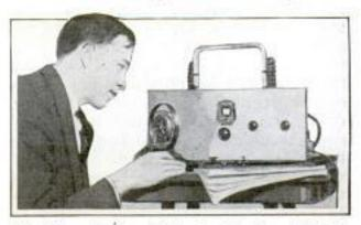
Short-Wave Receiver Equipped with Neon Tube for Visual Signals
