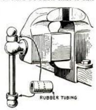
can be slipped directly on the shank, after which tape is wrapped around to hold it in place.
