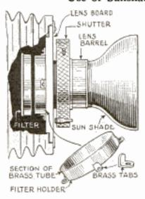
A filter and a sunshade can be used on a camera at the same time by mounting the former behind the lens inside of the bellows. Brass tabs are soldered to a brass ring of suitable diameter to fit the lens and the
