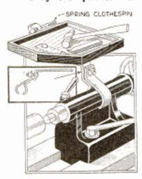
Machinists will find this tray convenient as it holds the tools at hand near the work. A flatmetal clamp is made to fit the tailstock and is screwed or bolted to the bottom of the tray. For holding delicate
