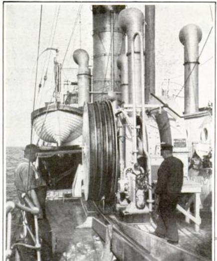
with water to keep the vessel on an even keel. In addition to the cable rolls in the hold and unreeling equipment on deck, the ship has comfortable cabins for officers and crew.
