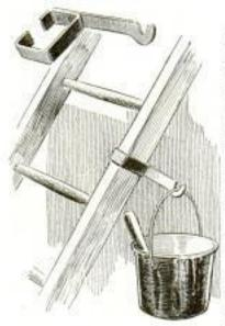
Where it is necessary to hold a paint bucket at various heights while progressing with the work, this sliding hook, which can be slipped up or down and set at any convenient position on the ladder, has been found to be of consid-
