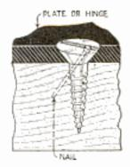
small hole diagonally through the screw head to receive a small brad.
