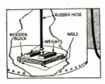
in the center of a weighted block, enables large tanks to be drained without attention. A nail is driven into each corner of the board, the
