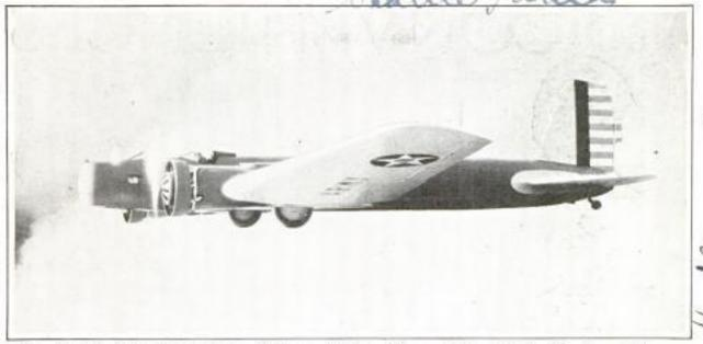
Army Bombing Plane Shaped Like an Albatross with Low Wings and Retractable Landing Gear; It Has a Long Flying Range and Its Top Speed Is Almost 190 Miles an Hour
