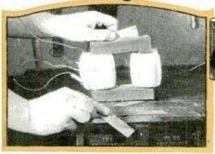
DELIVERING from 2 to 22 volts, a small step-down transformer can be used for operating doorbells, door openers, toy trains, small motors, Christmastree lights connected in parallel, signs with low-voltage lamps, tungar rectifier bulbs, thermostats, etc. Of course, a transformer can only be used in an alternating-current line and the one described here is designed for 110 volts at 60 cycles.
