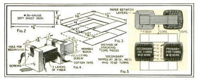
put the same number of turns in each layer except the last so that, if you lose count, it will be easier to check back. After you have wound the 590 turns, cut off the wire, allowing an 8-in. lead, and tie the coil tight with the four tapes. The end block is then removed and the coil carefully taken off the form. Taping the coil consists in wrapping it with a single overlap-
