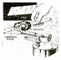
from running up the blade by means of a potato as shown in the drawing. Allow the heated portion to cool gradually and then drill a hole in it to fit the pin of a saw frame.
