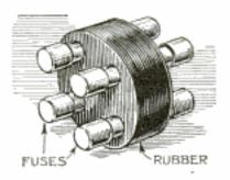
rubber disk as shown. When a fuse burns out, I need only to pull out the old one, turn the rubber disk and put in the new. —F. B. Stoner, Jr., Riverside, Calif.
