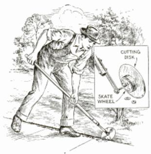
Sharp Rotating Disk on Homemade Lawn-Edging Tool Cuts Sod Quickly
