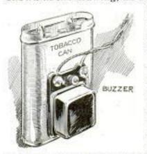
can be made to produce a greatly intensified sound. The can acts as a resonator and is attached to the wall. The lid is removed. This device was found especially
