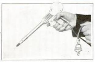
When This Soldering Iron Is Hot, Pulling Trigger Releases Solder from Barrel
