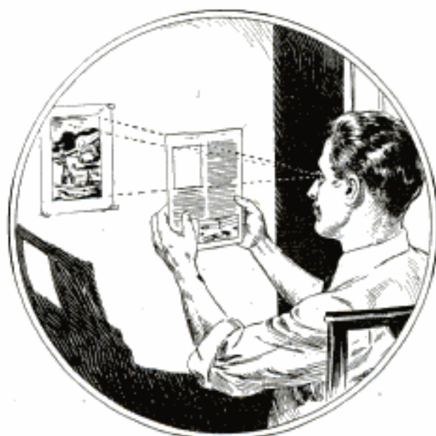
Method of Determining the Finished Size of Pictures for Use on Page of Type
