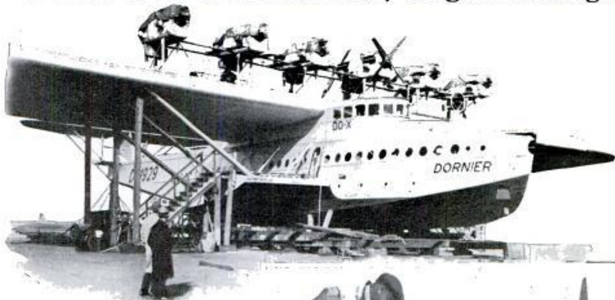
The "Do-X" in "Drydock" for Overhauling at Long Island, Above, and, at Right, Reinstalling the Engines After the Power Had Been Increased
