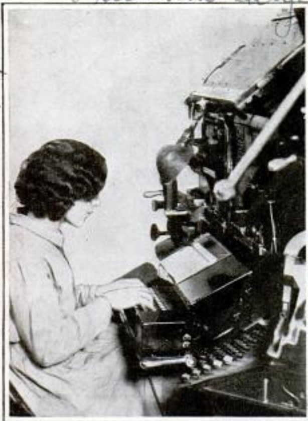
This Typesetting Machine, Fitted with a Typewriter Keyboard, Makes Work Easier for Operator
