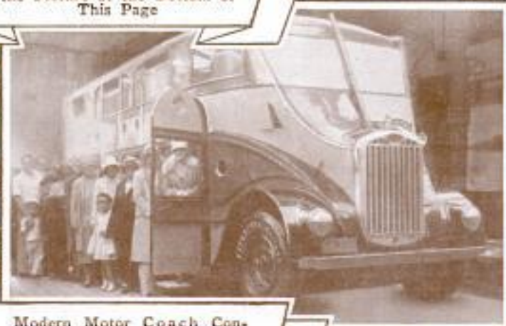
Modern Motor Coach Containing Seating and Sleeping Accommodations for Twenty-Six Passengers; Its Engine Can Be Quickly Removed
