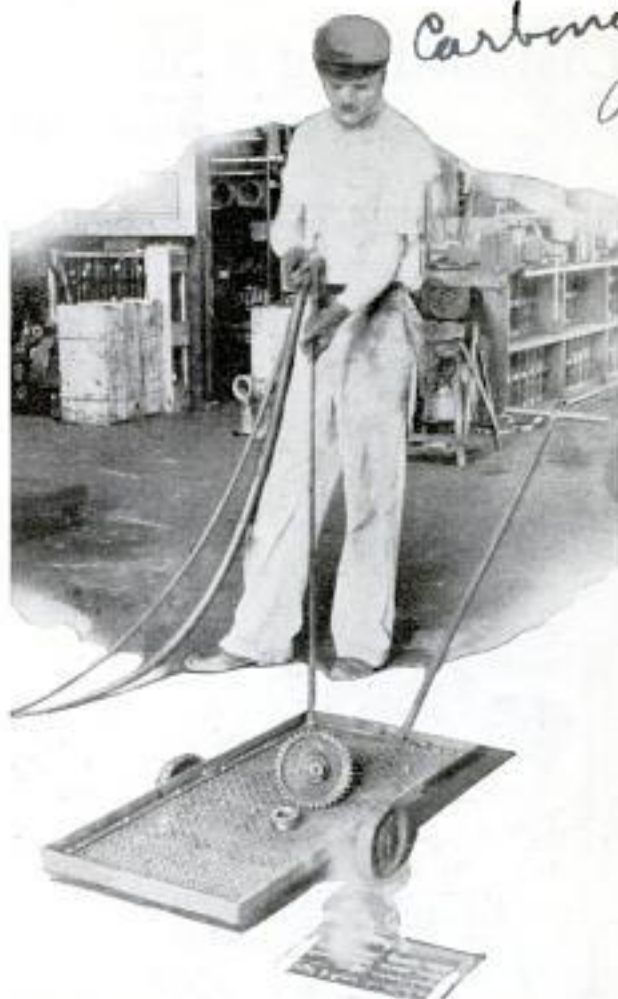
Small Parts Placed in Screen-Bottomed Truck Are Pushed over Drain and Quickly Cleaned with Steam
