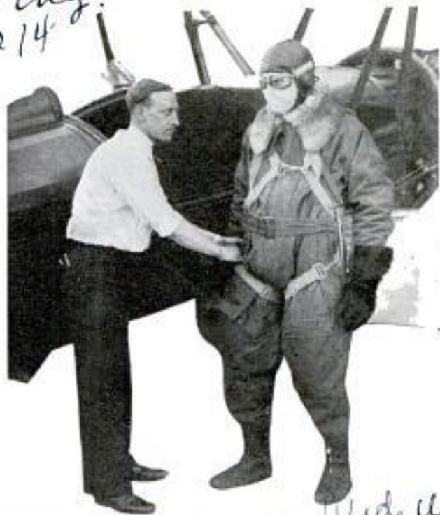
Wearing This Heated Suit, Wensinger Flies Three Miles High for Weather Information
