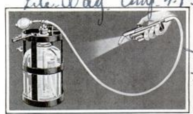
Filling the Auto Battery Is Easy with Siphon Which Has Light at End of Tube
