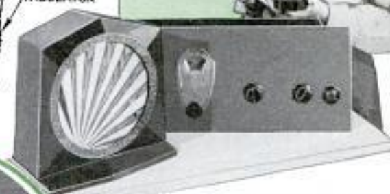
Above, Measuring Range of Coil Shunted with Variable Condenser; Hold Coil Close to Coil in Receiver Using Dial Calibrated in Kilocycles; Click in Speaker Indicates Both Coils Tuned to Same Frequency; Left, Baking-Powder Can Makes Good Coil Shield
