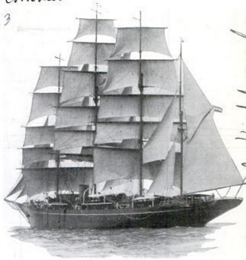
Four-Masted Bark with Giant Auxiliary Motor; Rigging on All Four Masts Is Operated Electrically
