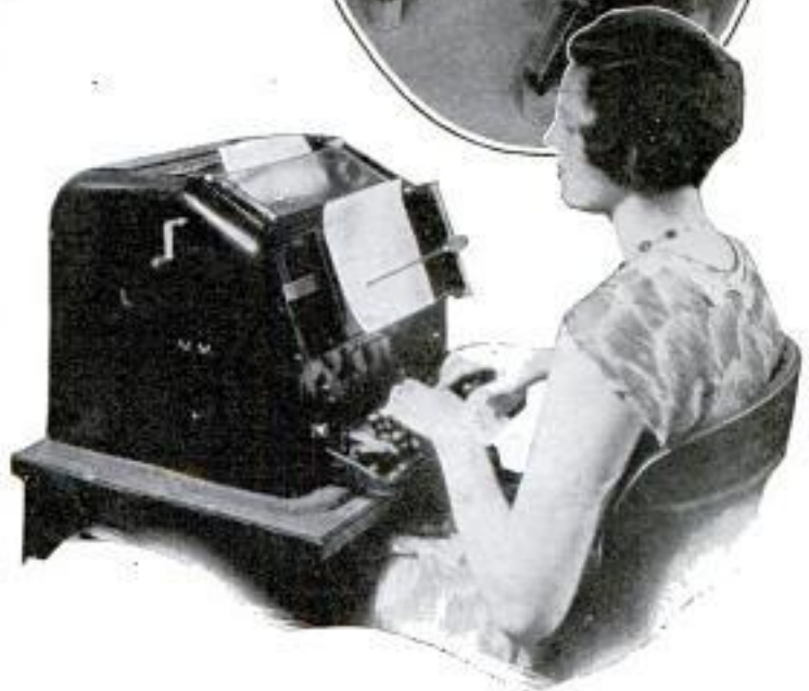
Teletypewriter Machines and Switchboard Making Possible a Two-Way Message Service between Subscribers
