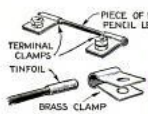
Above, 2 In. of Pencil Lead Makes Filament Resistor for 5-Volt Battery-Operated Tubes, Adjusted for Correct Voltage; Below, Small Fuse Protects Meter
