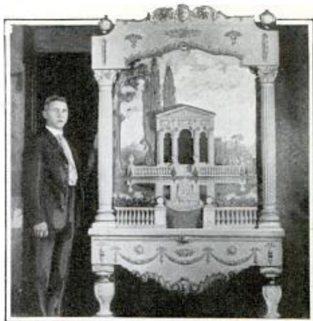
Large Speaker Baffle, Showing Cloth-Covered Grill at the Center
