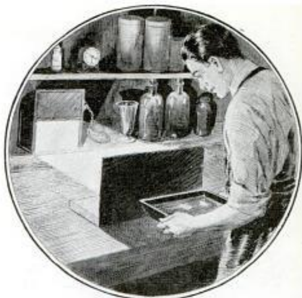
Developing Panchromatic Plates behind Screen Placed in the Light of Green Safe-Light
