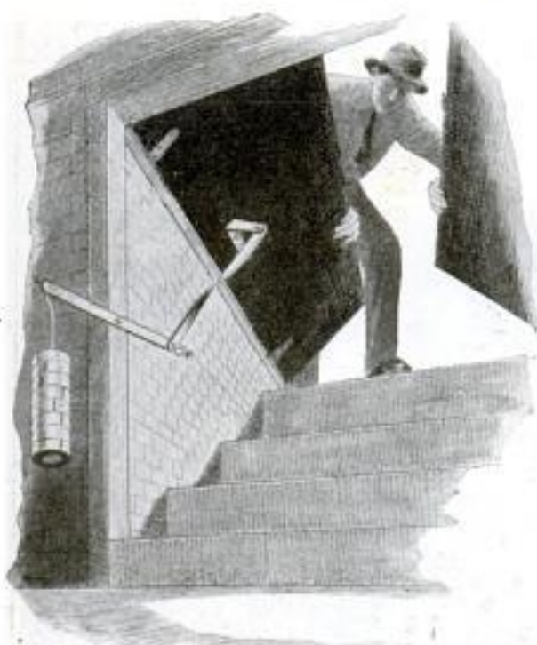
Counterweighted Cellar Doors Can Be Made to Operate Easily Enough for a Child to Open Them
