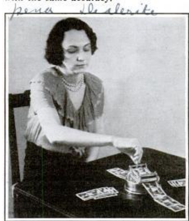
Delivering Thirteen Cards to Each Player in Ten Seconds, This Machine Makes No Misdeals
