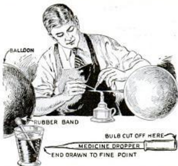
Blowtorch Made from Toy Balloon, Medicine Dropper and Alcohol Lamp Is Useful for Light Work
