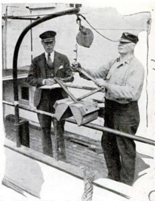
Small Clamshell Scoop Used by Bureau of Fisheries to Collect Samples from Lake Bottoms
