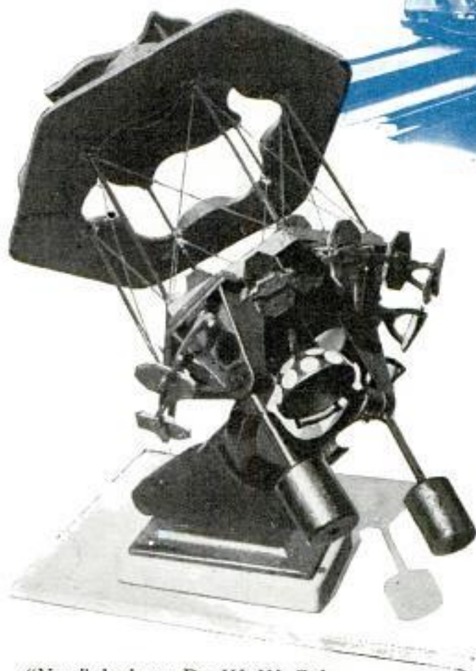
Above, Doctor Coblentz Showing How He Transforms Sunlight into Electricity; Left, Model of Solar Furnace Now under Construction
