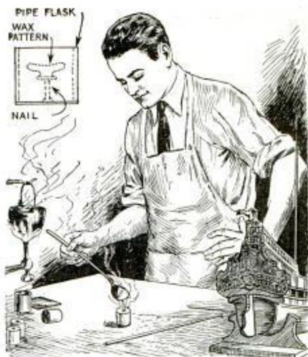
Molds for Small Model Fittings of Brass Made with Plaster Mixture and Wax Patterns
