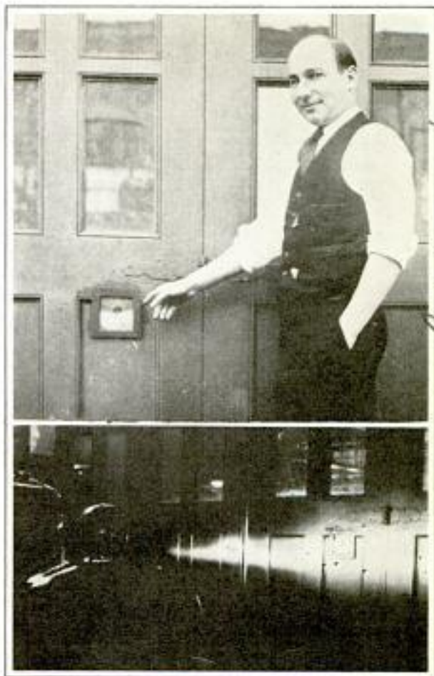
Electric Eye in Garage Door Which Actuates Opening Mechanism as Car's Lights Fall on It
