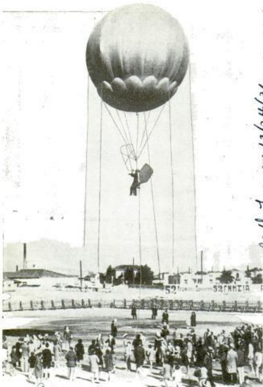
Testing a Balloon That Can Be Guided and Propelled by the Passenger, Who Manipulates the Gas Bag from His Perch beneath It
