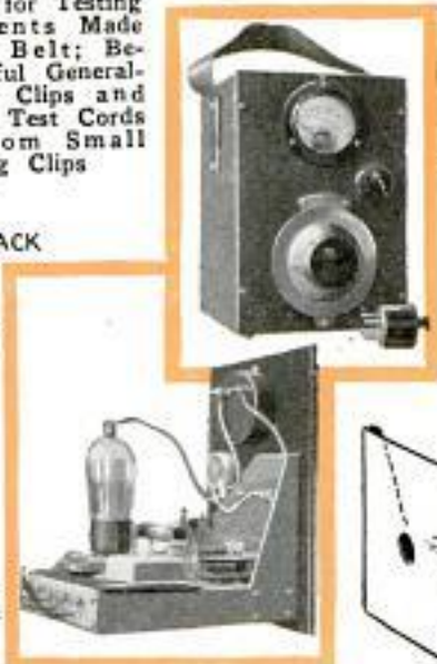
Above, Heavy-Duty Resistor That May Be Used as a Variable Load for Testing Batteries, Meters and Other Equipment; Below, Easily Made Shield and Chassis for Small Units
