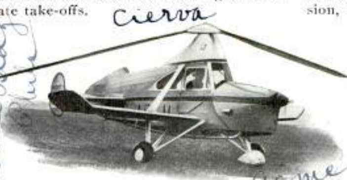
Autogyro That Offers Both Speed and Safety; It Cruises at 100 Miles an Hour and Has a 105-Horsepower Motor.
