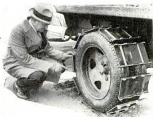
Steel Plates Attached to Truck Wheels to Give a Traction/Tread to Pneumatic Tires
