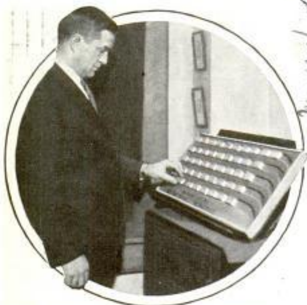
Block Board That Enables Terminal Manager to Switch Cars and Make Up Trains in Advance
