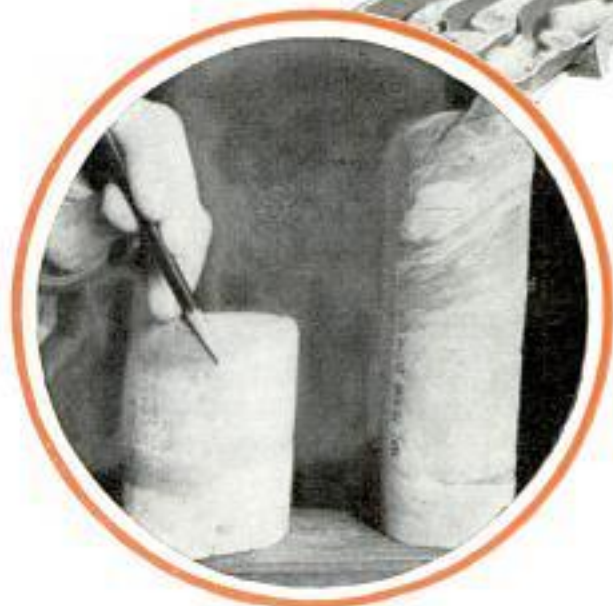
Core Samples from Wells Containing "Bugs"; Pencil Points to a Fault Shown in a Core
