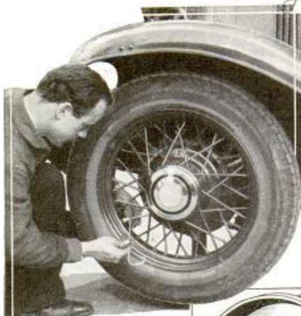
WIRE SOLDER WRAPPED AROUND SPOKE TO BALANCE WHEELS
