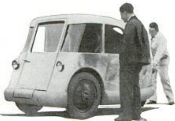
Powered with a Small Engine in the Rear. This Three-Wheeled Auto Attains High Speed
