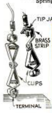
Right, Handy Carrying Strap for Testing Instruments Made from Old Belt; Below, Useful General-Purpose Clips and Jacks for Test Cords Made from Small Spring Clips
