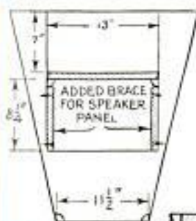
CROSS-SECTION VIEW LOOKING DOWN ON TOP SHOWS PANELS FITTED IN GROOVES
