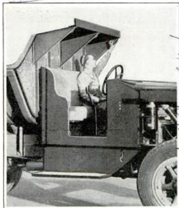
Steel Rock-Catching Shield Protects Driver
