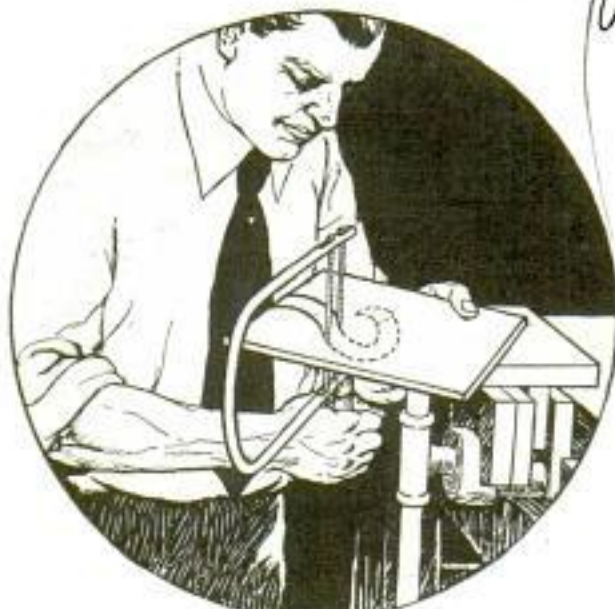
Coping Saw Equipped with Two Blades Assures Equidistant Spacing of Cuts When Sawing Scrolls
