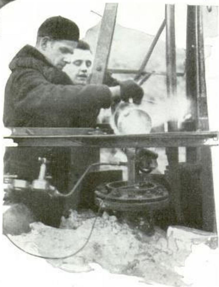
Above, Copper Lining of a Small Rocket Motor; Below, Pouring Liquid Oxygen into a Test-Stand Tank
