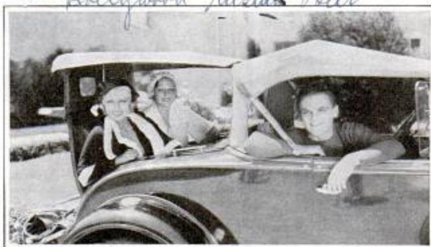
Collapsible Top for the Rumble Seat, Supported at Back by a Telescoping Standard So Top Can Be Raised as Passengers Enter or Leave
