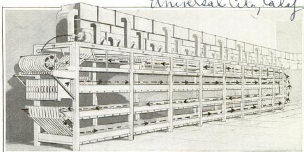
Continuous Movie-Film Developer That Will Develop Twelve Reels of Negative at a Time, Drying and Winding It Ready for Printing
