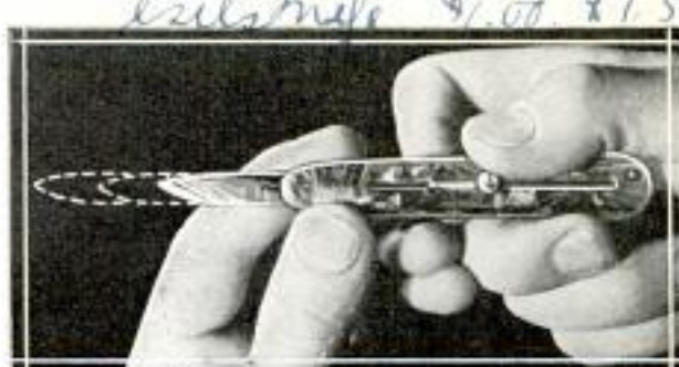
Pocketknife with an Extension Blade That Slides Out of Handle; the Blade Is Replaceable
