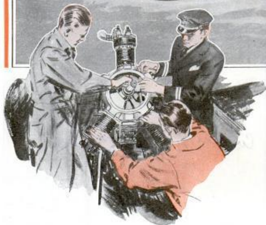
Class Being Taught Wing Alining, at Top, and Adjustment of Master Rod Bearing of Radial Engine, Below
