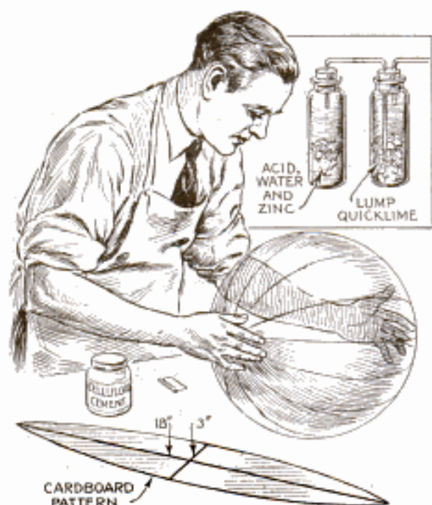
Toy Balloon Made of Cellophane Stays in Air Several Days and Travels Long Distances
