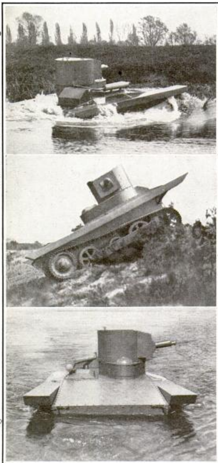
Views of Amphibian War Tank in Water and on Land; It Has a Land Speed of About Forty Miles an Hour
