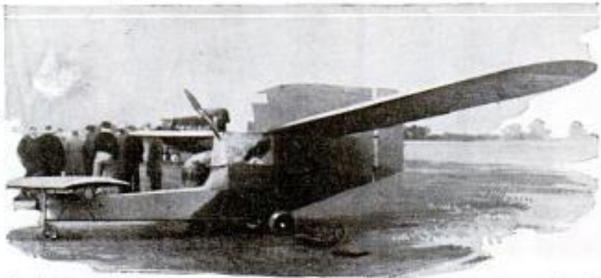
Small Plane Virtually without a Tail and with Its Elevator in Front; in the Air It Appears to Be Flying Backward
