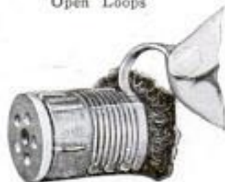
Coil-Spring Flour Sifter: When Handle Is Pressed, the Spring Is Extended, Letting Flour Enter through Open Loops
