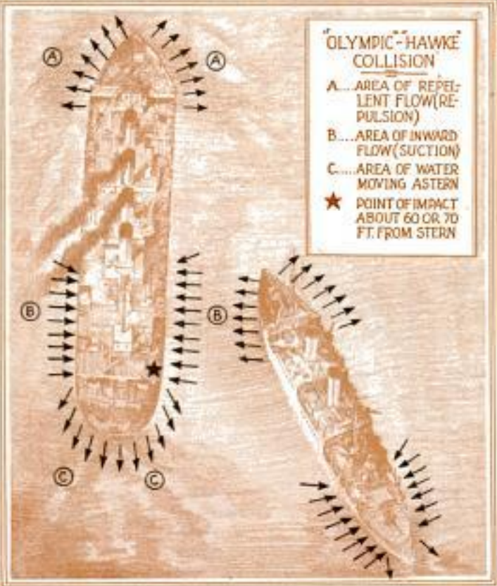
Above, Drydocking the "Majestic"; Below, Diagram Showing Forces Causing Collision of "Olympic" and "Hawke"
