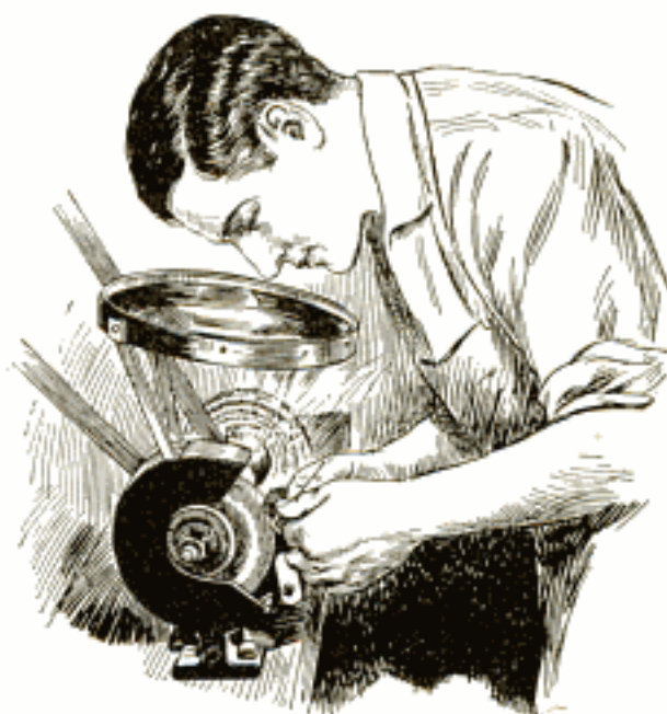
Glass Shield over Emery Wheel Allows Clear Vision without Getting Dust into the Eyes
