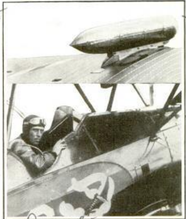
The Life Raft Is Incased in Streamlined Metal and Mounted on the Top Wing
