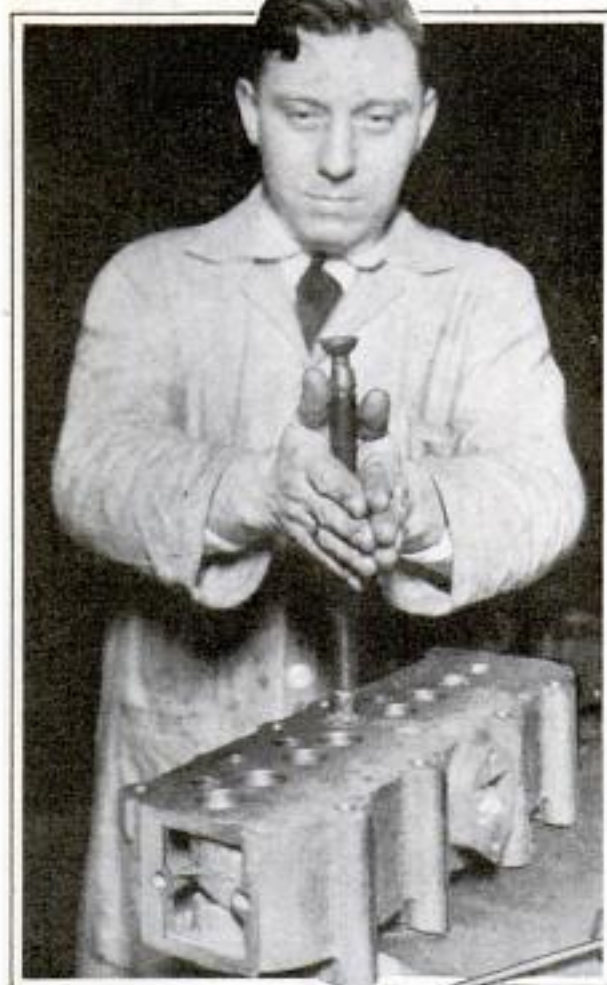
Valve Grinder with a Rubber-Tipped Vacuum Cup in Which the Abrasive Compound Is Placed
