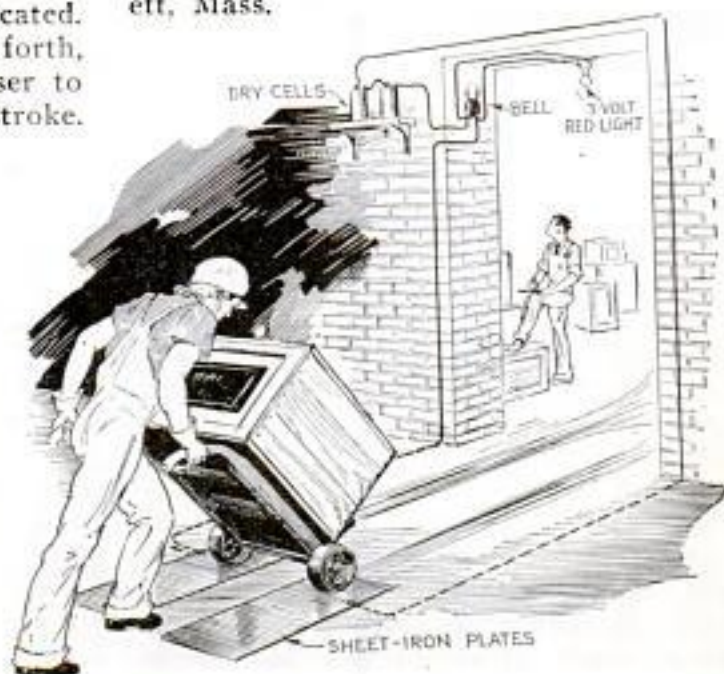
Trucks Passing over Metal Plates, Placed at Approach to Shop Door, Ring Signal Bell
