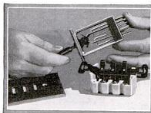
Anti-Capacity Switch for Table or Panel Mounting, Handy for Radio Experimenters and Service Men Making Comparative Tests
