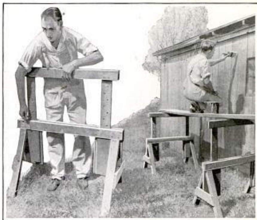
With a Couple of These Adjustable Horses, Scaffolding Can Be Quickly Raised to the Most Convenient Working Height
