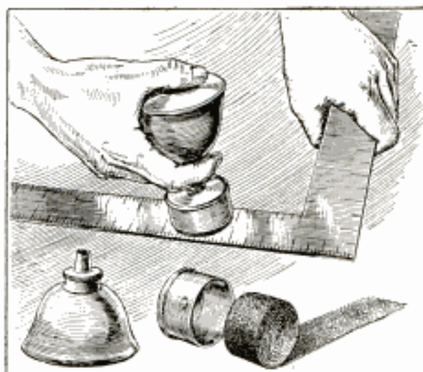
Can with Roll of Burlap Oils Tools without Waste of Lubricant
