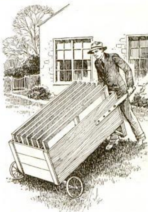
Box Fitted with Wheels and Handles Provides Safe Means for Moving and Storing Windows
