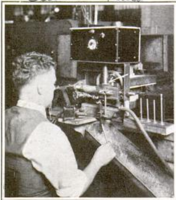
Placing Valve Tips in a Hardening Machine Which Is Controlled by an Electric Eye
