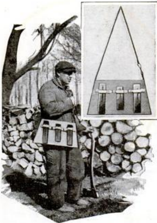
Holder Carries Steel Wedges Safely and Prevents Their Being Lost
