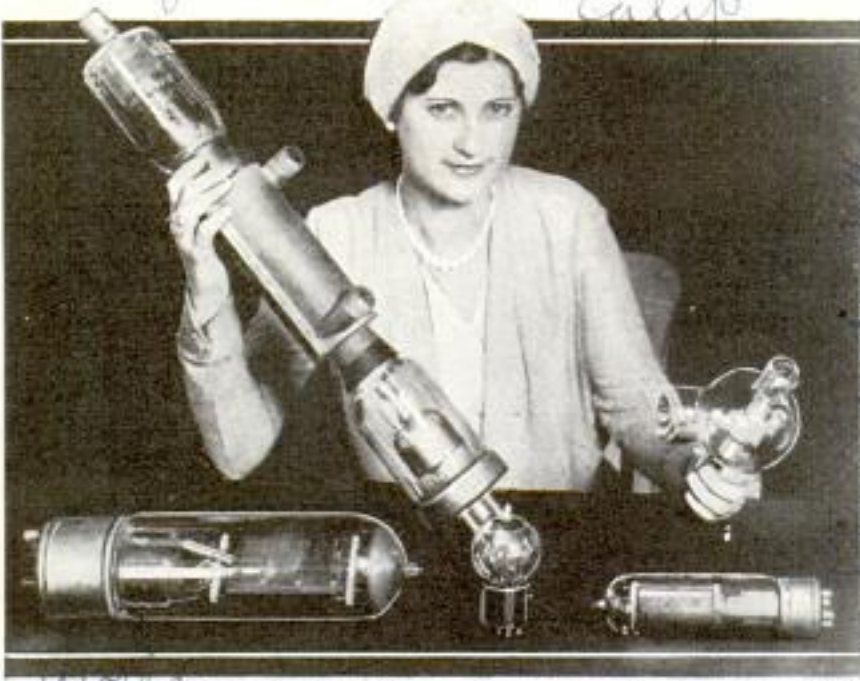
Giant Water-Cooled Tube That Bounces Waves from U. S. to Hawaii, in Right Hand; All the Tubes Are Used in One Sending Station
