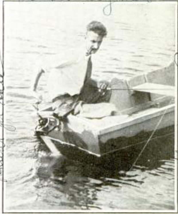
Oarless Rowboat with Propeller in Form of a Paddle Turned with a Crank
