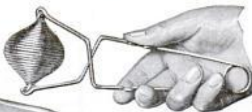
Coil-Spring Flour Sifter: When Handle Is Pressed, the Spring Is Extended, Letting Flour Enter through Open Loops
