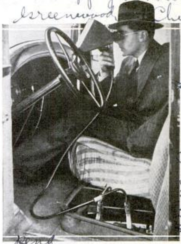
By Checking Battery with "X-Rayoscope" You Can Tell Quickly the Condition of Its Individual Cells
