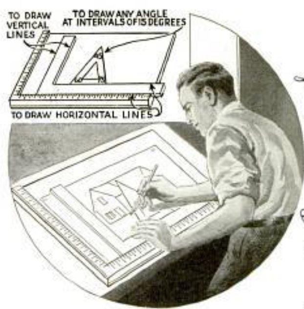
Drafting Equipment Requiring No T-Square or Tacks and Has Scale Built In
