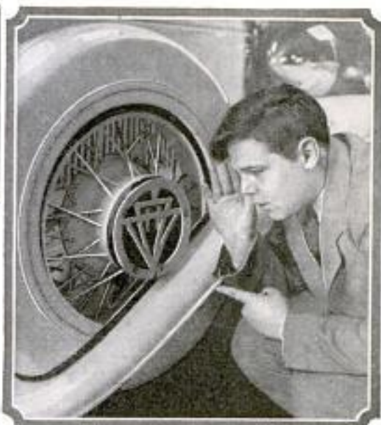
Above, Radio Speaker for Outdoor Advertising Installed in Hub Frame of Spare Wheel; the Homemade Grille Is Backed with Wire Mesh; Left, Using Hand Drill for Removing Prongs from Tube Bases When Shell Is Required for Choke-Coil Form; Base Is Held for Drilling as Shown
