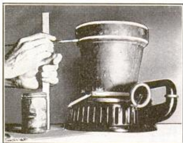
Stripes Quickly Painted on Small Circular Articles by Rotating Them with a Phonograph
