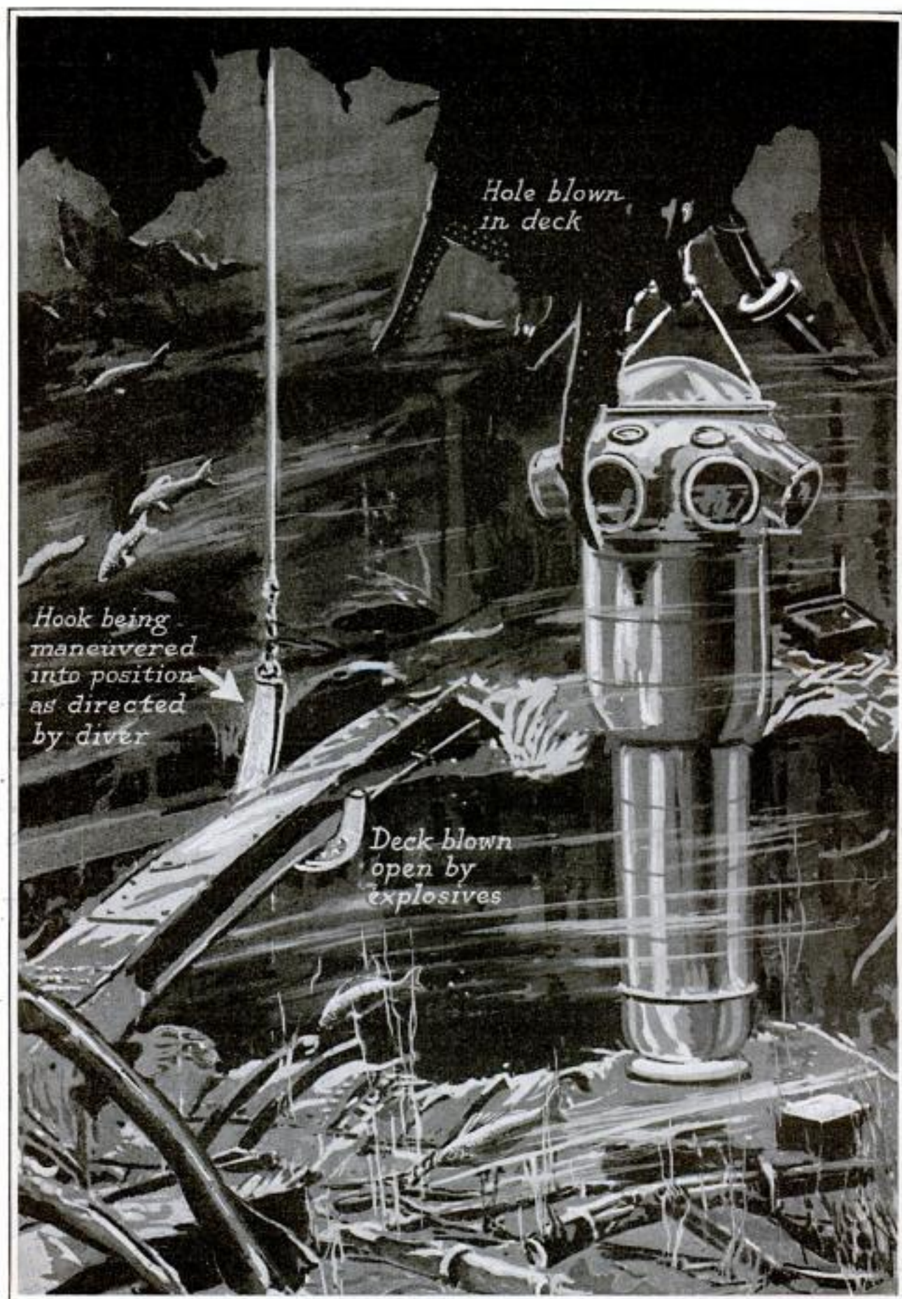
Steel Shell Inside of Which Is a Diver Who Serves as the Eyes for the Salvage Work; the Diver Is Connected by Telephone to the Salvage Ship Nearly 400 Feet Above
