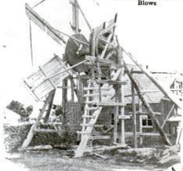
Crude Windmill That Is Used for Sawing Wood When the Wind Blows
