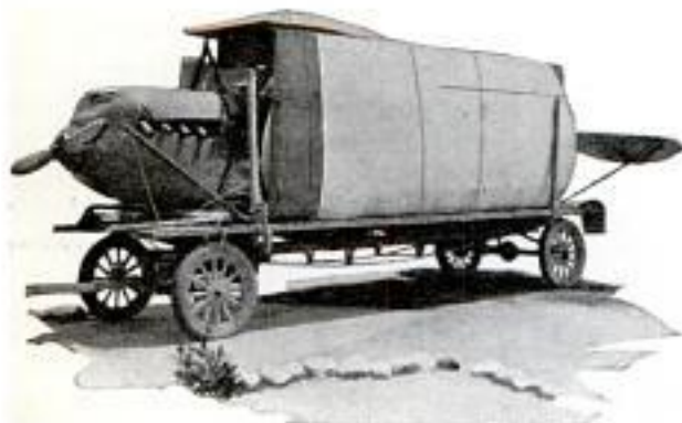
Two Auto Chassis Welded Together Form Trailer for Transporting Wrecked and Knock-Down Airplanes
