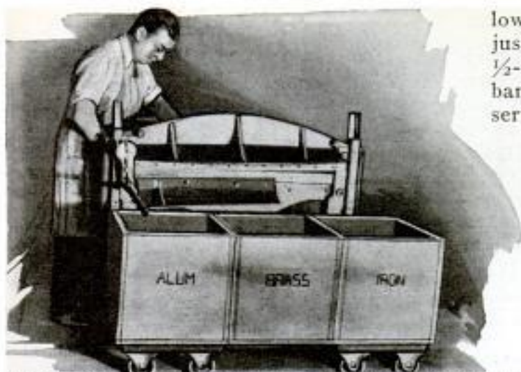
Boxes on Small Truck Placed in Front of Cutting Machine Provide Individual Receptacles for Waste Metal
