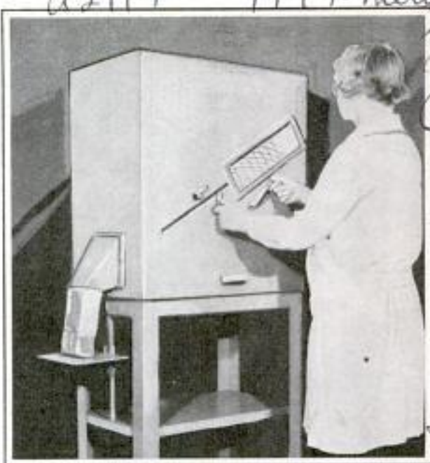
Automatic Scale Which Fills a Bag, Weighs Its Contents and Cuts Off Supply When Full
