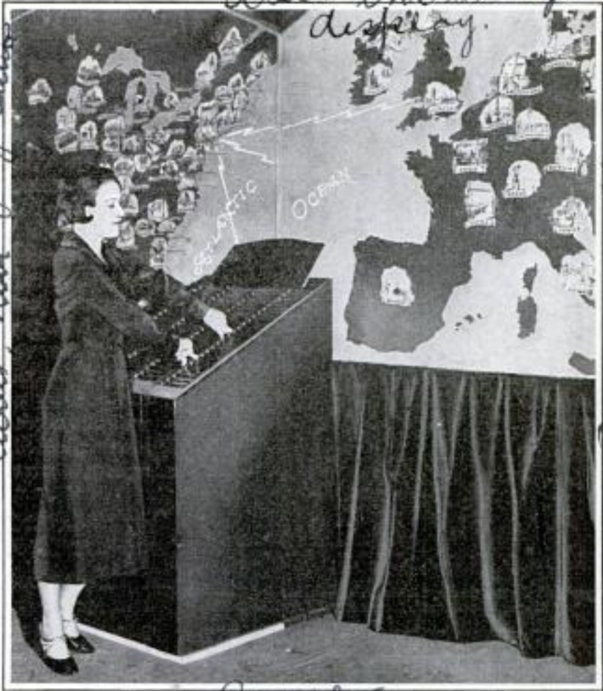
Telephone Map of World, and Control Cabinet Which Gives Phone Rates between Any Two Points When Proper Buttons Are Pressed
