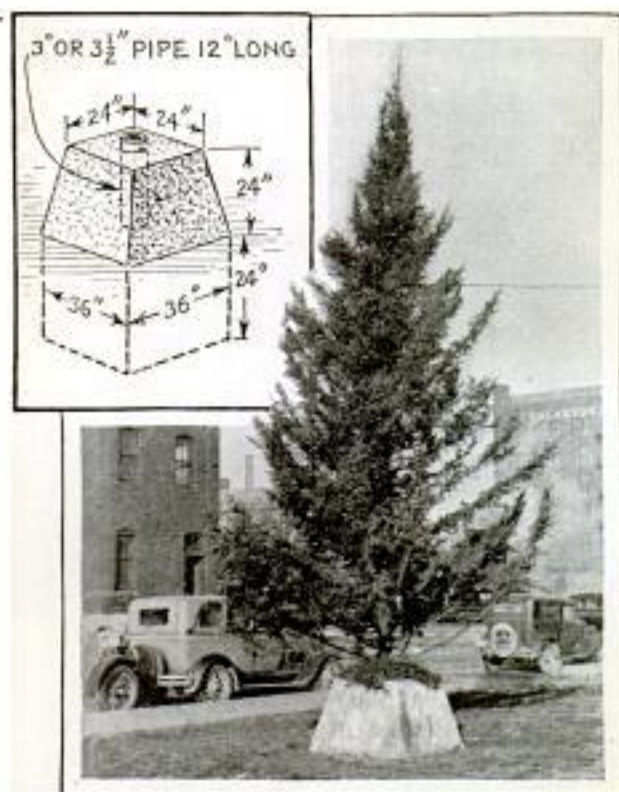
Concrete Base for Christmas Tree, Flagpole or Sign Has Neat Appearance on Lawn
