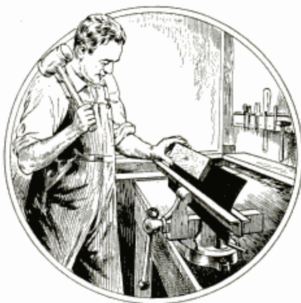
Sheet Metal Clamped in Vise Is Bent by Means of Wooden Block and Mallet
