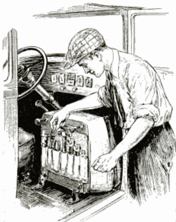
This Kit, Arranged under Front Seat of Coach, Makes Tools Readily Accessible
