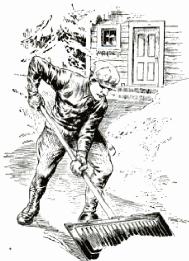
Snow Shovel Made by Nailing Part of Auto Hood to a Wooden Handle
