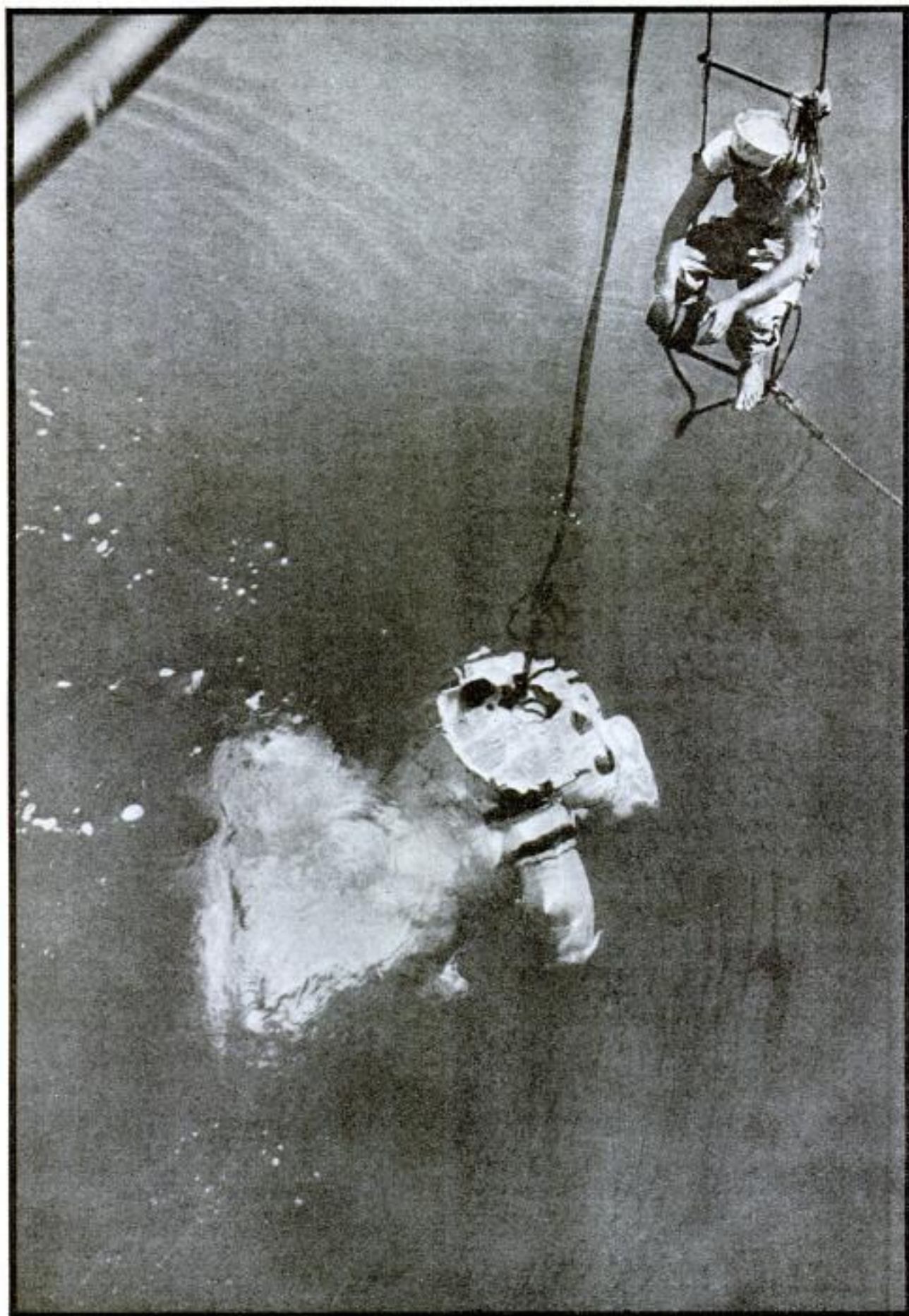
Diver Incased in Steel Shell Rising after Directing Salvage Work to Recover over $5,000,000 in Gold from the "Egypt." Lying in 396 Feet of Water off Coast of France
