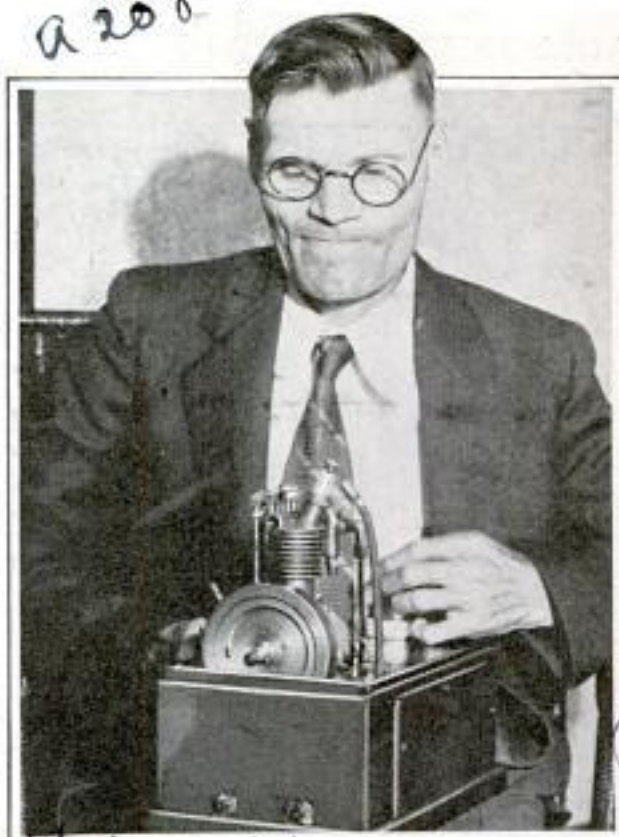
Little Gas Engine That Weighs Three and One-Half Pounds and Develops One-Twentieth Horsepower
