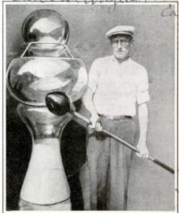
Five-Foot Goldfish Bowl Made from 100 Pounds of Glass and Pipe with Which It Was Blown
