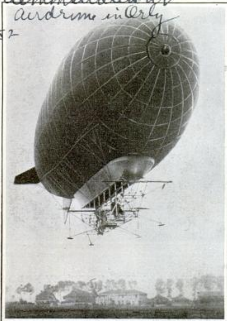
Helicopter, Controlled from Pilot's Seat, Enables This Dirigible to Fly Straight Up
