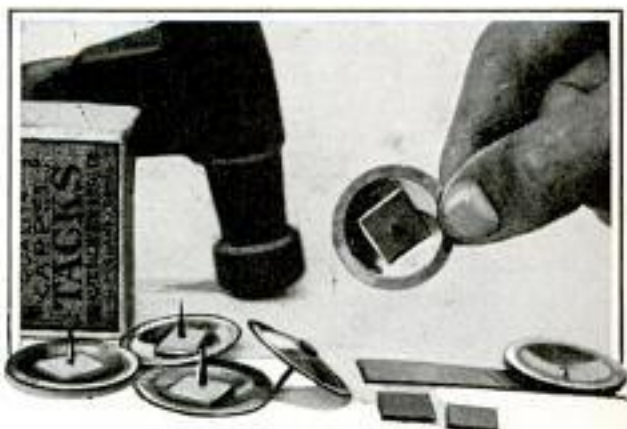
Small Squares of Rubber Hold Nails and Roofing Washers Together Until Driven into Place
