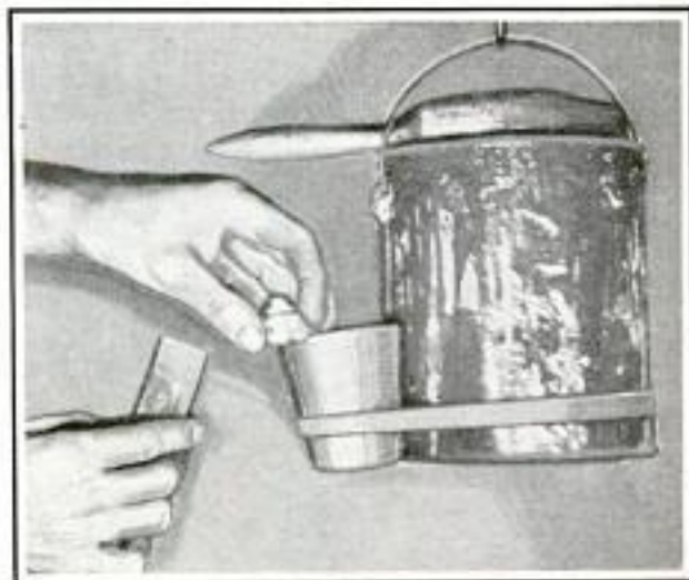
Small Cup Clamped to Paint Bucket with Rubber Band Holds Supply of Putty
