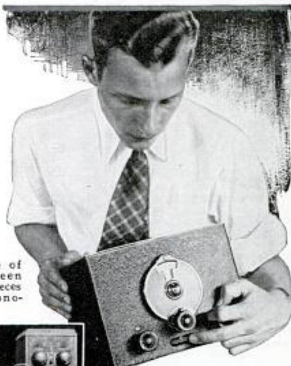
Wheel Acts as Volume Control and Audibility Meter; Left, Filter in Series with Detector Plate Supply Prevents Hum
