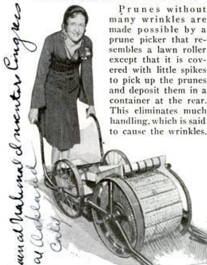
Prune Picker Like Lawn Roller Which Spears the Fruit on Prongs as It Moves
