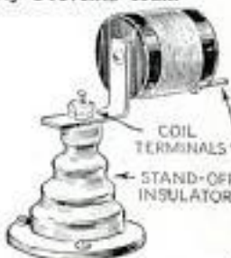
Above, R. F. Choke Coil for Amateur Transmitter May Be Wound on an Old Tube Base and Mounted as Shown
