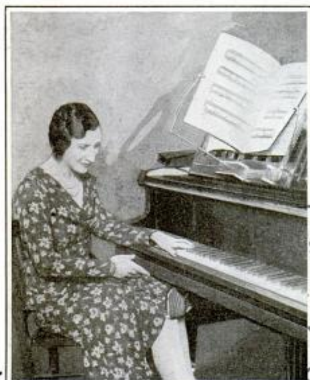
Music-Page Turner for the Piano Which Is Operated by Pressing a Lever with the Knee
