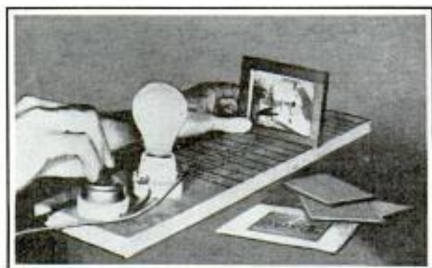
Ruled Board Fitted with Lamp Aids in Getting Photographic Prints Correctly Exposed
