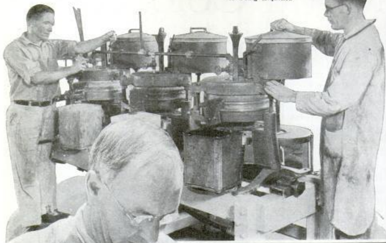
Machine That Grinds Pure Metals to Powder, Below, and Examining Complex Ore Before It Is Being Liquefied
