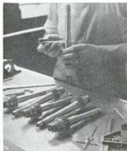
Wright inspector checking the camshaft idler shaft of a Curtiss-Wright Conquest engine with a Starrett Micrometer No. 2. The dimension is 1.0605 plus or minus .0005.
