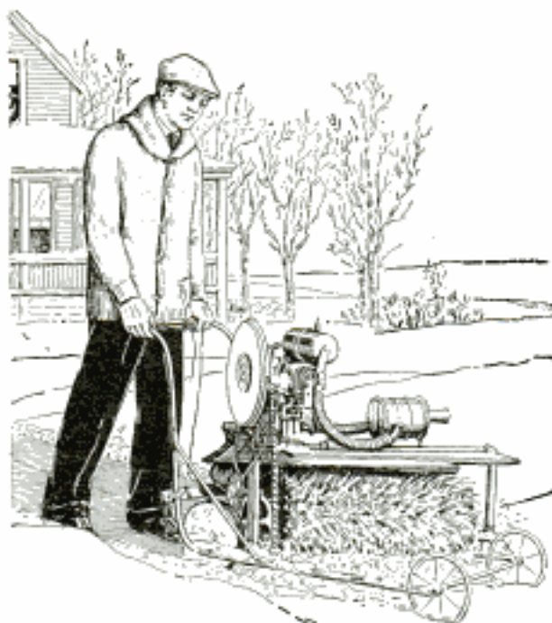
Efficient Homemade Snow Sweeper Made from a Discarded Rotary Brush and a Two-Cylinder Engine
