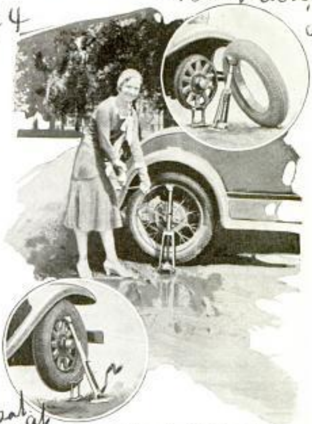
Rim Jack for Auto That Can Be Operated from a Standing Position without Soiling Hands
