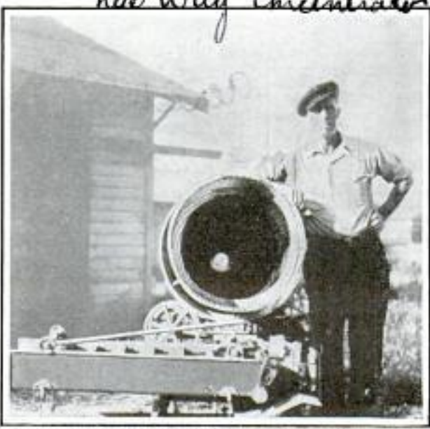
Portable Gold-Washing Machine That Can Be Operated without Water if Material is Dry
