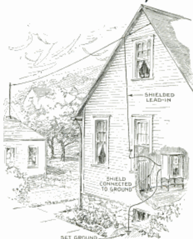
Antenna Installation with Shielded Lead-In for Eliminating Interference
