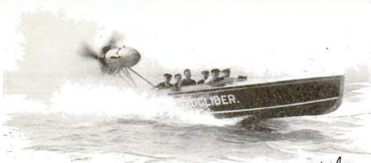
High-Speed Hydroglider, a Motorboat with an Air Propeller Mounted at the Rear; the Craft Travels Better Than Forty Miles an Hour and Can Be Used in Very Shallow Water
