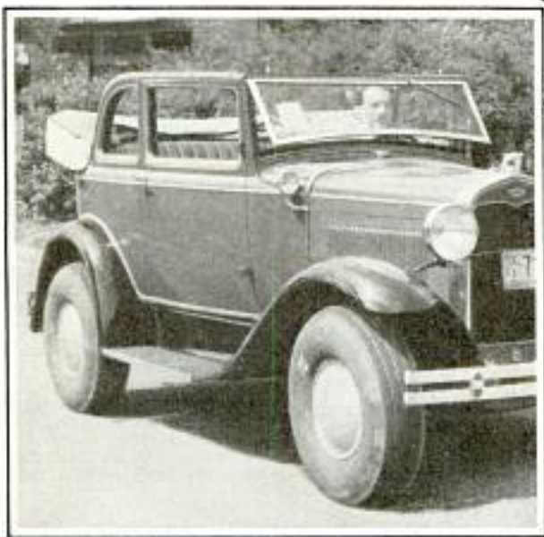
Small Car Equipped with Doughnut Tires Similar to Those Used on Airplanes
