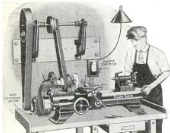
8" x 24" Junior Back Geared Screw Cutting Precision Bench Lathe with Simplex Countershaft instead of Tight and Loose Pulley Countershaft with Plain Rest. $100.00
