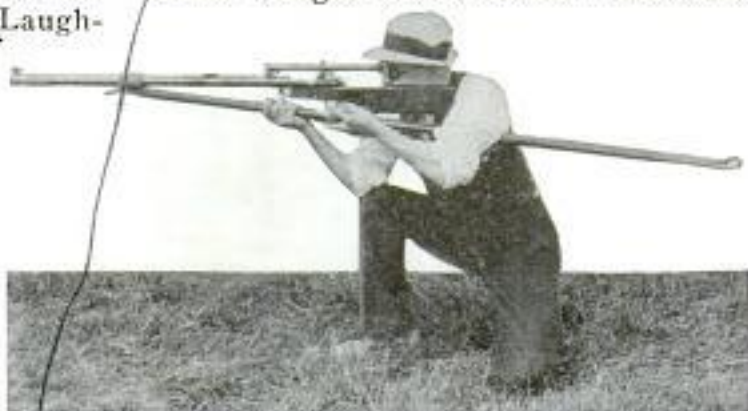
Counterbalance for a Target Rifle to Improve Marksman's Aim; It is Made from an Automobile Radius Rod
