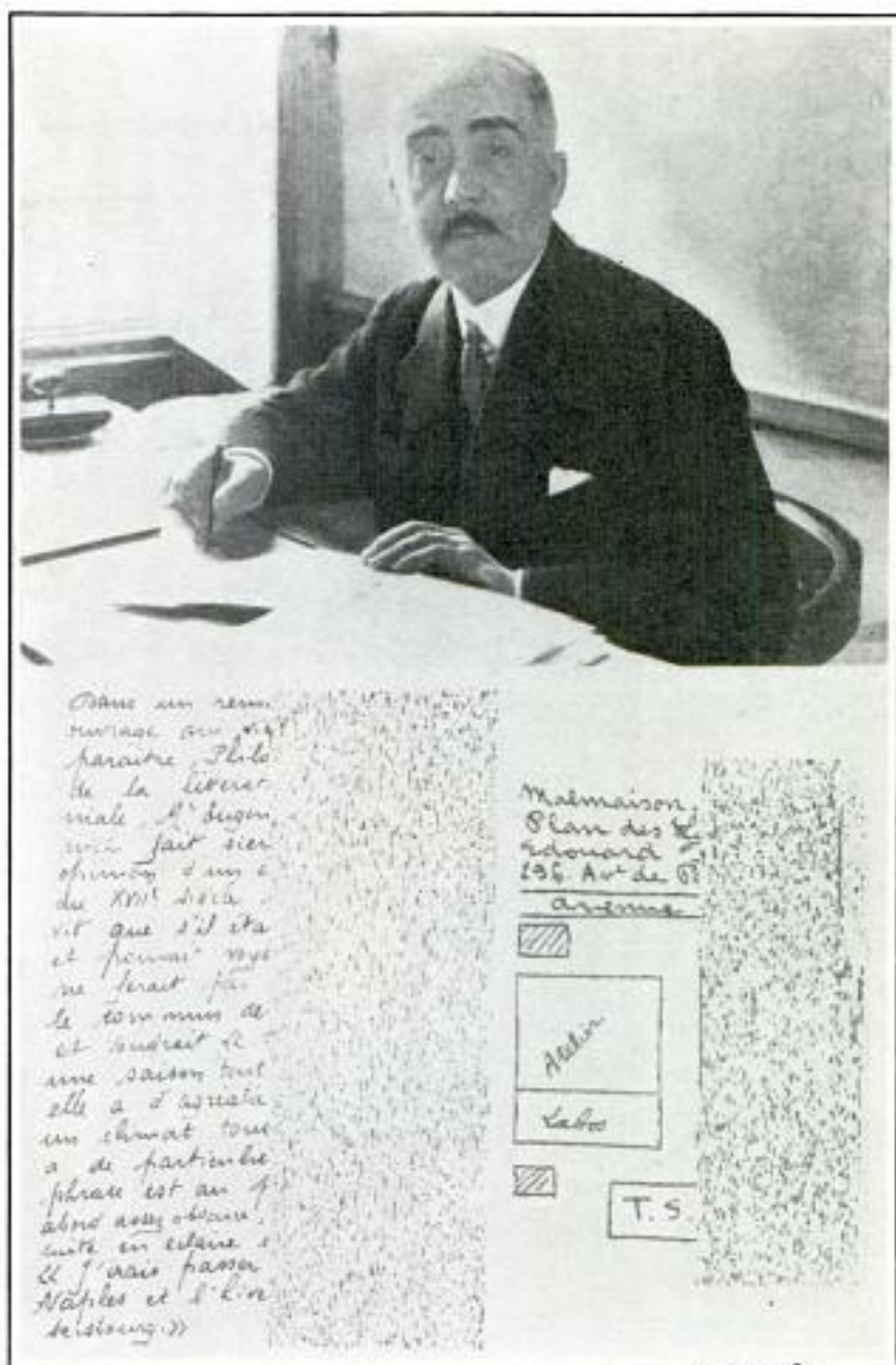
Examples of Documents as They Appear on Keyed Receiver, Left, and on Any Other Set at the Right; Inventor at Top
