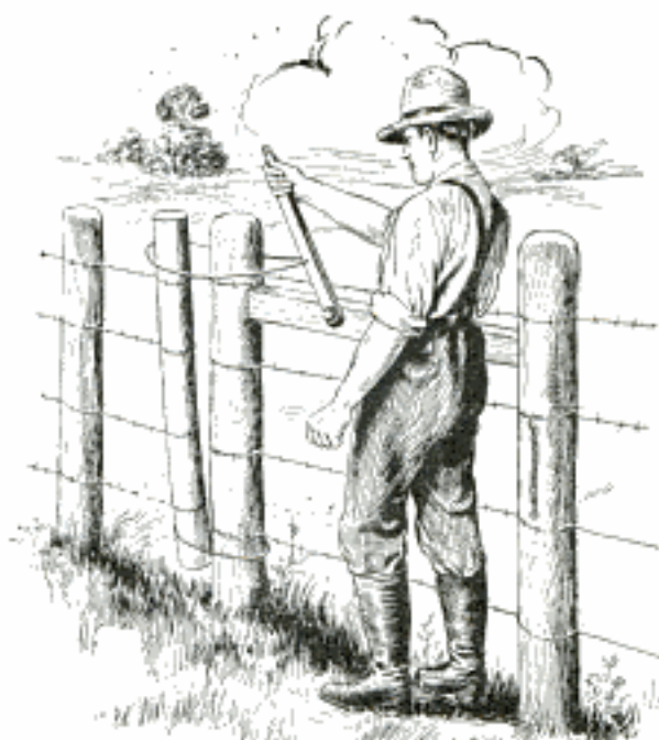
Lever Latch on Wire Gate Cannot Be Opened by Stock and Is Easily Operated
