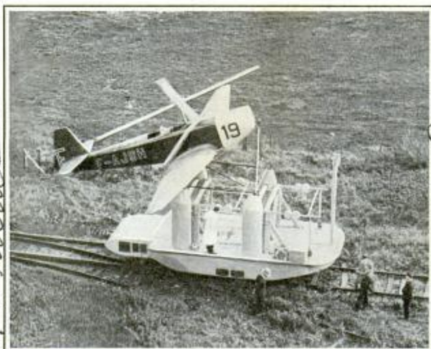
New Type of Plane Being Tested on a Self-Propelled Rail Car; the Car Travels at High Speed and the Plane Imitates Real Flight
