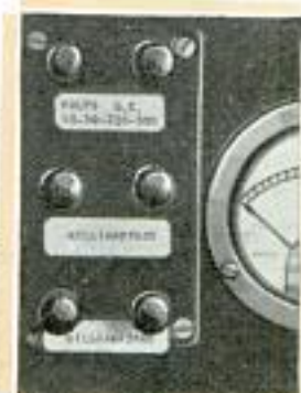
Typed Labels, Glued to Panel, Indicate Tester Connections
