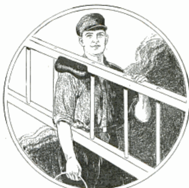
Making It Easier to Carry a Heavy Ladder by Providing a Comfortable Shoulder Pad
