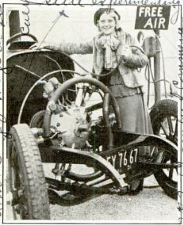
Filling Up the Air Tank of Compressed-Air Auto; Note the Small Radial Engine
