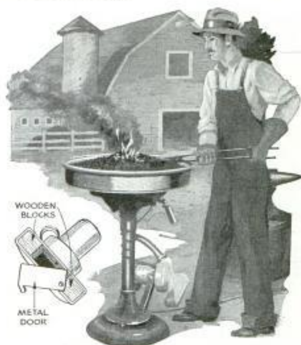
Improved Electric-Driven Forge for the Farm or Workshop Is Made from Scrap Parts
