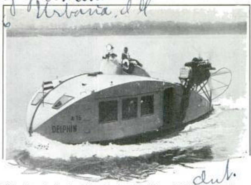
Glider Boat Equipped with an Airplane Propeller and Driven by 400-Horsepower Motor; It Makes a Speed of Fifty Miles an Hour
