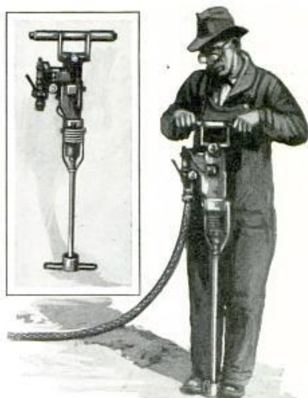
Guide Aids in Starting Air Drill on a Smooth Surface without Slipping or Jumping
