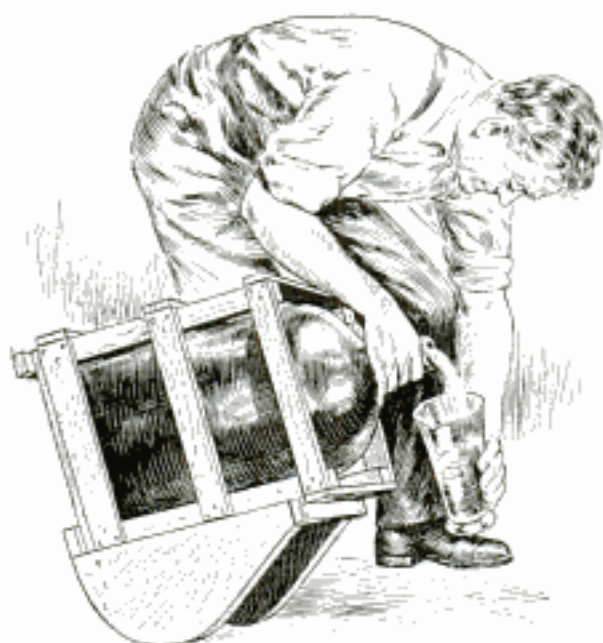
Carboys Fitted with Rockers Can Easily Be Tipped to Fill Small Containers
