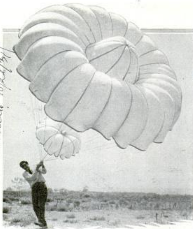
Bulbous Parachute Which Opens in the First Ten Feet of Descent; Small Chute Acts as a Shock Absorber
