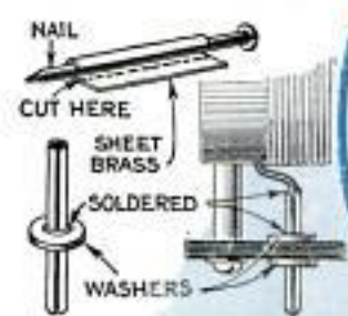
Above, Tips for Plug-In Coils; Right, Well Soldered Connections Important in Multi-Range Voltmeter Assembly
