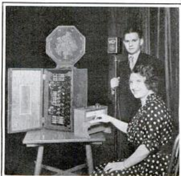
Radio Organ Controlled by a Tiny Piano, the Tones Being Produced by Thyatron Tubes
