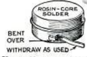
Handy Method for Holding Flat Strip Solder during the Soldering Operation
