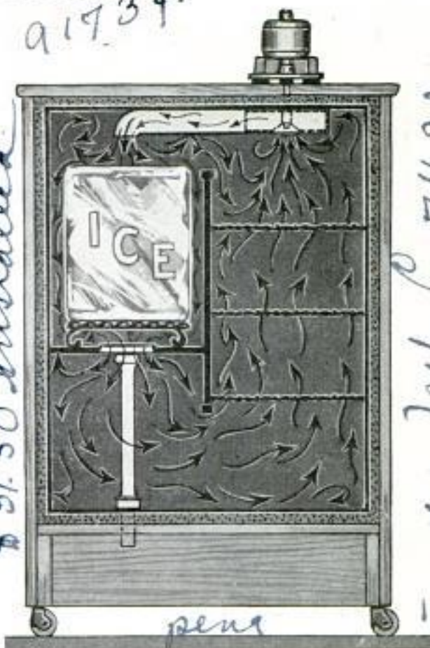
Air Fanned over Ice and Circulated through the Food Chamber Keeps the Ice Box Several Degrees Cooler
