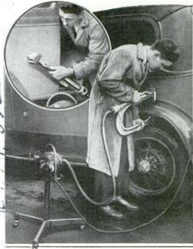
Electric Hammer That Takes Dents Out of Auto Fenders at Rate of 1,500 Blows a Minute
