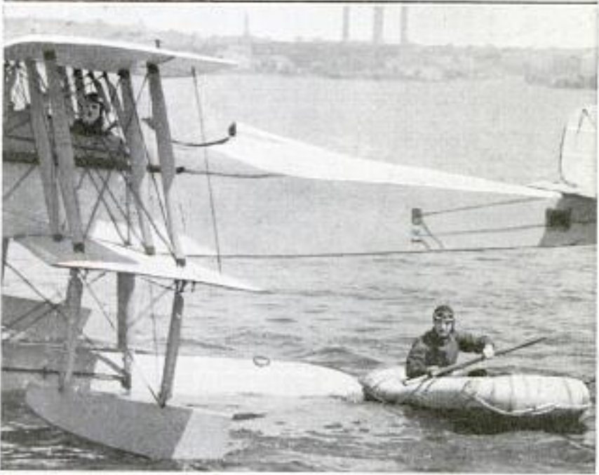
The Three Views from Top to Bottom Show How a Rubber Lifeboat Is Unfolded from Its Storage Space in the Naval Seaplane, Inflated with Air and Launched
