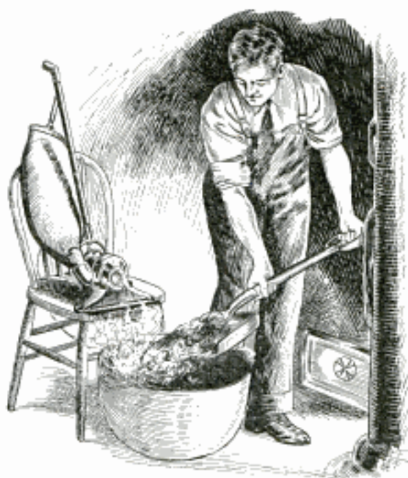
Dusty Task of Removing Ashes from Furnace Made Less Dusty with Aid of Vacuum Cleaner
