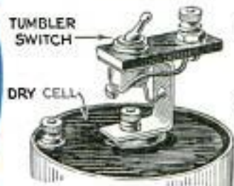
General Utility Switch of Tumbler Type Mounted Directly on Dry Cell
