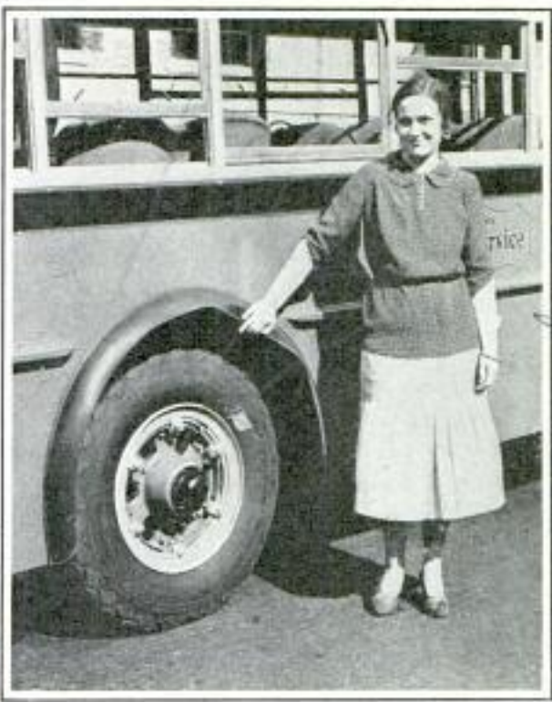
All Jokes about Rubber Fenders Are Stopped by This Bus Equipped with Semi-Flexible Mudguards
