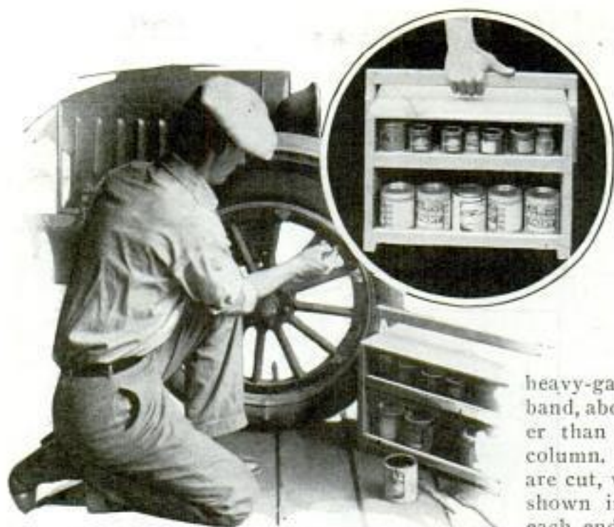
Painters Who Have a Number of Small Jobs Requiring Different Paints Will Find This Carrying Case Handy
