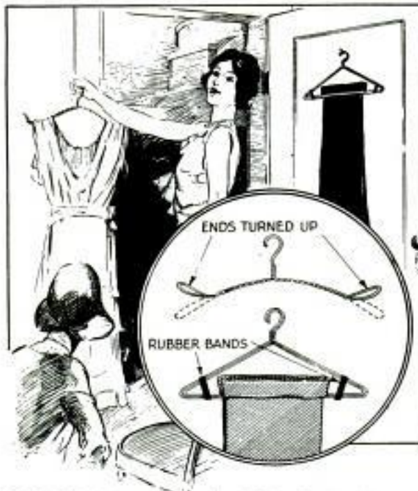
Simple Methods of Improving Wire Clothes Hangers for Holding Trousers and Sleeveless Dresses
