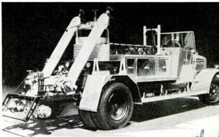
Fire Engine That Extinguishes Flames by Spraying Powder on Them; the Powder, Unlike Water or Other Liquids, Does No Damage to Goods
