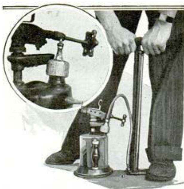
Blowtorch Tank Fitted with Valve Stem Quickly Filled with Tire Pump
