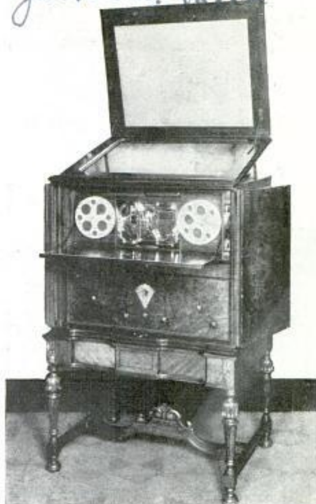
Home Talkie and Radio Installation Showing Film Reels and Screen in Position
