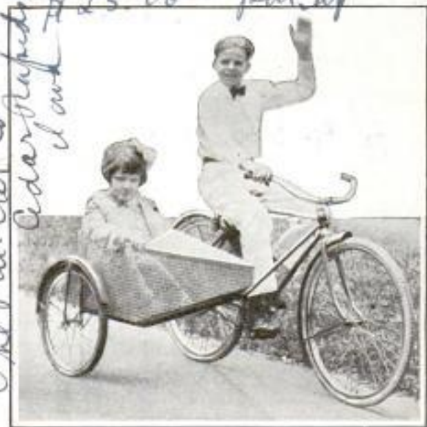
Bicycle with Light but Sturdy Sidecar for Carrying Extra Passenger or Luggage
