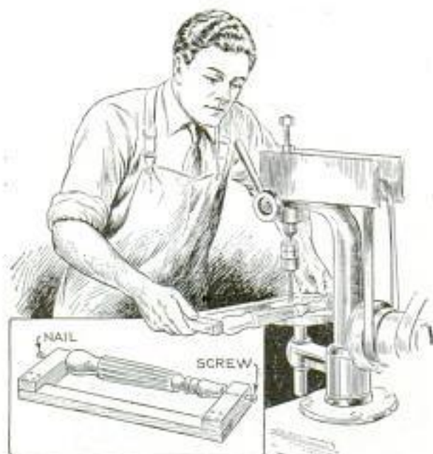
Fluting Work Done on Drill Press by Means of This Jig and Homemade Shaper Knife
