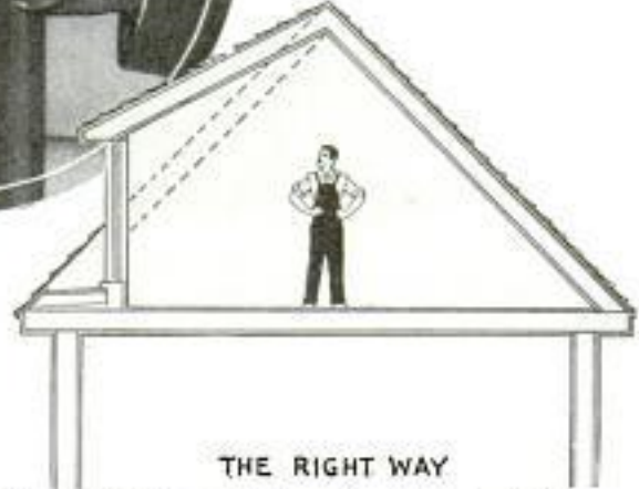
Example of Poor Construction to Save Labor; the Joints Should Be Mitered, Above; the Right and Wrong Way to Raise the Roof to Add a Room in the Attic
