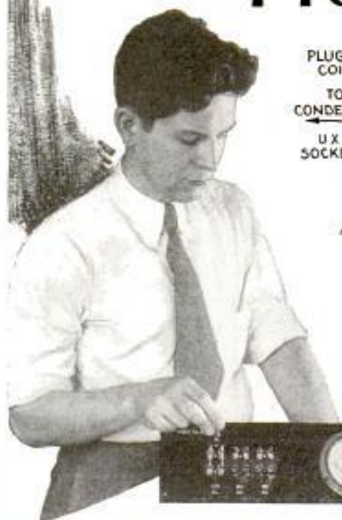
Small Double-Pole-Single-Throw Switches Mounted on Transmitter Panel to Shift Multi-Range Voltmeter for Different Circuit Readings
