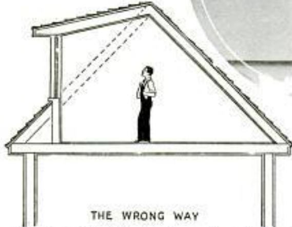
Example of Poor Construction to Save Labor; the Joints Should Be Mitered, Above; the Right and Wrong Way to Raise the Roof to Add a Room in the Attic
