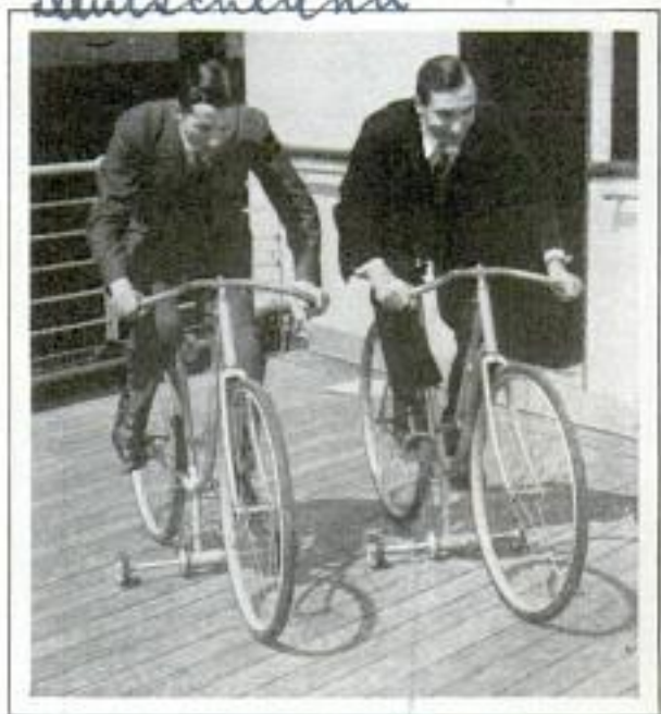
Courtesy Hamburg American Line Bicycles for Use on Shipboard; the Auxiliary Wheels Slow Down Speed of the Vehicles
