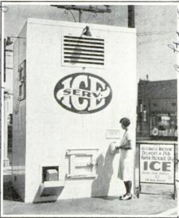
Coin-in-the-Slot Machine That Vends Cube Ice in Packages of Twenty-Five Pounds
