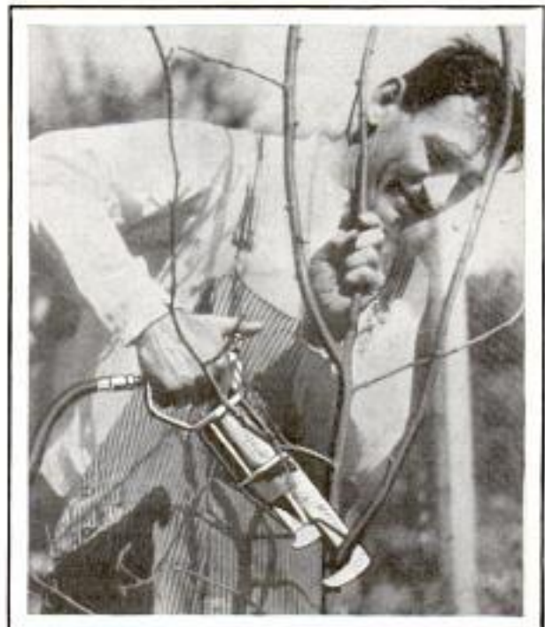
Faster Pruning Is Possible with This Compressed-Air Knife; the Pruner Does the Work of Thirty Men
