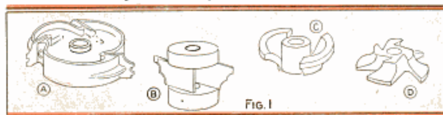
Various Types of Cutters for Small Shapers Permit an Infinite Variety of Molding Shapes
