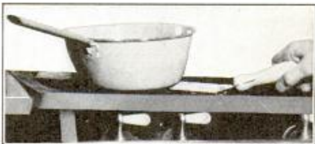
Cooking Utensils Can Be Tipped and Held in Position with This Angle-Iron Tilter
