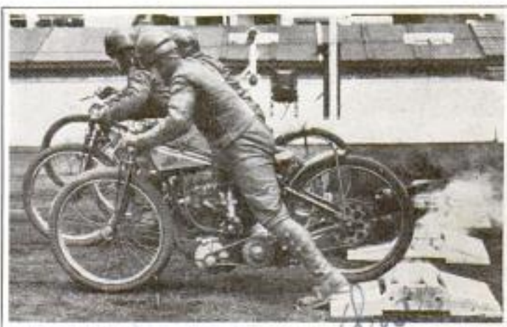
Rollers under Rear Wheels Used as Automatic Starters to Enable Motorcycle Racers to Get Away Together
