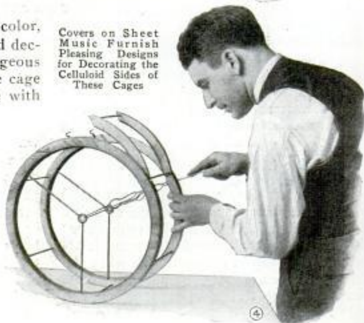
Two Wooden Auto Steering Wheels Make a Sturdy Frame on Which the Wire Bars Can Be Quickly Assembled
