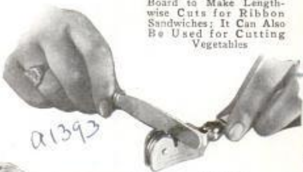
Above, Knife Sharpener That Puts Edge on Blade as It Is Drawn through the Slot
