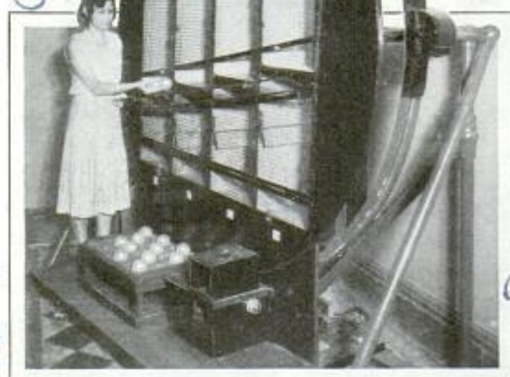
"Torture Wheel" through Which a Percentage of Each Type of Bulbs Made Must Pass Unscathed
