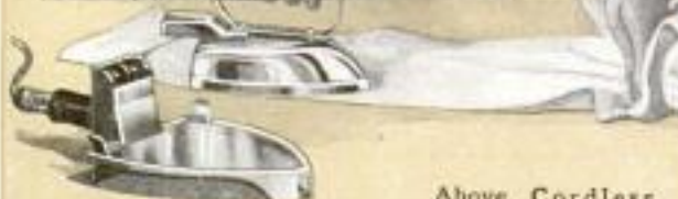
Above, Cordless Electric Flatiron That Allows More Freedom in Operation; the Cord Is Attached to the Stand Instead of the Iron, and the Latter Is Heated as It Rests on the Stand
