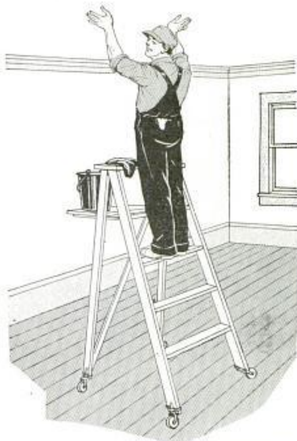
Equipped with Casters, This Stepladder Can Be Moved About without Getting Off
