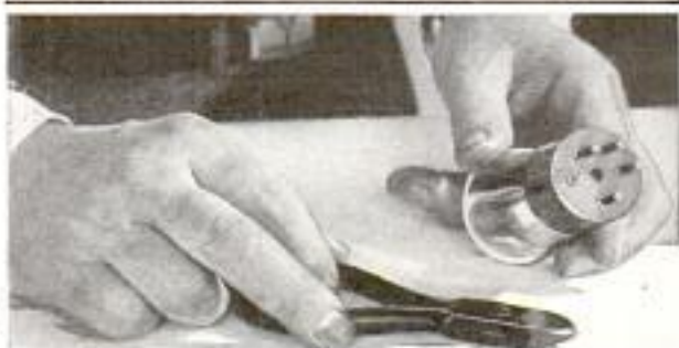
Cathode Prong Clipped from 227 for Neutralizing, for 226-Clip Filament Prong
