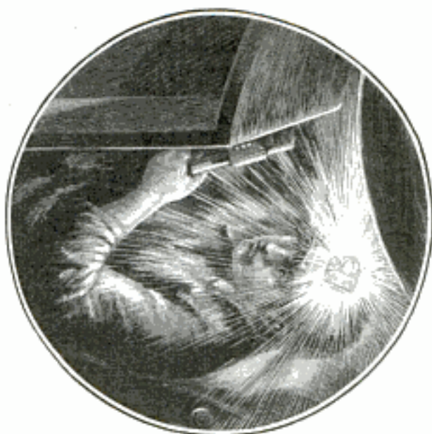
Light on Auto Mechanic's Cap Throws Light Where Needed and Leaves Both Hands Free
