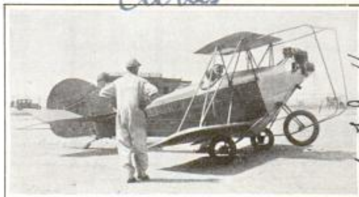
Plane with Stubby Wings and a Small Motor for Training Students; Note Safety Wheel in Front
