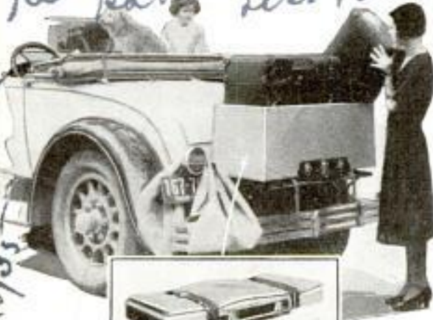
Collapsible Fabric Trunk That Fits Any Luggage Rack or Rests on the Auto Running Board
