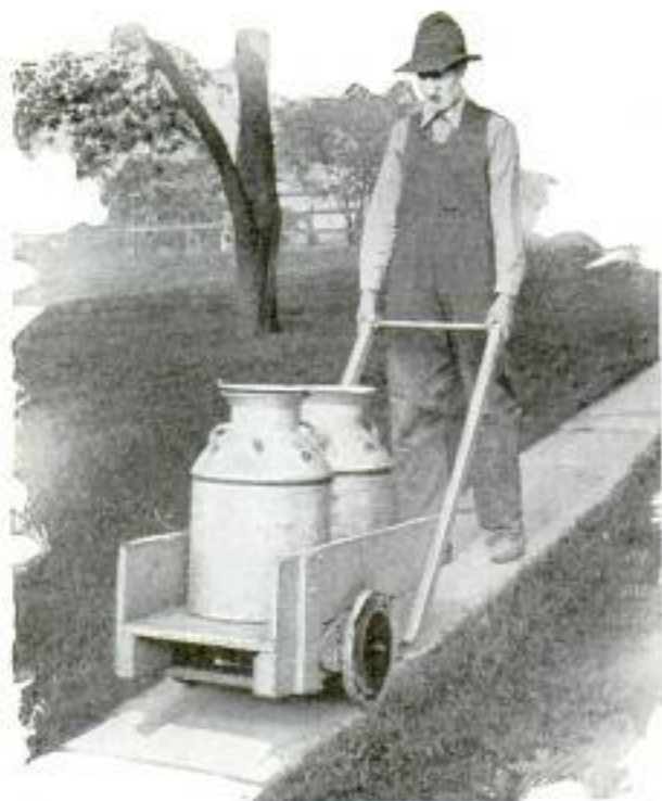
Old Lawnmower Chassis Fitted with Wooden Body Makes Handy Cart for Milk Cans
