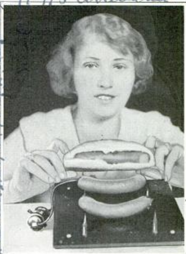
Cooking of "Hot Dogs" Is Easy with This Equipment Which Sends Electricity through the Meat
