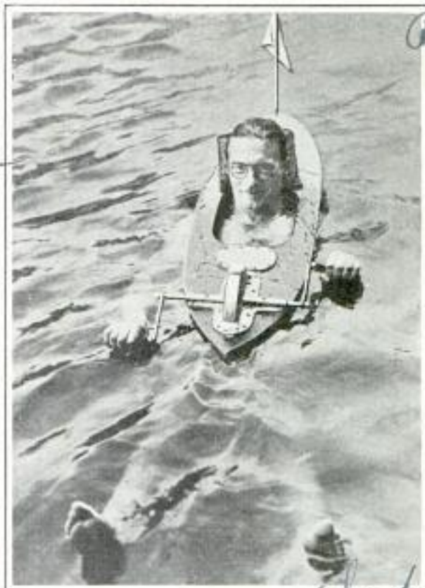
Propellers Worked by Hand Push This Swimmer Backward or Forward; Note How "Boat" Is Worn
