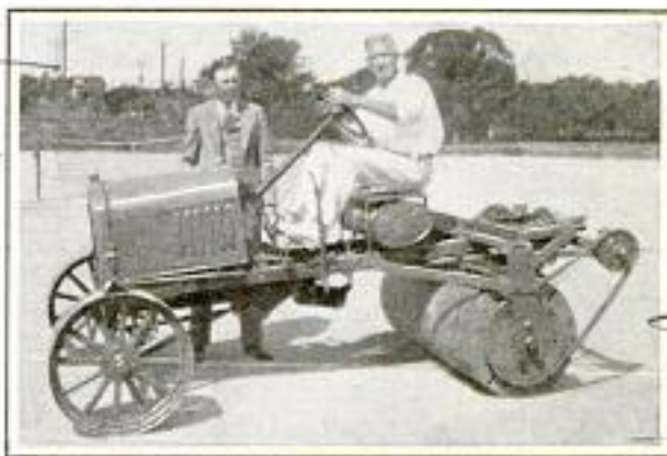
Tennis-Court Roller Made from Parts Found in Auto Junkyard; It Does Work of Five Men
