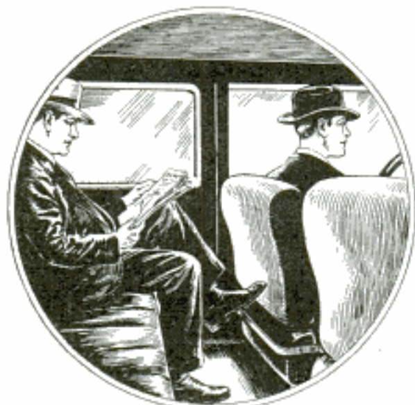
Length of Pipe Forms Comfortable Footrest and Prevents Passengers from Soiling Front Seat
