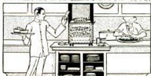
Automatic Elevator Rises from Kitchen to Table with Food Ordered by Dropping Card into Slot
