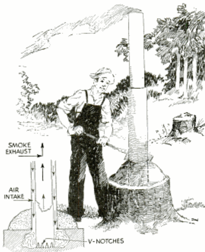
Stumps Are Easily Burned Out with Two Pipes Arranged to Furnish Sufficient Draft to Keep the Fire Alive
