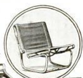
Auto Seat of Flexible Steel Tubing, Bent to Resemble Chair and Covered with Cloth or Leather
