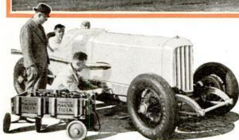
Thirty-Thousand-Mile Test Run of Studebaker Cars. Above; Below, Cranking the Cummins Diesel Car with Batteries on Service Wagon
