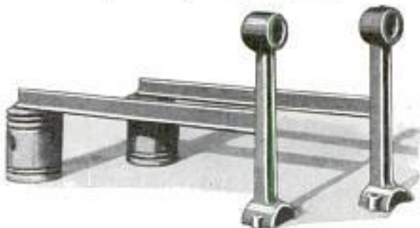
Serviceable Andirons Can Be Made from Discarded Pistons, Connecting Rods and Angle Iron
