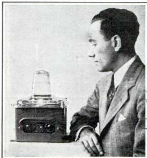
Photo-Electric Relay, Which Turns on Office Lights as Darkness Approaches, Saving the Eyes of Workers
