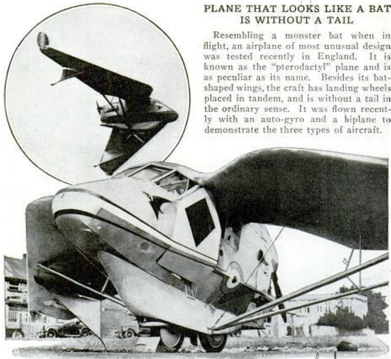
The British Pterodactyl Plane, So Named Because of Its Resemblance to a Prehistoric Monster, the Wings of Which Form Rudder and Elevator Surfaces
