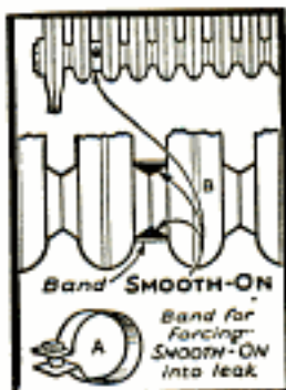
Leak at radiator joint stopped with Smooth-On
