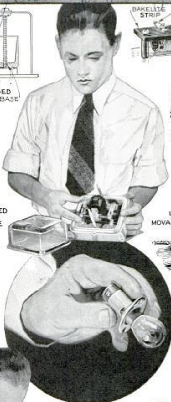
Below, Transmitter-Filament Supply Units That Operate on Either 110 or 220-Volt a.c. Lines
