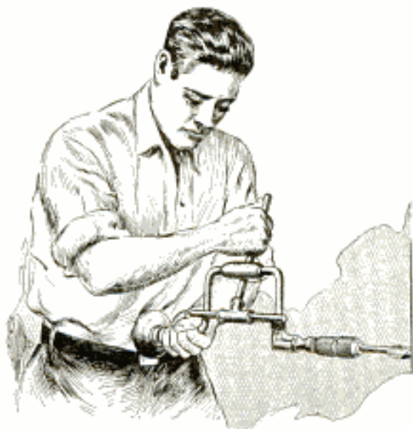
Leverage of Brace Increased by Using Extension Handle When Drilling in Hardwood with Large Auger
