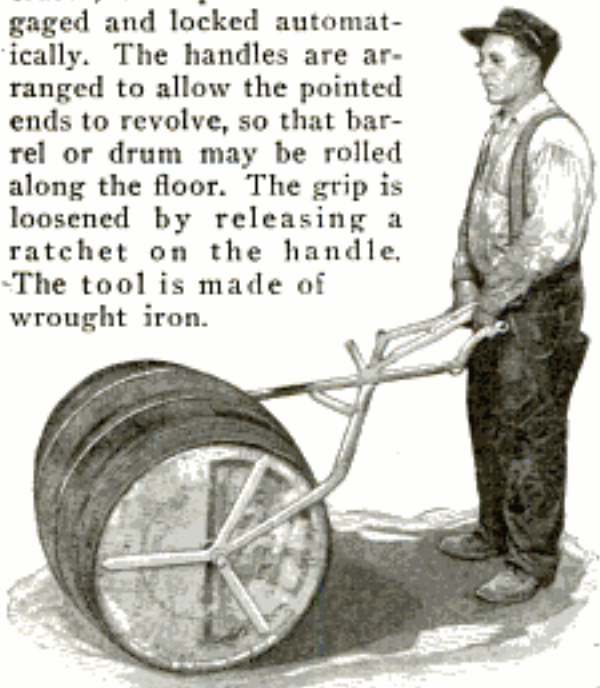
Barrel Handling Is Made a Simple Matter with the Speedy New Tool Shown Here
