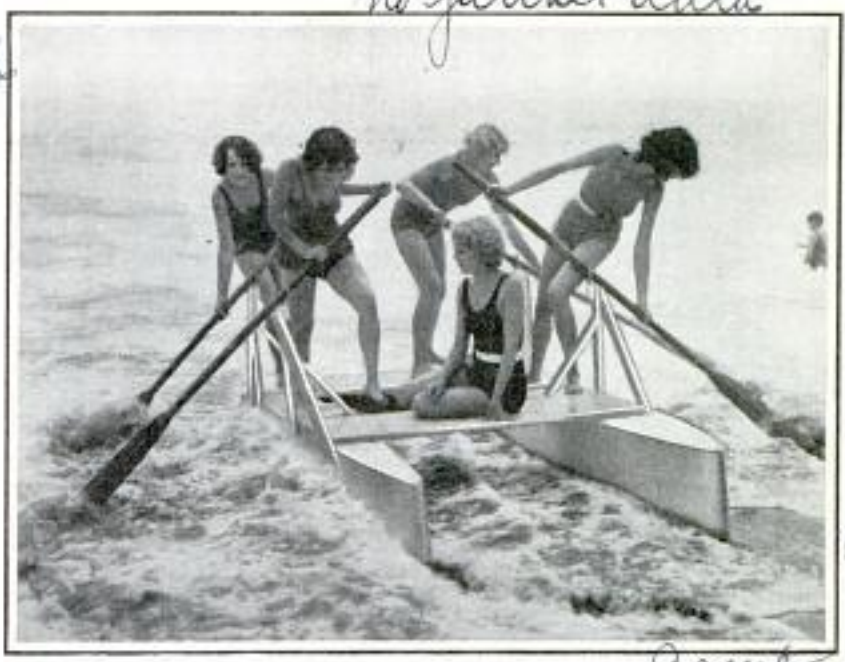
Riding the Surf on a Catamaran, a Raft Set on Twin Pontoons with Waist-High Oarlocks for Rowing in Standing Position
