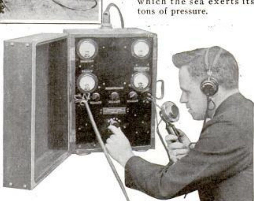
Diver Ready to Descend to Connect the Rescue Chamber with the Submarine; Below, Operator Demonstrating the Subsea Two-Way Phone
