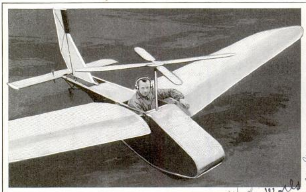
Glider Equipped with Auto-Gyro Vanes; While the Four-Vaned "Windmill" Is Too Small to Increase the Lift Materially, It Is Believed to Add to the Craft's Stability
