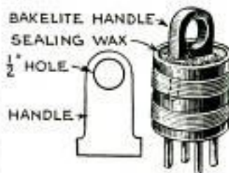
Voltage-Divider Terminal Panel and Handle for Plug-In Coil Made from Scrap Bakelite
