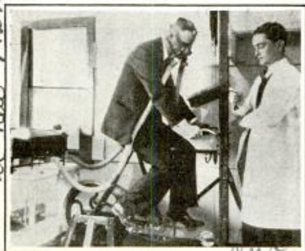
Trick Bicycle That Shows How Much Oxygen Is Used Doing Certain Kinds of Work
