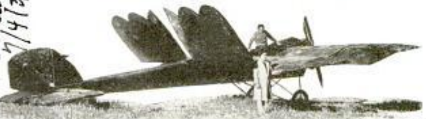
"Turkey Plane" Which Is Able to Climb at Sixty-Degree Angle and Is Equipped with Device to Prevent It Falling in Nose Dive
