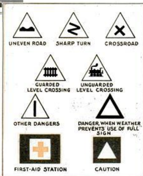
Proposed International Signals; No Words Will Be Used, so They Will Be Intelligible to All
