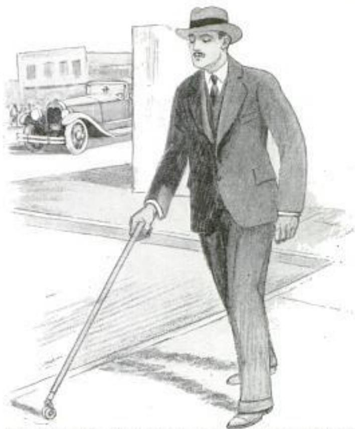
Cane Fitted with a Swivel Caster Is a Great Improvement over the Type Ordinarily Used by Blind People
