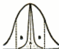
STENODE selectivity is compared above to that of ordinary receivers. All background noise is contained in outer curve. Stenode's curve, shaded, contains but 1/30 the total noise.
