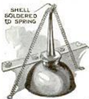
Coil Spring Holds the Oil-can Down, While Rifle Shell Caps the Spout
