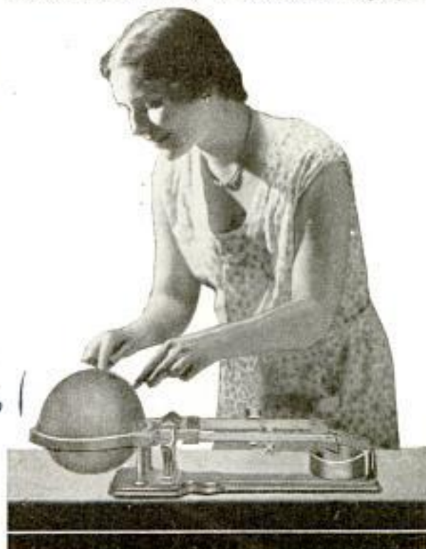
Testing Bowling Ball in Scale That Measures Its Balance as Well as Its Weight
