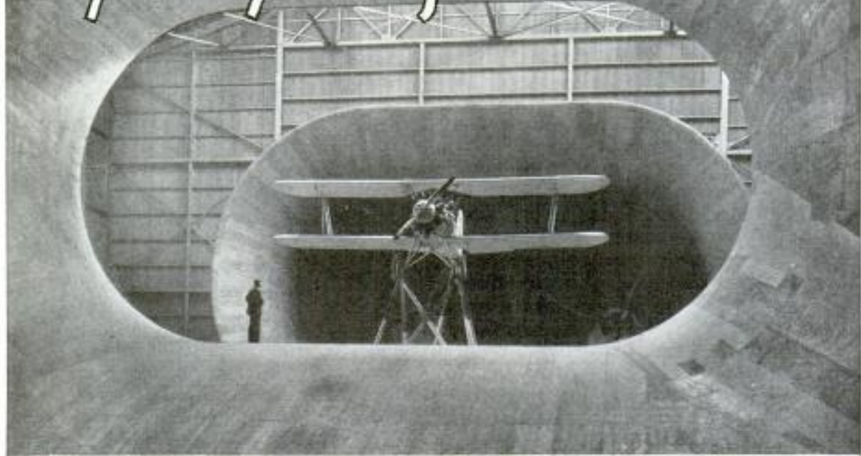
This Giant Wind Tunnel Has a Mouth Sixty Feet Wide and Thirty Feet High; a Full-Sized Airplane Is in Position to Be Blown by 100-Mile-an-Hour Wind
