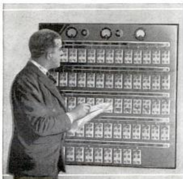
System of Meters in One British Relay Station Which Shows Popularity of Radio Program
