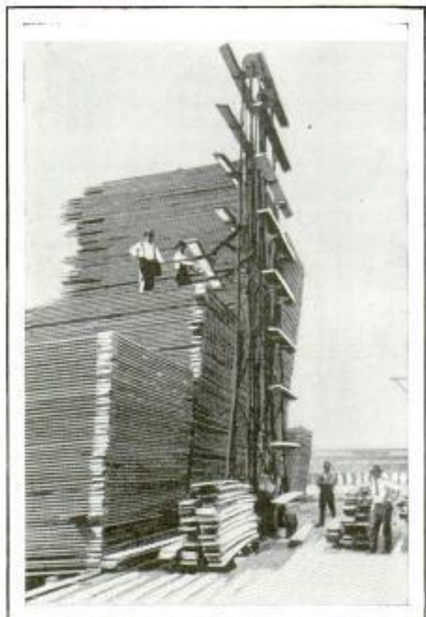
Lumber-Piling Machine Which Is Capable of Building a Stack Thirty-Eight Feet High
