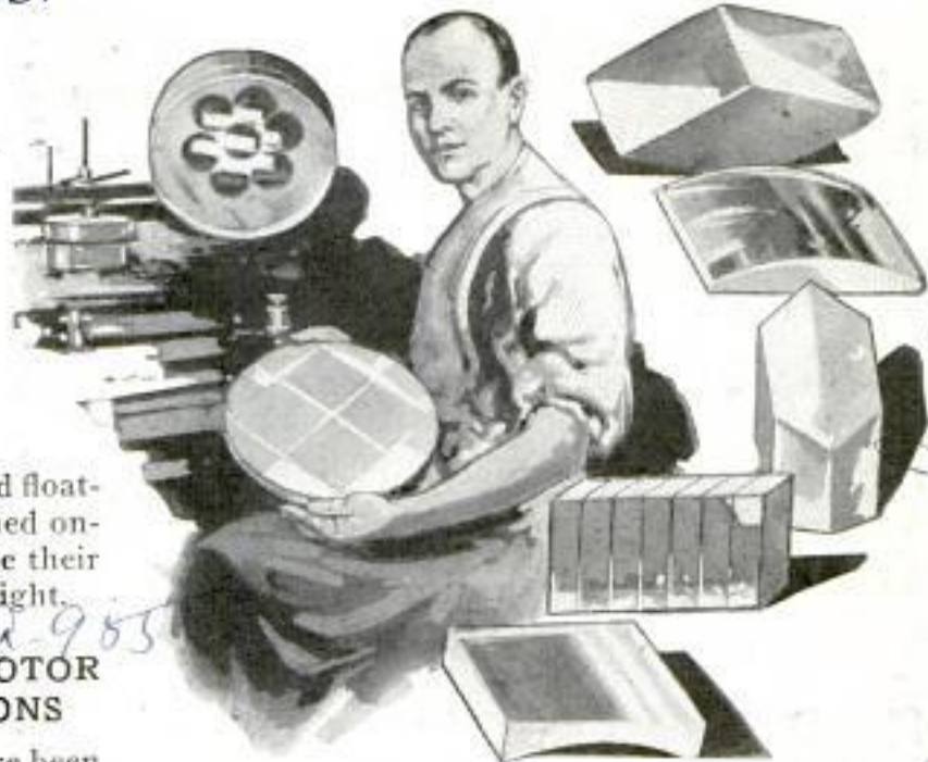
Expert Lens Grinder and Some of the Lenses of Odd Shapes That Produce the Unusual Effects in the Movies
