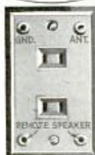
Lamp Used as an Artificial Load for Testing B-Power Units under Working Conditions; Below, Wall Plates Adapted for Switch Panel; Left, Phone-Tip Jack Arrangement
