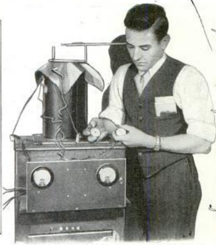
Left, Rubbing Apparatus for Measuring the Wearing Qualities of Cloth; Right, Testing Cloth for Warmth; the Cylinder Is Heated and the Heat Escapes Only through the Cloth at Top
