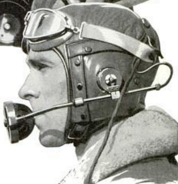
Right, Pilot Wearing Radio-Equipped Helmet and Attached Microphone; Earphones Are Built into It
