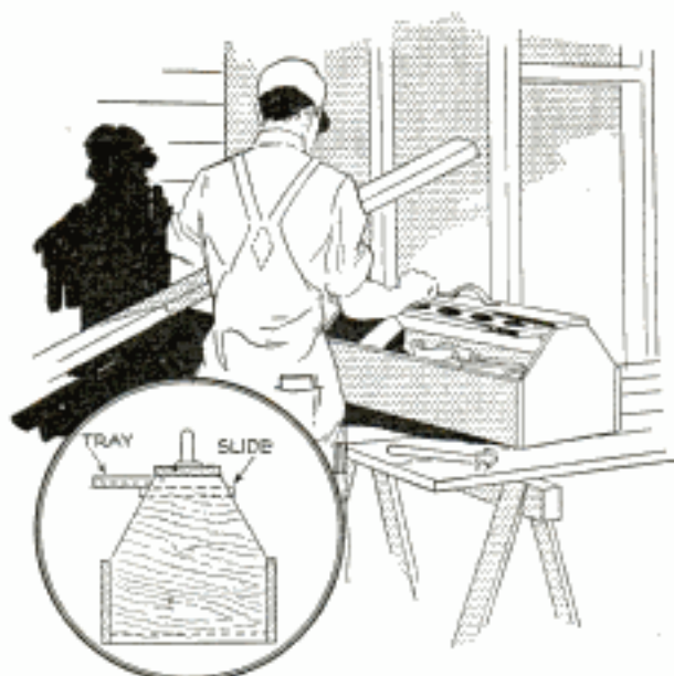
Small Brads and Tacks Are Always Ready to Hand When Kept in a Sliding Drawer of the Toolkit
