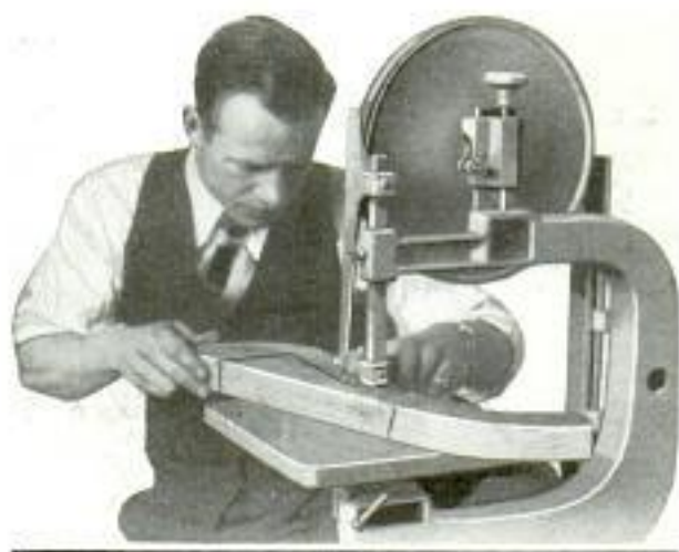
Cutting the End Frames for the Reversible Swing Takes Very Little Time on a Bandsaw
