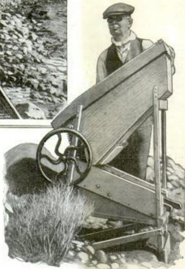
Top, a Makeshift Flume to Recover Gold from River Gravel; Right, a Homemade "Dry Wash" for Concentrating Pay Dirt
