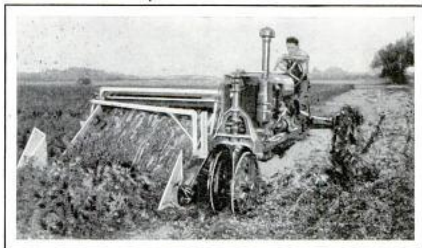
Power Mower That Runs Hay or Alfalfa through a Crusher, Made Like a Clothes Wringer, to Lessen Time Required for Curing
