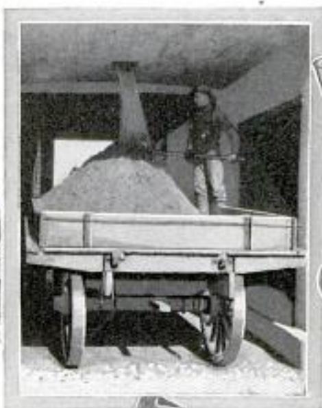
Below, Labor-Saving Method of Loading Feed on Wagons from an Overhead Storage Bin into Which It Is Blown
