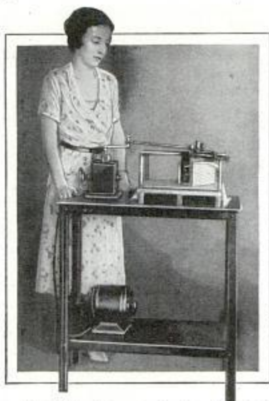
Left, Rubbing Apparatus for Measuring the Wearing Qualities of Cloth; Right, Testing Cloth for Warmth; the Cylinder Is Heated and the Heat Escapes Only through the Cloth at Top
