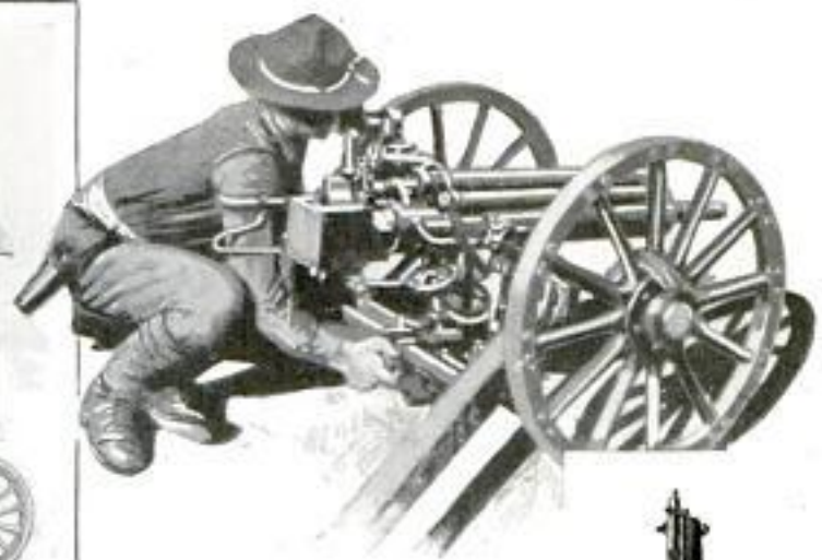
Above, Anti-Tank Gun with Well-Balanced Carriage, Which Makes It Easy to Train the Weapon on a Moving Target; Right, Semi-Automatic Rifle That Is Gas-Operated to Decrease Shock of Firing; It Weighs About Nine Pounds and the Magazine Holds Ten Shells
