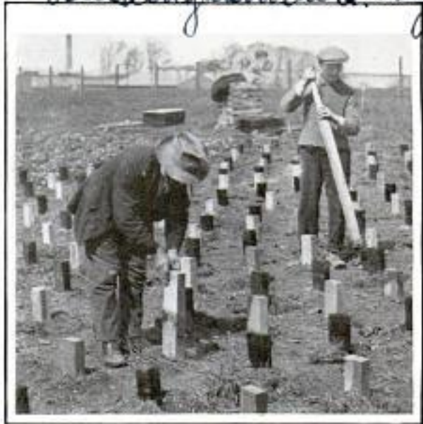
Posts Treated with Different Forms of Wood Preservative in Test to Find Best Kind
