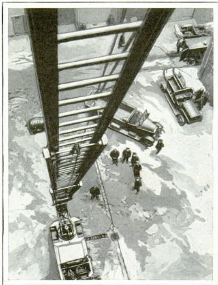
Automatic Extension Ladder Mounted on German Fire Truck; the Ladder Is Electrically Controlled by Means of a Push Button
