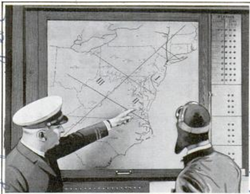
Electric Weather Map for Aviators Which Shows by Means of Colored Lights Flying Conditions to Be Encountered in Any Area
