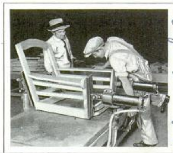
Air Clamp by Means of Which an Entire Furniture Frame May Be Put Together in One Operation
