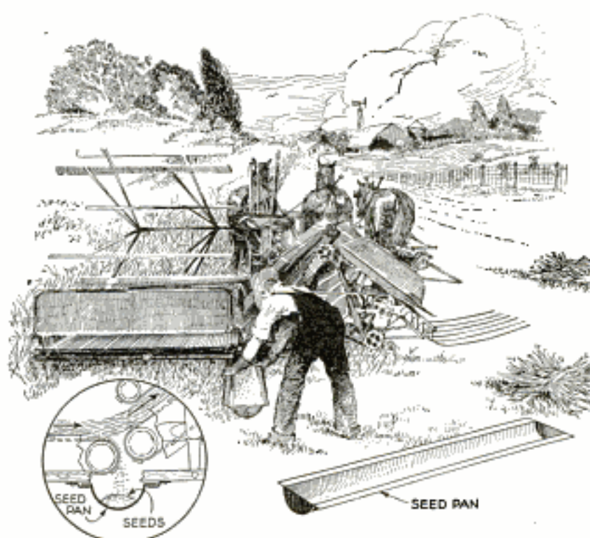
Sheet-Metal Seed Pan on Farm Binder Collects Ripe Weed Seeds and Checks Further Distribution and Growth
