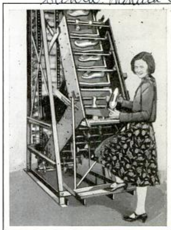
Automatic Shoe Soler That Fits and Attaches Soles to Uppers, Increasing Output of Workmen
