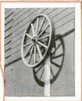
Above, Wagon Wheel Forms Flywheel on Driveshaft of Farm Hoist; Left, Bushel Basket Fitted with Funnel Avoids Spilling Seed or Fertilizer, and Extension Boxes Increase Capacity of the Planter
