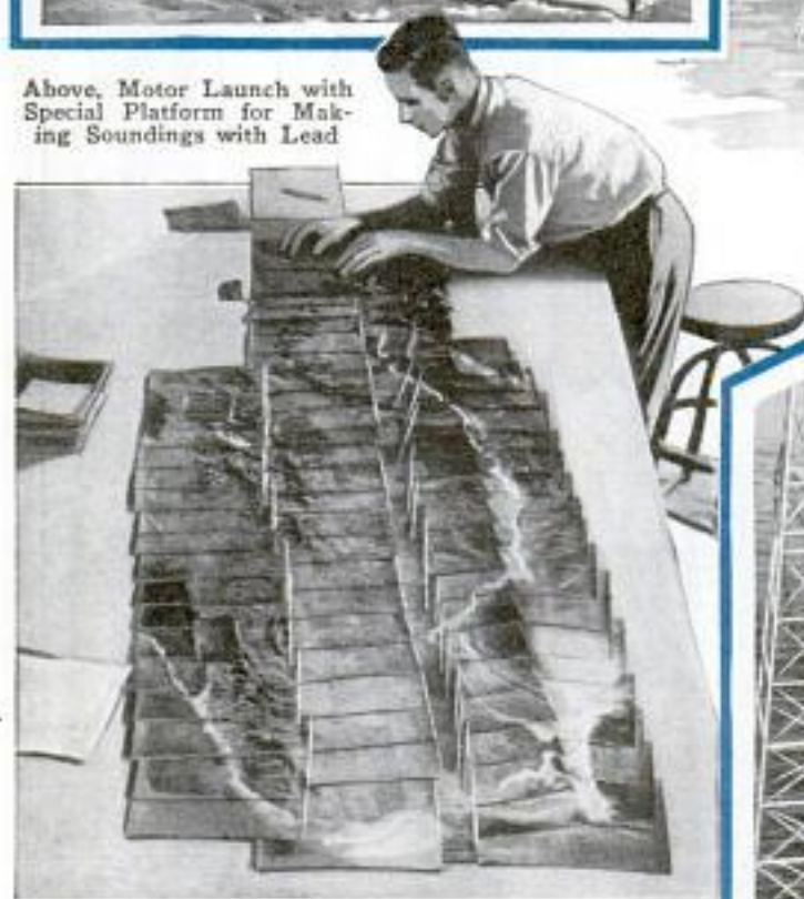
Above, Air Photographs of Porto Rico Taken by Naval Planes and Pieced Together to Form a Mosaic; the Photographs Are Systematically Taken to Overlap
