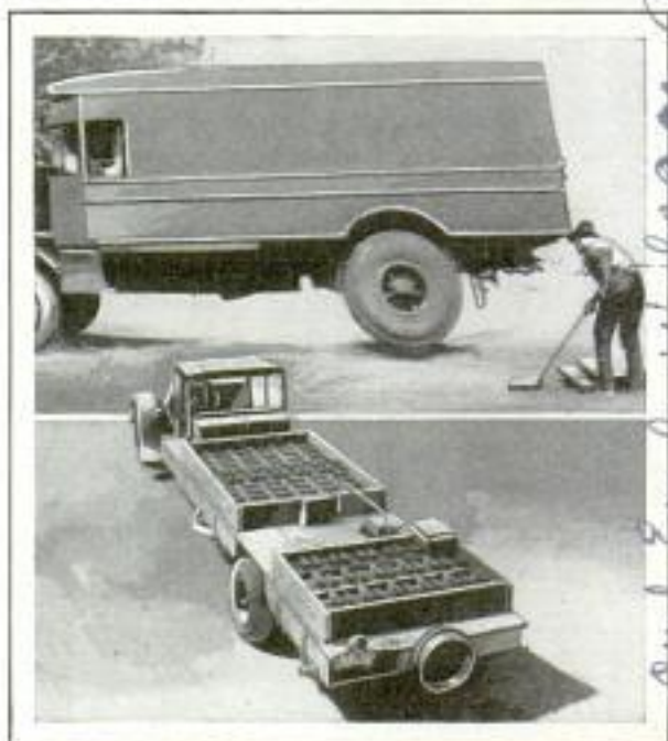
Truck Equipped for Measuring Shocks from Bumps; Small Compartments Hold 100-Pound Weights
