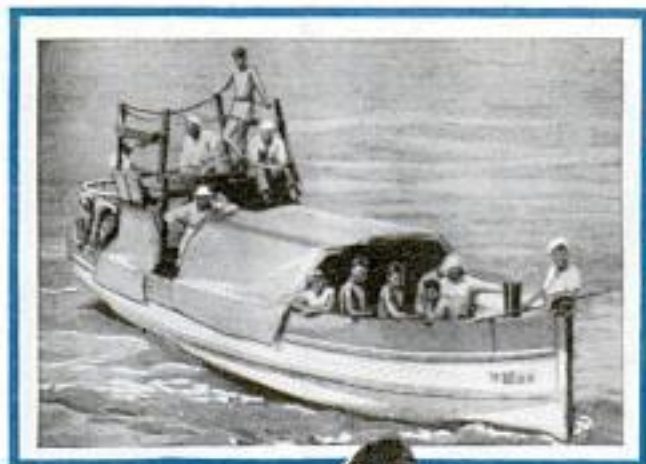
Above, Motor Launch with Special Platform for Making Soundings with Lead
