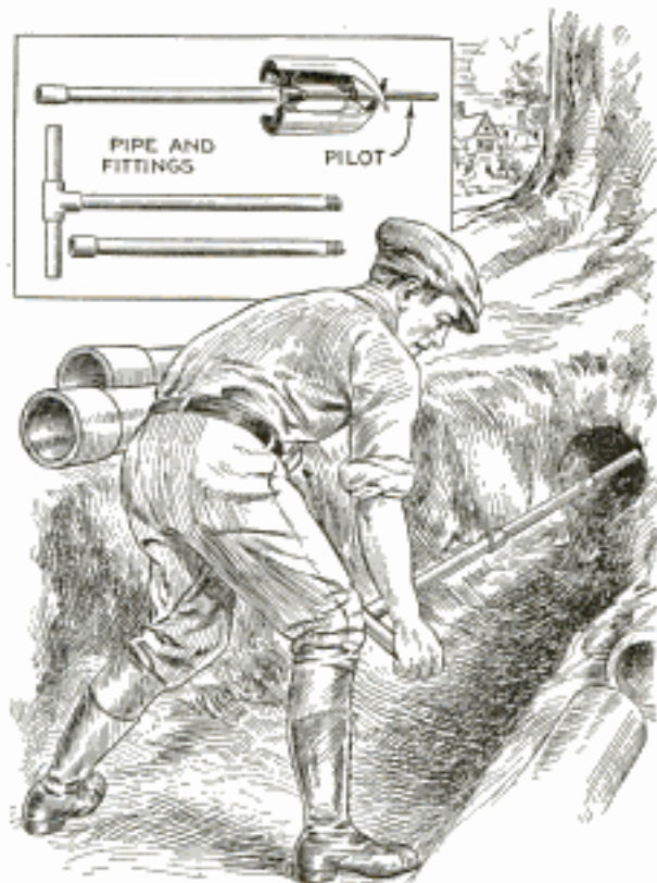
Pipe Extension on Post-Hole Auger for Boring Drainage Holes under Obstructions
