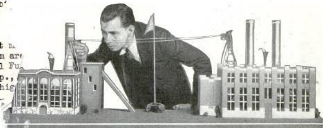
Demonstrating the Transmission of Noiseless Power from a Model Station by Use of Grid-Glow Tubes Which Can Change Alternating Current to Direct Current or Reverse the Process
