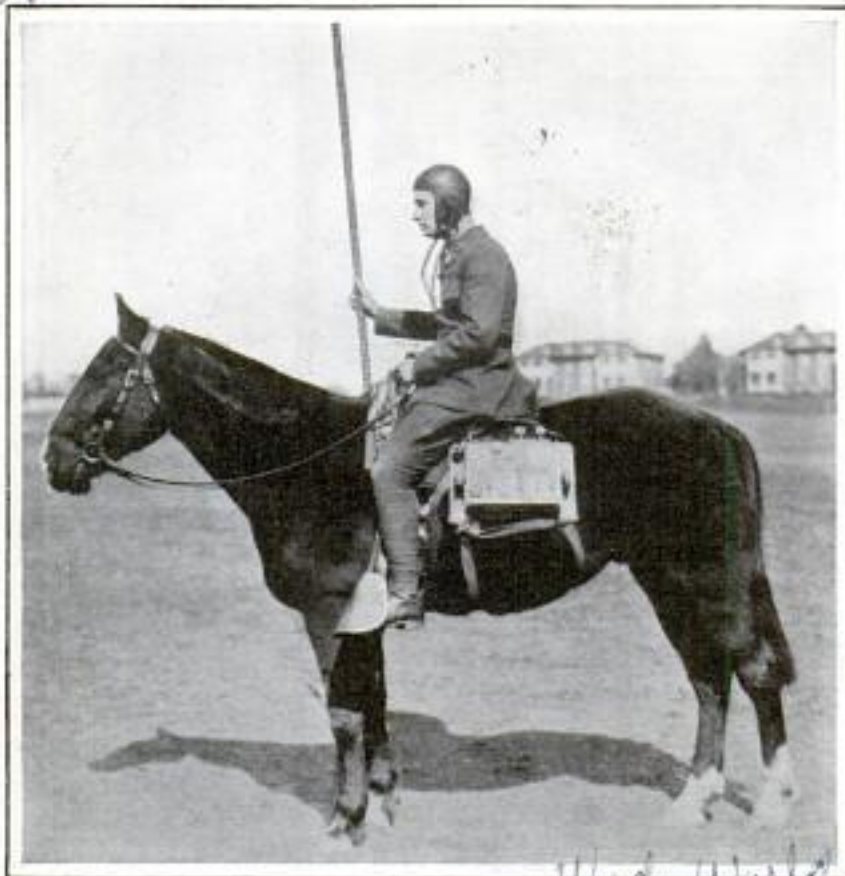
Radio Set Developed by the Signal Corps for Use by Cavalry; the Pole Held by the Rider Acts as the Aerial
