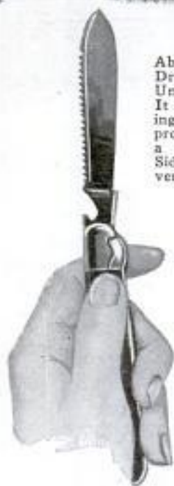
Above, Camper's Knife with Safety Blade Which Locks into Position When Thumb Is Pressed on Section to Snap It Open; Note the Fish Scraper and the Bottle Opener
