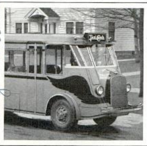
The Driver of the Taxi-Coach Sits over the Engine So He Can See the Road
