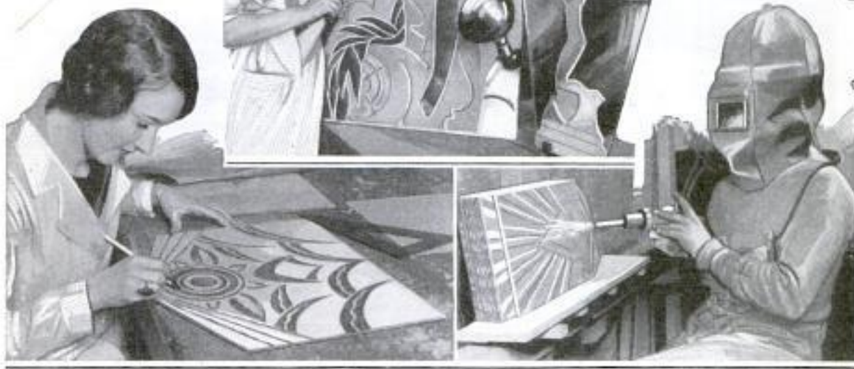
Top, Colored-Glass Design Carved with Sand and Compressed Air; Left, Cutting Design from Cardboard Glued to the Glass; Right, Using the Sand Blast to Impress a Design in Glass
