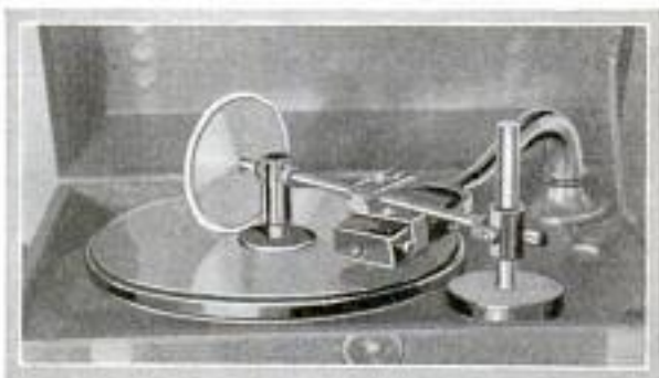
Complete Recorder Applied to an Electric Phonograph is drilled clear through this arm, to take the small end of the lead screw.
