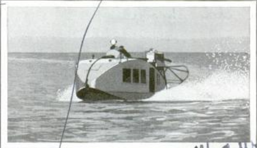
Glide Boat with Steps in Bottom to Keep It Horizontal at High Speeds; It Can Travel in Shallow Water as It Has No Keel
