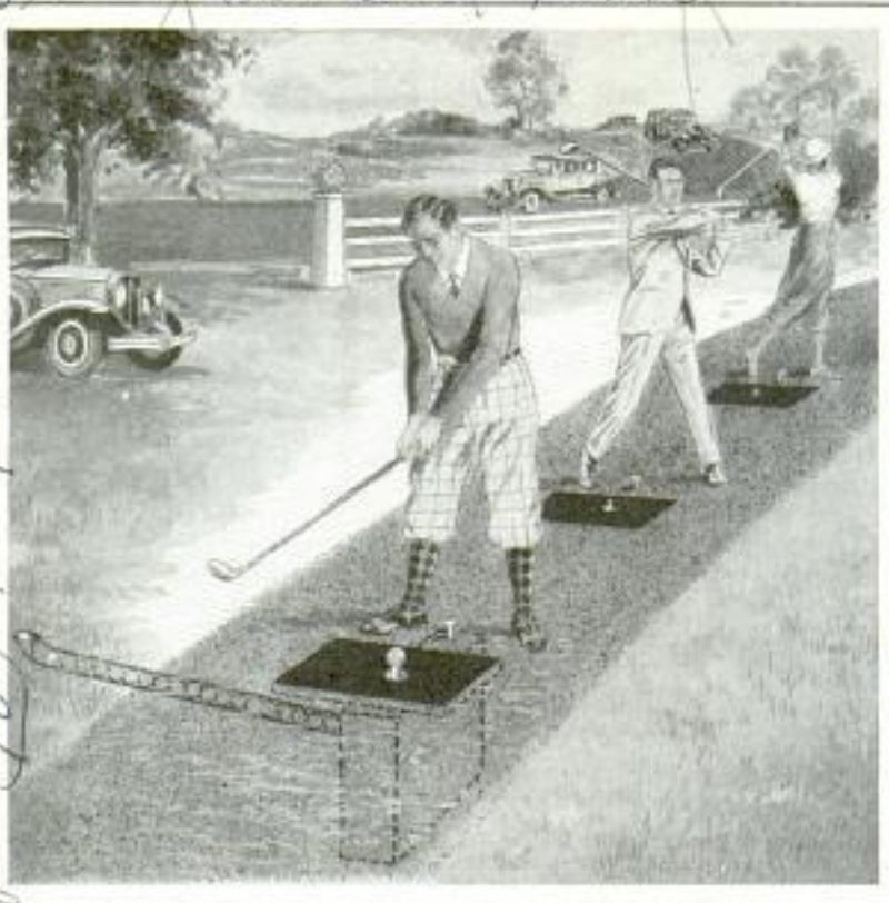
Automatic Golf Tee for the Driving Range, Which Places a Ball in Position to Be Hit When Plunger Is Pressed with Foot
