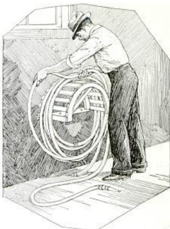
There Will Be No Kinks in Your Garden Hose if It Is Coiled on This Rack
