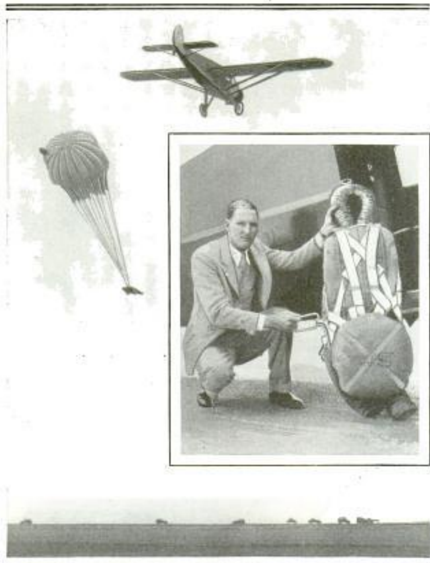
Parachute That Opens Instantly and Intended for Leaps from Very Low Altitudes; It Is Shown as It Was Tested with a Dummy
