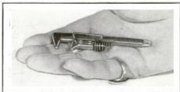
Tiny Monkey Wrench for Fine Work; the Tip of the Handle May Be Used as a Screwdriver
