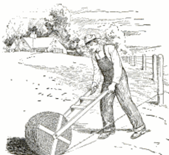
Improvised Reel Holder Pushed Along Single-Handed, Unwinds Barb-Wire Fencing
