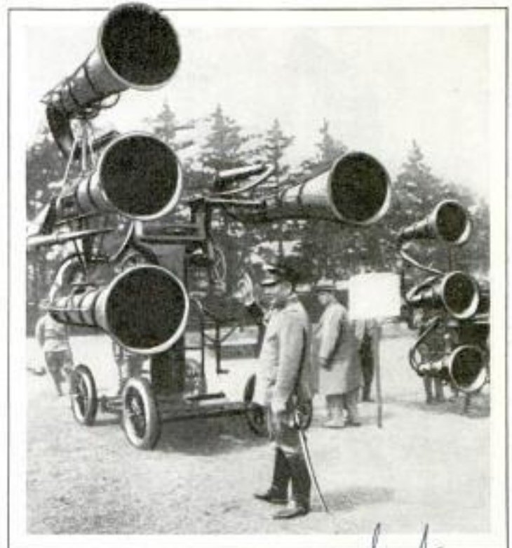
Portable Detectors Developed for Japanese Army; They Warn of the Approach of Enemy Planes
