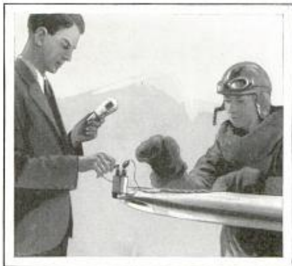
Attachment for Plane Wing Which Warns Pilot of Danger of Structural Failure in Flight
