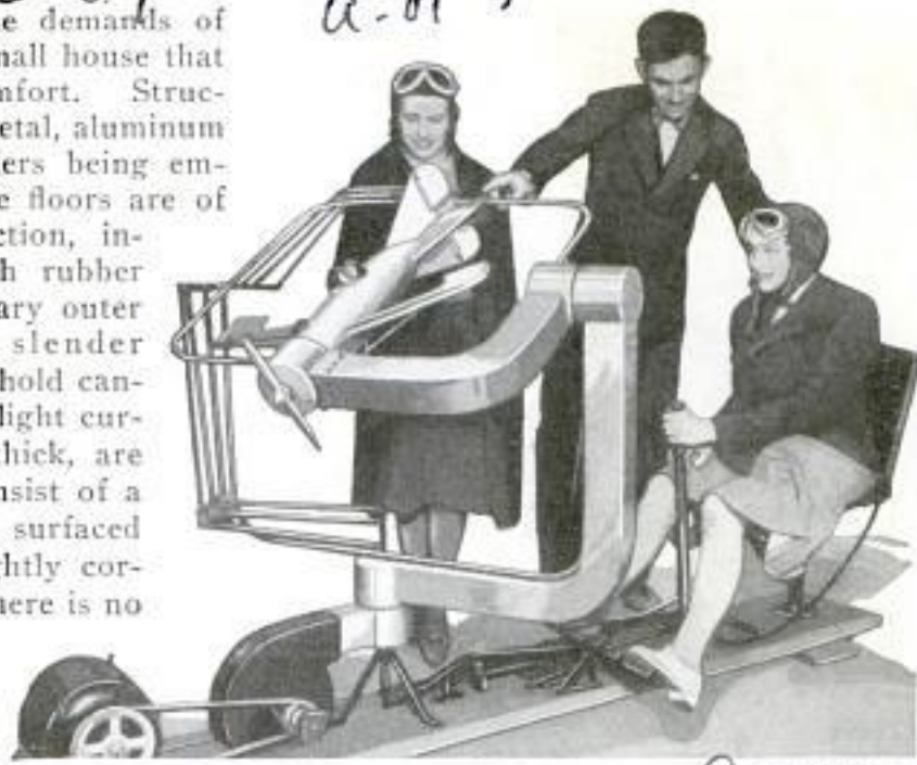
Ground Trainer for Flyers in Which Standard Controls Manipulate a Small Plane as Jets of Air Are Directed against It
