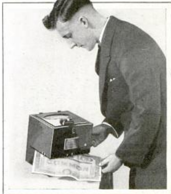
Electric Detector Which Spots Counterfeit Certificates by Identifying the Paper Stock
