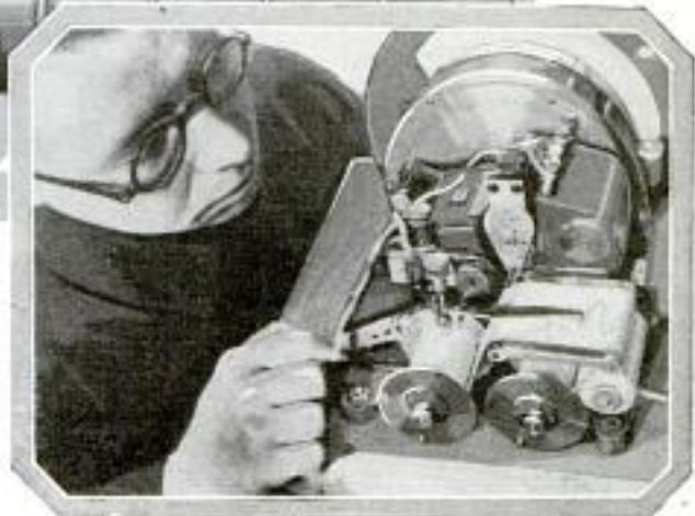
Above, Huge Loud Speakers Built on Entirely New Lines and Curves in Order to Attain a Purity and Volume of Sound Hitherto Impossible; Right, Delicate Apparatus Constructed to Measure Vibrations; It Was Built to Record the Vibrations in the Hull of a Faultily Constructed German Cruiser so the Origin of the Vibrations Could Be Found and Steps Could Be Taken to Correct the Errors
