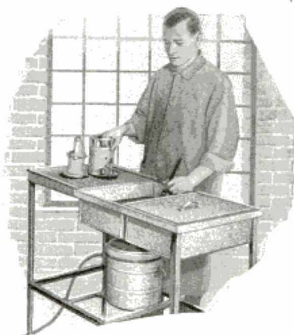
This Stand, Made of Angle Iron and Sheet Metal, Is Handy for Garages
