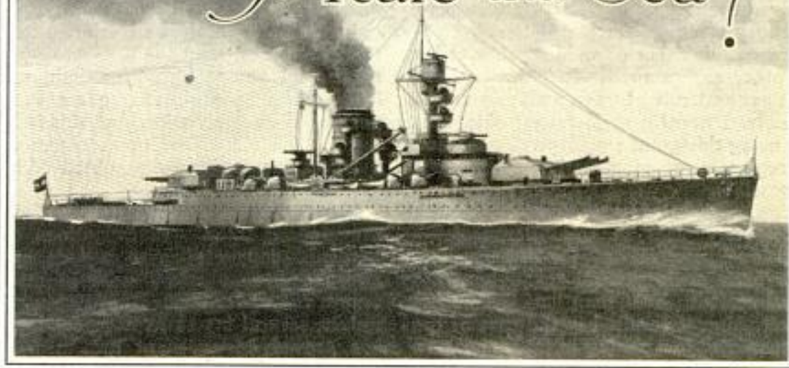
Germany's First "Pocket Battleship," a 10,000-Ton Armored Cruiser; Her Hull Is Electrically Welded and Her Eight Diesel Motors Develop a Total of 50,000 Horsepower
