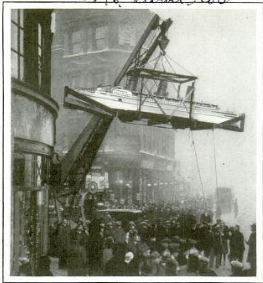
Crane Being Used to Hoist Model of Liner "Empress of Britain" to Second-Story Display Window; the Craft Weighs Half a Ton
