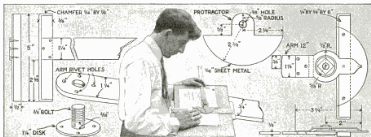
This Light, Portable Drafting Board Has a Double-Headed T-Square and a Protractor That Serves the Purpose of Triangles, Enabling Accurate Work and Making It Ideal for Outdoor Sketching
