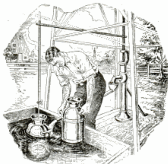
Stirring Rod Actuated by Windmill Helps to Drive Out Heat from Milk
