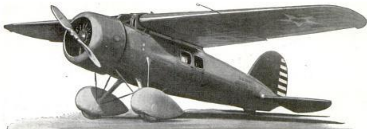
One of the Newest Army Planes; an All-Metal Monoplane with a Speed of 221 Miles an Hour; Note Its Fleet Lines and the Streamlining of the Body and Landing Gear
