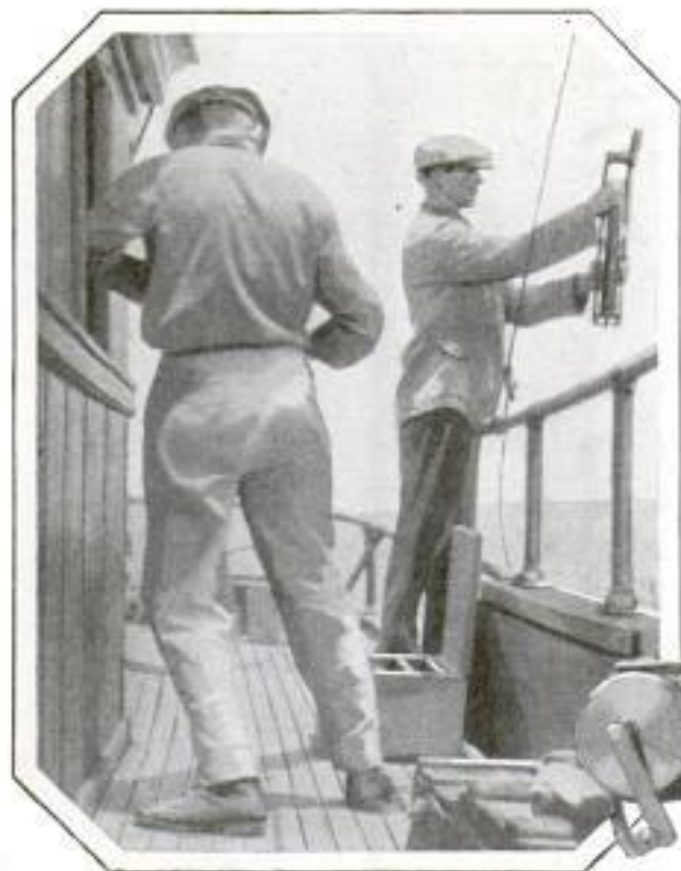
Above, Bottle for Taking Temperatures and Water Samples at Different Depths; Right, Apparatus for Taking Animal and Plant Samples from Deep Water
