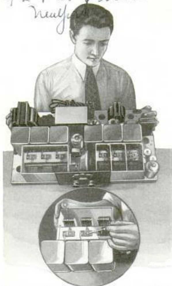
Completely Assembled Set Showing Power Unit at Rear, and Band Filter with Trimmers Indicated
