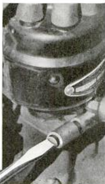
Screw Adjustment on Timer
