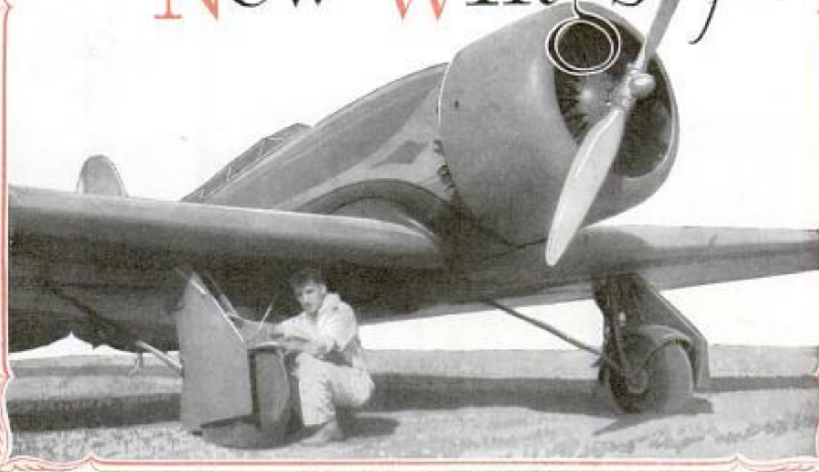
Army's Newest Low-Wing Plane with Its Wide Tread for Safety in Landing; Note the Retractable Landing Gear; the Wheels Can Be Raised or Lowered in Only Fifteen Seconds
