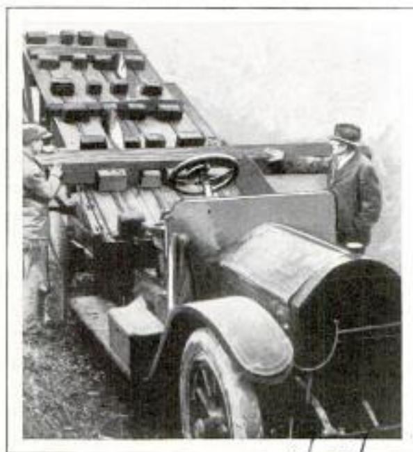
Portable Sawmill Built on Auto Chassis and Operated by the Engine of the Car
