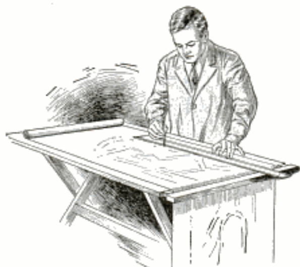
Drawings of Any Length Can Be Handled on the Drawing Table by Using a False Edge
