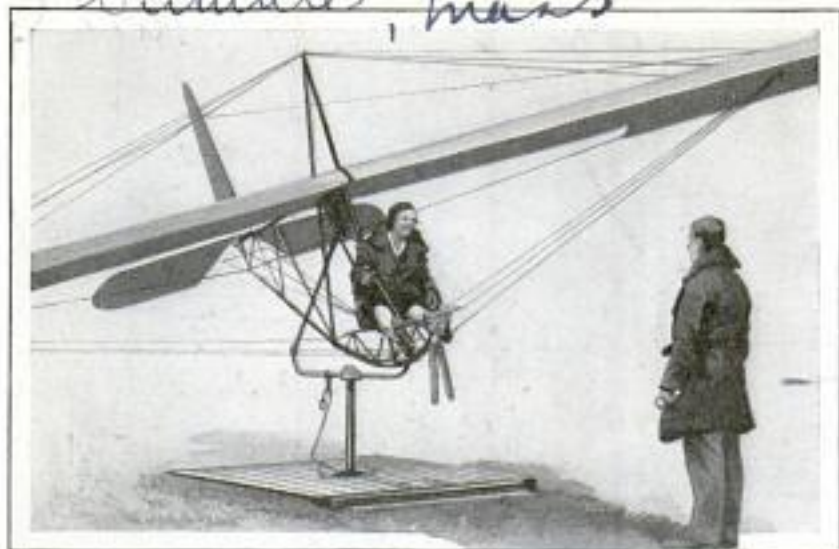
Safety Glider for Students; the Craft Has Standard Controls and Is Attached by a Universal Joint to Top of a Steel Plunger
