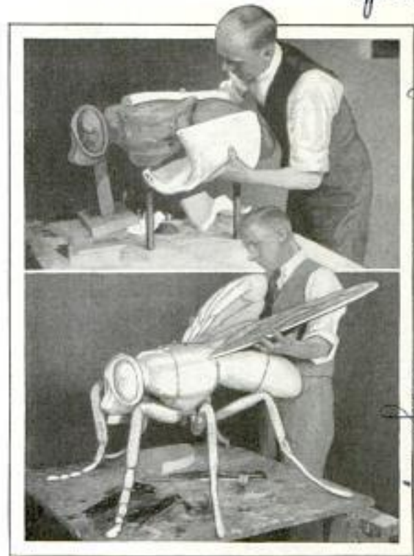
Making Model of Giant Housefly; Electric Motor Inside Body Raises and Lowers the Head
