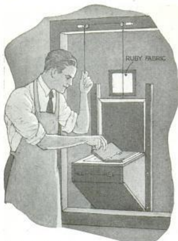
Practical Printing Frame, Attached to Darkroom Window, Utilizes Daylight to Expose Prints
