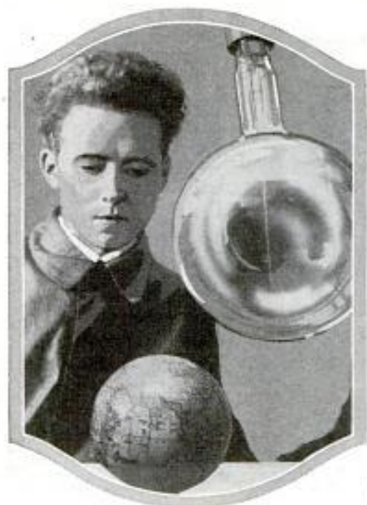
Apparatus Which Makes Electron Rays Visible by Diverting Them from Their Path by Means of a Magnet, Represented in the Photograph by the Globe
