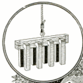
Battery of Magnets Dragged along the Bottom, Recovers Lost Iron and Steel Articles
