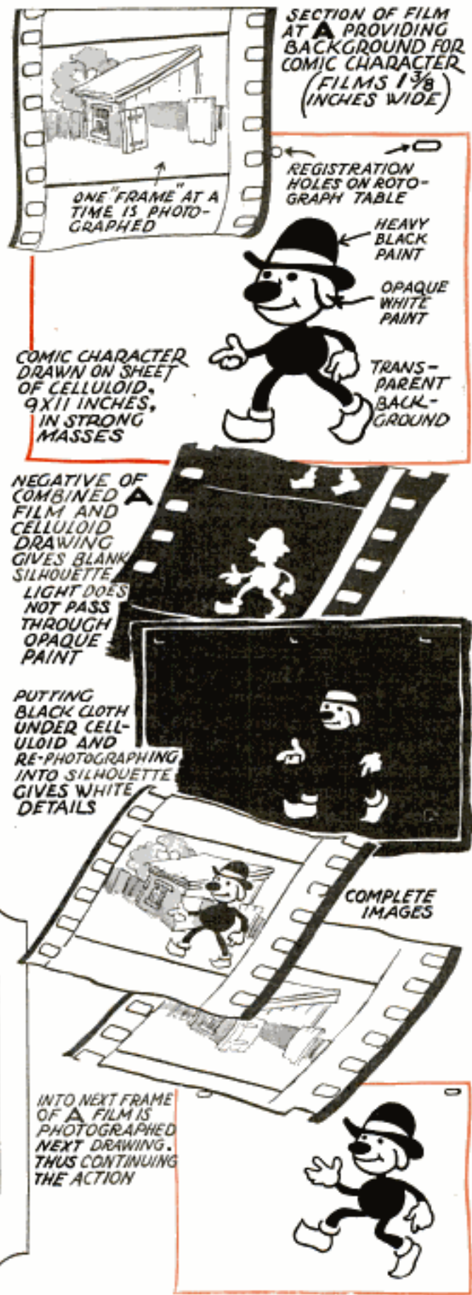
The Various Operations Necessary to Produce One Single View in a Talking Cartoon and the Sound Effects; on the Screen the Picture Is Viewed But an Instant
