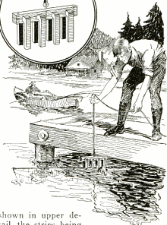
Battery of Magnets Dragged along the Bottom, Recovers Lost Iron and Steel Articles
