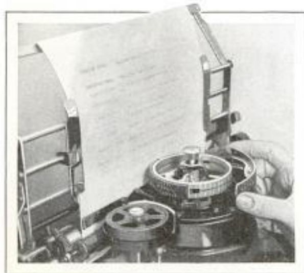
Electric Typewriter with Circular Frame on Which Different Type Faces Can Be Mounted
