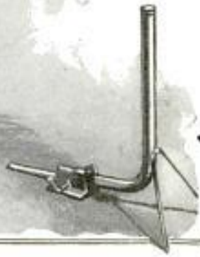
Automatic Golf Tee for the Driving Range; It Delivers a Ball When a Pedal Is Pressed
