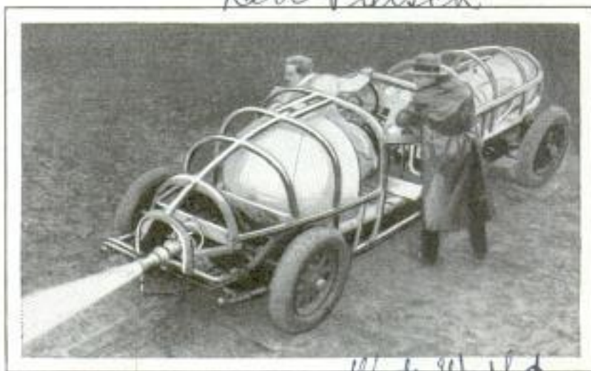
Rocket Auto Recently Tested in Berlin; Propulsive Power Is Supplied by the Successive Explosions of a Series of Rockets
