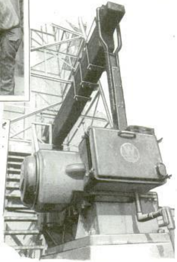
Lowering String of Large Casing in Well: Right, Silent Electric Motor and Gears Inclosed in Single Box for Pumping a Deep Well
