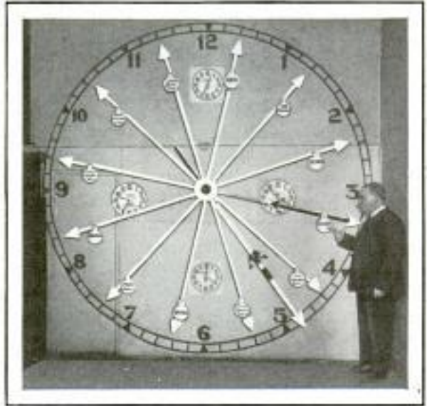
Clock with Many Dials and Hands Which Indicate Time in All Parts of World Simultaneously
