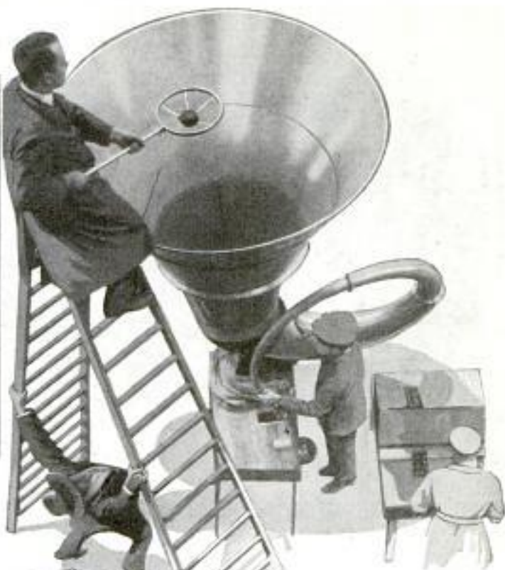
Testing Giant Loud Speakers with the Aid of a Microphone; to Allow the Waves to Spread to All Sides, the Speakers Are Held Up Vertically
