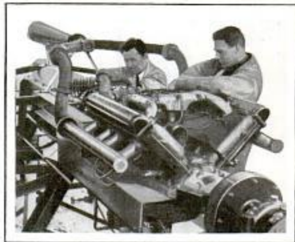
Trying Out a Muffler on Airplane Engine in Effort to Reduce Noise without Decreasing Power
