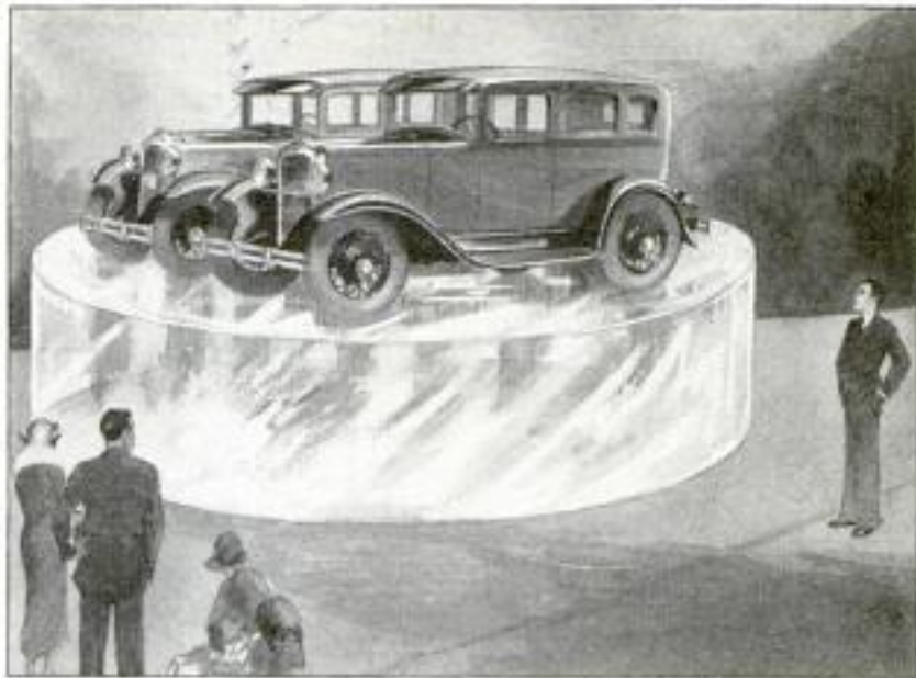
Huge "Frozen Eye" of Fused Quartz Which Will Become Reflector for Giant Telescope; the Two Autos Emphasize Its Magnitude
