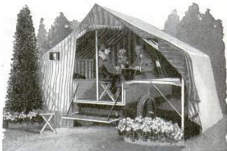
Automobile for Campers with the Tent Set Up and Ready for Use as Soon as the Destination Is Reached
