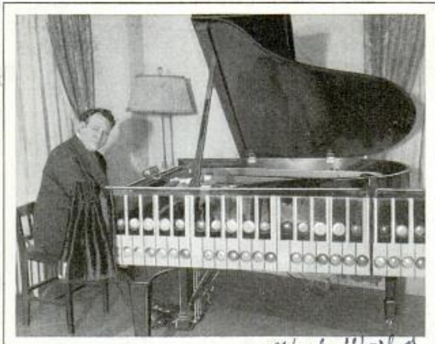
This Piano Transforms Sound Waves into Color Tones, Thus Making the Music Visible, a Different Shade of Light Representing Each Note
