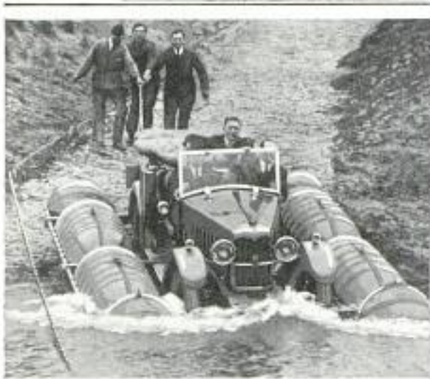
Seagoing Auto, Showing Detachable Floats Being Inflated and the Car Entering a River
