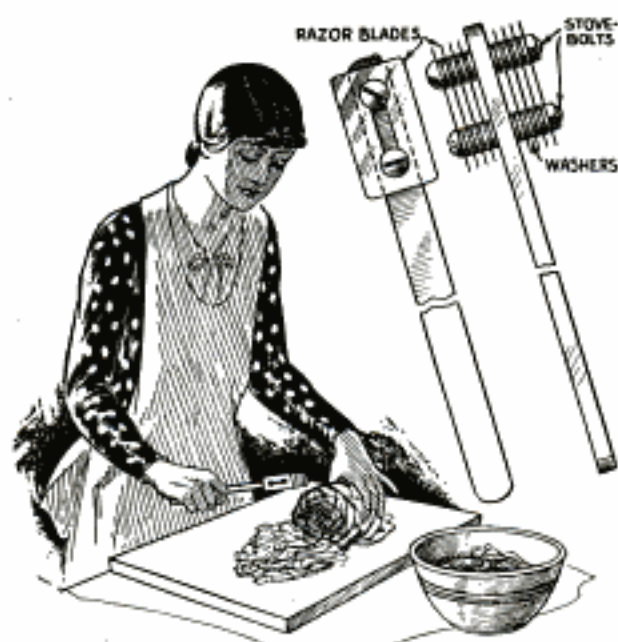
Many Uses Can Be Found for a Sharp Food Chopper Consisting of Razor Blades
