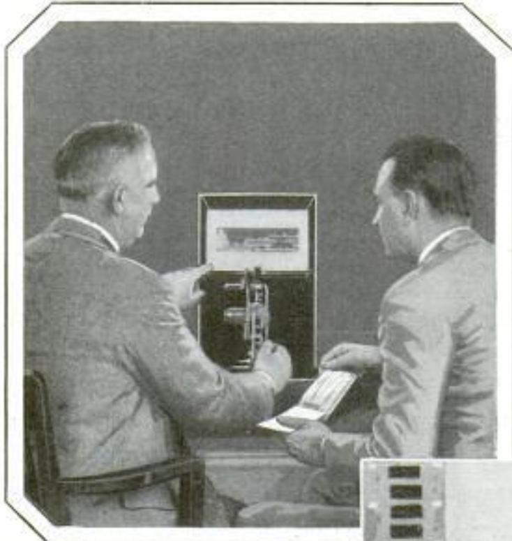
Projector Used to Examine Checks After They Have Been Recorded on Movie Film; Right, Fingerprinting Outfit That Utilizes a Tiny Movie Camera to Make a Permanent Record of Checks Dropped into the Hopper
