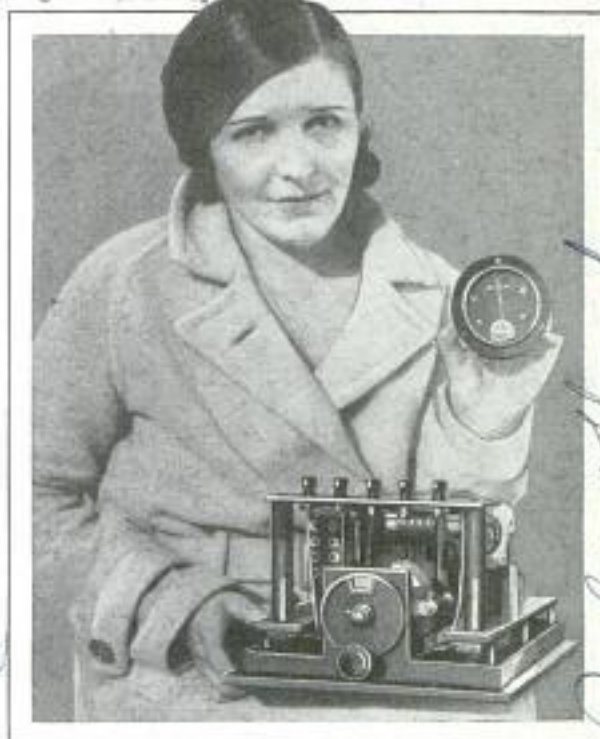
Small Radio Set Which Will Guide a Navy Plane Back to Carrier Ship, and the Pilot's Indicator
