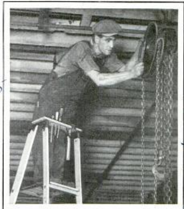
Ladder Containing a Platform and a Tool Rack in the Top, to Save Steps for the Workman
