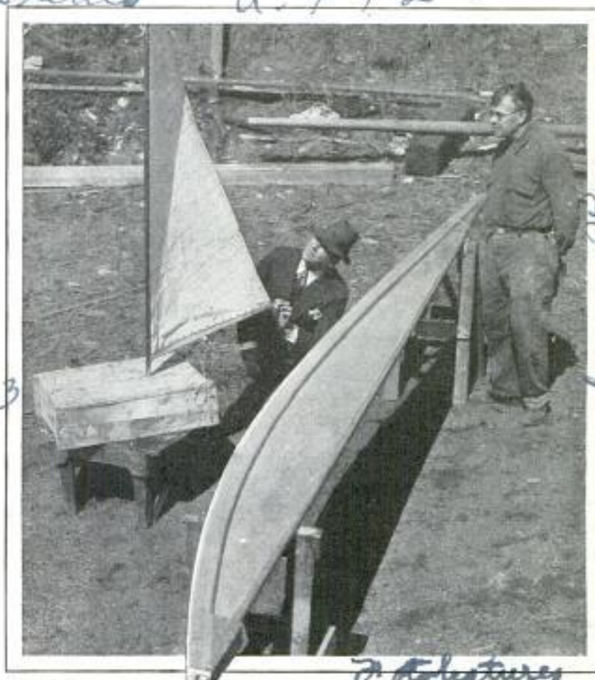
Swivel Boom for Racing Yachts and a Model Showing It in Use—the Unusual Shape Helps Hold Sail in Most Effective Position
