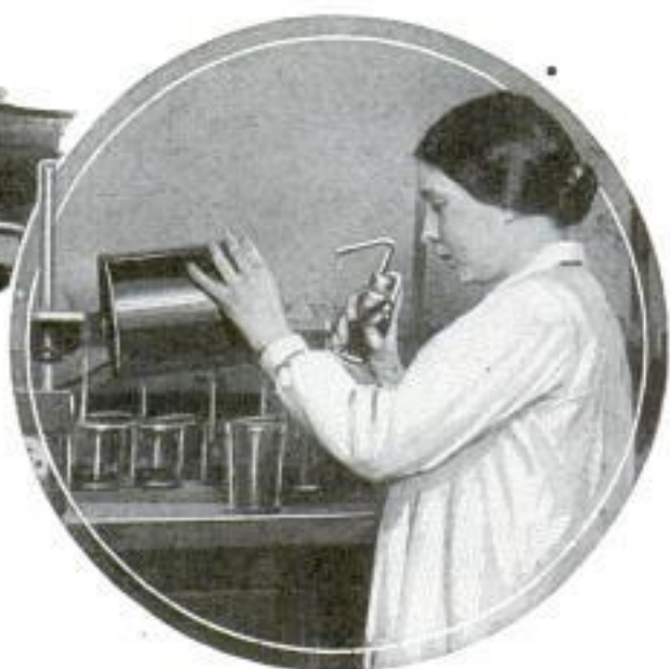
Above, Collecting a Sample of Air with a Jet Dust Counter; Right, Measuring Dust Deposited from the Atmosphere
