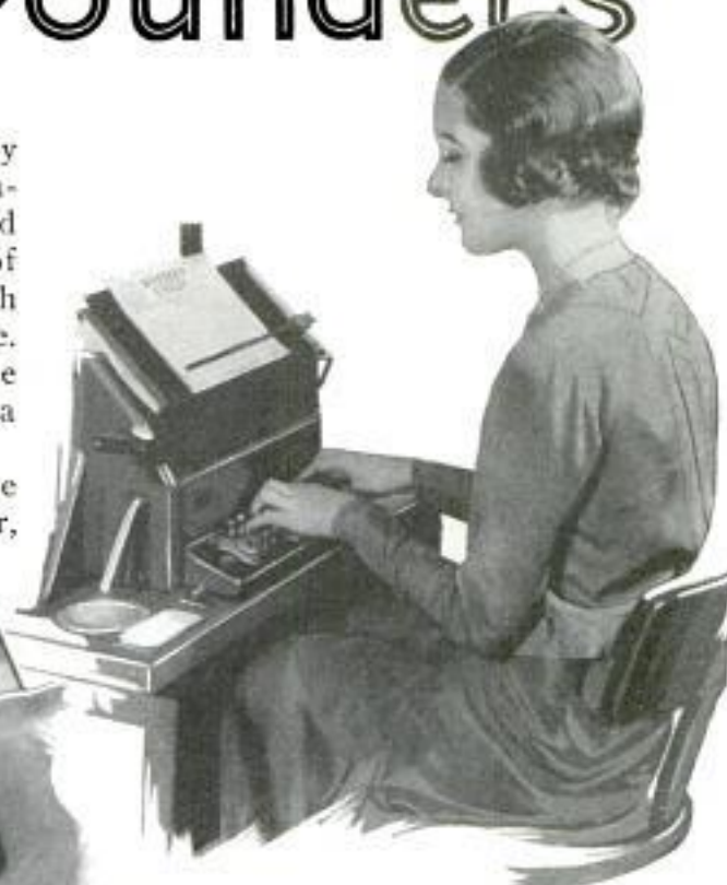
Above, Operator Typing Message on a Keyboard; It Is Transmitted and Automatically Printed on a Tape, Then Gunned to Receiving Blank as at Left
