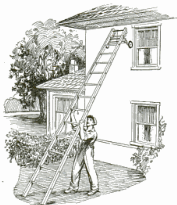
Rubber-Tired Coaster Wheels Fitted to Ladder Make It Easy to Raise against Walls
