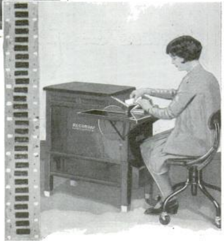
Projector Used to Examine Checks After They Have Been Recorded on Movie Film; Right, Fingerprinting Outfit That Utilizes a Tiny Movie Camera to Make a Permanent Record of Checks Dropped into the Hopper
