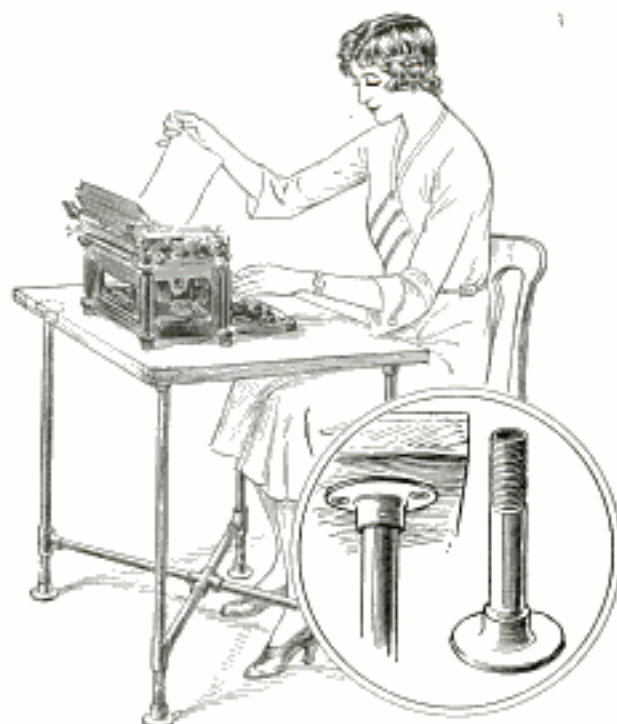
Pipe Legs and Crosspieces, Connected with Suitable Fittings, Provide Support for Typewriter Table
