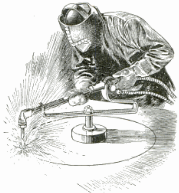
Simple Holder Which Makes It Easy to Cut Circles with an Acetylene Torch
