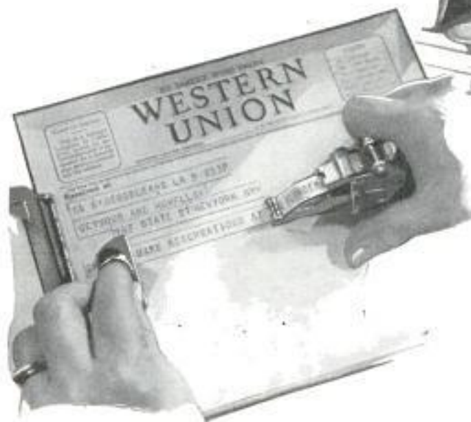
Above, Operator Typing Message on a Keyboard; It Is Transmitted and Automatically Printed on a Tape, Then Gunned to Receiving Blank as at Left
