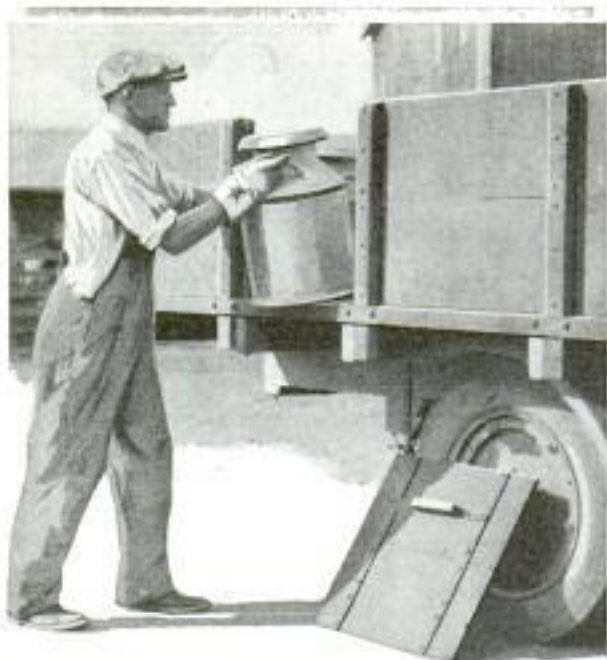
Lightening the Task of Loading Heavy Cans on Trucks by Providing a Sliding Side Door
