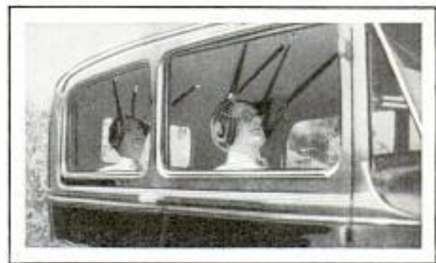
Headrest for the Auto Which Is Suspended from the Roof of the Car by Means of Straps
