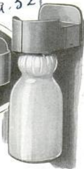
Above, Milk-Bottle Holder Which Locks Automatically When Top of Container Is Fitted into It and the Sides Are Closed around It
