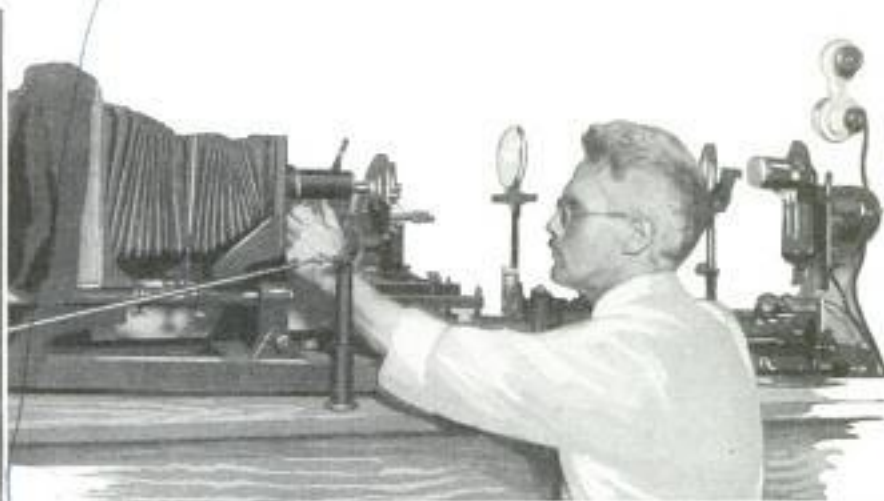
Mirror and Lens Arrangement of Photographic Outfit for Making Large Pictures of Microscopic Objects, and Example of Such a Picture
