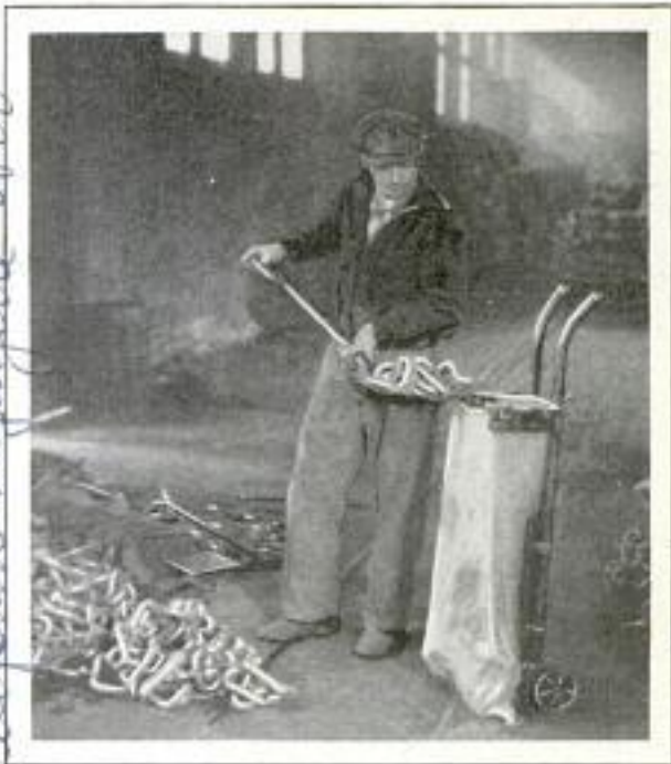
Hand Truck with a Semicircular Arm Which Holds a Sack Open, Thus Making Filling Easy
