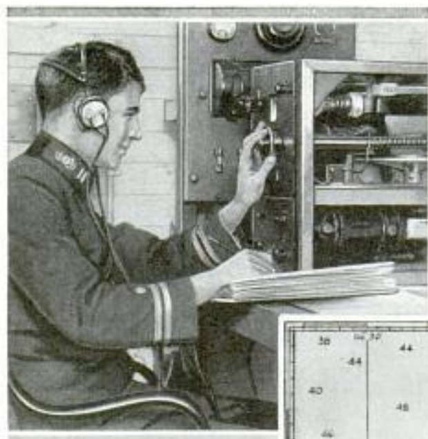
Sounding and Plotting the Ocean Bottom by Radio aboard a Ship; Right, Contour Map Showing Ocean Depths
