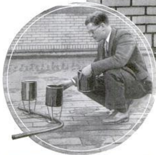
Above, Quartz Spectograph for Measuring Solar Radiation; Below, Apparatus Used to Collect Samples of Dust for Analysis
