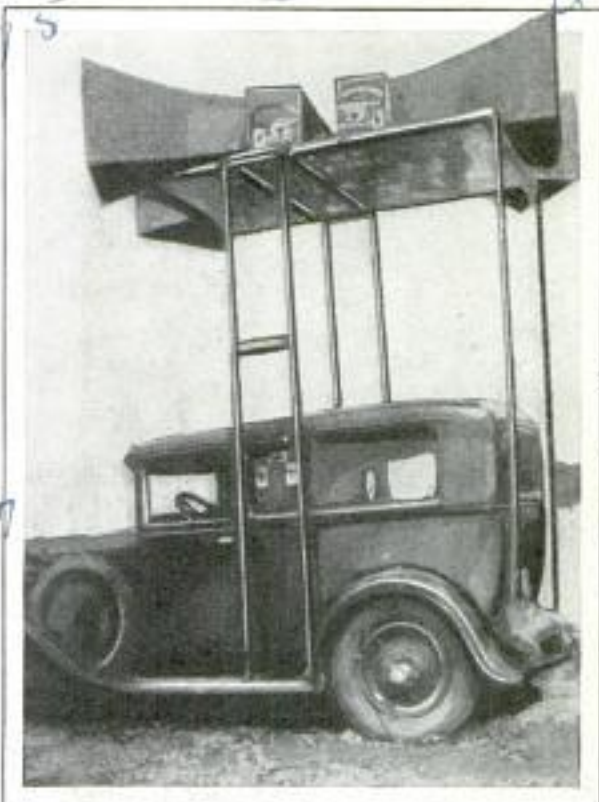
Loud Speakers Mounted on Extension Platform on Auto to Make a Portable Public Address System
