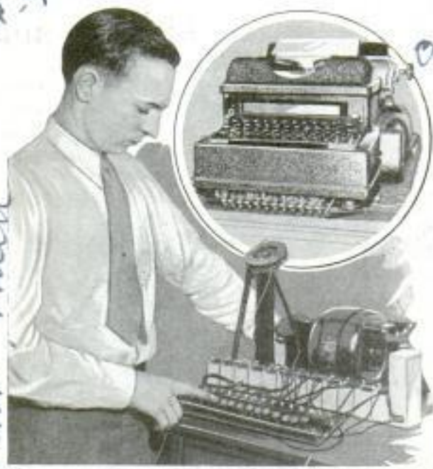
Sending and Receiving Equipment of a Radio Typewriter Which Is Actuated by Wireless Impulses
