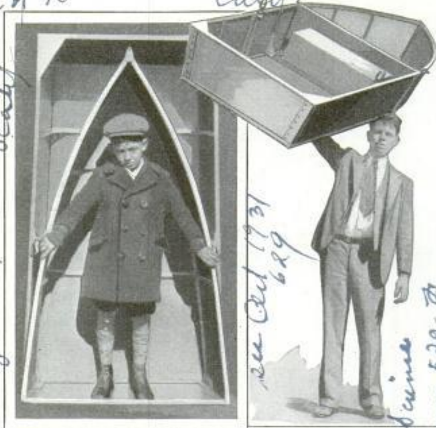
Collapsible Rowboat Made of Aluminum Alloy That Weighs Only Thirty Pounds; It Will Carry More Than Thirteen Times Its Weight
