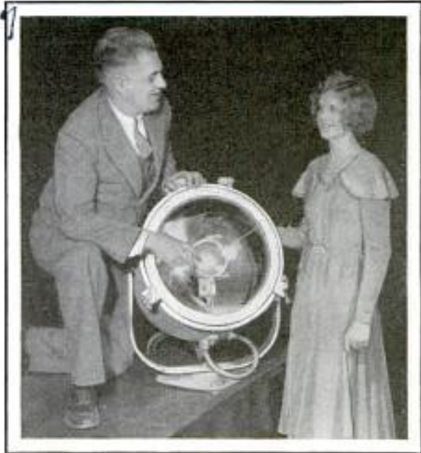
Small but Powerful Searchlight for Measuring Cloud Heights; It Casts a Beam Five Miles
