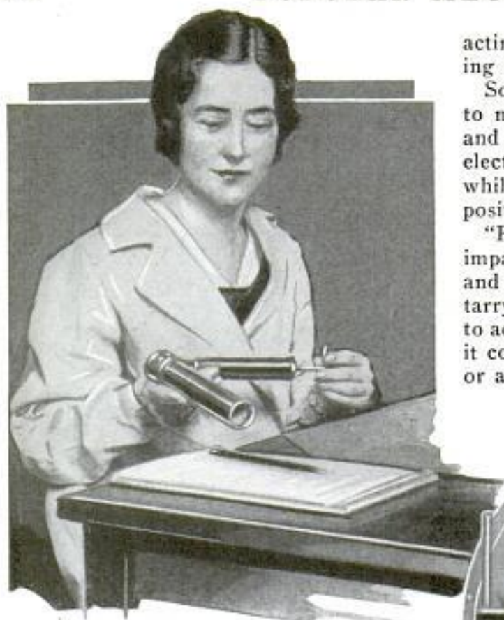
Above, Collecting a Sample of Air with a Jet Dust Counter; Right, Measuring Dust Deposited from the Atmosphere
