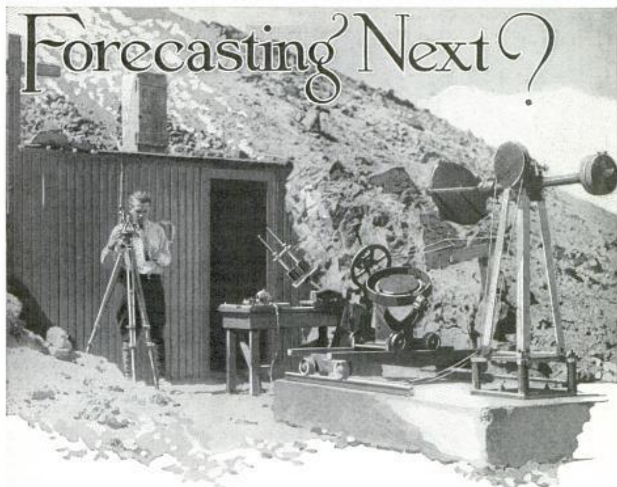
Smithsonian Solar-Radiation Observatory at Calama, Chile; the Man Is Using the Theodolite, an Instrument with Telescope Attachment for Measuring Horizontal and Vertical Angles
