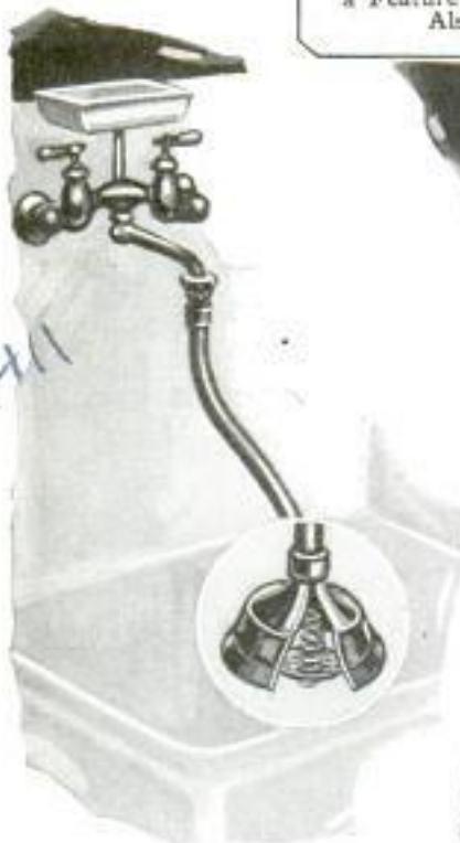
Water-Pressure Drain Cleaner with a Corkscrew Spring Which Fastens Cleaner to Strainer or Crossbar in Sink, Creating a Tight Seal and Allowing Pressure of Water System to Clean Drain
