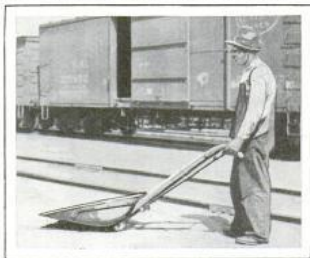
Scraper for Cleaning Ends of Box Cars Made from Dirt Scoop Fitted with Handles
