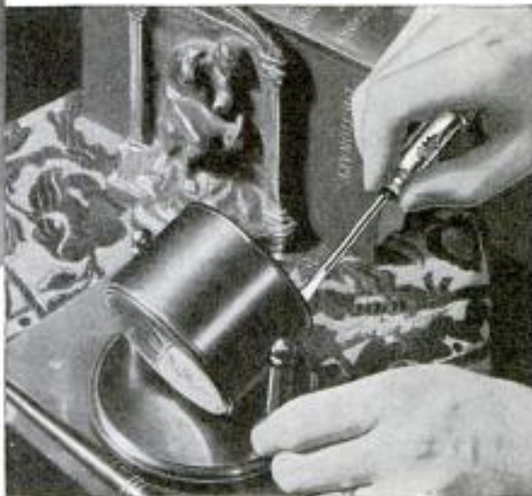
Working on "Yankee" ratchet, the handle moves to and fro with your hand. (ABOVE)
