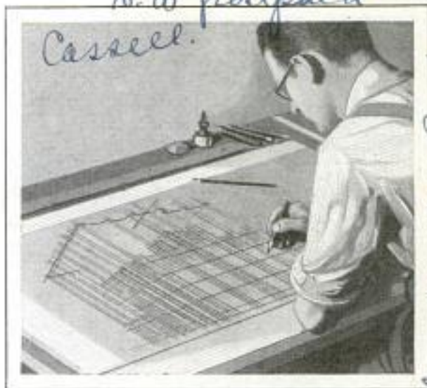
Example of Perspective-Indicator Chart, by Use of Which Depth Is Added to Line Drawings
