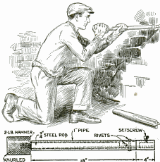
A Sliding Hammer and Drill Reduces the Task of Drilling Holes through Brick and Concrete
