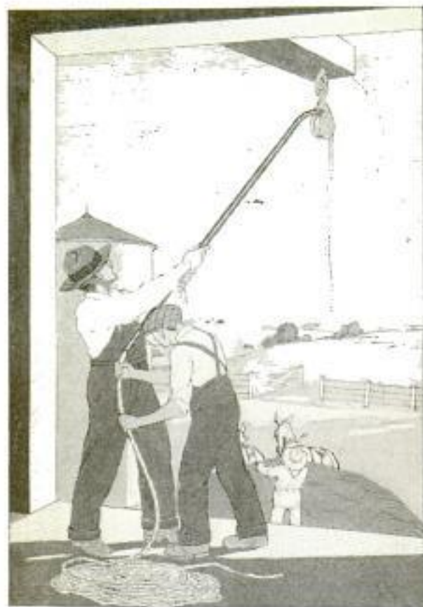
For Threading Pulleys in Places Hard to Reach, a Length of Pipe Will Prove Helpful
