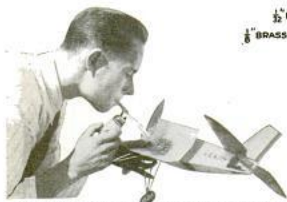
This "Lung-Power" Outfit for Spraying and Stenciling Model Planes Consists of a Pencil Cap, Two Lengths of Copper Tubing and a Screw-Top Glass Jar
