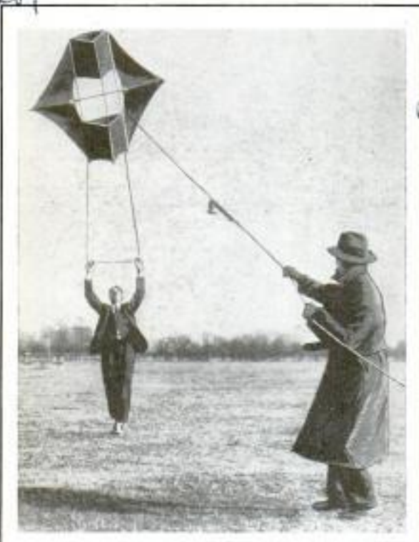
Kite Equipped with a Radio Transmitter, Which Is Used in England in Direction-Finding Tests
