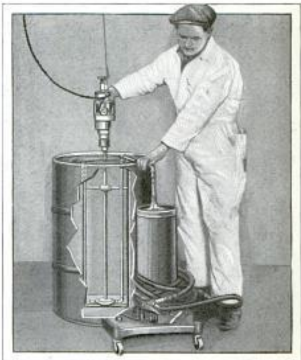
Auto Pump, Set in Grease Drum and Driven by Electric Drill, Fills Grease Gun Quickly
