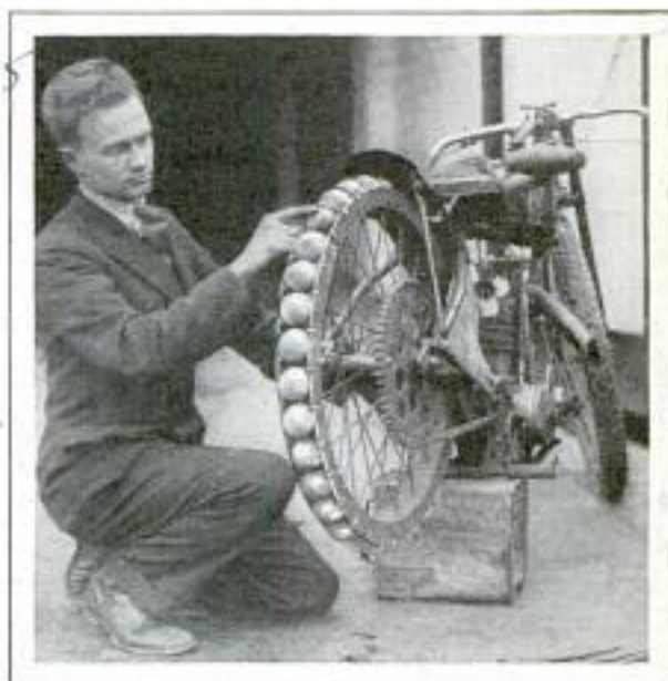
Ball-Bearing Tread for Motorcycle Wheel. Enabling Racer to "Broadside" on the Turns
