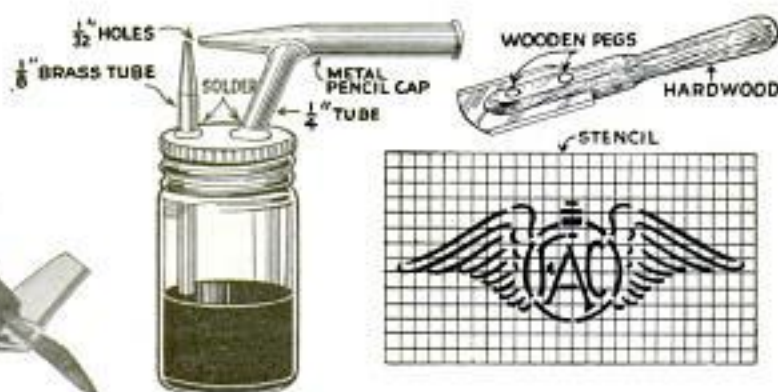
This "Lung-Power" Outfit for Spraying and Stenciling Model Planes Consists of a Pencil Cap, Two Lengths of Copper Tubing and a Screw-Top Glass Jar
