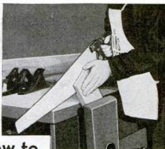
Cutting half-lap joint with Atkins Silver Steel Rip Saw No. 55.
