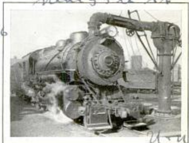
Hood Connected to Locomotive Smokestack Which Draws Off Smoke While Engine Is Standing
