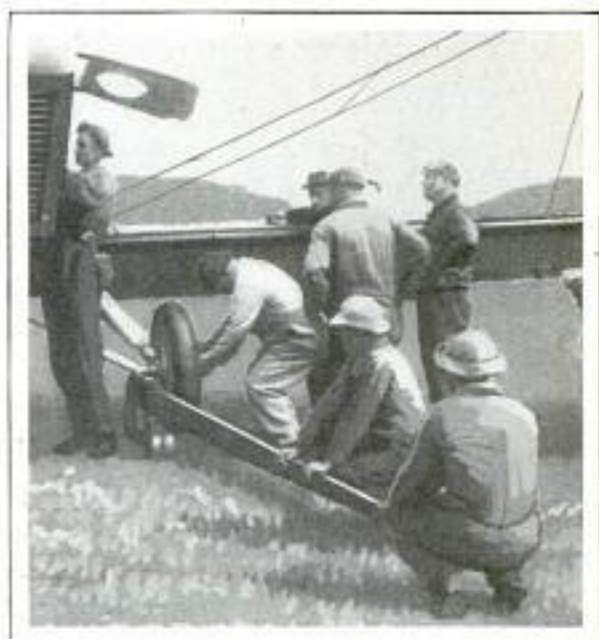
With This 12-ft. Level Jack Mounted on Casters, One Man Can Raise an Airplane
