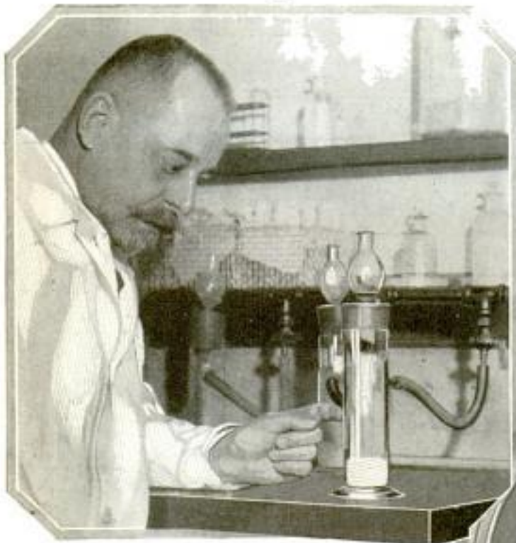
Vacuum Filter Used to Separate Bacteriophages from Bacteria; Right, Bacteria Being Destroyed
