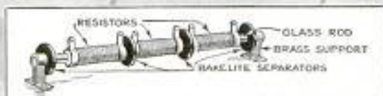
Tubular Resistors Make a Good Voltage Divider
