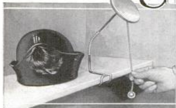
Hat Holder with a Spring for Use on High Shelf; a Slight Pull on the Cord Brings Hat and Holder within Easy Reach
