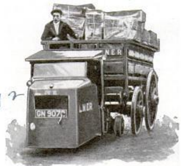
Compact Motor Unit Pulling Trailer; in Crowded Quarters It Is Easily Operated
