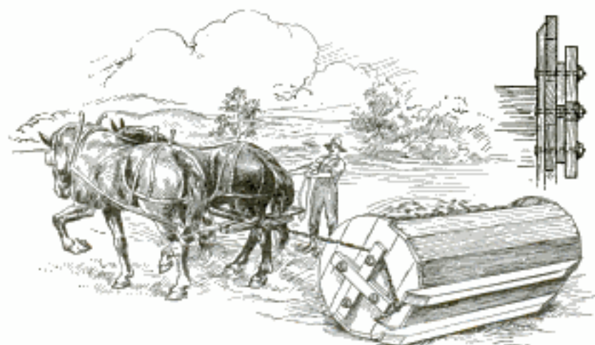
Dumping the Load Is No Job at All with a Stone Boat of Cylindrical Shape
