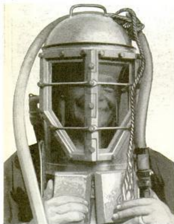
Diving Mask for Deep-Sea Work Filled with Synthetic Air to Decrease Time for Decompression
