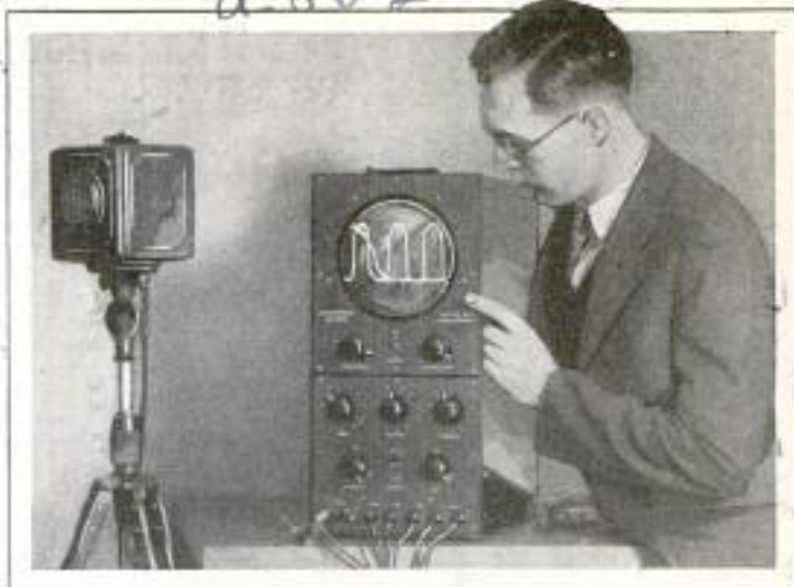
Apparatus Which Makes a Moving Picture of the Human Voice; on the Screen Is Shown the Image of One Voice
