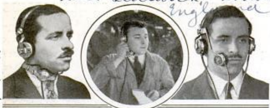
Telephone Receivers That Exclude Noise; the Transmitter Rests against Check or Throat and is Actuated by Vocal-Cord Vibrations
