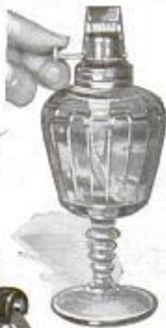
Right, Perfume Diffuser Operating through Oxidation to Disseminate Liquid in Base through Wick with Platinized Heating Element at Top
