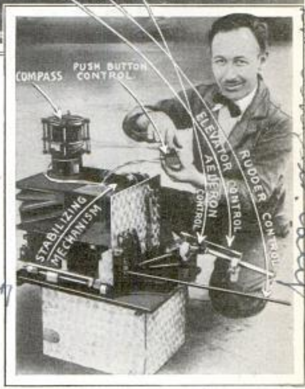
"Iron Skull" Which Pilots Plane in Flight; It Operates by Magnetic-Compass or Push-Button Control
