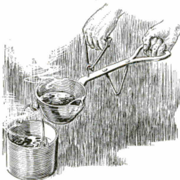
An Extra Rest, Spout and Two Hooks Make This Pouring Ladle Exceptionally Handy
