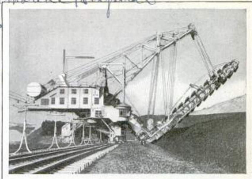
Giant Power Shovel Which Loads Cars in Germany; It Can Move More Than 850 Cubic Yards an Hour and Is Eighty Feet High
