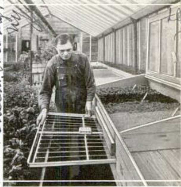
Sliding-Frame Electric Heater Which Slips under Hotbeds and Keeps the Soil and Plants Warm
