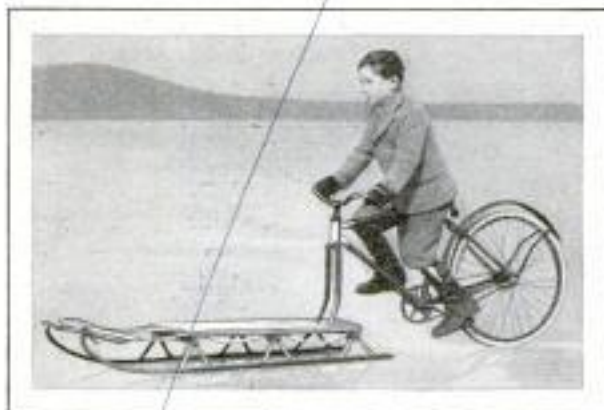
Bicycle and Sled Combined into One Vehicle for Travel on Ice by Twelve-Year-Old Inventor
