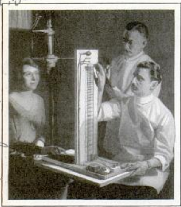
Apparatus Which Measures Time a Motorist Requires to Apply Brake after Seeing Red Light
