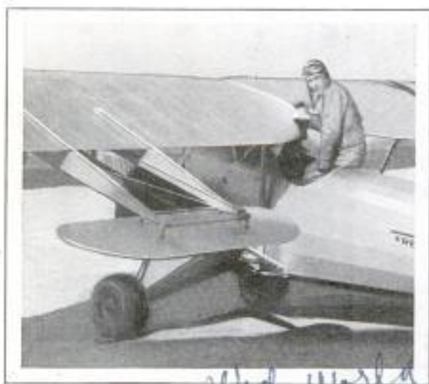
Airplane with "Free Suspension" Wings, Which Cause Ship to Assume Proper Landing Position
