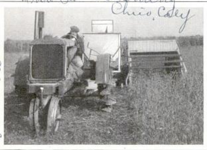
Combine Equipped with Wire-Brush Cylinder, Which Beats Out the Grain as the Straw Passes over the Brush; One Man Operates It
