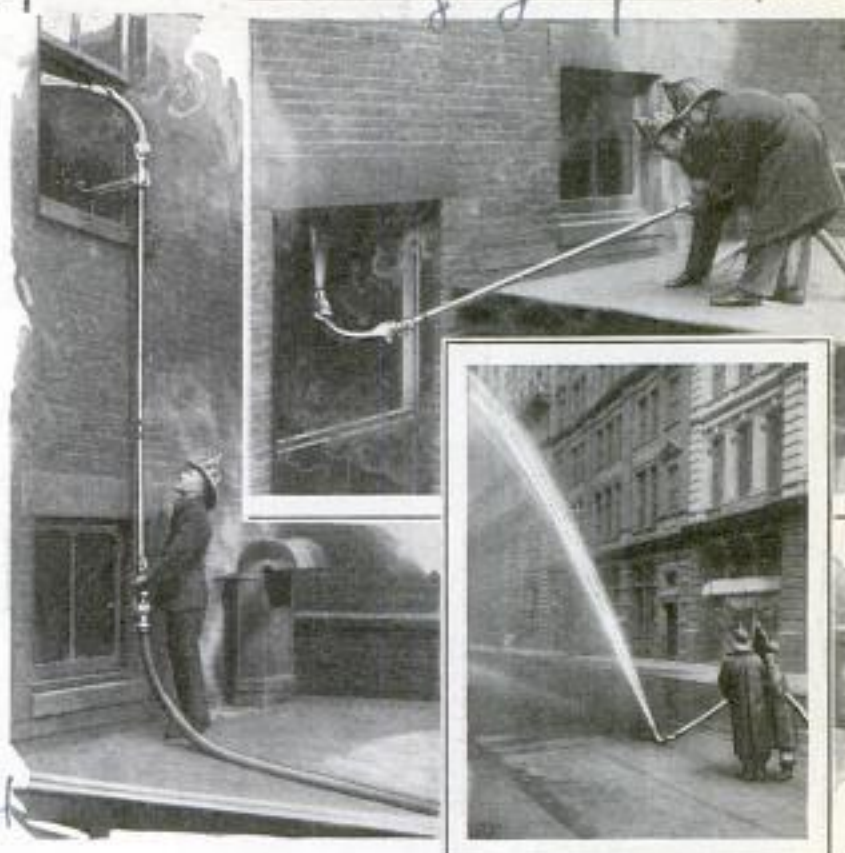
Various Applications of a Fire Hose with an Extension Nozzle, Capable of Making a Powerful Stream of Water Turn Corners
