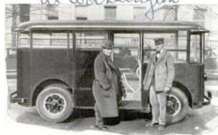
© U. & V. Mail Truck with Low Body and Doors on Each Side; the Unusual Vehicle Is Expected to Speed Up Collections
