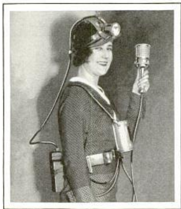
Electrical Tester Which Quickly Detects the Presence of Dangerous Gases in Coal Mines
