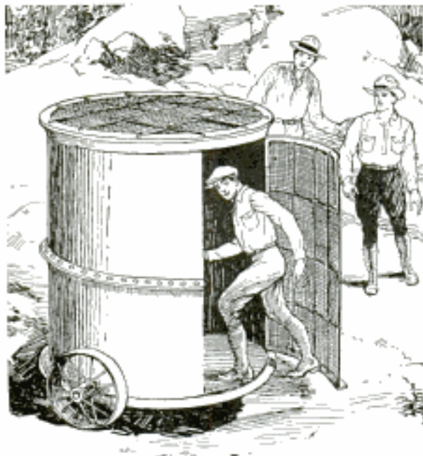
Wheeled Metal Tank Provides Shelter against Flying Stones and Dirt Thrown by Dynamite Blasts
