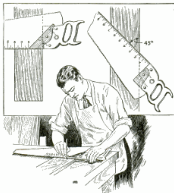
A Straight-Back Handsaw Can Be Improved by Equipping It with a Square, Bevel and Rule
