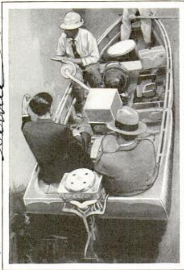
Outboard-Motor Boat Equipped with Power Blower Used to Dust Mosquito-Infested Waters
