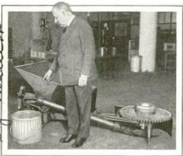
Furnace Stoker That Also Contains an "Ash Worm" Which Removes Contents of Pit Automatically
