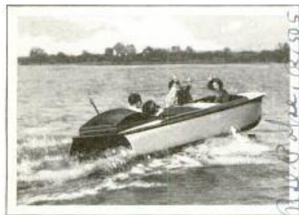
Inclosed Hatch over Outboard Motor Which Protects Engine and Gives Runabout Appearance
