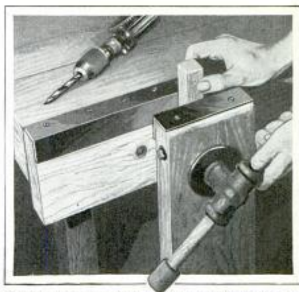
Woodworkers' Vise Can Be Greatly Strengthened by Fitting It with Angle-Iron Jaws
