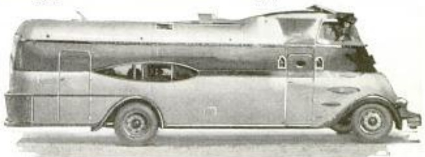
Giant Truck Containing a Complete Talking-Picture Projection Apparatus; the Vehicle Has Living Accommodations for Six Persons
