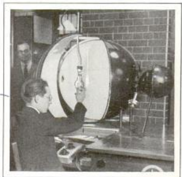
© Planet News, Ltd. Testing Brilliance of Electric-Light Bulbs in Cylinder with Aid of Photo-Electric Cell
