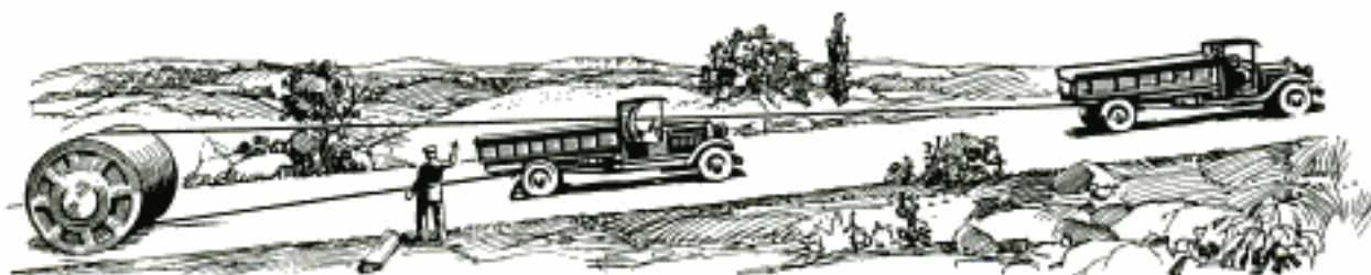
Moving Large and Heavy Circular Castings with the Use of Two Trucks and a Length of Steel Cable
