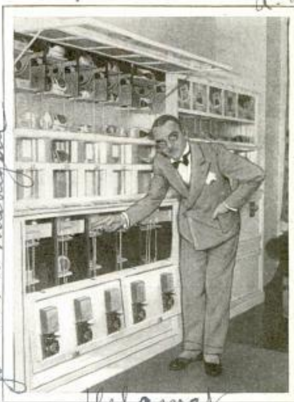
Automatic Grocery Where the Purchaser Inserts Coin in Slots to Obtain Any Article Desired
