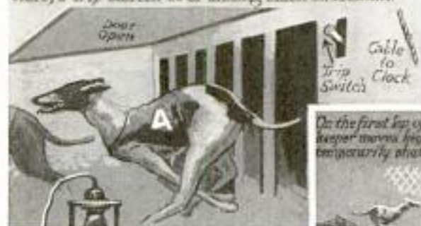
As the Door of the Trap flies open, starting the Race, a Trip Switch sets Timing Clock in Action.
