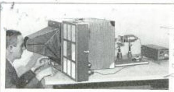
Measuring Fabric Fibers in Special Gauge Which Compares Their Size with Known Standards
