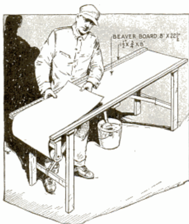
Paste Table Fitted with a Roller for Holding the Paper Makes Work Easier and Saves Time
