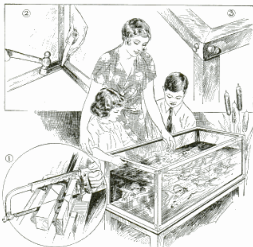
A Plate-Glass Aquarium with a Frame of Angle-Iron Will Accommodate a Large Number of Goldfish
