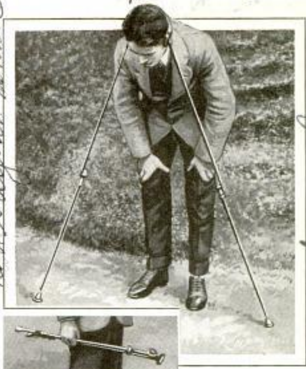
Elongated Stethoscope with Folding "Ears" That Is Used to Locate Leaks in Water Pipes
