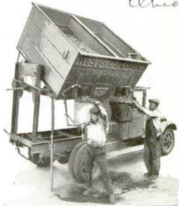
Coal-Truck Body Elevated and Tilted to Allow Loading of Bags through Chutes in the Sides
