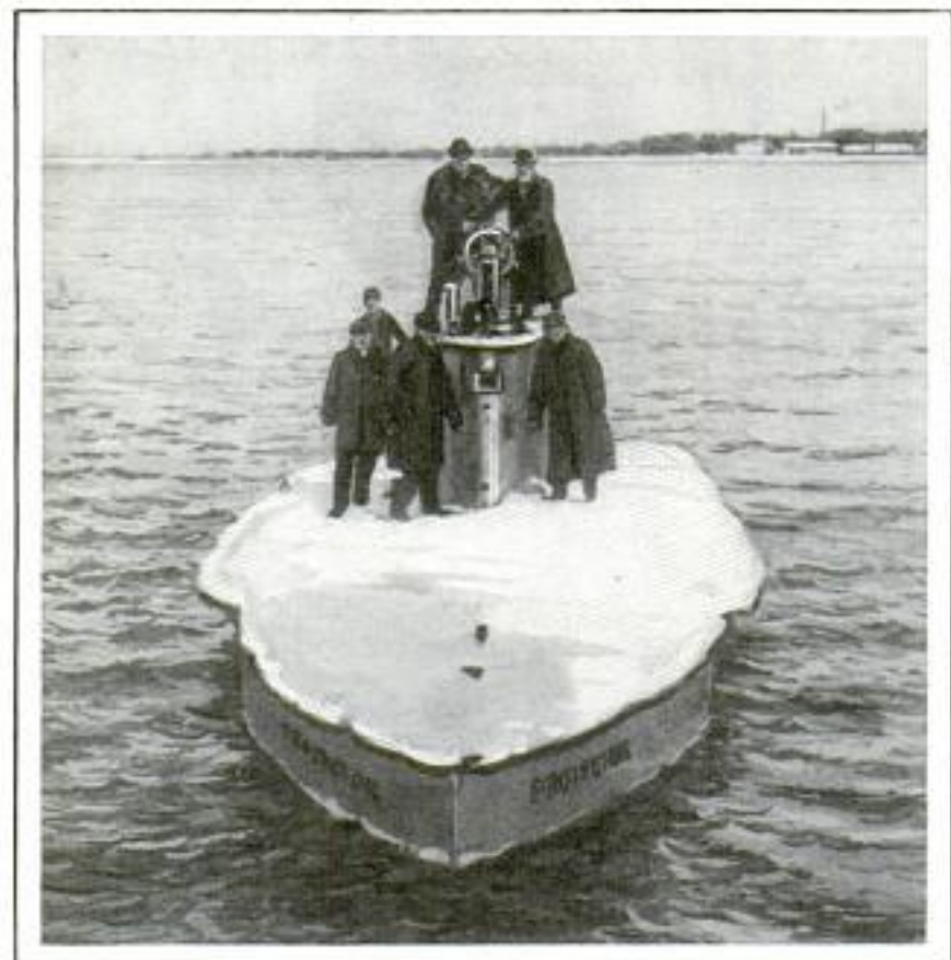
A Small Submarine Returning to Harbor after Demonstrating Its Ability to Break through Fields of Ice by Rising from Beneath Them
