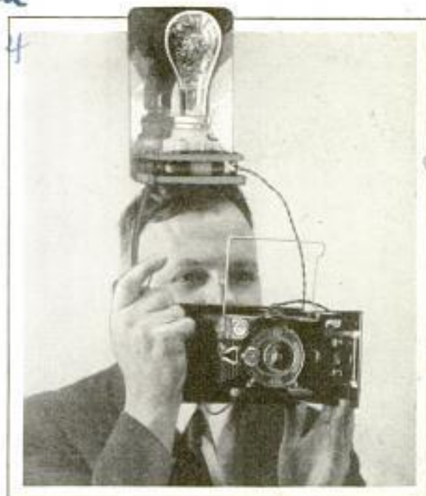
Headrest for Photo Flash Bulb and Battery; the Camera Shutter Sets Off the Flashlight
