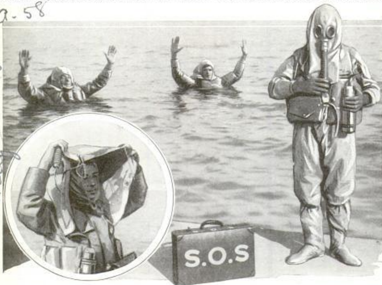
Testing the New Life-Saving Suit Which Permits the Wearer to Remain in an Upright Position While Floating; Note Breathing Equipment and the Hood That Completely Covers the Face
