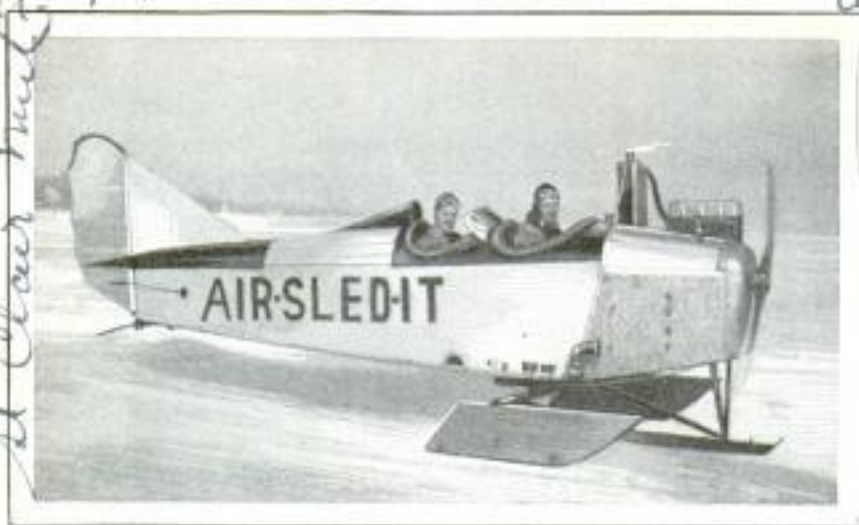
Fuselage of Wrecked Airplane Mounted on Runners and Powered by Airplane Motor; the Craft Makes Seventy-Five Miles an Hour
