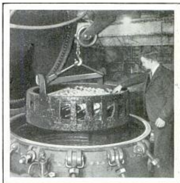
Preparing to Apply Solventless Varnish Insulation to Electric Equipment in Container
