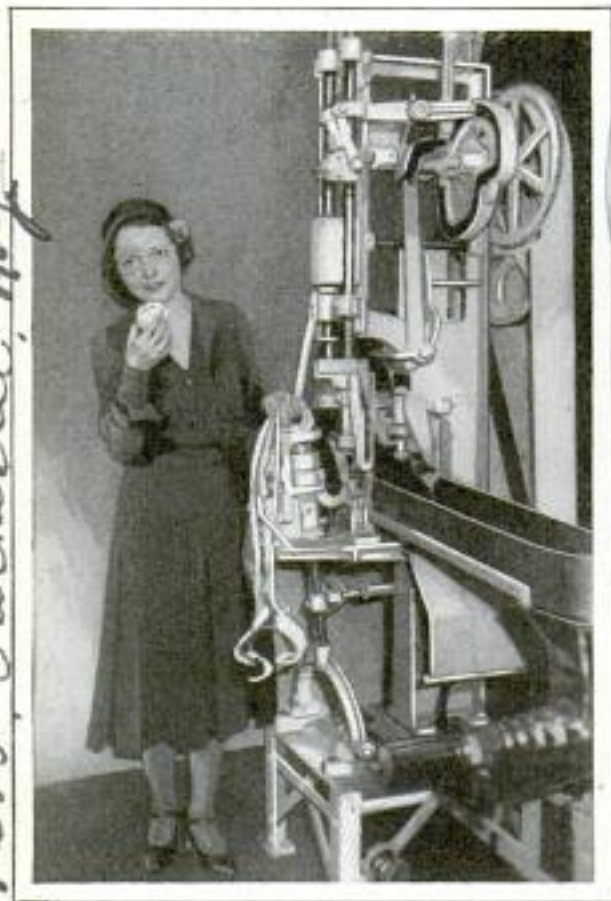
Orange-Peeling Machine That Removes the Skin without Injuring or Crushing the Pulp
