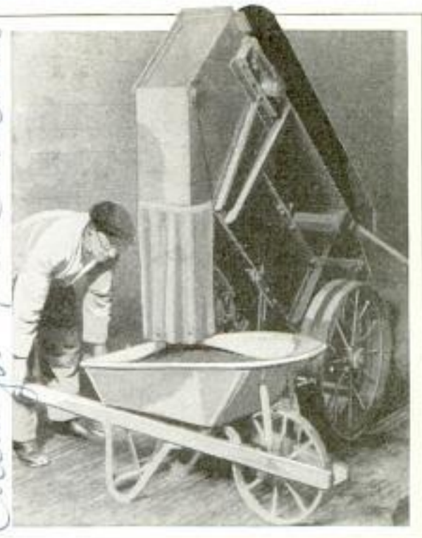
Electric Loader Which Handles Bulk Material; It Is Used to Empty Freight Cars Quickly
