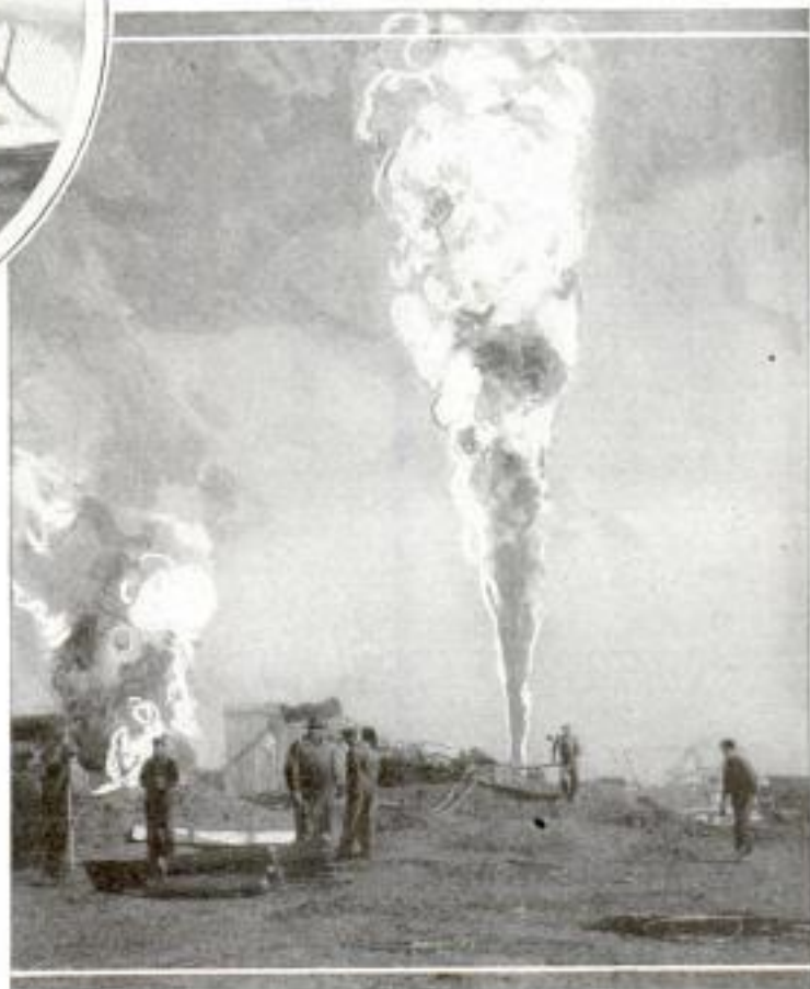
Pouring Water on Debris around "Wild Abe" from Behind Steel Screen, and Getting Ready to Shoot Out the Flame
