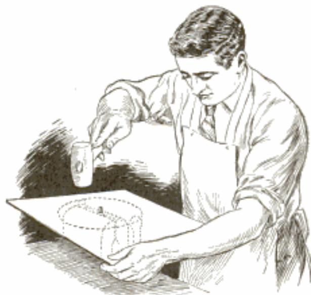
Vise, Hammer and Cold Chisel Are the Only Tools Required for Cutting Neat Sheet-Metal Disks
