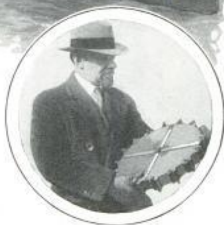
Upper Left, Submarine Fitted for Trip to Pole under the Ice; Note Framework Like Inverted Sled Runners for Ice Protection; Above, Ladder That Will Be Used by Diver; in Circle, the Ice-Cutting Disk
