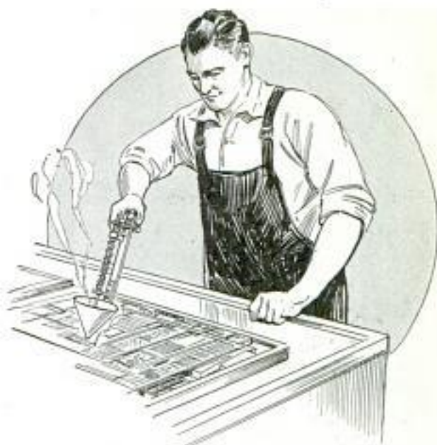
Self-Closing Funnel on Printers' Ladle Is Handy for Filling Irregular Spaces in Forms
