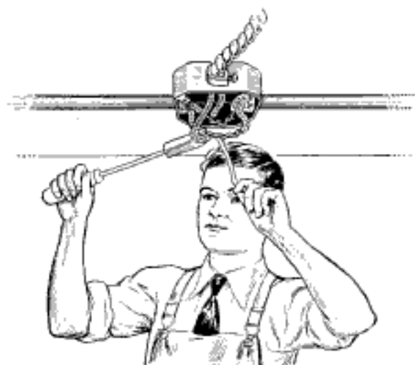
Soldering the Connections Is Important and Should Not Be Omitted for Any Reason
