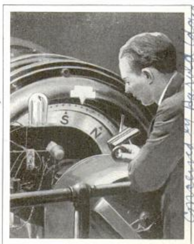
"Still" Picture of Machinery Moving at High Speed, Taken to Study the Parts in Motion
