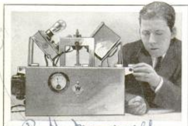
Sorting Machine Which Utilizes Electric Eye to Detect Packages of Yeast with Missing Labels
