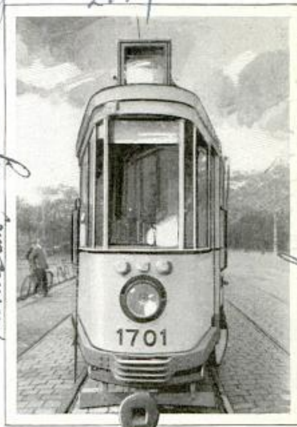
Streamlined Street Car Used in Germany to Attain Greater Speed; It Is Only Seven Feet Wide
