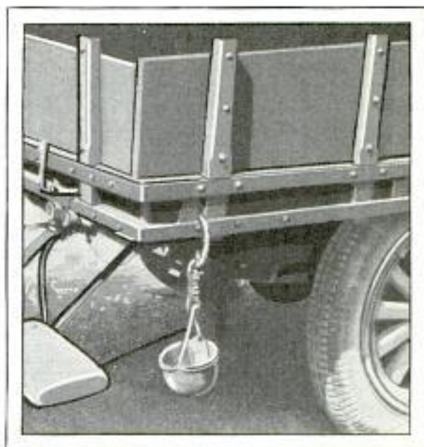
Double Harness Snap Suspended from Body of Truck Holds the Hot Pot Safely and Securely
