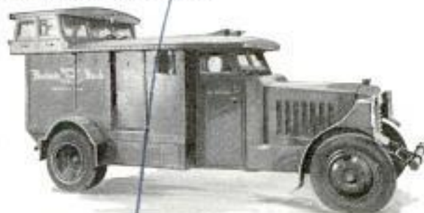
Armored Truck for Transporting Money and Securities; Note the Cupola That Serves as a Lookout
