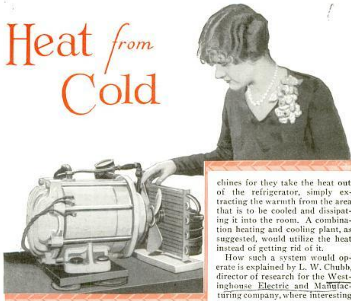
Units in an Electrical Refrigerator; Here Are Essentials for a Much Larger Outfit to Warm and Cool Homes and Offices.
