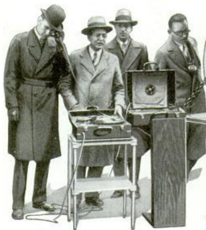
Investigators Analyzing Noises at Busy Intersection in New York City with the Noise Meter
