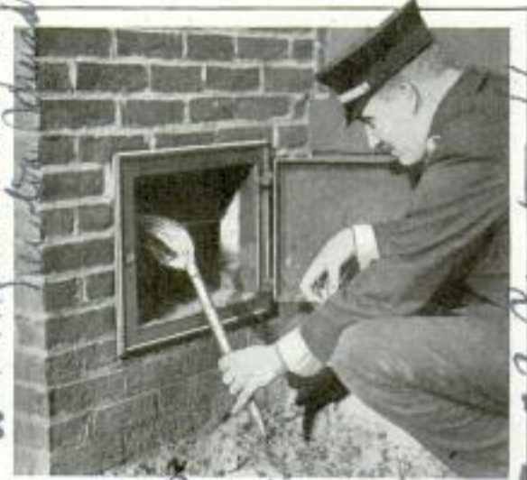
Fusee Which Generates Gases That Quickly Smother Chimney Fires or Other Inaccessible Blazes
