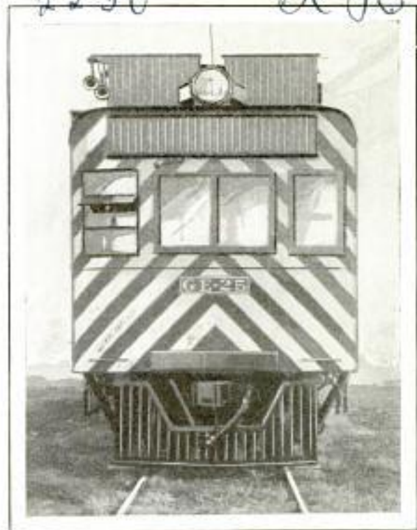
Gas-Electric Rail Car Painted in Stripes in Order to Be Visible at Greater Distances
