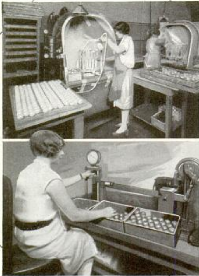
Spraying Balls with Paint and Measuring Them in Gauge to Test Resiliency before the Covers Are Put On
