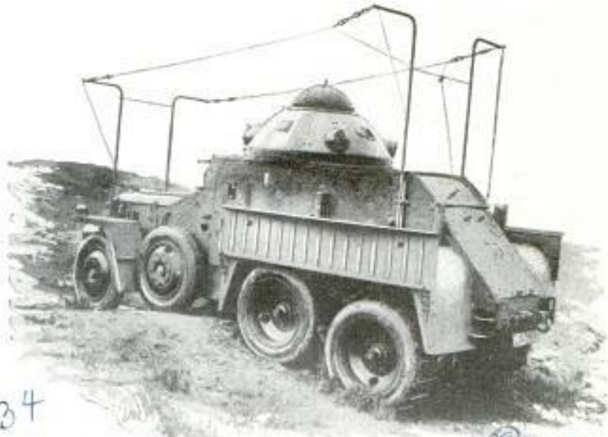
Eight-Wheeled Armored Tank Equipped with Wireless; Two of the Wheels Are Spares and Are Used Only in Traveling over Rough Ground
