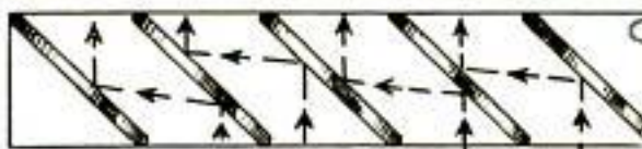
Front View of the Steel-Paneled Cage Window and Diagram Showing Position of Plates
