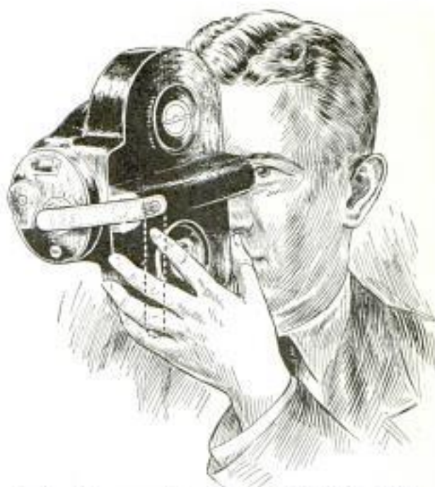
Leather Strap over Focusing Tube Tells Movie Operator That Lens Is Covered
