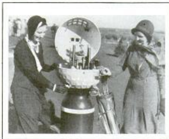
Slot Machine Which Lacquers and Dries Golf Ball When a Coin Is Deposited
