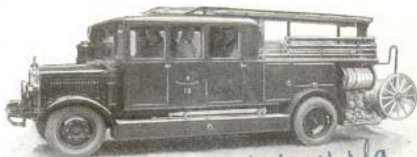
Inclosed Fire Wagon Used in Berlin; It Shields the Men from the Weather on the Way to and from Fires
