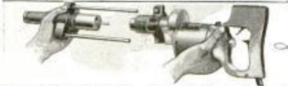
Lightweight Electric Handdrill, Which Is Equipped with Both Twist and Hammer Attachments
