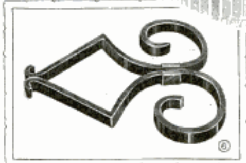
FIG. 7 U-FRAME FOR GATE, 1\frac{1}{2} " WROUGHT IRON, ONE REQUIRED
