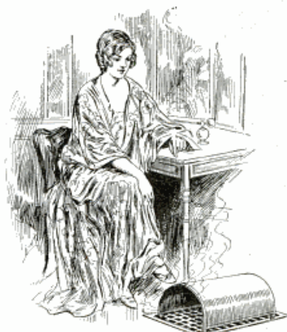
Heat of Pipeless Furnace Can Be Distributed More Evenly by a Sheet-Metal Hood
