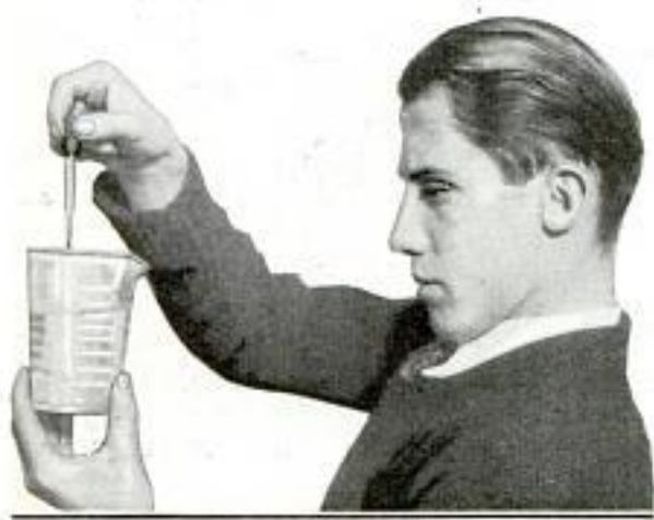
Accuracy in Mixing the Ingredients for the Silvering Solution Is Important
