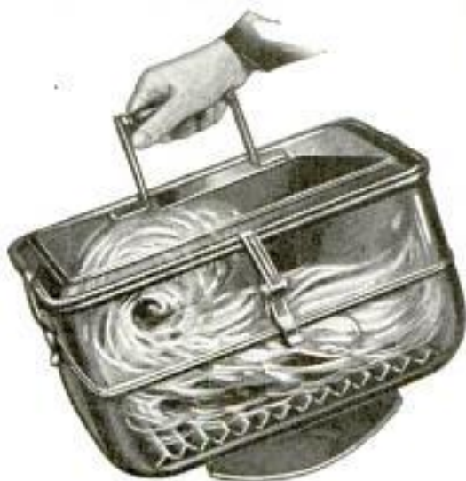
Efficient Unit for Dry-Cleaning Clothes at Home; It Rests on Rocker So That It Can Easily Be Tipped Back and Forth to Speed Cleaning; Corrugated Bottom Also Aids the Cleaning Operation
