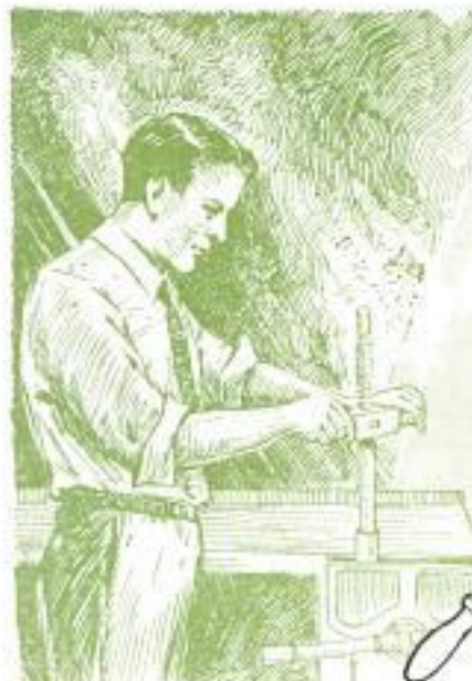
Above, Photo of Finished Candle Stand; Center, Assembly Drawing, and, Left, Threading the Post with the Screw Box before Finishing
