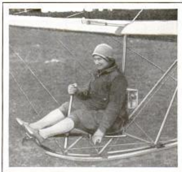
Buzzer Is behind Pilot, and Diaphragm, Operated by the Wind, above Her Head
