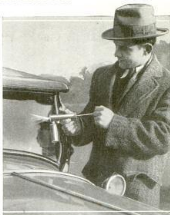
Spraying Auto Windshield with "Gun" Which Distributes Liquid Especially Effective in Removing Grease
