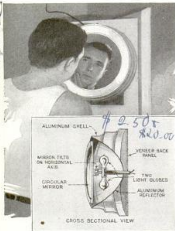
Mirror behind which are light bulbs and a reflector that illuminate objects in front of it
