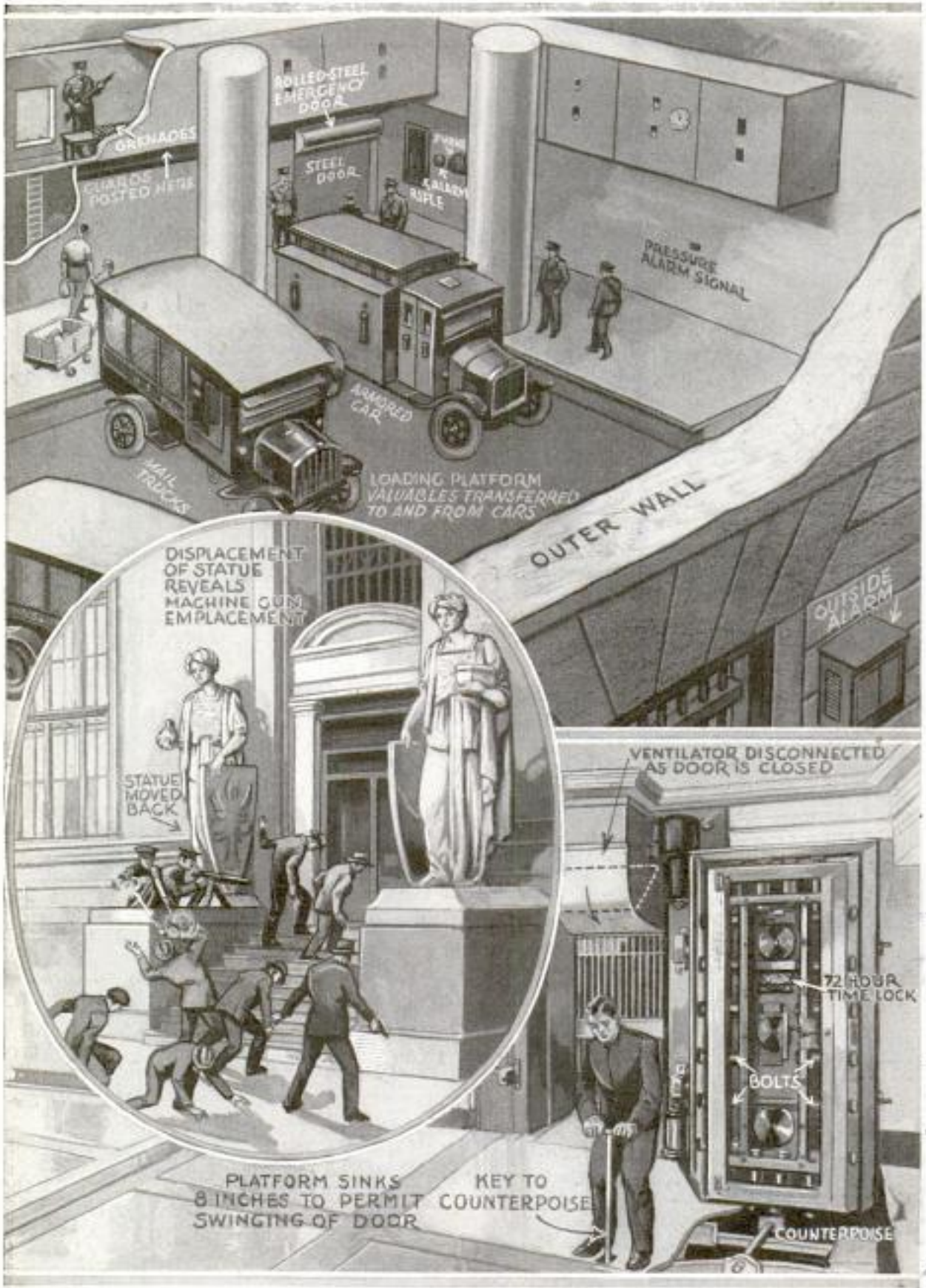
Loading Platform at a Reserve Bank Showing Cage for Guards; Inset, Statues That Move Back to Expose Machine Guns and Vault with Twenty-Five-Ton Door and Floor That Rises and Sinks
