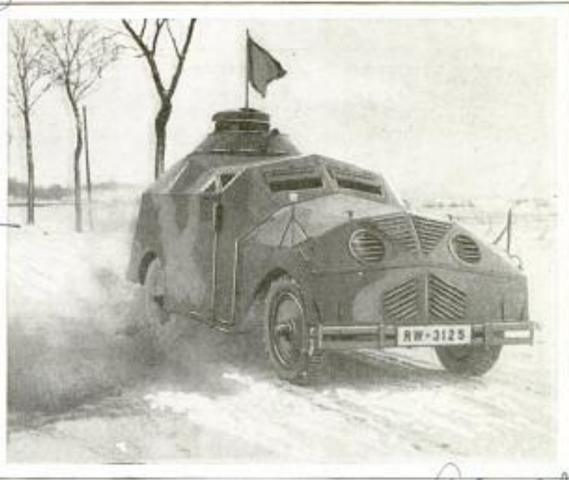
Small and Speedy Armored Tank Employed in German Army Maneuvers; Note the Cupola for Gunners and the Shield over Radiator
