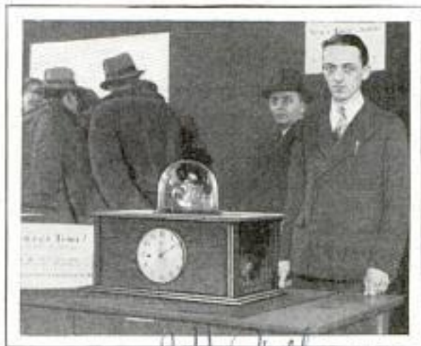
© Acme—P. & A. J. H. Colleman Clock Controlled by Vibrating Crystal Which Has Error Ratio of One Second in 100 Days
