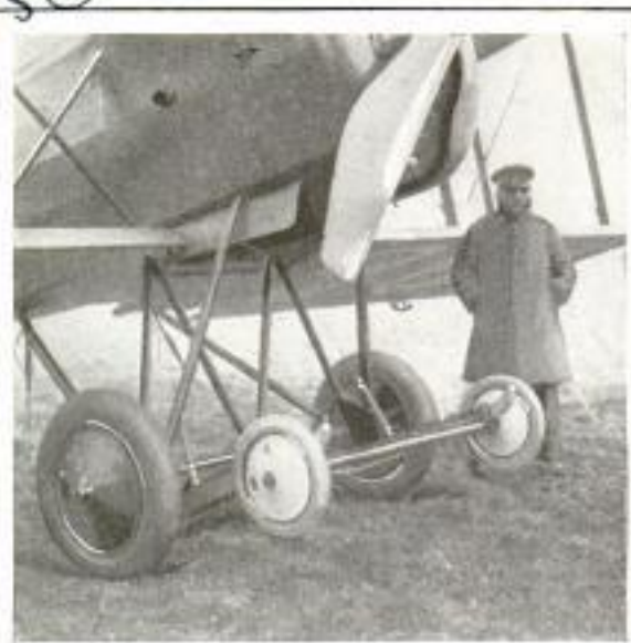
Auxiliary Landing Wheels Which Prevent a Plane Nosing Over if Tail Is Elevated Too Much
