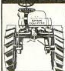
Rear view shows new HIGH ARCH which enables tractor to clear tall corn, cultivating 1 to 2 rows at one time.
