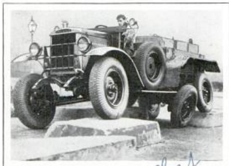
The Wheels of This Truck Accommodate Themselves to Uneven Road Surfaces While the Body Remains Always Level
