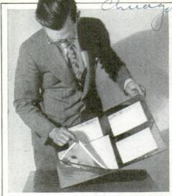
Squeegee Plates, for Drying Glossy Prints, Coated with Chromium for Greater Durability
