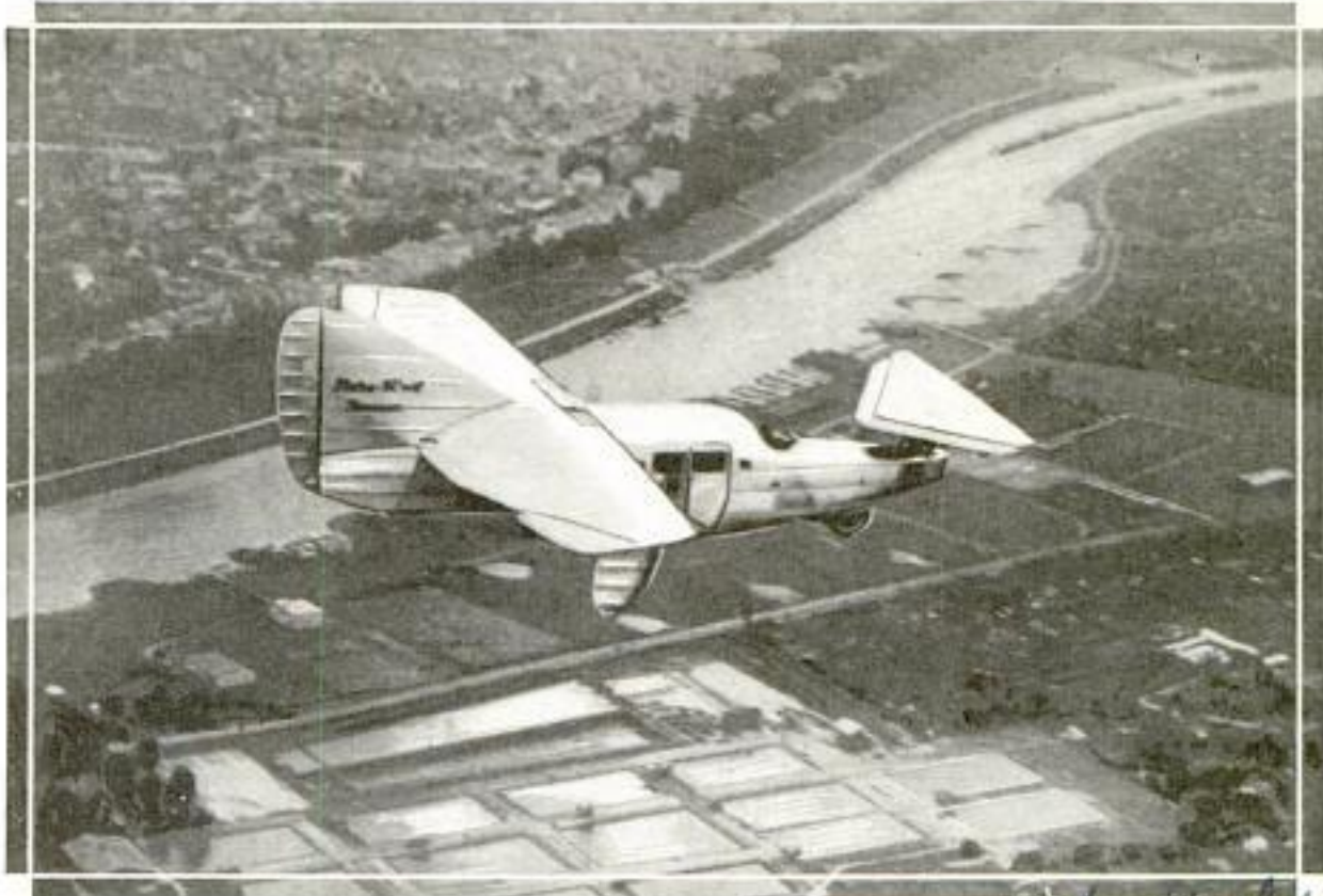
Airplane with Wing and Vertical Rudder in the Rear and Elevators in Front; Its Odd Design Gives It the Appearance of Flying Backward; the Ship Has Several Unusual Safety Features
