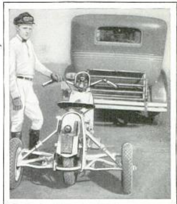
Motorcycle with Two Auxiliary Wheels, Which, When Lowered, Allow Towing behind Auto
