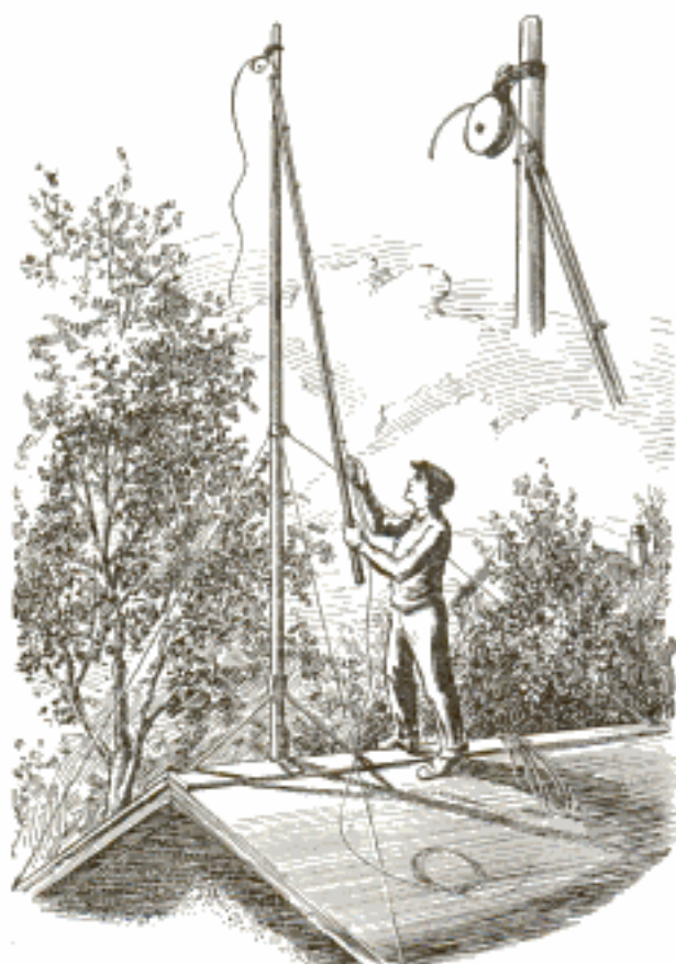
How the Wire Is Threaded through the Pulley to Raise the Fallen Antenna
