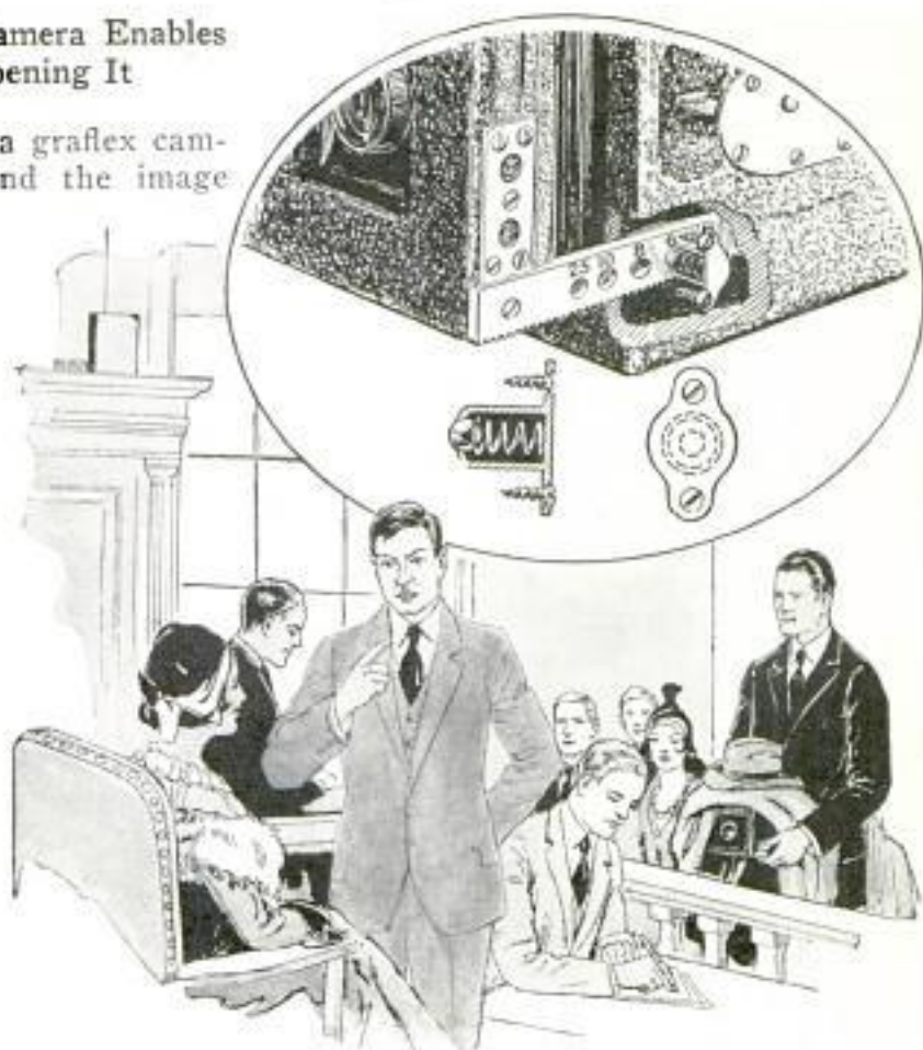
Attachment on Graflex Camera Permits User to Put It in Focus without the Trouble of Opening It
