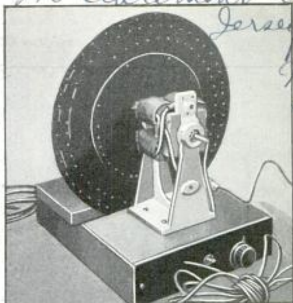
View of Completed Televisor from the Front, but without the Magnifying Lens
