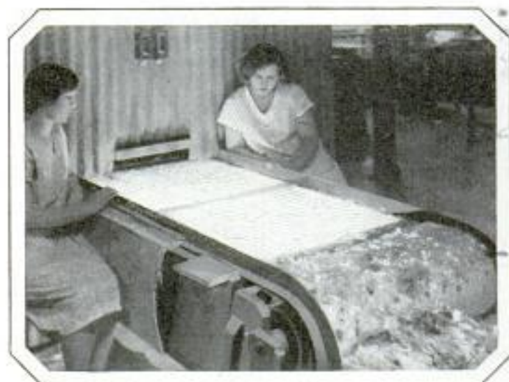
Inspecting Mica Which Is Moving on a Translucent Belt with Electric Light beneath It
