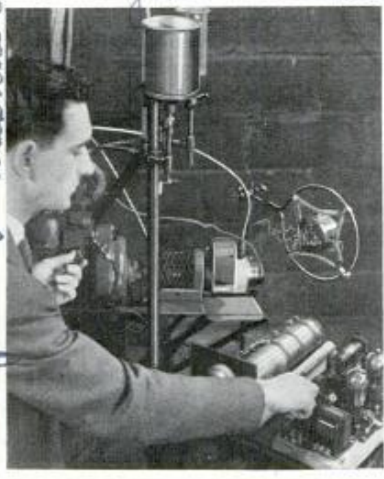
Using the Electric "Ear" to Test a Motor: It Picks Up the Knock but Cuts Out Other Noise
