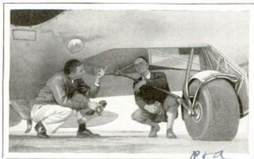
Retracting Landing Gear and Wing Developed for Colonel Lindbergh's Plane; the Wheel Folds into the Recess in Underside of Wing
