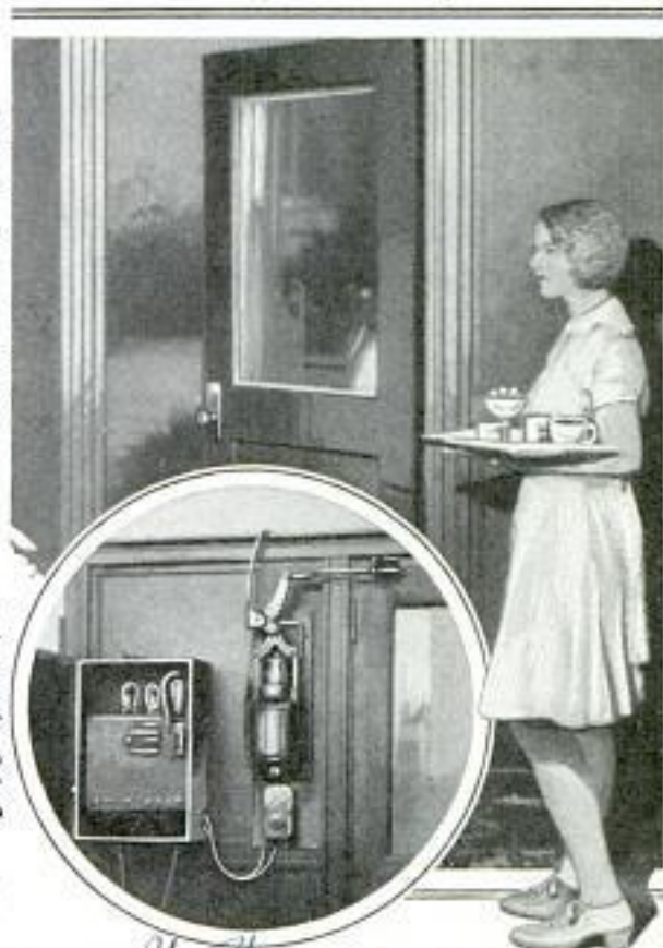
Door That Is Opened by Electric Eye When Approached, and Apparatus Which Operates It
