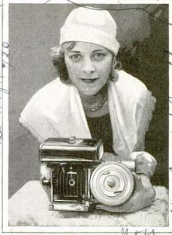
Tiny Air-Cooled Gasoline Motor, Weighing Eleven Pounds and Developing One Horsepower
