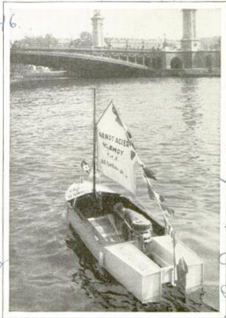
Small All-Steel Boat That Will Not Sink and Can Be Taken Apart Easily; Air-Filled Caissons Support It
