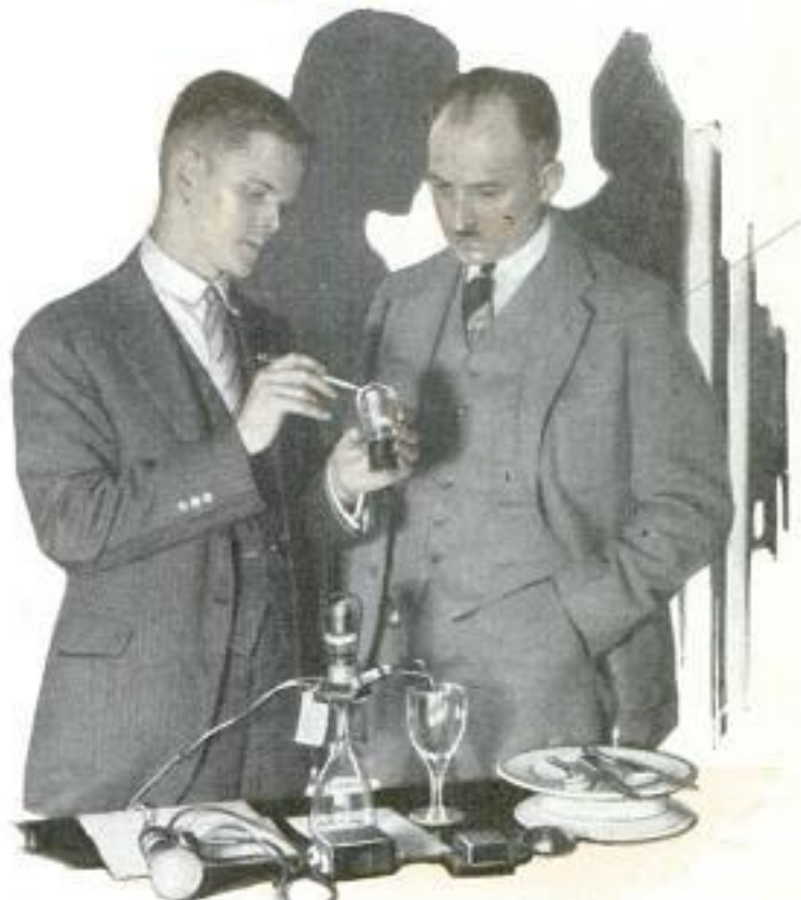
The Grid Glow Tube. Resembling an Ordinary Radio Tube, but Capable of Magnifying Energy 100,000,000 Times
