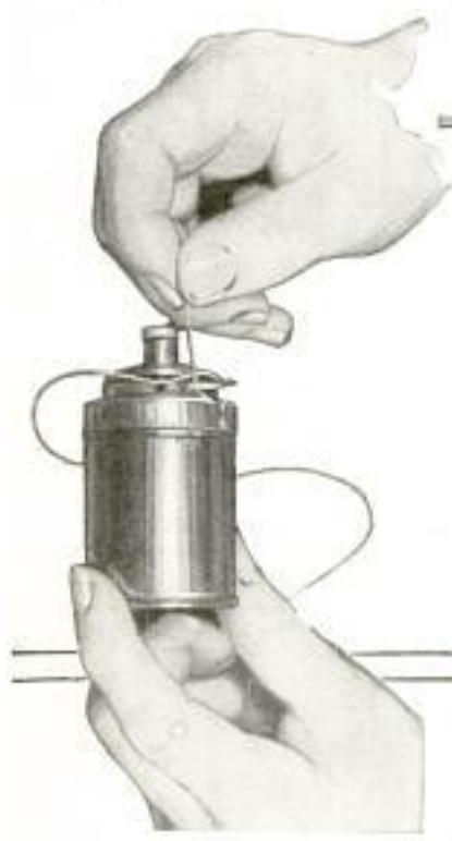
Needles Can Be Threaded in the Dark with This Holder That Has Metal Prong
