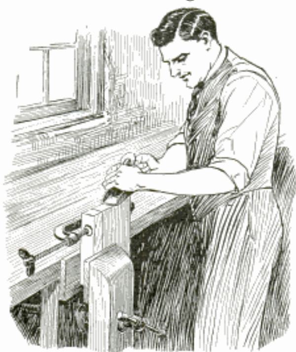
Small Block of Wood, Clamped to Piece to Be Butt-Planed, Prevents Splitting
