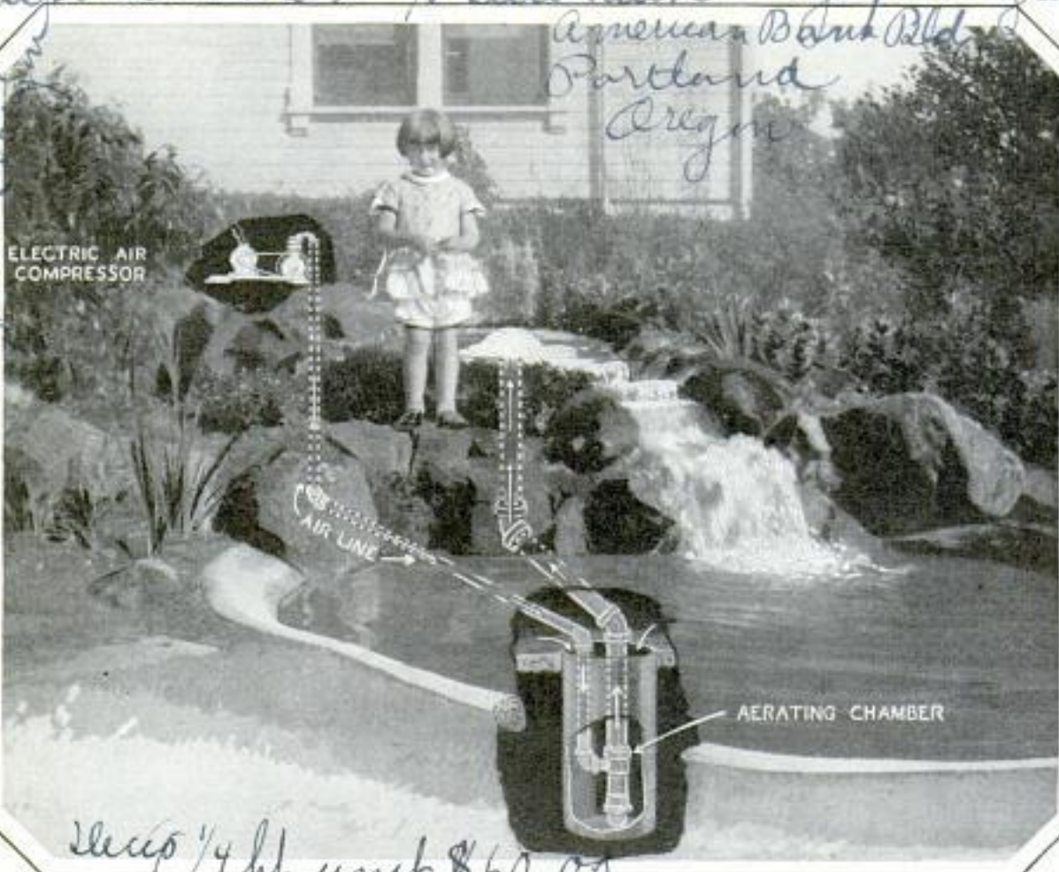
Artificial Waterfall Produced by an Altered-Gravity Pump and Air Compressor; the Diagram Shows How the Pump Aerates and Lightens the Water, Thus Forcing It to Lift Itself
