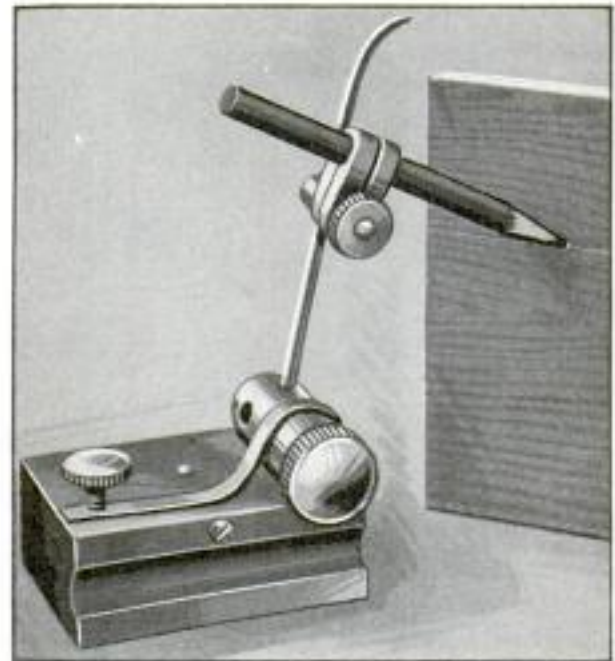
Using a Pencil in the Spindle Hole of a Scriber for Marking Wood
