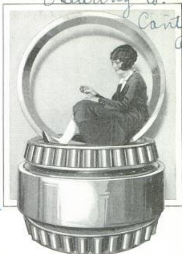
Big Roller Bearing for Steel-Plate Mill; the Girl Holds a Small Bearing for Comparison
