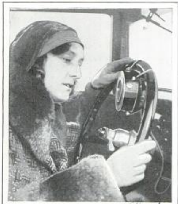
Microphone for the Motorist Enabling the Driver to Use His Voice to Supplement the Horn
