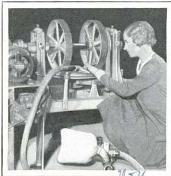
© U. & V. Machine Employed by the Bureau of Standards to Test the Wearing Qualities of Carpets
