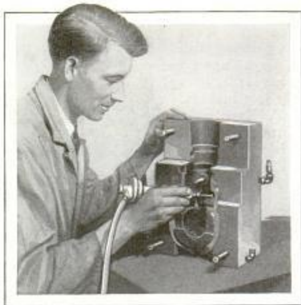
Tiny Grinding Tool, Powered by Compressed Air, and So Small It Is Used Like a Fountain Pen
