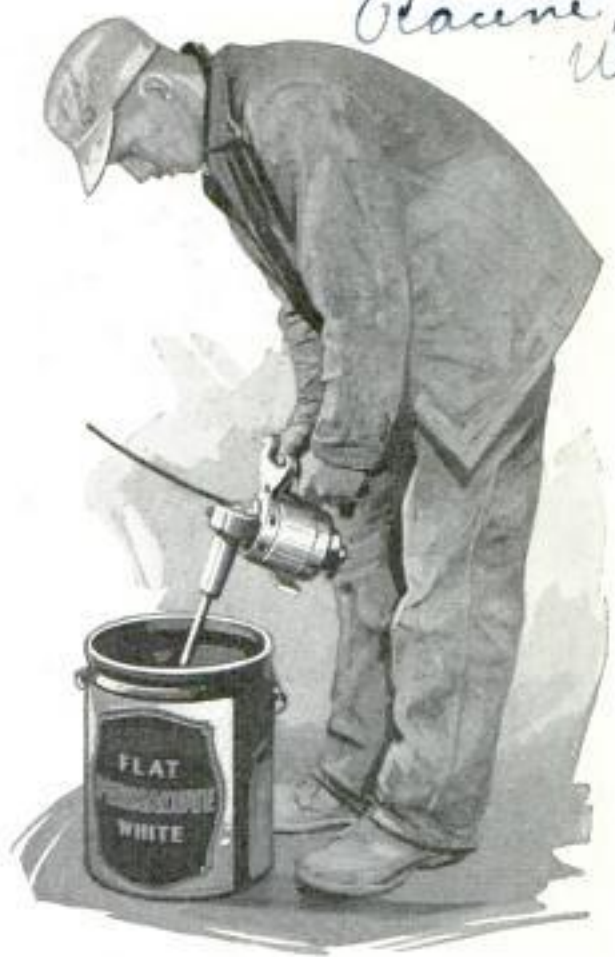
Portable Electric Paint Mixer That Stirs a Five-Gallon Can of Paint in a Few Seconds
