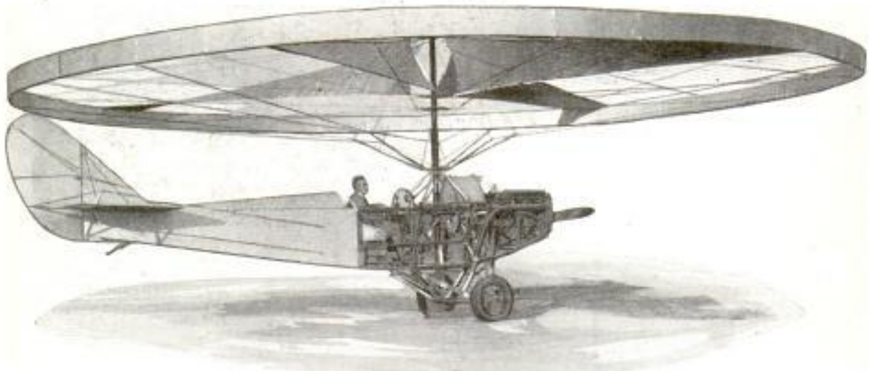
Airplane with Whirling Wings That Are Expected to Act as a Balancing Gyroscope and Lifting Propeller, and Also to Serve as a Sort of Parachute for Descending
