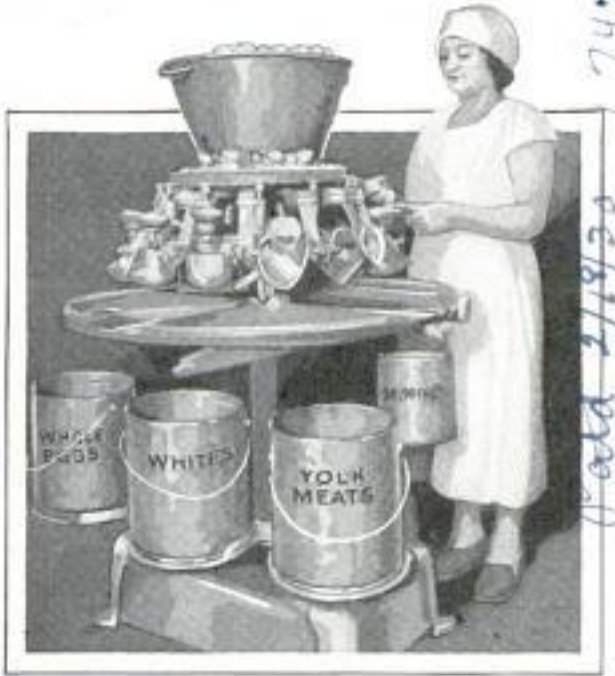
Egg Separator That Sorts Whites and Yolks at the Rate of More Than Sixty a Minute
