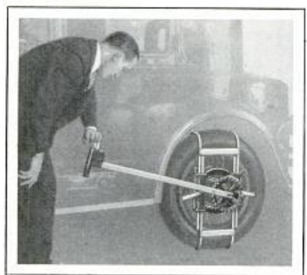
One-Man Brake Tester Which Indicates Defects on a Gauge When Applied to Auto Wheel
