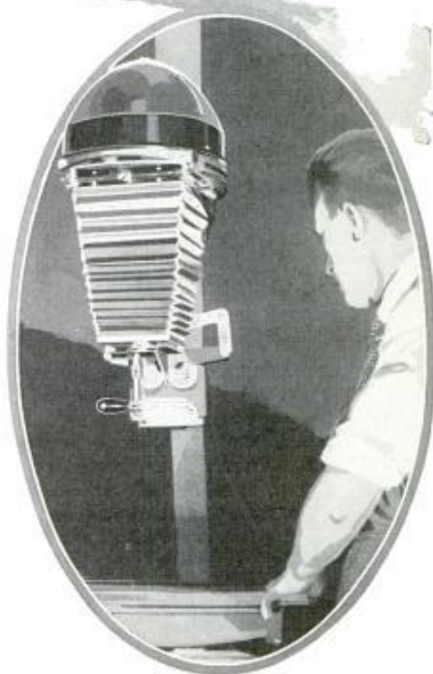
A Copying Camera Which Is In General Use by Police Bureaus for Duplicating Important Records
