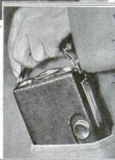
Electrically Operated Pocket Projector. Accommodating 250 Still Pictures, Which Is Ready to Operate When Plugged into Light Socket
