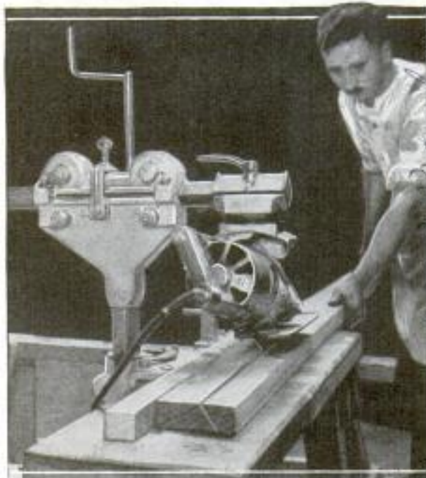
Radial Arm for Electric Handsaw Which Converts a Portable Outfit into a Handy Bench Unit
