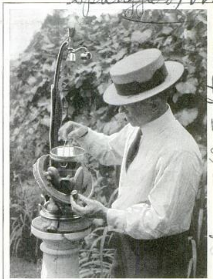
Combination Sundial and Telescope, Showing the Mirror and the Adjustable Eyepiece to the Left of the Man's Hat
