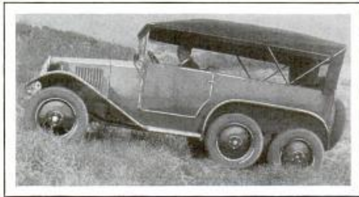
Six-Wheeled Auto for Traveling Rough Ground; It Has Five Axles, Eight Forward Speeds and Four Reverse
