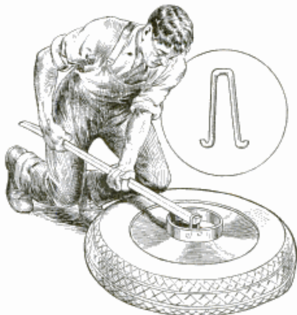
U-Shaped Hook and a Pinch Bar Are Used to Pull a Wheel Bushing
