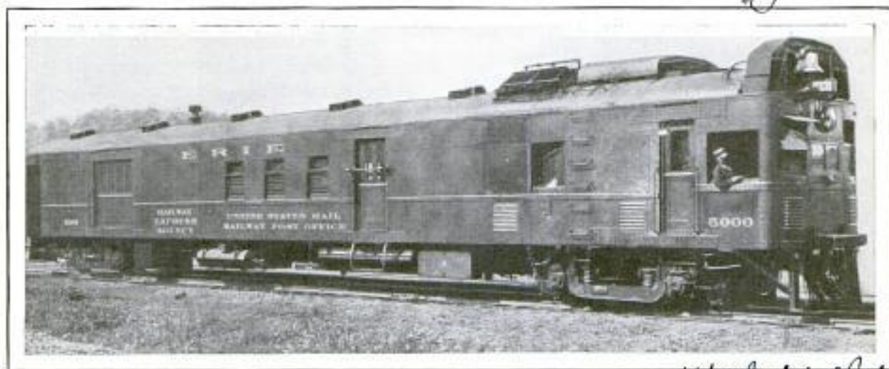
Oil-Electric Railway Car Which Operates under Its Own Power Supplied by Motors and Generators in Forward Compartment; It Can Travel at Eighty-Five Miles an Hour
