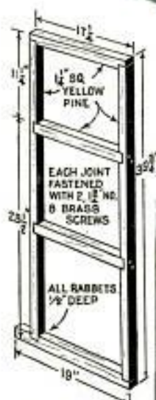
FIG. 1 SHOWING CONSTRUCTION OF REAR CABIN FRAME
