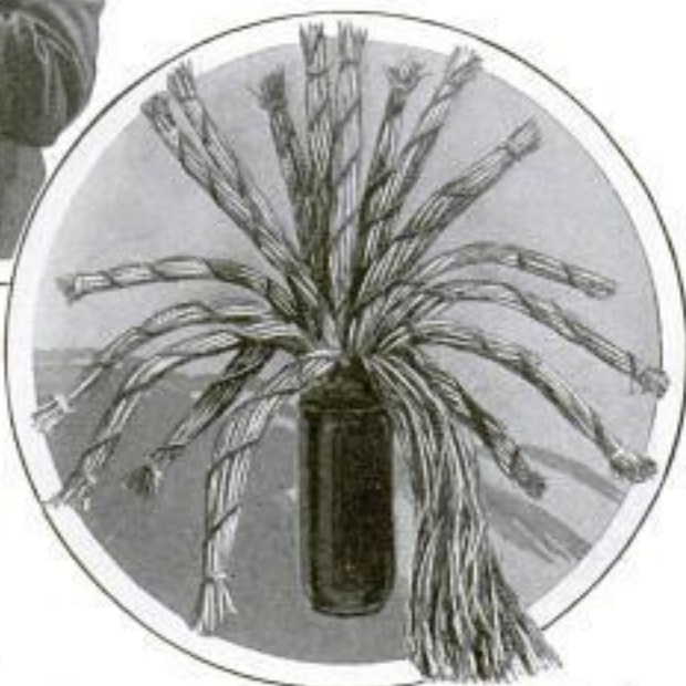
Using the Artificial Larynx, and End of New Ocean Cable Which Contains 3,600 Wires
