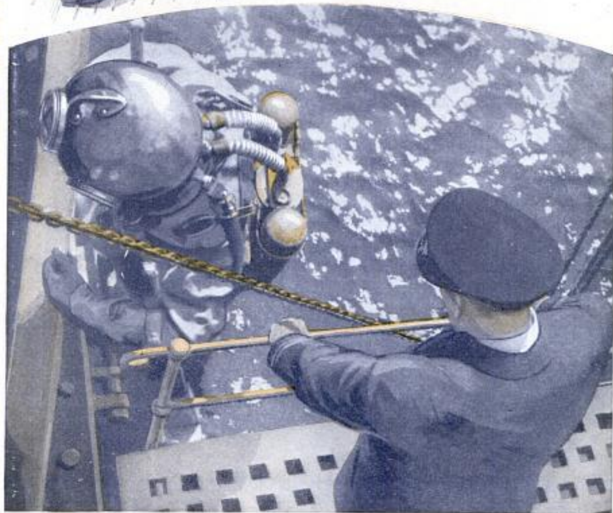
Making Final Preparations for a Descent, and, Below, Going down the Ladder with His Emergency Oxygen Outfit on His Back; Extra Tanks Such as This Add More Weight, but This Is Not an Objectionable Feature for Extra Weights Are Needed at Great Depths, and the Oxygen Container Serves a Double Purpose
