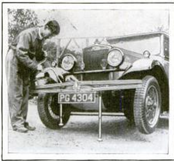
Permanent Jacks, Installed on Auto and Operated by a Crank, Save Time in Making Tire Changes
