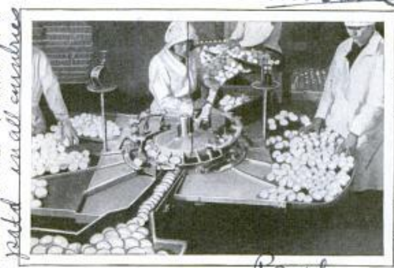
Sorter and Candler Which Automatically Tests Eggs, Weighs Them and Distributes Them into Five Different Grades
