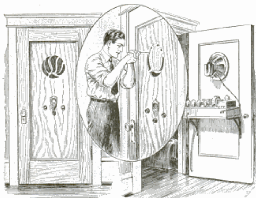
Right, Rear View Showing Method of Mounting Receiver and Speaker; Center, Cutting Speaker Grill with Hacksaw; Left, Completed Installation
