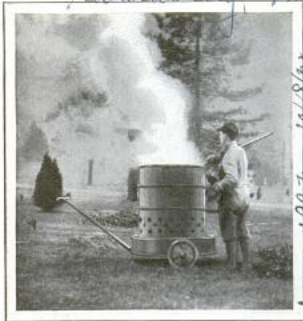
Portable Trash Burner in Which Leaves Can Be Destroyed without Doing Damage to the Lawn
