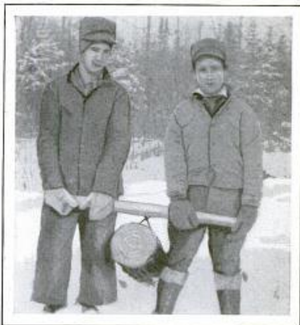
This "Choker," Which Takes the Place of Lug Hooks, Makes It Easy to Drag Logs
