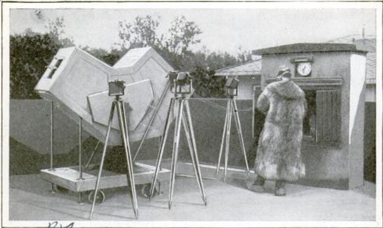
Spectrograph Apparatus at Northern Lights Observatory at Tromsø, Norway, Which Splits the Colors of the Northern Lights so That This Phenomenon Can Be Subjected to Study
