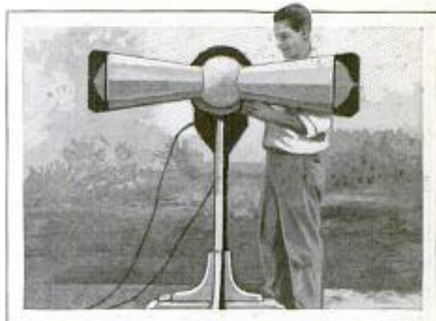
Dynamic Speaker with Double Air Column for Directional Public Address
