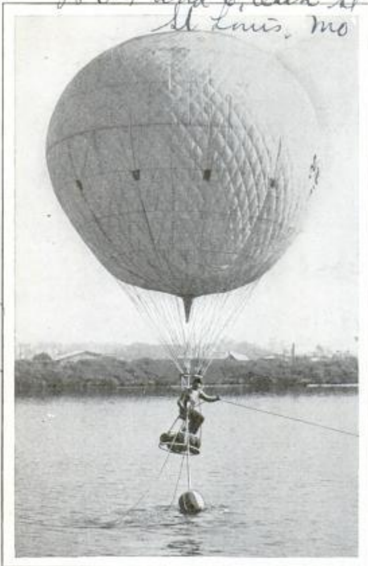
Jumping Balloon Whose Buoyancy Counterbalances Weight of Occupant, Allowing Him to Leap for Great Distances
