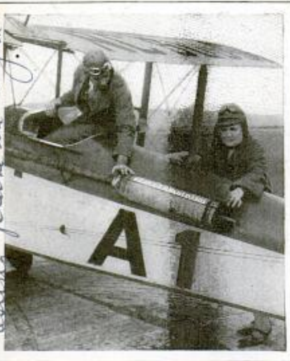
Muffler for Airplane Motor, Which "Chews Up" Sound Waves from Engine and Deadens the Noise
