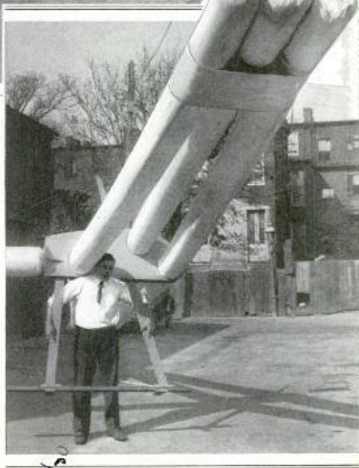
Rubber Airplane with Wings, Tail and Fuselage Made of Inflated Rubber Tubing; Note, at Right, That One Man Can Lift It
