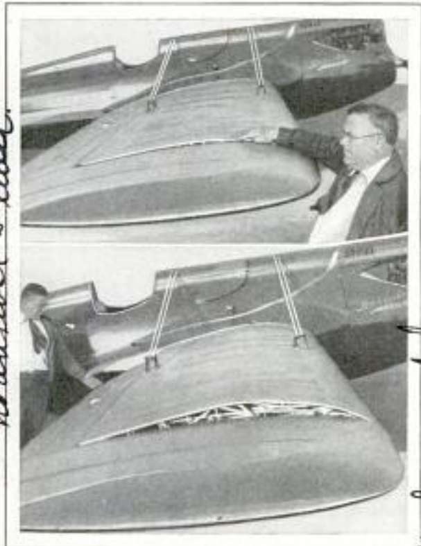
Adjustable Airplane Wing Whose Thickness May Be Altered to Increase Speed or Lifting Power
