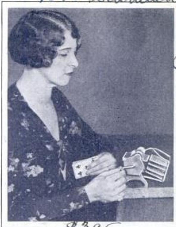
Card Shuffler Which Mixes the Pack and Deals Four Hands of Bridge in Twenty Seconds
