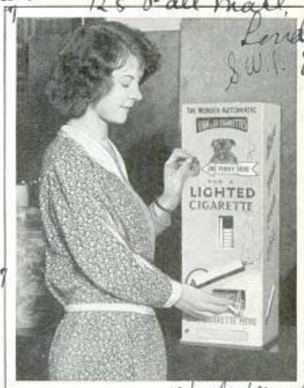
Removing Lighted Cigaret from the Coin-in-Slot Dispenser; the "Smoke" Is Ready in Five Seconds
