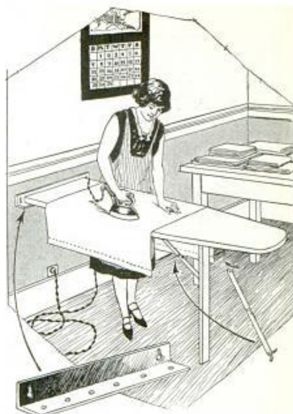
Angle-Iron Bracket on End of Ironing Board Hooks on Screws in the Wall
