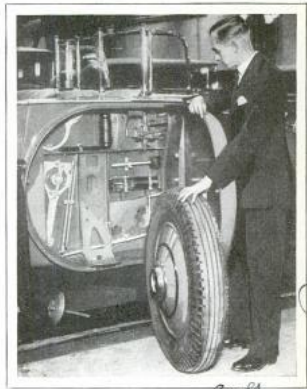
Tool Chest Built into Body of Auto; the Spare-Tire Rack over It Makes It Invisible
