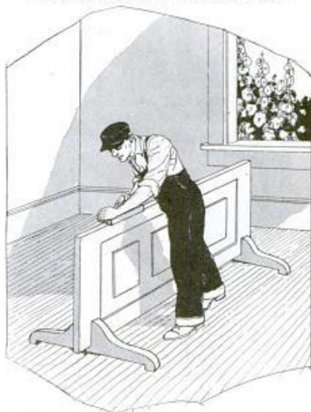
Weight of Door, When Placed in These Brackets, Causes Them to Grip It Tightly
