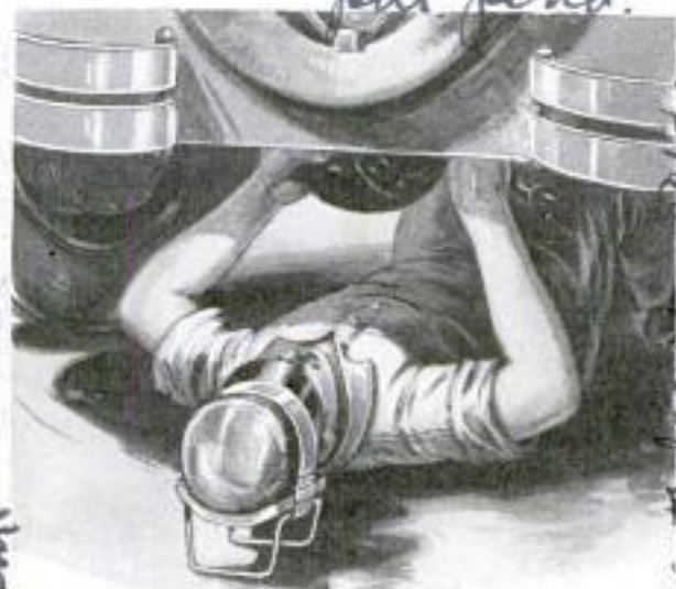
Work under the Automobile Can Be Done in Greater Comfort by Using the Headrest Shown
