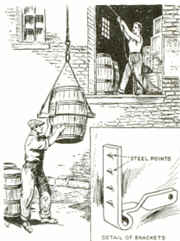
Pointed Brackets, Pivoting on Ring, Make a Quick and Efficient Barrel Hoist
