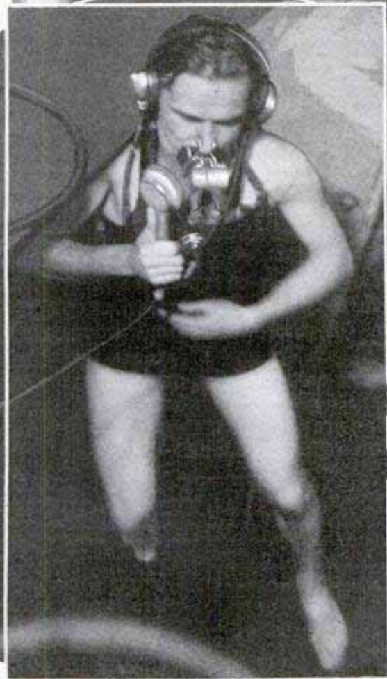
Above, Remarkable Photograph of Diver in Action, Using the Batteryless Telephone, and, at Right, Pose to Show How Instrument Would Be Used in Actual Operation; Man on Left Is Communicating with the Diver; the Line Is a Combination Lifeline and Telephone Cable, and Voice Is Amplified through Special System That Gives the Effect of a Loud Speaker
