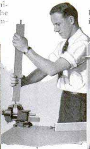
Center, Screwing Bolt into End of Crosspiece; Left, Table Assembled, Showing Fastening of Top Pieces; Right, Table with Drawing-Board Top in Place
