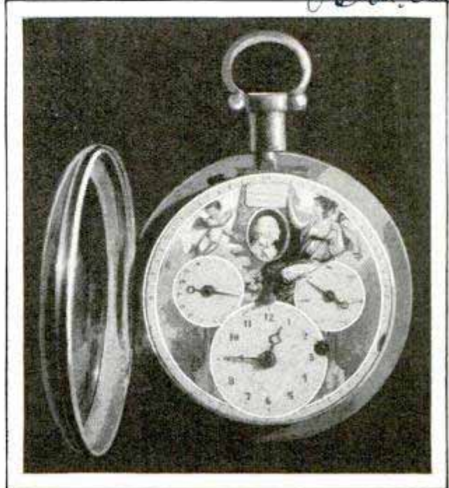
Old Watch with Four Dials and Five Hands; It Shows Days of the Week and Date of the Month
