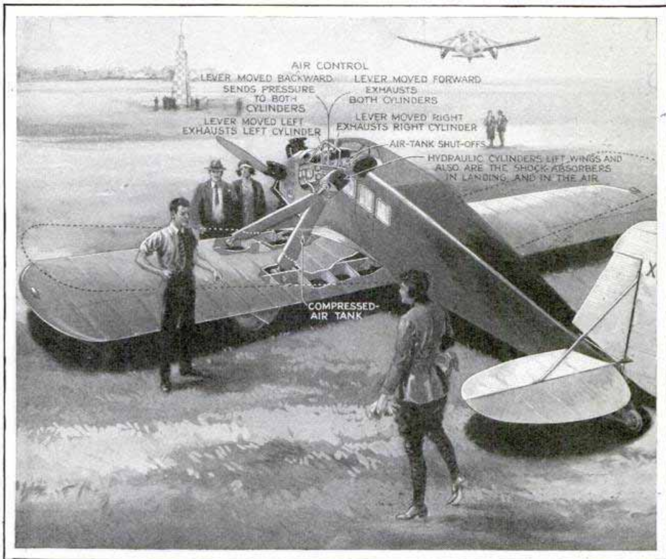
Variable-Wing Monoplane Which Depends on Compressed Air to Alter the Angle of Incidence of the Wings; Hydraulic Cylinders Which Lift the Wings Serve as Shock Absorbers in Landing
