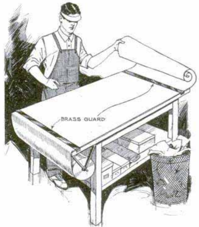
Roll of Kraft Paper Makes It Easy to Keep the Bench Cover Clean
