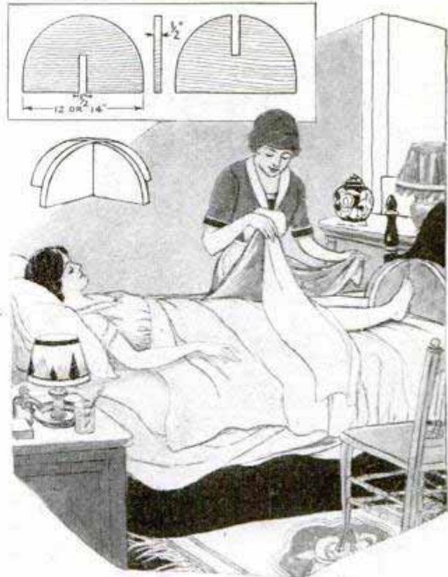
Bed Covers Can Be Kept off Injured and Tired Feet with This Wooden Frame
