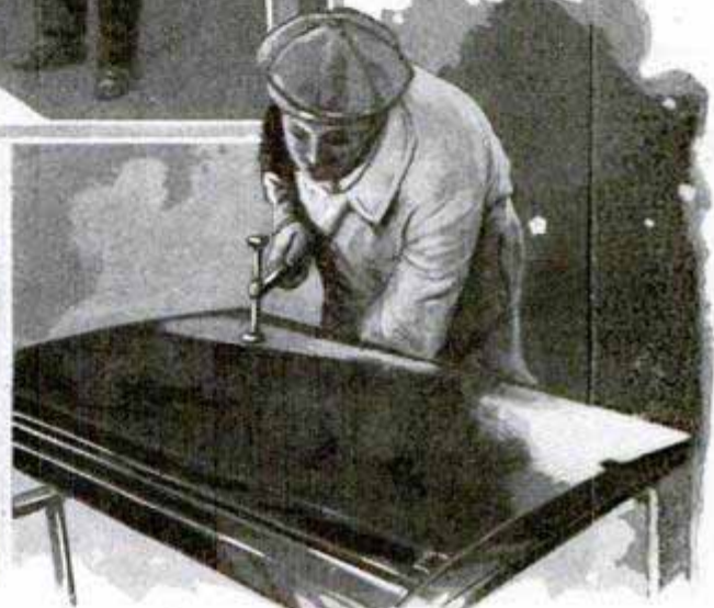
When Car Panels or Other Parts Are Badly Dented, the Metal Can Be Shrunk by Heat Treatment before Pounding Out to Prevent Wrinkling and Bulging
