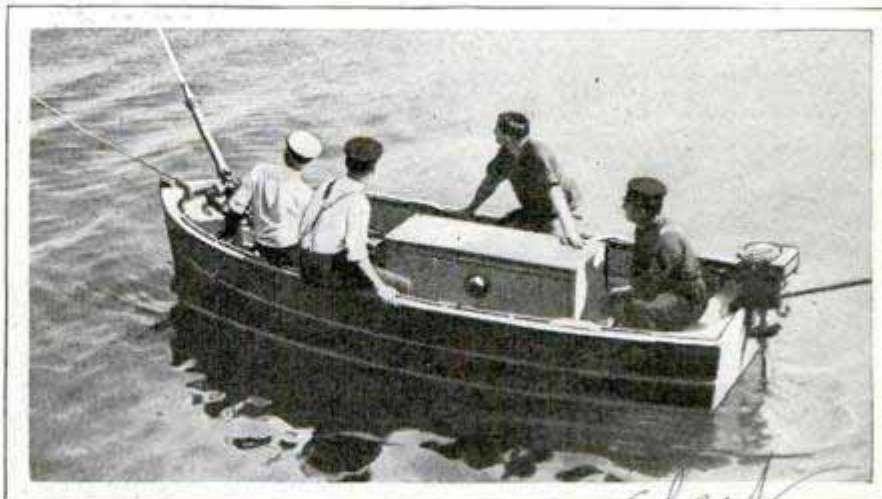
Tiny Fireboat Which Has Been Found Highly Useful in Boston in Fighting Pier Blazes Which Often Are Almost Inaccessible
