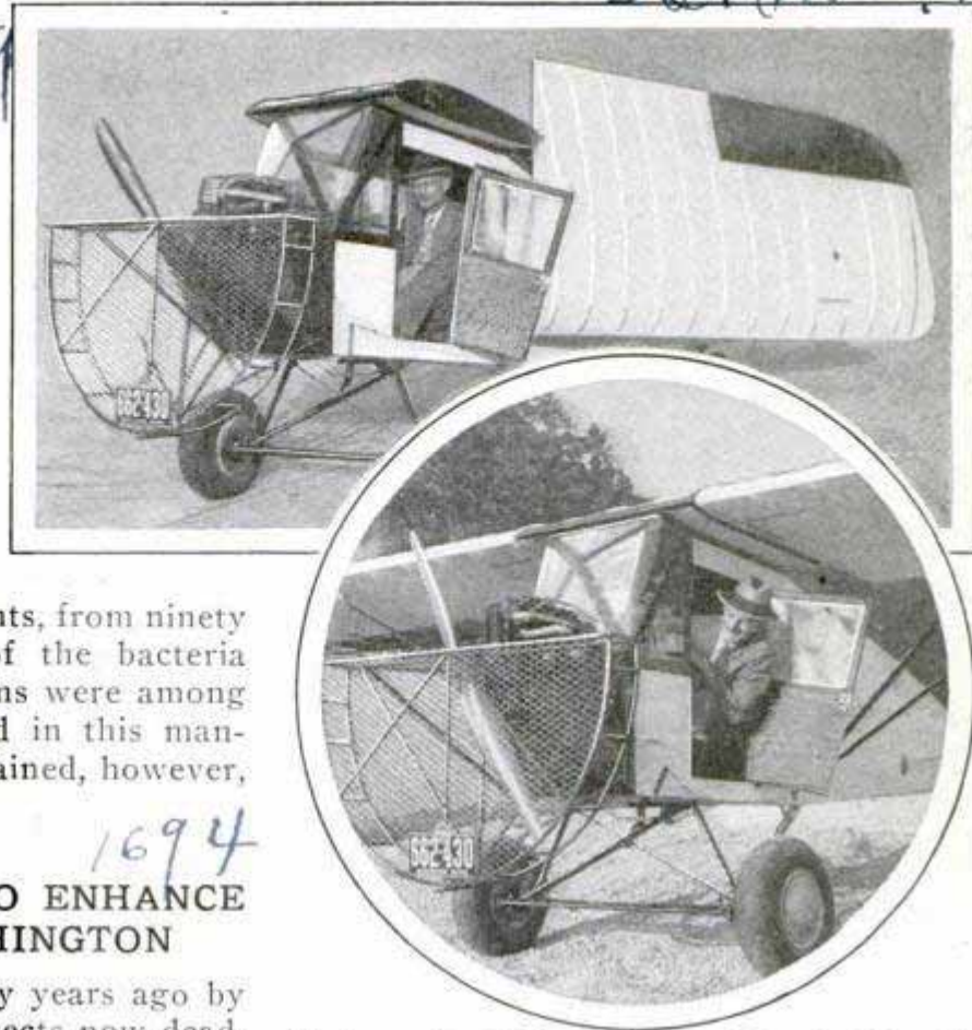
Airplane with Folding Wings and Guarded Propeller to Travel on Ground or in the Air
