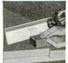
Saving shoulder of half splice joint with ATKINS Silver Steel Back Saw No. 2.
