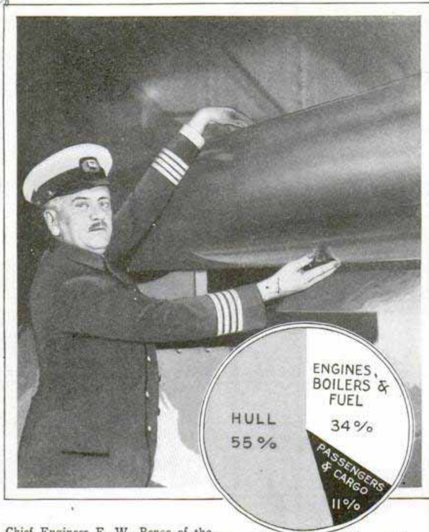
Chief Engineer E. W. Bence of the U.S.S. "California," Showing Size of Propeller Shaft, and, Inset, Diagram Illustrating Distribution of Weight in a Liner of 60,000 Tons' Displacement
