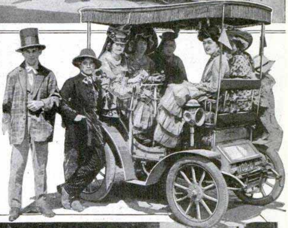
Above, a Modern Locomotive beside a Tiny Buddicum Engine, Built in 1840 and Which Has Been in Service between Granville and Paris for Seventy-Five Years; at Right, an Early Model of the Automobile; Its Top Is Borrowed from the Horse-and-Buggy Days; Note the Smaller Front Wheels and the Steering Grips Operated from the Right Side; Remarkable Improvements in Design Constitute One of the Chief Triumphs in Motor-Vehicle Progress, a Development Second Only to the Gain in Mechanical Efficiency of Engines and Other Parts
