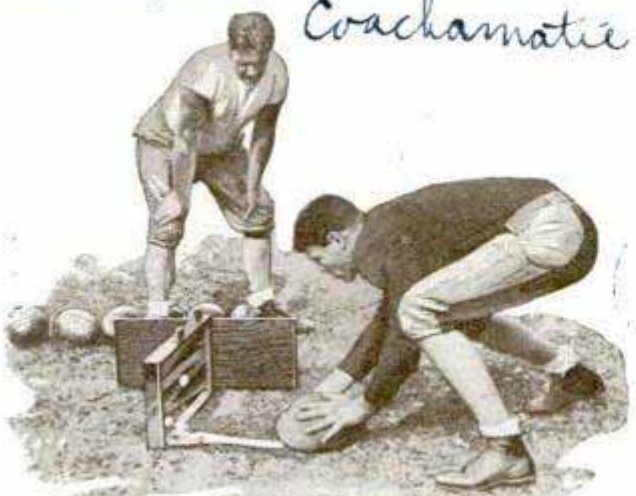
Football Timer Which Rings a Bell Two Seconds After the Ball Has Been Snapped by Passer
