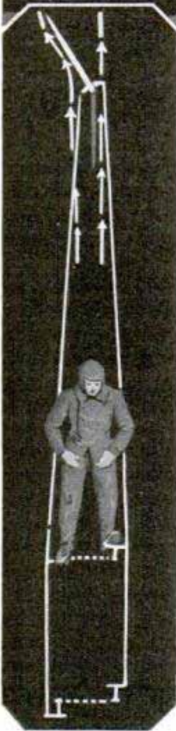
© Standard Oil Co. of Indiana Diagrams of Plane Showing What Happens to the Rudder When Its Pedals Are Pushed; in This Case Right Rudder Is Being Applied
