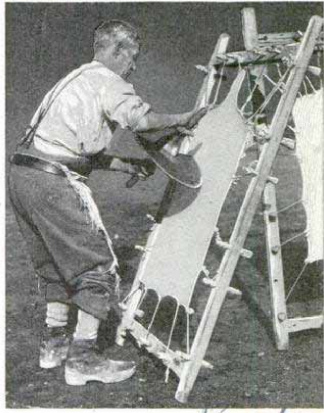
Dry-Shaving a Sheepskin in Making Parchment; the Process Is the Same as Was Used Centuries Ago
