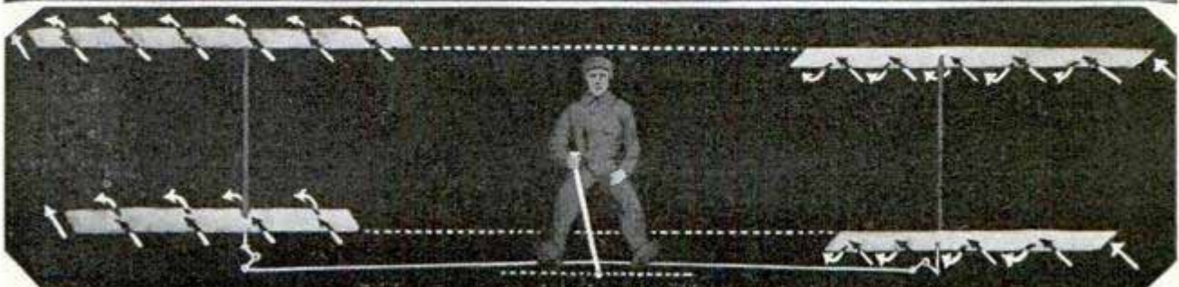
What Happens to the Ailerons When the Stick Is Moved to the Side; in This Case, Movement of the Stick to the Right Is Banking the Plane for a Right Turn
