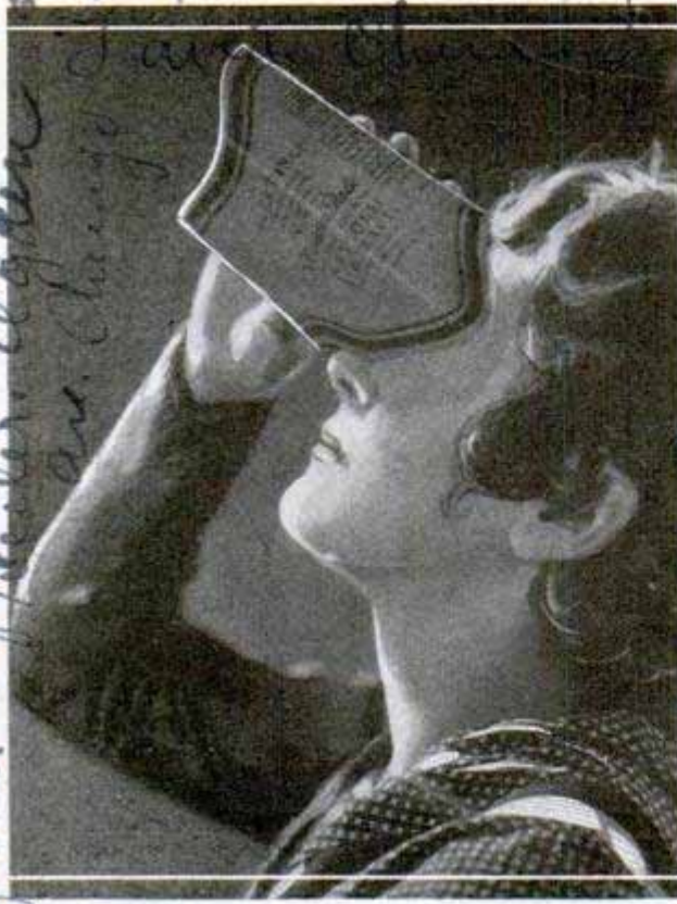
Cardboard Glare Shield Which Protects the Eyes from Bright Background While Watching Planes
