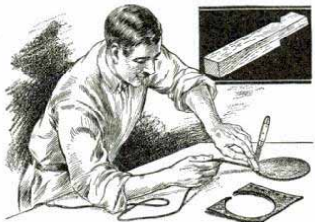
Disk of Leather, a Short Piece of Wood and a Knife Are All That Is Necessary to Make Neat Lacing
