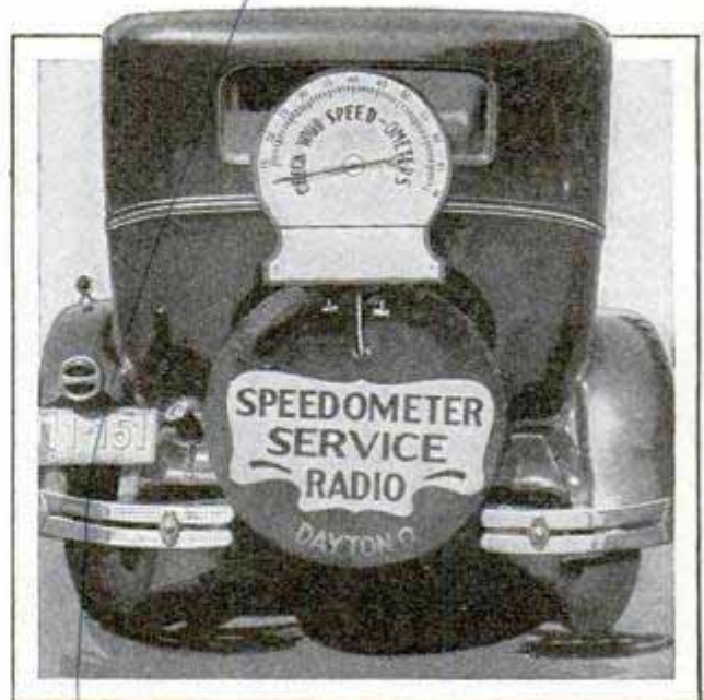
This Large Speedometer on Rear of Auto Enables Other Drivers to Check Their Speed and Instruments
