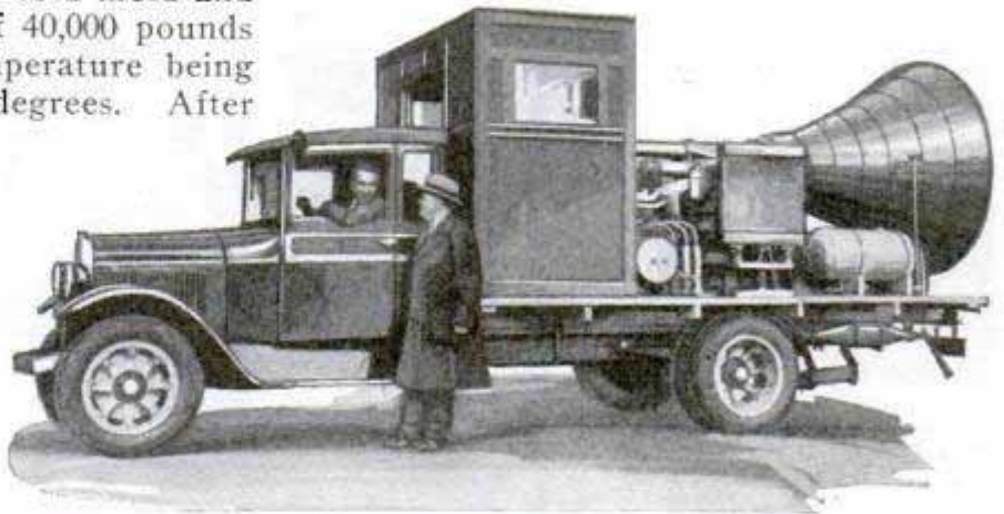
Loud Speaker with a Four-Mile Voice Mounted on a Truck; the Truck Actually Constitutes a Complete Broadcasting Station
