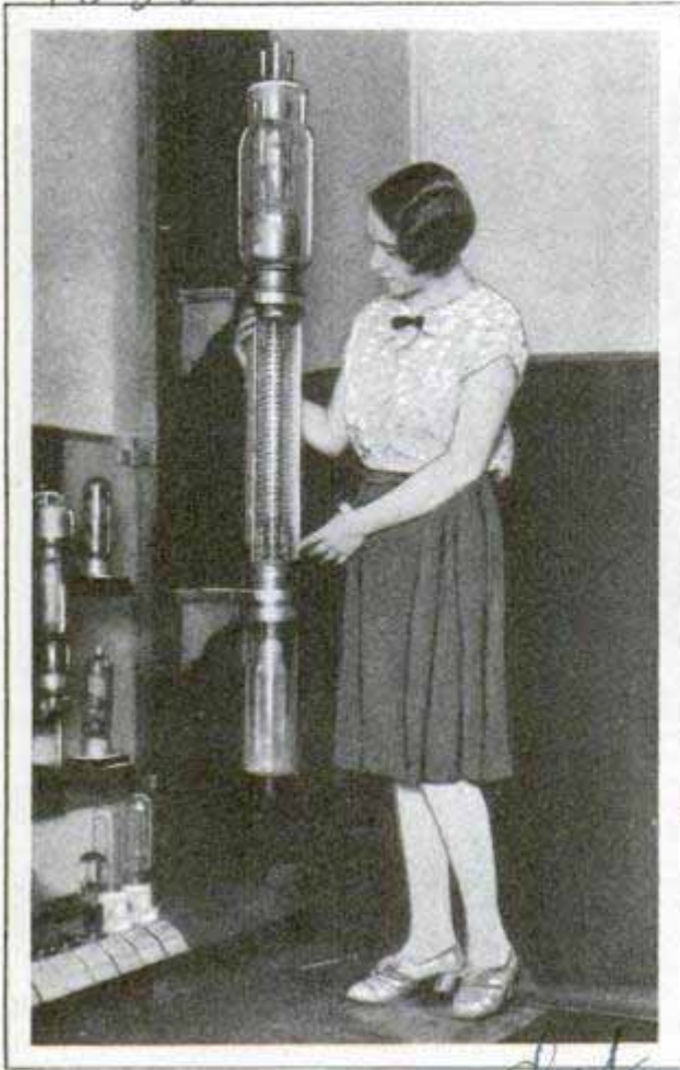
Giant Radio Tube for Broadcasting Which Requires Five Tons of Water an Hour for Cooling
