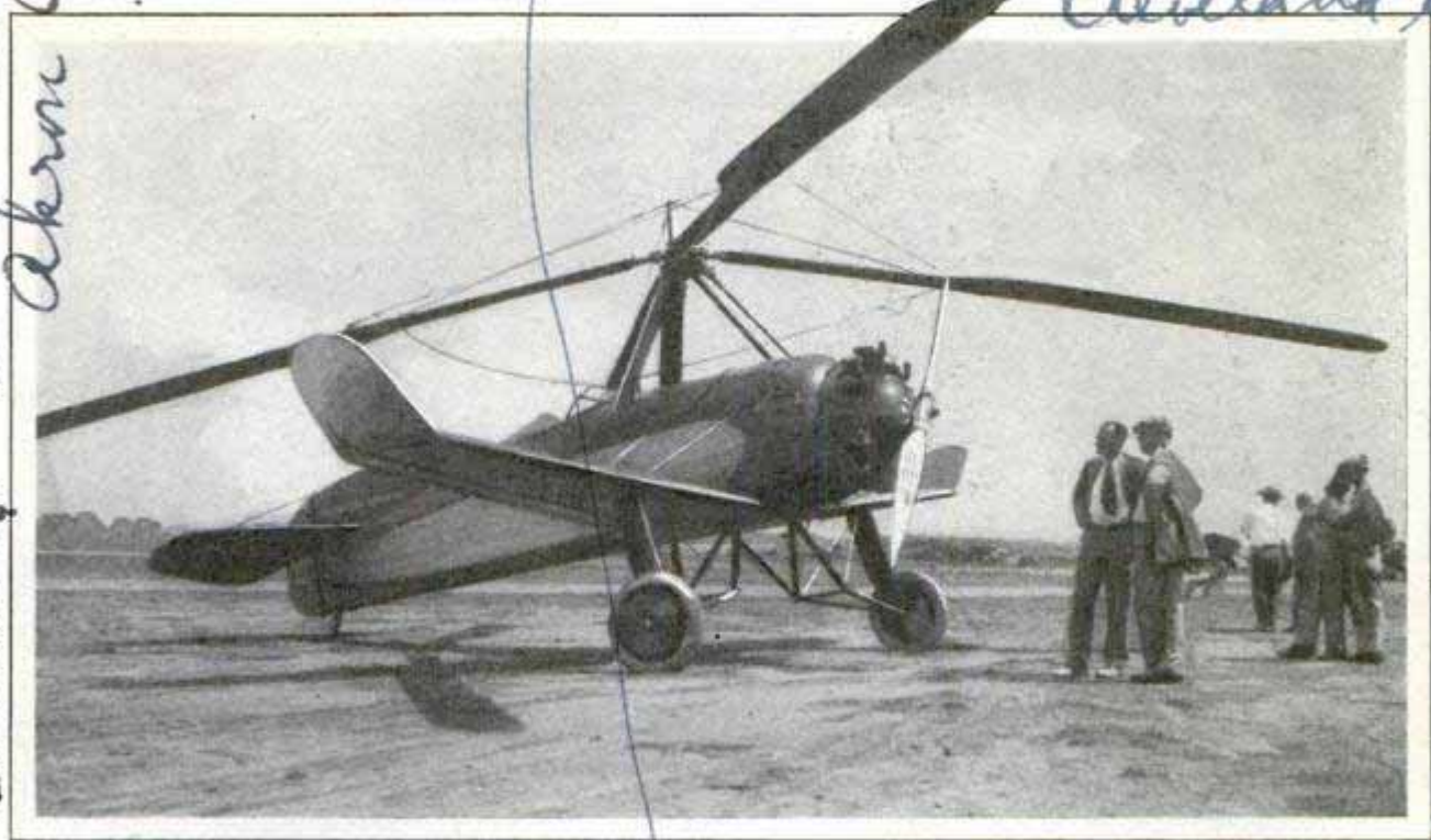
One of the Latest Model Windmill Planes Demonstrated at the National Air Races; Some of Them Now Have a Clutch Permitting the Engine to Whirl the Vanes at the Take-Off
