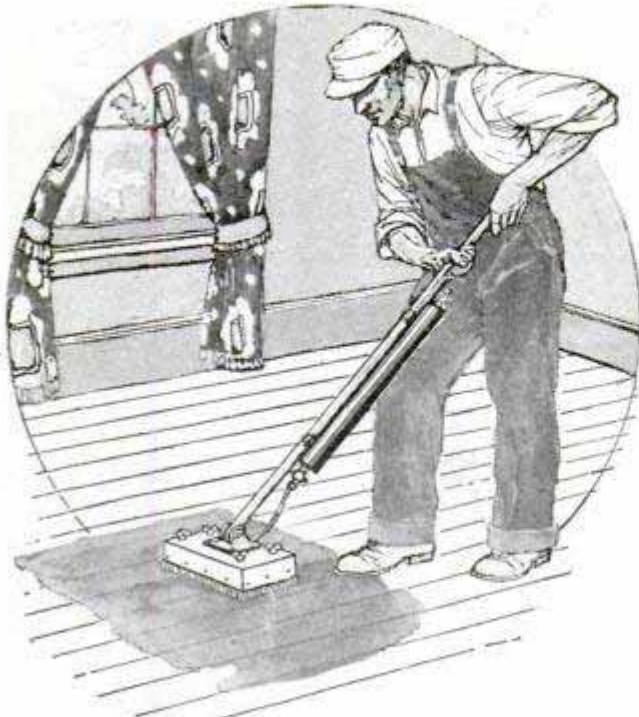
This Floor Oiler Lightens the Task and Also Affects a Considerable Saving in the Oil Applied
