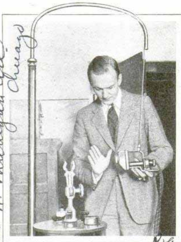
Water-Cooled Violet-Ray Lamp Used with Stencil to Tan Names on Backs of New-Born Babies
