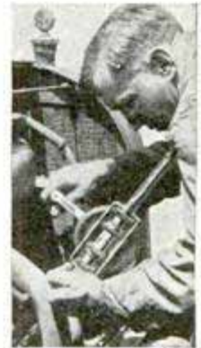
Any movement of crank, forward and back, no matter how slight, causes drill to cut continuously.
