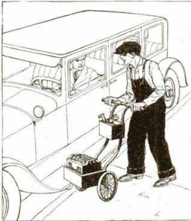
A Battery-and-Tool Truck for the Service Station Is Highly Convenient
