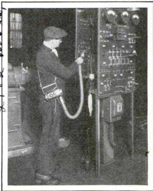
Portable Vacuum Cleaner Slung from the Shoulder; It Also Can Be Employed as a Blower
