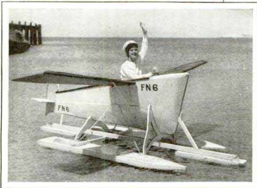
Waterplane with Stubby Wings Which Is Towed behind a Speedboat; When Sufficient Momentum Is Gained, the Craft Rises from the Water
