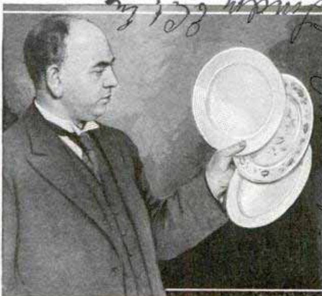
Samples of Lightweight Unbreakable Plates, Which Have Been Made Entirely from Cotton
