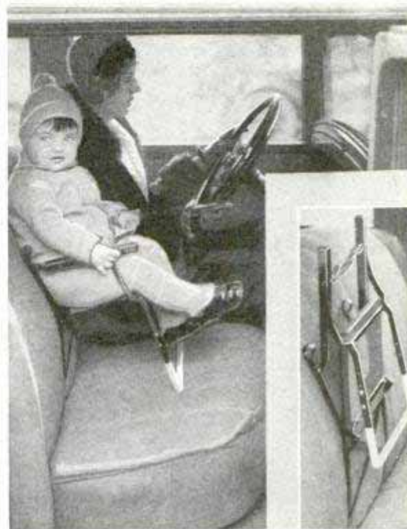
An Auto Chair for the Baby; Insert Shows How It Can Be Folded When It Is Not in Use
