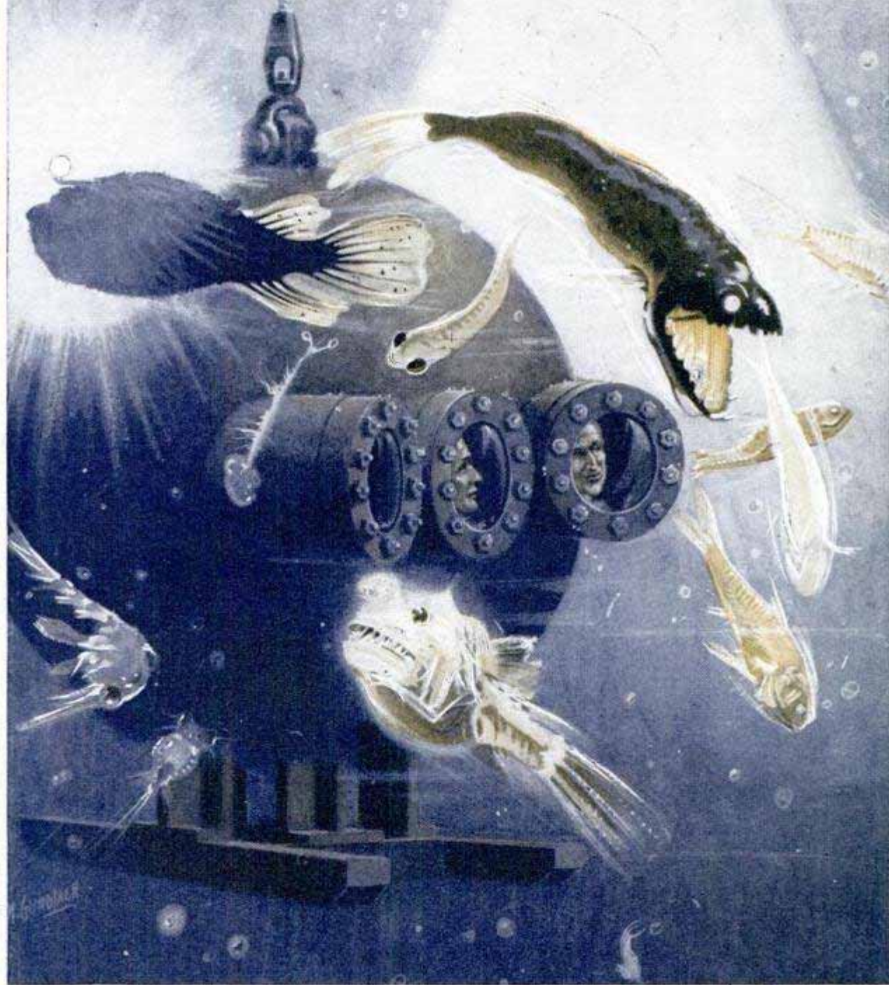
Two-Ton Steel Chamber, Six Feet in Diameter, in Which William Beebe and Otis Barton, His Assistant, Descended to a Depth of 1,426 Feet below the Surface of the Sea
