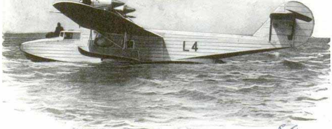
Two Views of Eight-Passenger Air Yacht Recently Completed in England for Service in Canada; Note the Design of the Hull and How the Wheels Are Folded Up under the Wings
