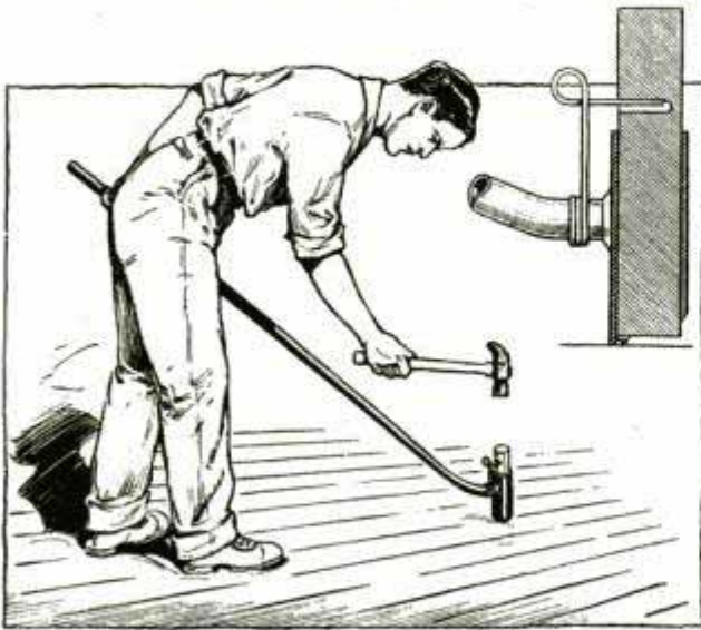
This Tool Detects and Hammers Down Dangerous Projecting Nails in the Floor
