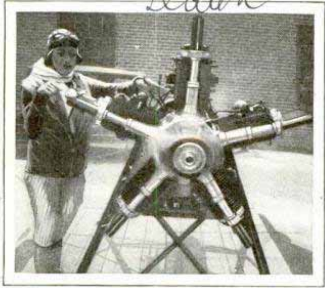
Testing the Vibration of an Airplane Motor with an Egg in a Spoon Clamped to the Engine
