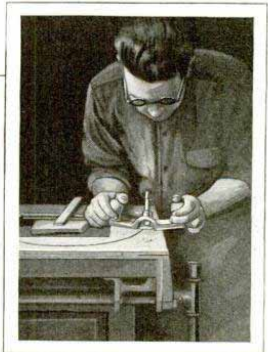
Top. Scribing the Groove; Bottom, Right, Cutting Groove with Router; Left, Clamping the Wood to the Caul
