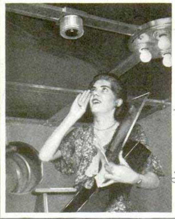
Microphone in Top of Bank Vault Which Sets Off a Police Alarm at Any Slight Noise
