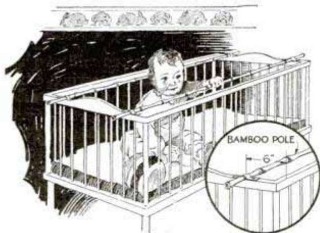
Two Bamboo Poles Lashed to the Crib Prevent Baby from Falling Out
