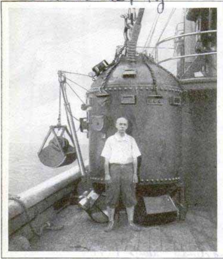
Diving Bell Large Enough to Hold Three Persons; It Is to Be Used in Salvaging the Cargo of a Wrecked Ship
