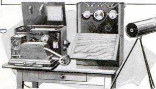
Car-Timing Apparatus Set Up for Clocking a Race, and Close View of the Apparatus
