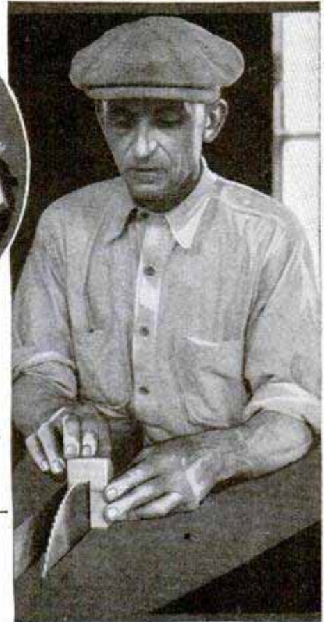
Above, Cutting the Semicircular Groove in Block B on the Circular Saw; Below, Placing an Opened Pack on the Ledge in the Groove
