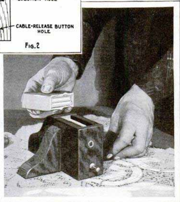
Above, Cutting the Semicircular Groove in Block B on the Circular Saw; Below, Placing an Opened Pack on the Ledge in the Groove
