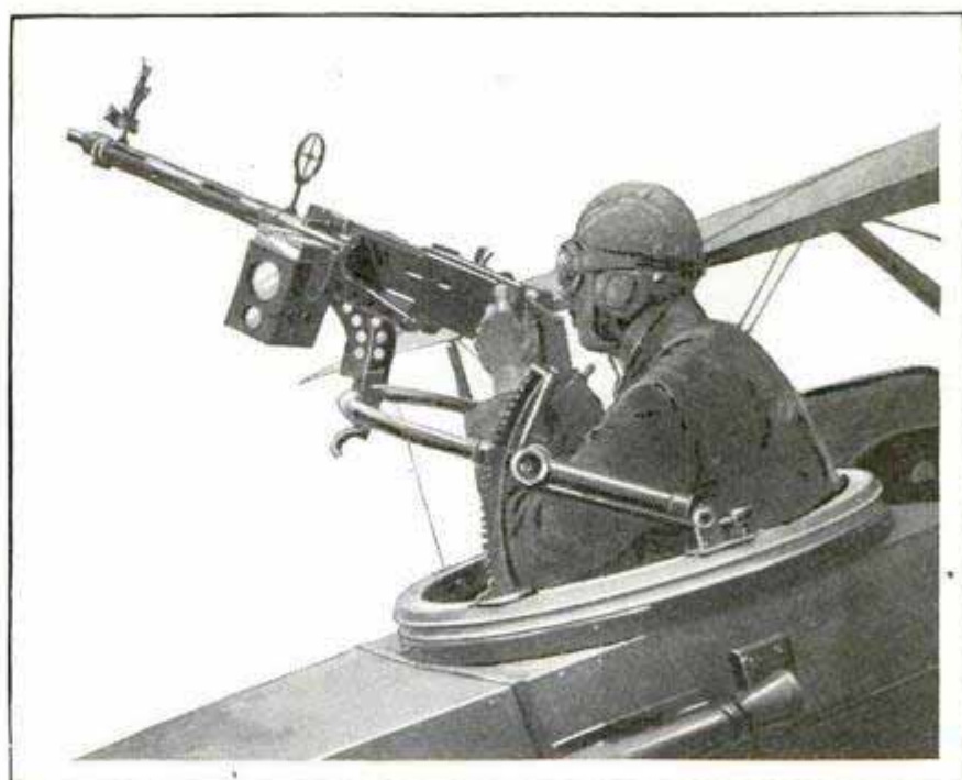
Rapid-Fire, Air-Cooled Machine Gun Mounted in Cockpit of Airplane; It Is Capable of Firing from 600 to 800 Rounds a Minute
