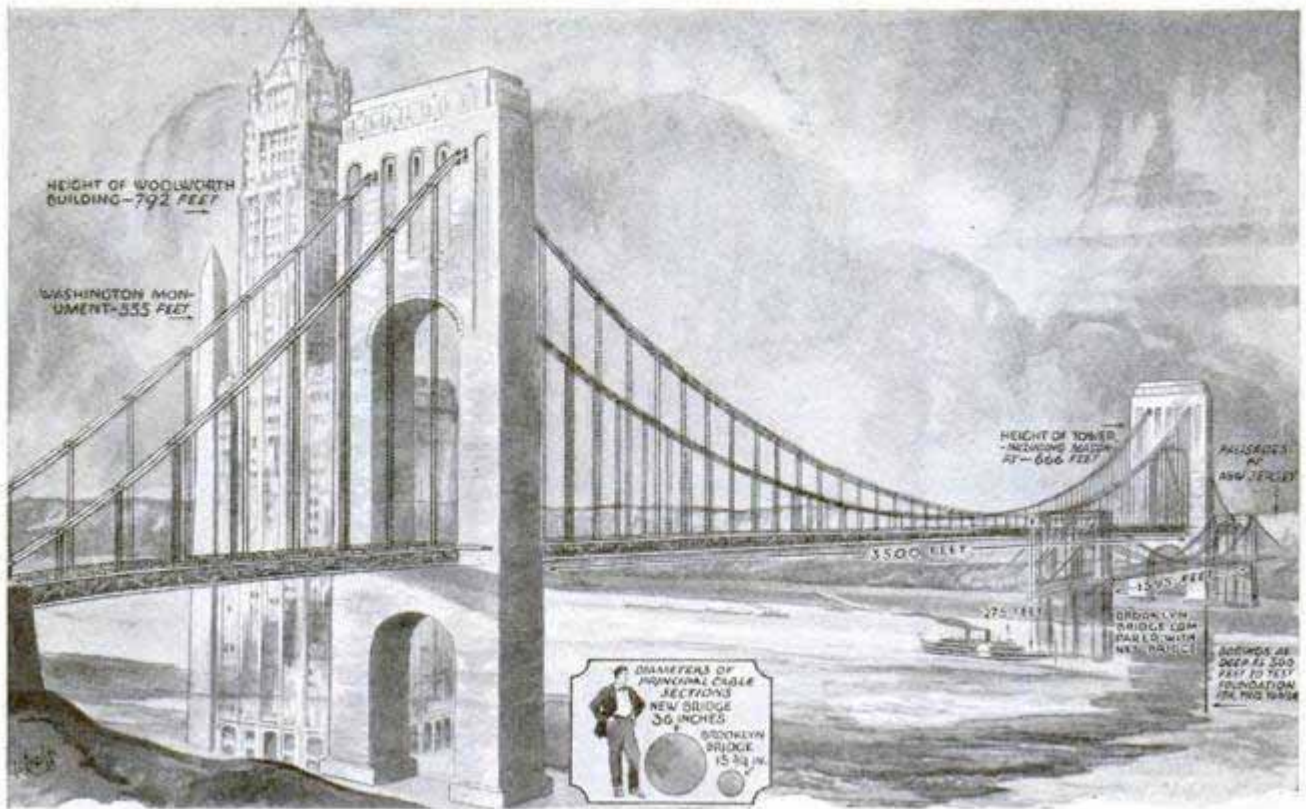
Artist's Drawing of the New Hudson River Bridge, Now under Construction, Compared with Other Famous Structures; Note Comparative Size of Brooklyn Bridge
