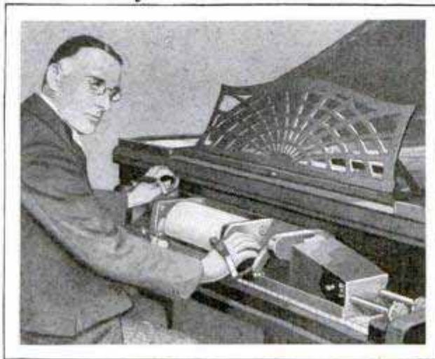
Inventor with Player Unit That Is Adjusted on Top of Piano Keys for Automatic Operation
