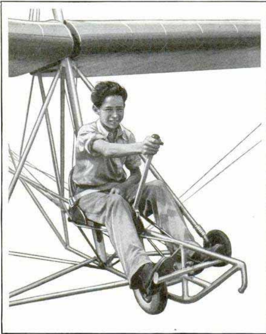
Demonstrating Proper Position for Flight in Primary Training Glider; Steering Is Done with Feet through Rudder Controls
