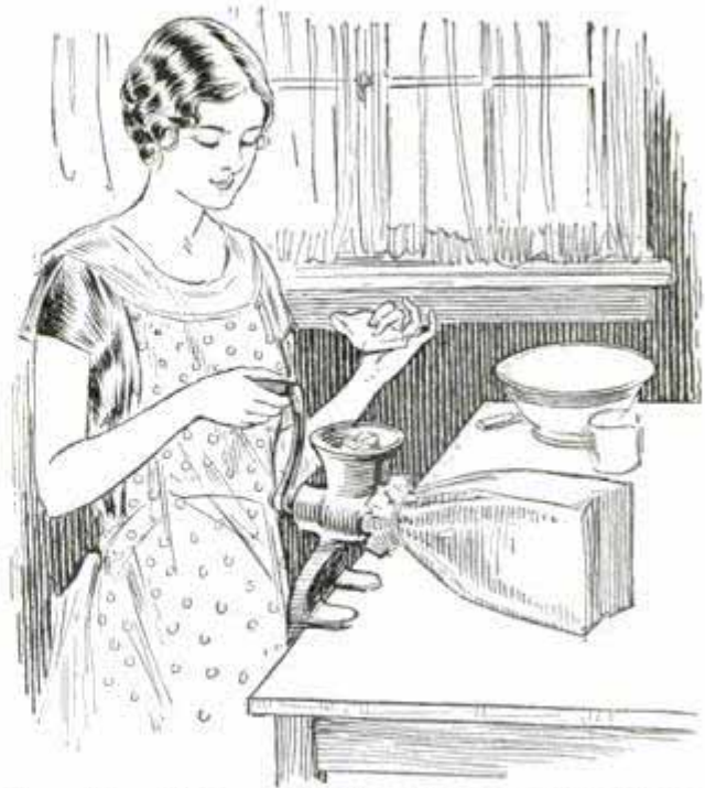
Paper Bag Tied over Mouth of Food Grinder Catches the Crumbs
