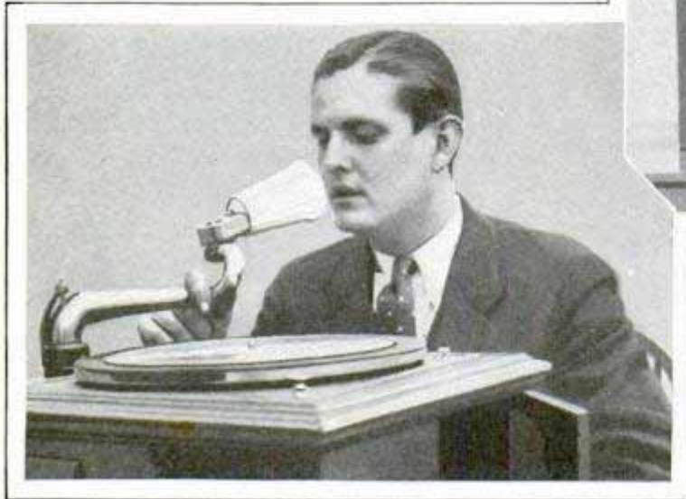
Left, Phonograph Pick-Up Employed as a Microphone; Above, Sound Effects Produced by Holding Loud-Speaker Microphone Up to Set Speaker
