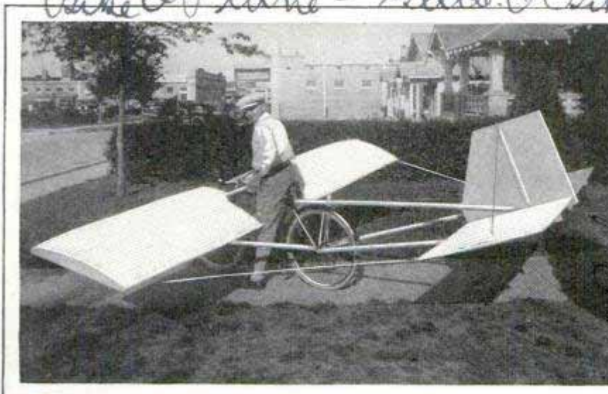
Bicycle Equipped with Glider Wings and a Tail; the Wings Lift the Front Wheel off the Ground When the Wheel Is in Motion
