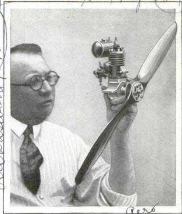
Miniature Gas Engine for Operating Model Planes or Boats; It Comes Ready for Assembling
