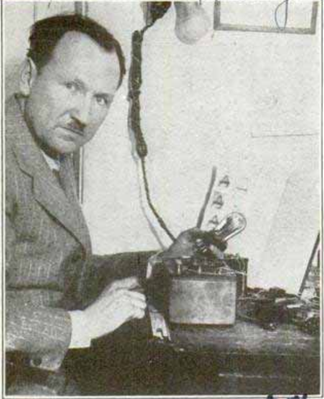
Humless Alternating-Current Tube That Eliminates Much of the Noise of Electric Radio
