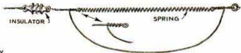
Small Choke Coils Suitable for Modern Circuits May Be Conveniently Mounted on Short Metal Brackets; Below, Screen-Door Spring Used to Take Up Antenna Strain; the Wire Loop Prevents the Antenna from Falling if the Spring Breaks
