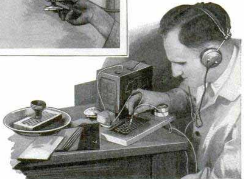
Driving Hacksaw through Steel Bar; Testing Rubber Fabric's Waterproof Qualities, and Electrical Test on Paint; the Needle Makes an Electrical Contact if Paint Has Cracked on Metal
