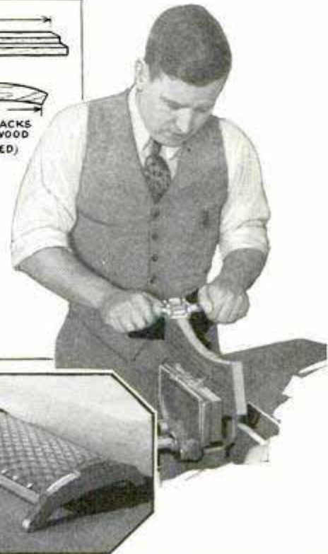
Lower Left, Footstool, Upholstered in Tapestry; Right, Finishing a Curved Surface with the Spokeshave
