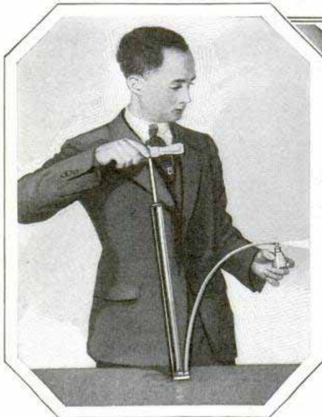
Auto Pump and Perfume Atomizer Make a Good Improved Spray Gun for Painting and Stenciling
