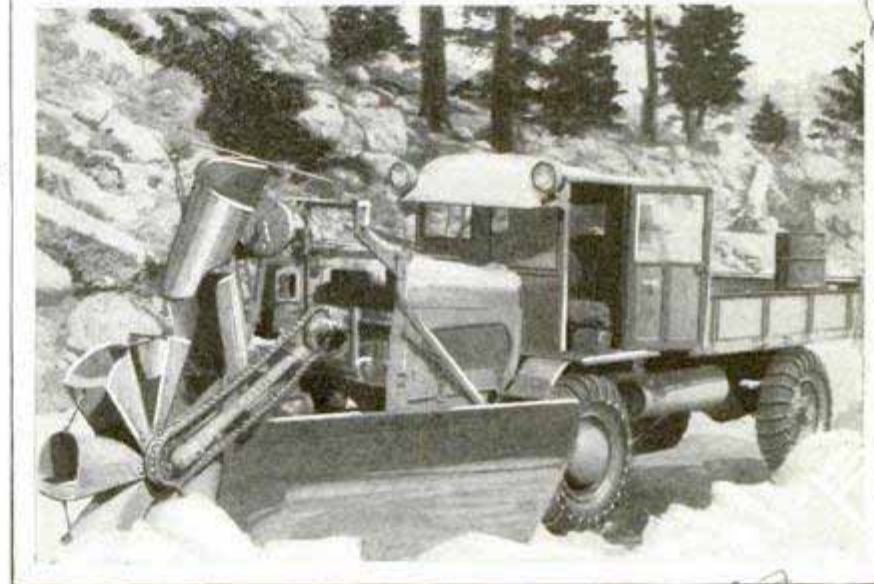
Rotary Snowplow Which Is Attached to Front of Four-Wheel-Drive Truck; It Makes Better Speed Than Tractor-Driven Plows
