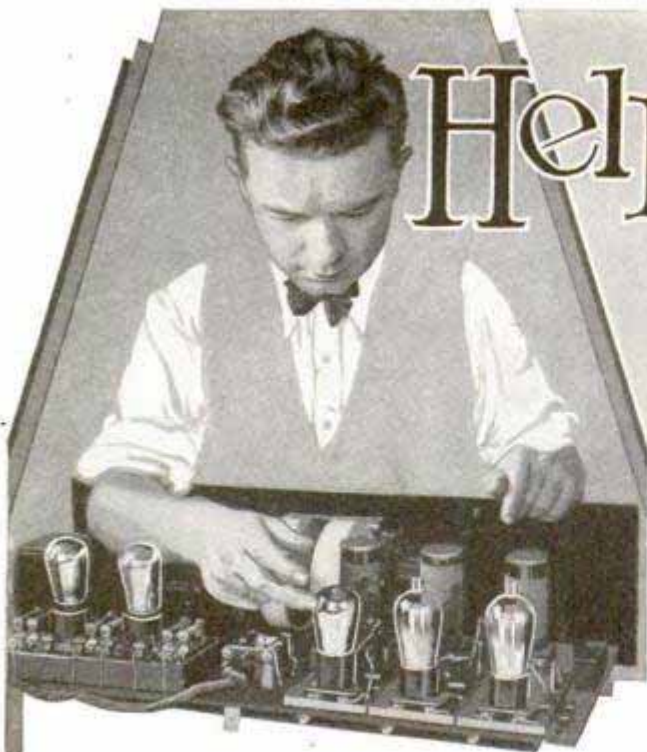
Noisy Microphonic Tubes Are Easily Located by Lightly Tapping Each Tube While the Receiver Operates
