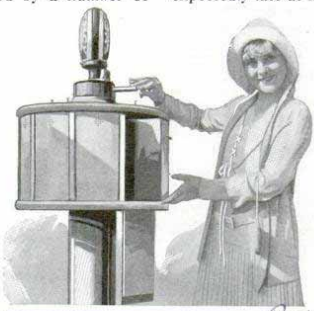
Automatic Gasoline Vender Which Dispenses a Gallon Can of Fuel When Coin Is Dropped in Slot
