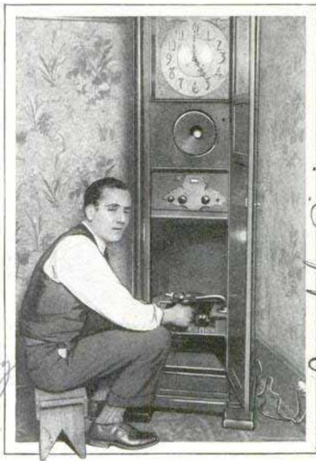
Talking Clock That Speaks the Hours and Half Hours; It Also Contains a Radio and Phonograph
