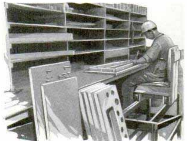
Seat on Rollers That Will Slide along the Entire Length of the Workbench
