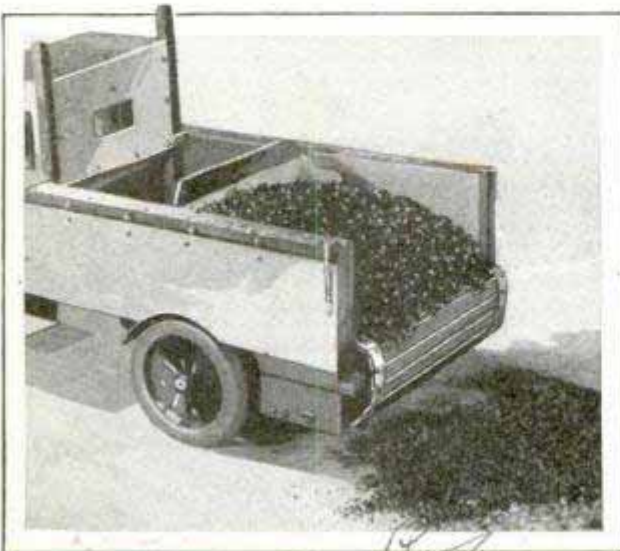
Truck with Flexible Flooring on Endless Conveyor, Which Loads and Unloads Automatically
