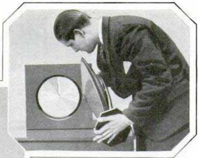
Left, Phonograph Pick-Up Employed as a Microphone; Above, Sound Effects Produced by Holding Loud-Speaker Microphone Up to Set Speaker
