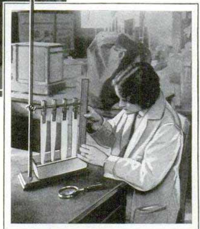
Measuring Effect of Synthetic Sunshine on Paint Samples, and Testing Absorption Qualities of Cloths; Conditions of Natural Exposure Are Accurately Duplicated
