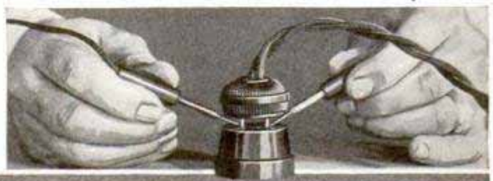
Left, a Pendant Switch and a Length of Lampcord Extending from the Radio Receiver to the Telephone Form a Time and Patience-Saving Device, As It Is Usually Necessary to Turn Off the Set When the Phone Is in Use; the Switch Is Merely in Series with One Lead of the A-Battery or in One Side of the A.C. Supply Line to the Set; Below, Taking A.C. Line-Voltage Reading with Meter Equipped with Test Prods; Partly Withdraw Attachment Plug from Wall Socket as Shown
