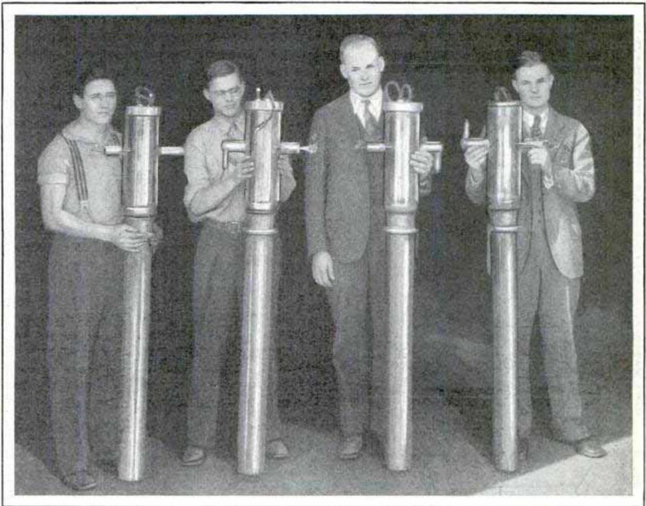
Battery of 100-Kilowatt Radio Tubes; Six of These, in a Recent Test, Transmitted a 200-Kilowatt Long-Wave Broadcast, Which Was Heard West of Hawaii
