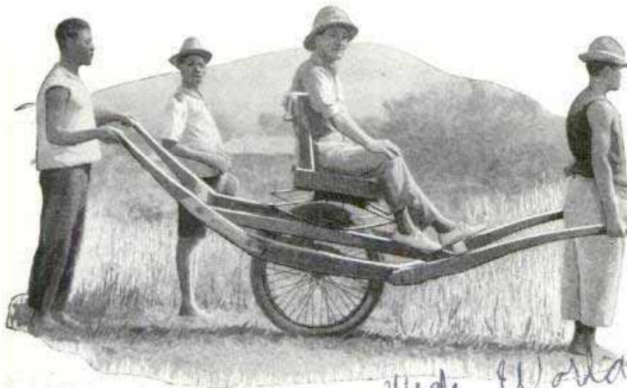
Single-Wheeled Bush Chair with Double Shafts Used for Taxi Service in Parts of Africa Served Only by Rough Trails
