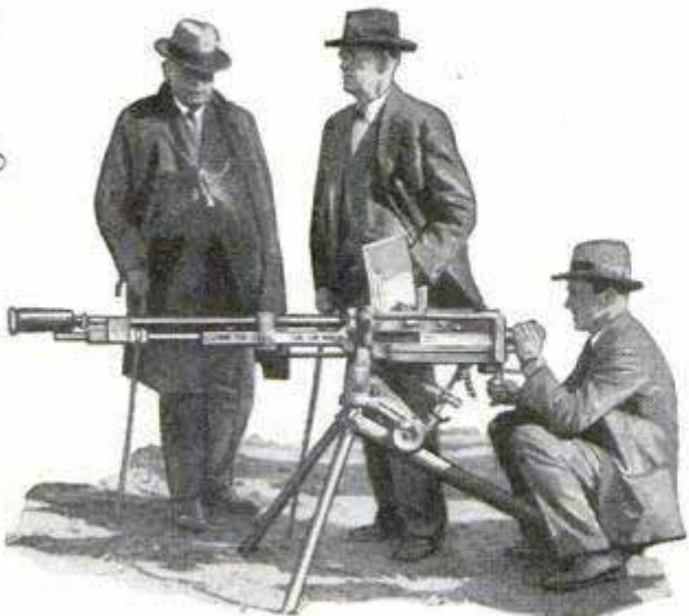
Machine Gun That Shoots Fifty-Caliber Bullets at the Rate of 800 a Minute for Nine Miles
