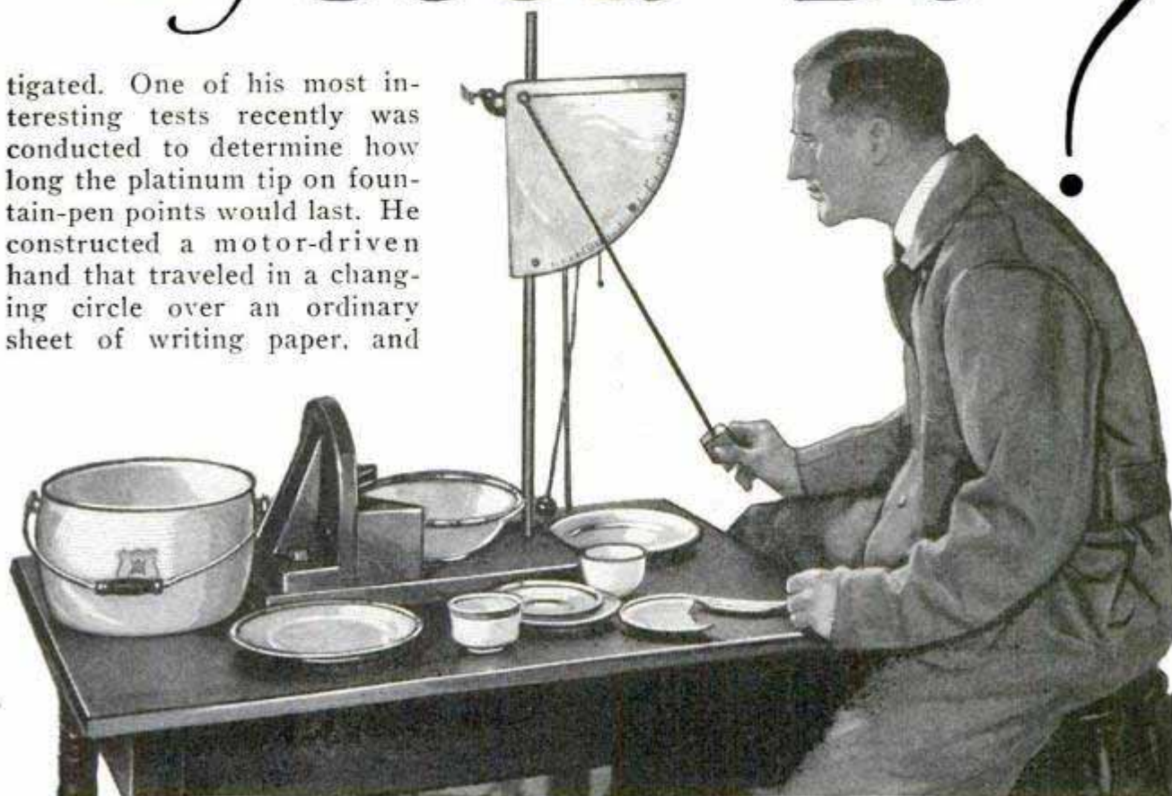
How Durable Are Dishes? With This Swinging Weight, the Tester Can Determine the Strength of Blow Required to Shatter Plates, Bowls and Other Dishes
