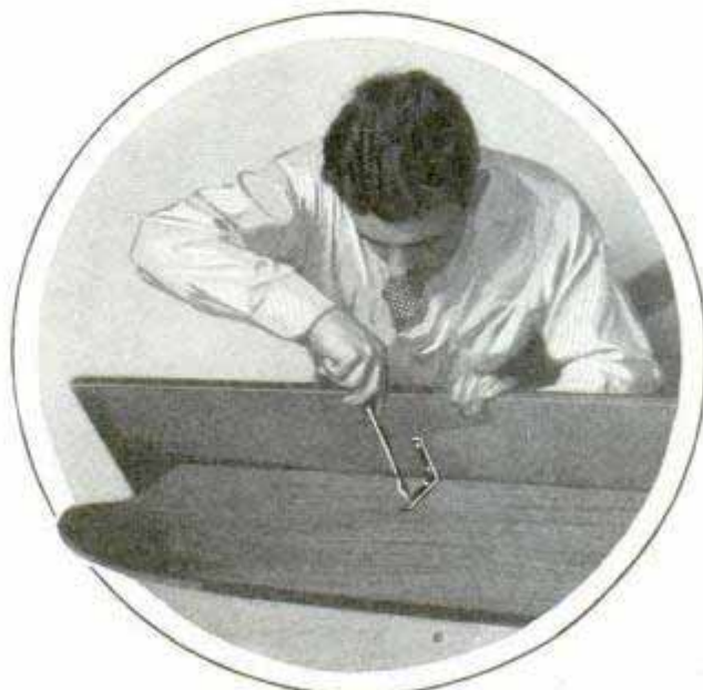
Fig. 2. In Addition to Screwing the Centerboard to the Deck, It Is Strengthened by Angle Brackets
