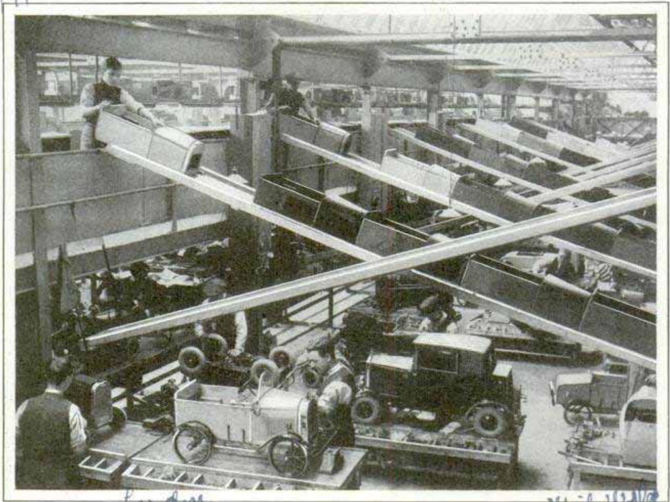
London Toy Car Factory in England Which Has Applied American Methods of Automobile Production; Conveyors Carry the Autos to Workmen Who Turn Them Out at the Rate of a Thousand a Day Wide World
