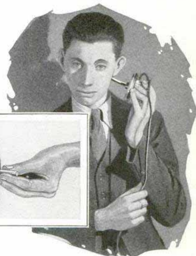
Insert Shows Short Stick Cemented to Diaphragm; Right, Station JAW Broadcasting
