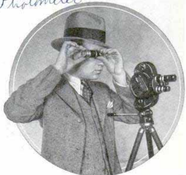
Looking into a Photometer Which Measures Light Intensity on a Subject to Be Photographed
