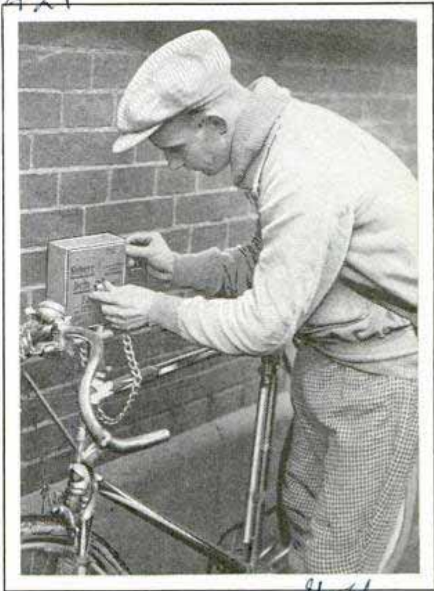
Coin-in-Slot Bicycle Lock; the Owner Deposits a Coin and Receives the Key to the Lock
