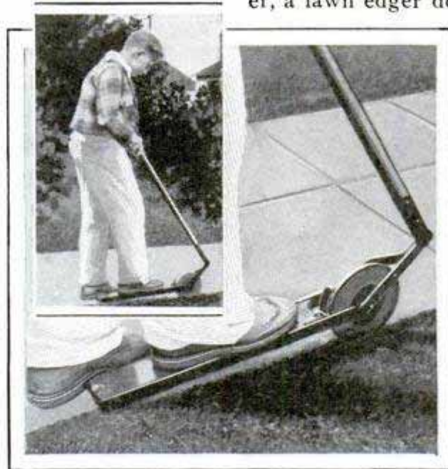
Lawn Edger, Shaped and Operated Like a Child's Scooter, Which Makes This Hard Task Easier
