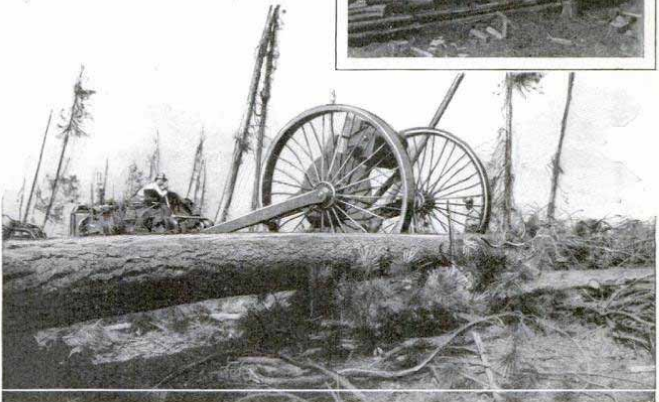
Spar Tree, to Which a Log Is Just Arriving by the High-Lead Method, and, Below, Another View of the Tractor-Powered High-Wheeled Rig for Snaking Logs Out of the Woods
