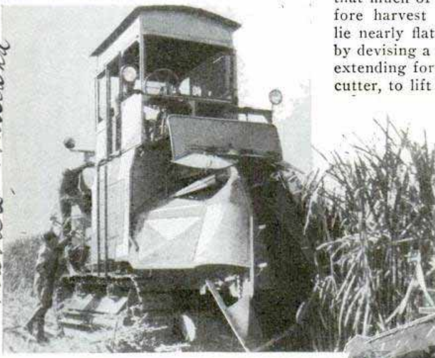
Two Views of Sugar-Cane Harvester That Cuts the Stalks, Strips Them of Leaves and Then Piles Them
