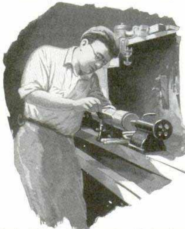
Laying Off Guide Lines on the Curved Surface of the Table Column
