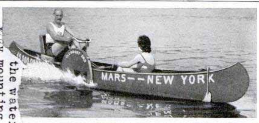
Fitted with Sidewheel Paddles, Handlebars and Pedals for Guiding and Propelling the Bicycle-Boat
