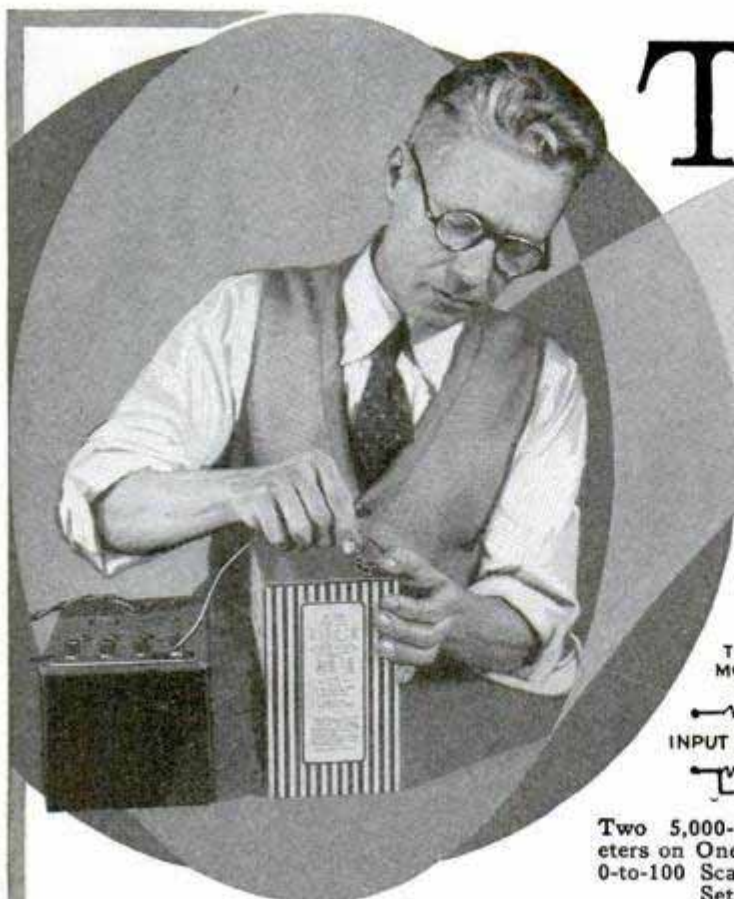
Connecting 45-Volt B-Battery in Series with a 90-Volt B-Eliminator to Obtain 135-Volt Output; Right, Copper Screen on Rear of Console Solves Antenna Problem in Apartment Buildings; Antenna Lead Is Soldered to Screen; It Provides Ventilation and Does Not Interfere with Speaker Operation
