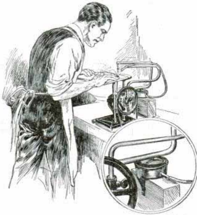
Improved Sawdust Blower for the Jigsaw Made from Powder Bellows
