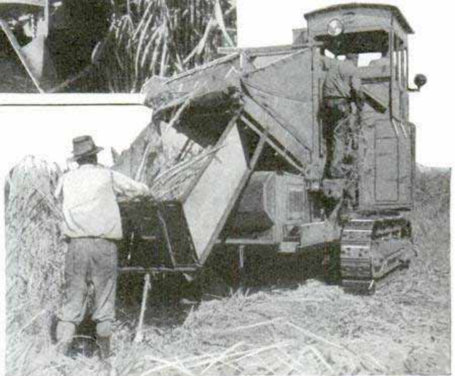
Two Views of Sugar-Cane Harvester That Cuts the Stalks, Strips Them of Leaves and Then Piles Them
