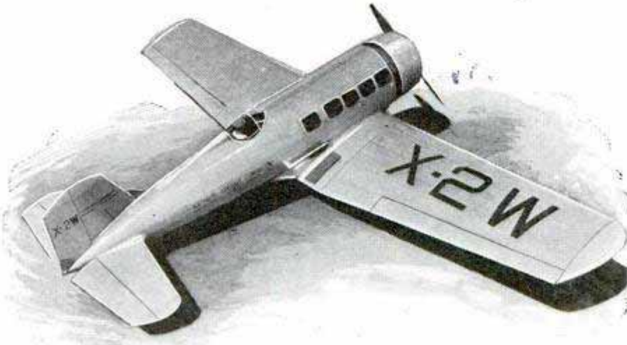
All-Metal, Low-Wing Cabin Monoplane, Whose 435-Horsepower Motor Develops a Cruising Speed of 150 Miles an Hour or More
